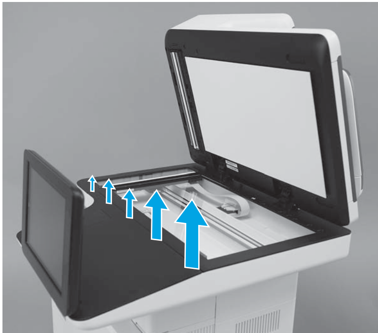
Figure 1-4984 Release five tabs
