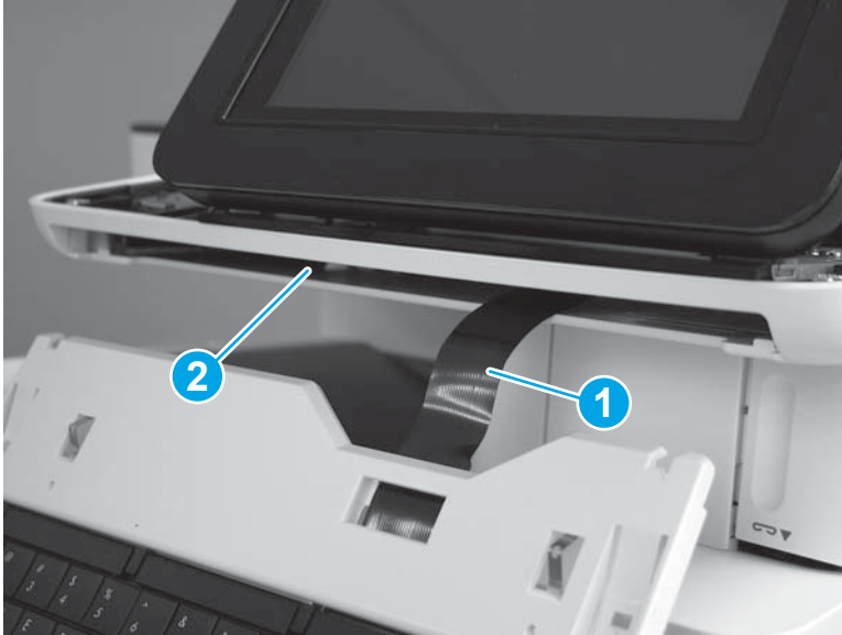
Figure 1-155 Install the flat cable through the slot
