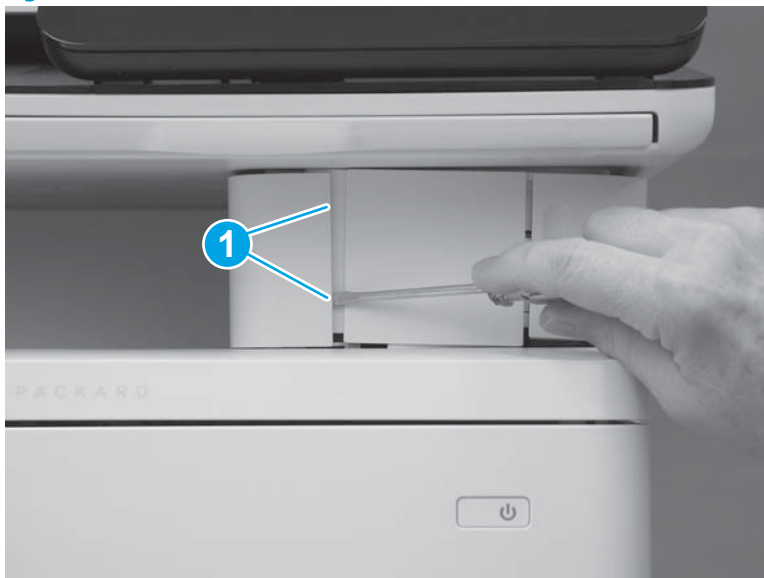
Figure 1-3972 Release two tabs
