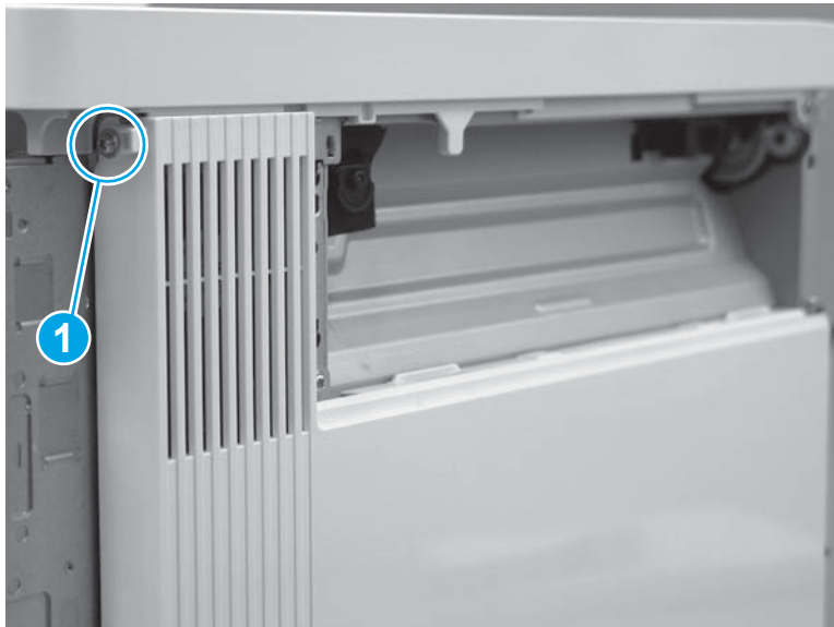
Figure 1-1390 Remove one screw
