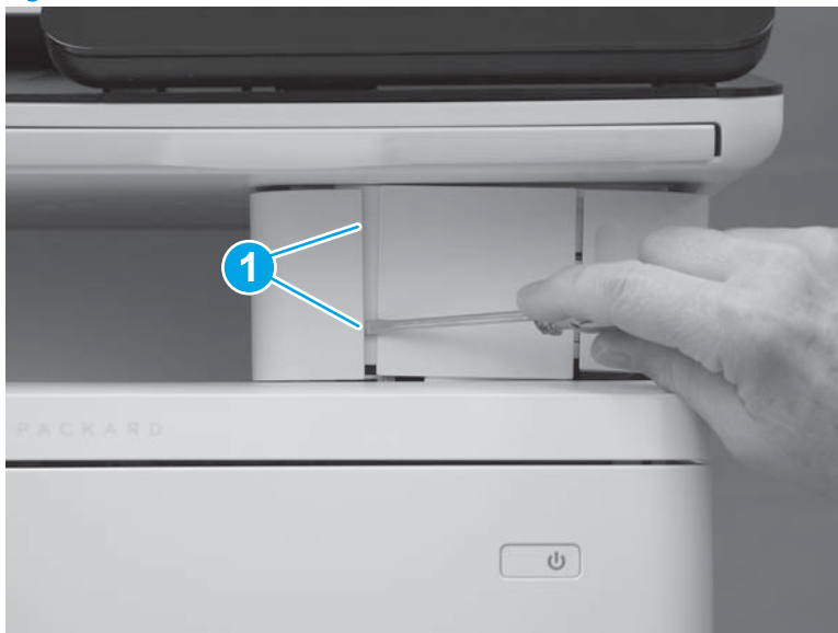
Figure 1-1973 Release two tabs
