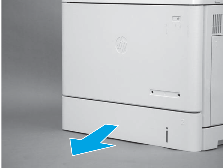
Figure 1-4424 Pull the tray out
