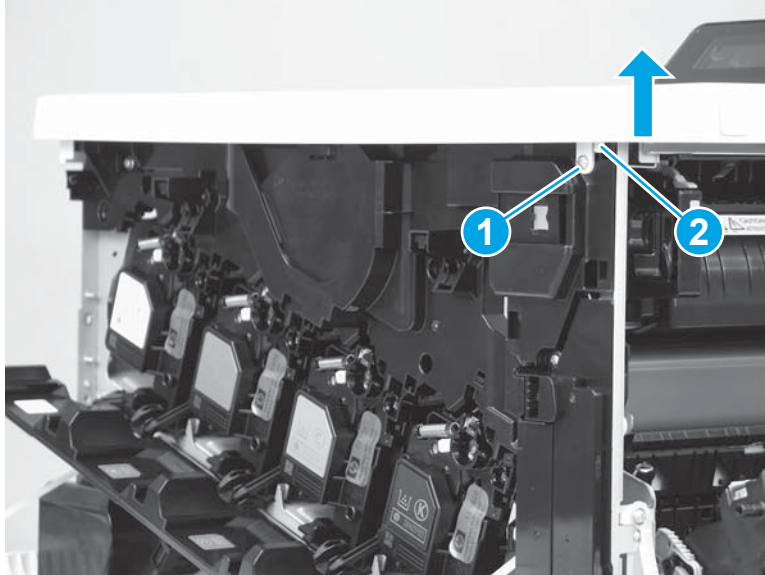
Figure 1-1023 Remove one screw and release one tab
