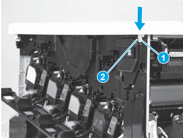
Figure 1-1299 Engage one tab and install one screw
