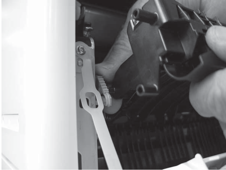
Figure 1-4413 Disengage the blue arm and pin
