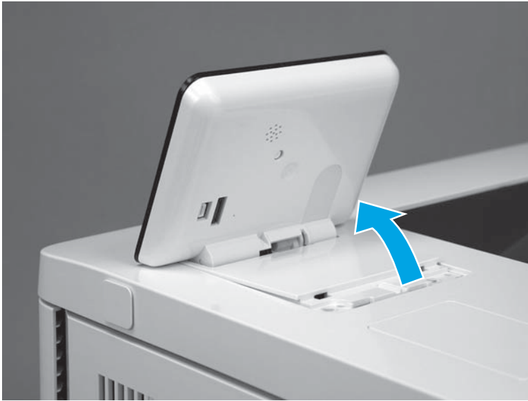
Figure 1-719 Rotate the control-panel base up
