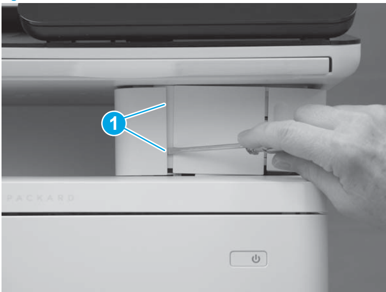
Figure 1-744 Release two tabs
