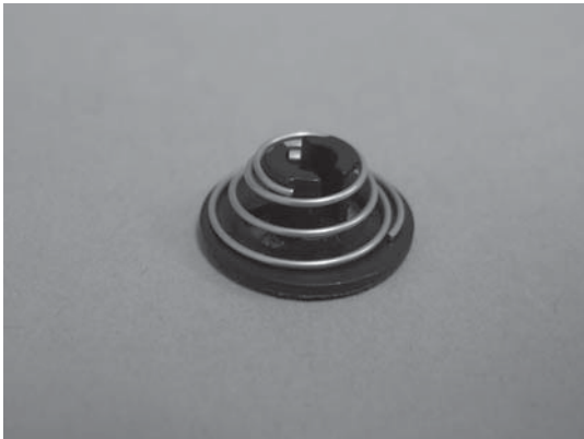
Figure 1-165 Check the retention clip spring
