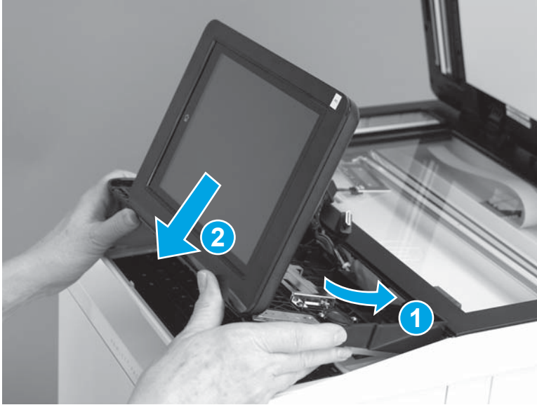
Figure 1-139 Install the control-panel
