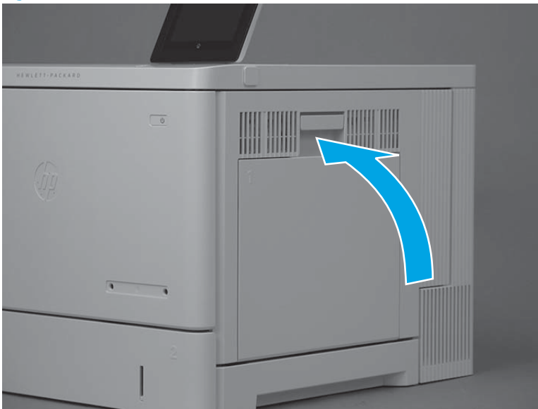
Figure 1-3481 Close the right door
