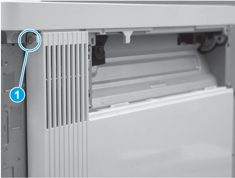
Figure 1-2140 Install one screw
