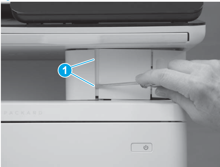
Figure 1-2972 Release two tabs
