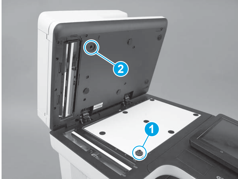
Figure 1-4987 Check the retention clips
