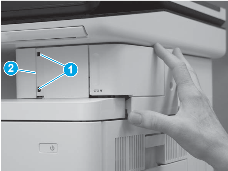
Figure 1-918 Install two tabs
