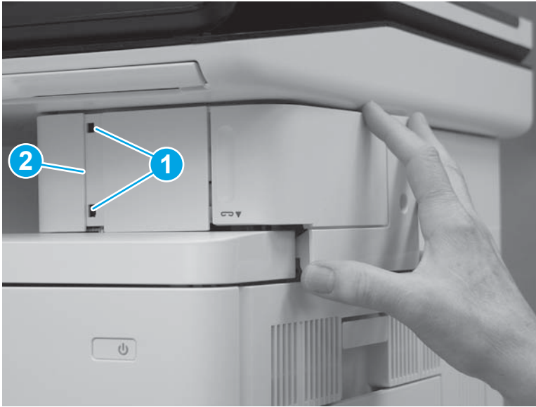
Figure 1-345 Install two tabs
