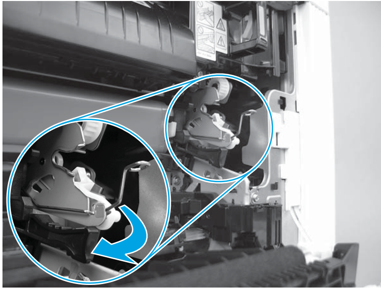
Figure 1-4639 Remove the spring from the holder
