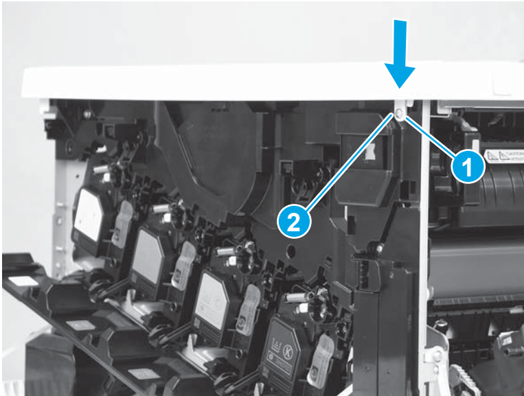
Figure 1-1511 Engage one tab and install one screw
