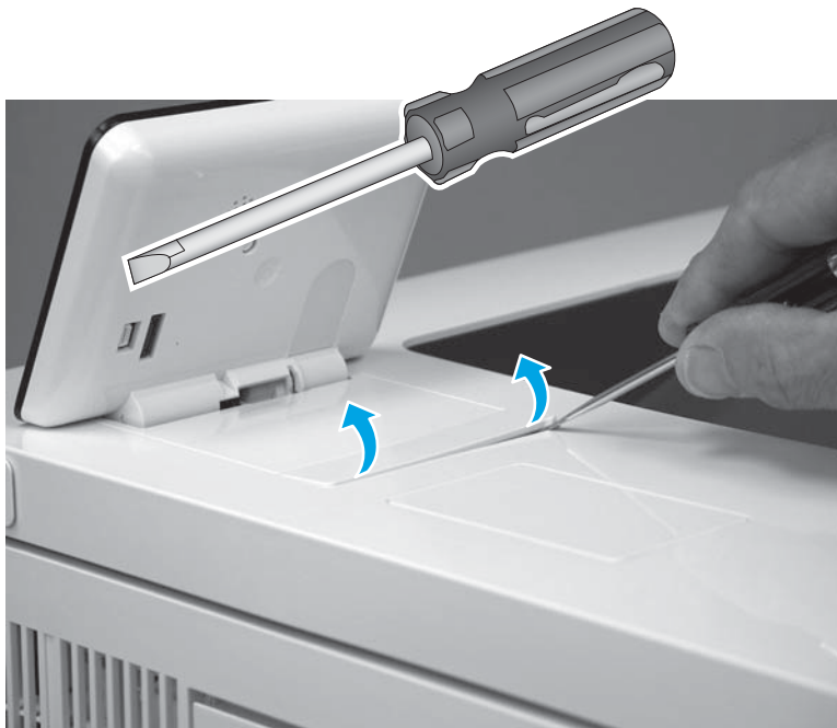
Figure 1-1197 Release the control-panel screws cover tabs
