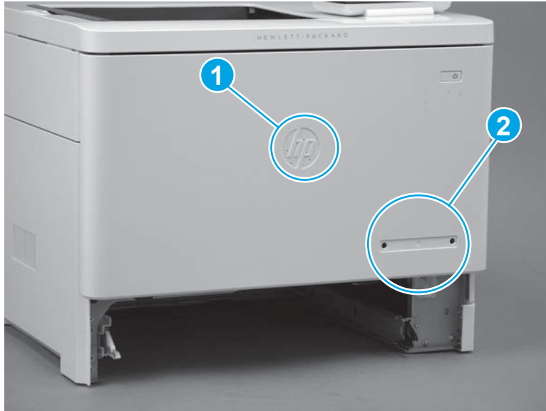
Figure 1-592 Install nameplate and HP jewel
