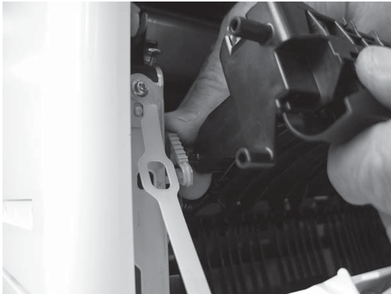
Figure 1-4150 Disengage the blue arm and pin
