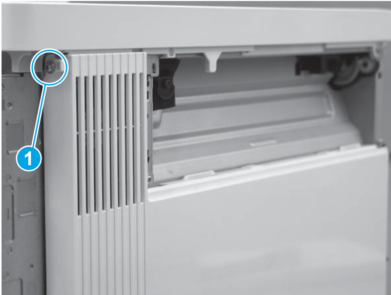
Figure 1-2426 Install one screw
