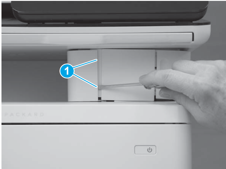
Figure 1-5016 Release two tabs
