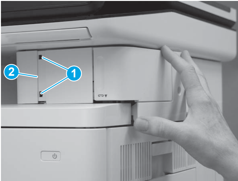
Figure 1-2042 Install two tabs
