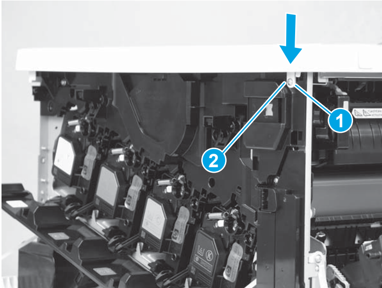
Figure 1-3408 Engage one tab and install one screw
