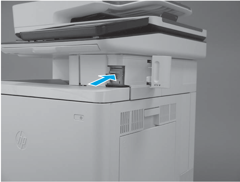
Figure 1-1334 Install the staple cartridge
