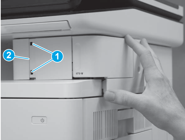
Figure 1-2564 Install two tabs
