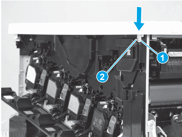
Figure 1-2543 Engage one tab and install one screw
