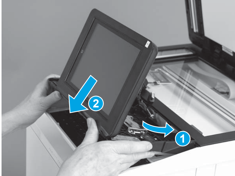
Figure 1-5078 Install the control-panel
