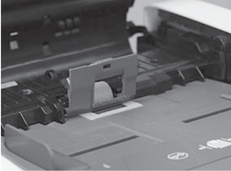
Figure 1-194 Position the separation roller cover
