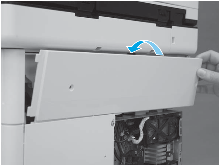
Figure 1-620 Rotate the top of the cover
