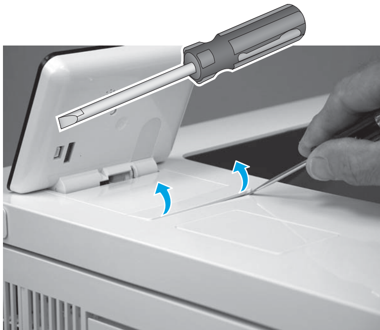
Figure 1-3096 Release the control-panel screws cover tabs
