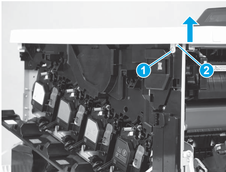
Figure 1-1209 Remove one screw and release one tab
