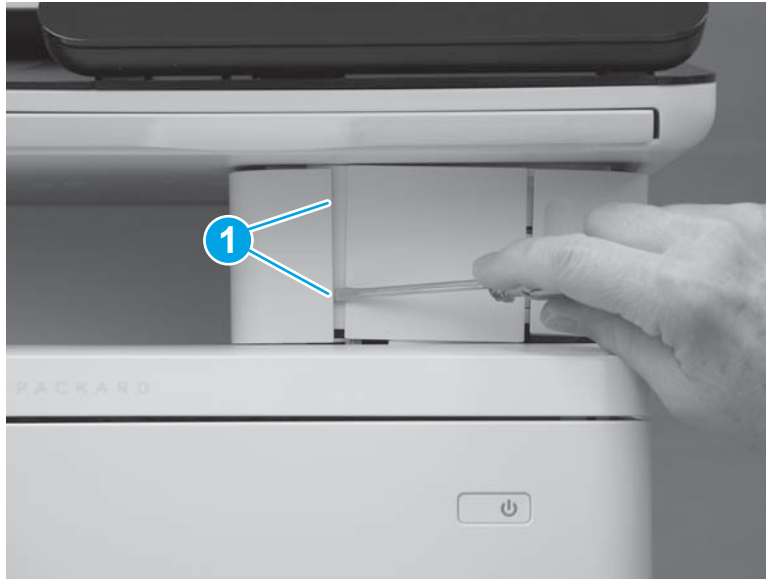
Figure 1-1413 Release two tabs
