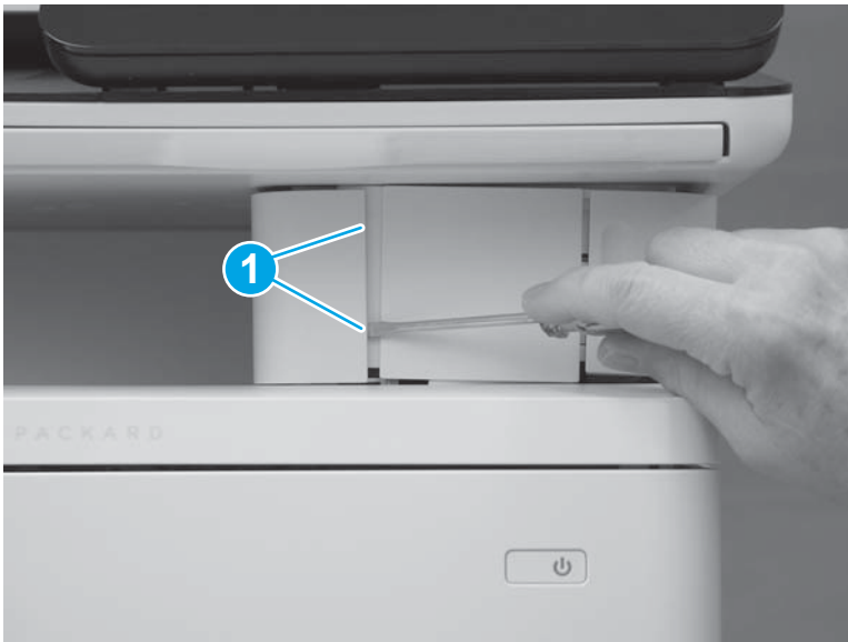
Figure 1-2493 Release two tabs
