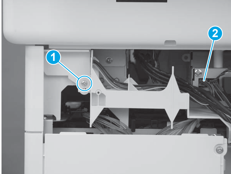
Figure 1-4346 Install one screw and connector
