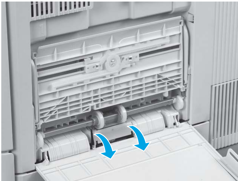
Figure 5-700 Open the roller cover
