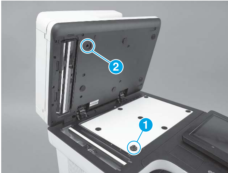
Figure 5-166 Check the retention clips
