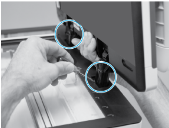
Figure 5-272 Release two tabs
