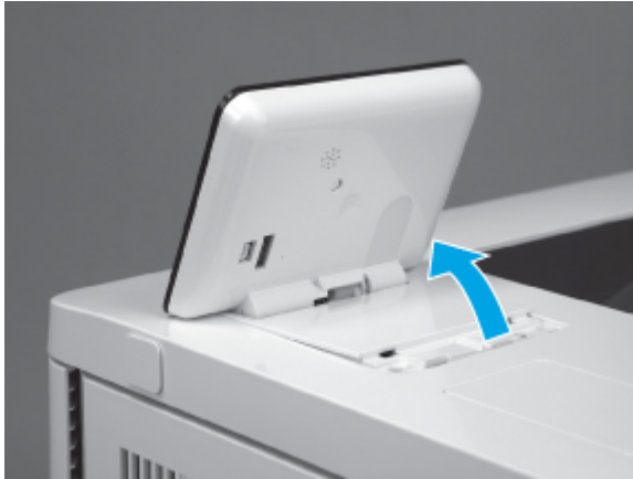
Figure 5-1955 Rotate the control-panel base up
