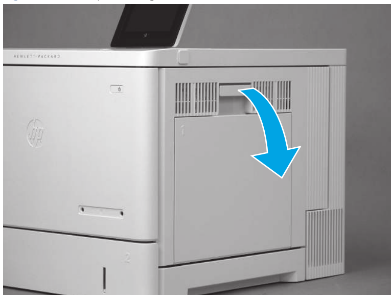
Figure 5-2395 Open the right door
