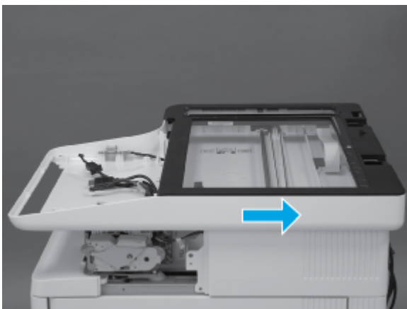
Figure 5-340 Release the image scanner
