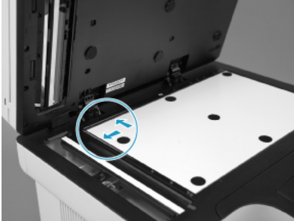
Figure 5-274 Install the white backing
