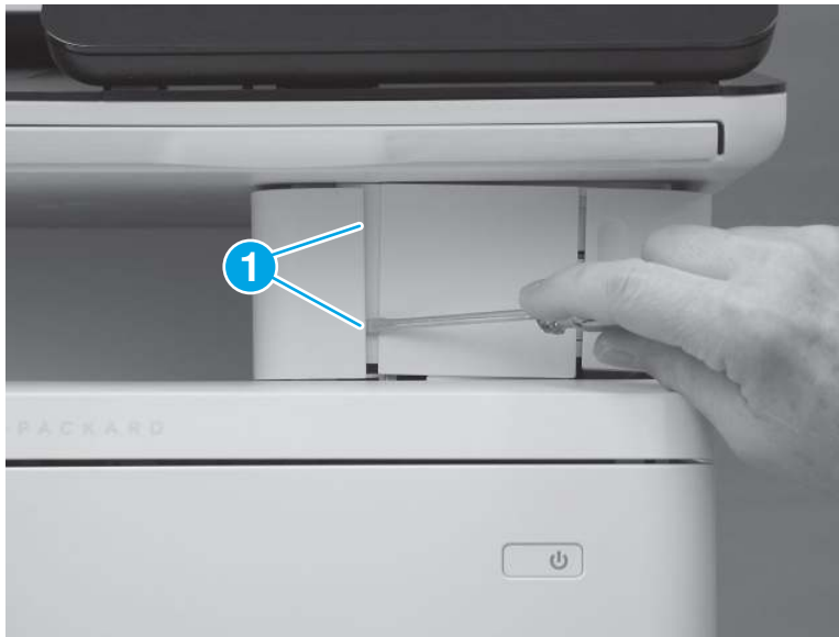
Figure 5-1991 Release two tabs
