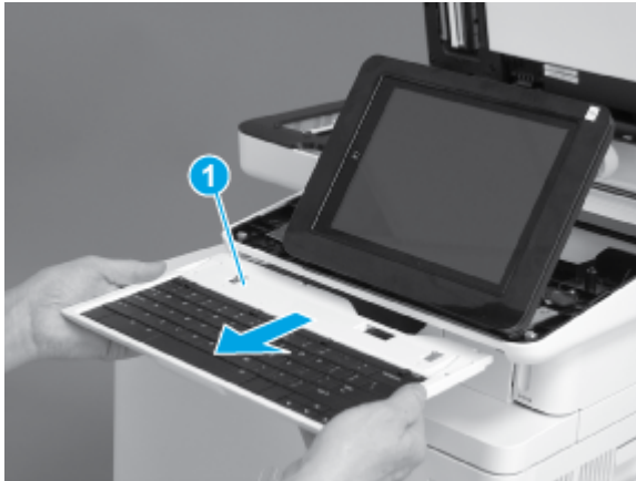
Figure 5-299 Remove the keyboard
