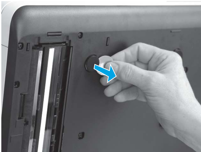
Figure 5-177 Loosen damaged clips
