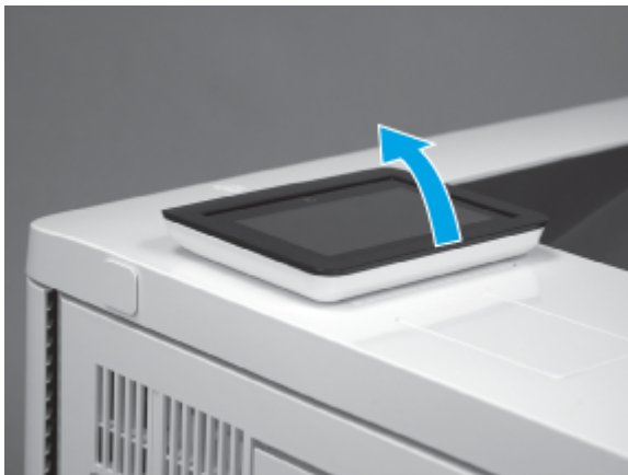
Figure 5-541 Tilt the control panel up
