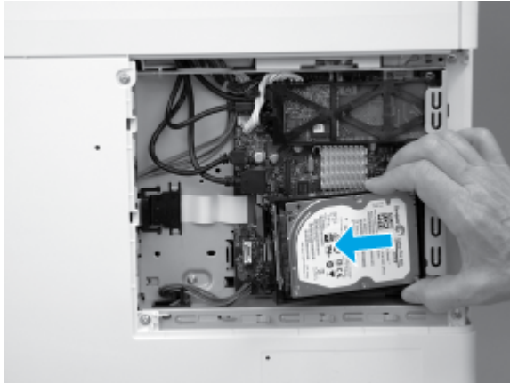
Figure 5-2185 Remove the HDD
