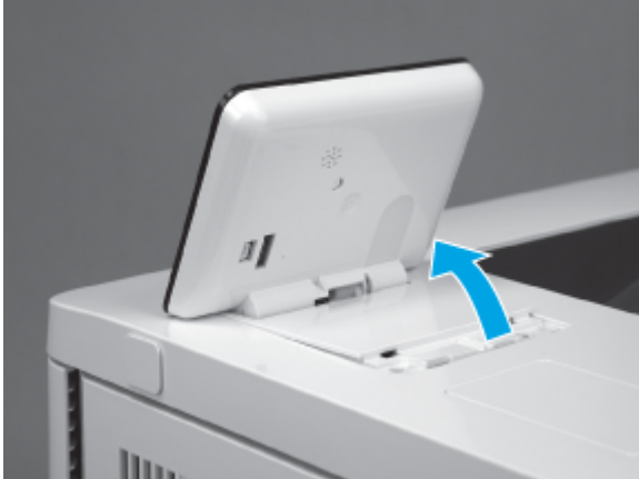
Figure 5-1664 Rotate the control-panel base up
