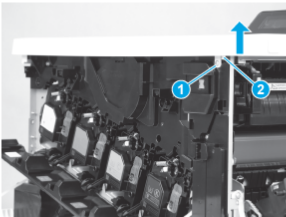
Figure 5-1639 Remove one screw and release one tab
