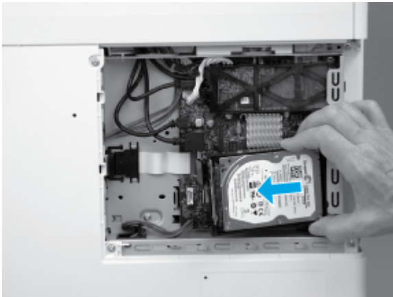
Figure 5-1677 Remove the HDD
