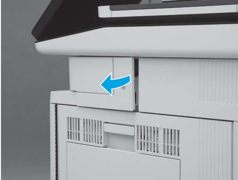
Figure 5-349 Release the back edge of the cover
