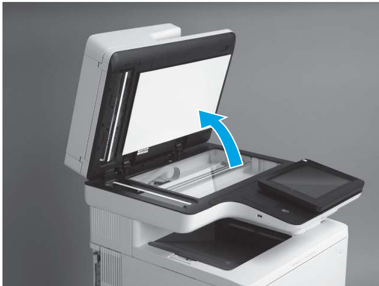
Figure 5-184 Check the white backing
