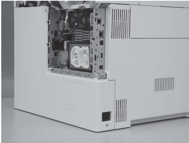
Figure 5-530 Remove four screws
