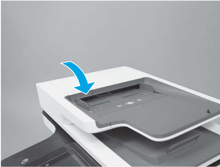
Figure 5-198 Close the document-feeder jam access door
