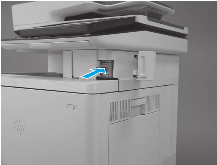
Figure 5-21 Install the staple cartridge
