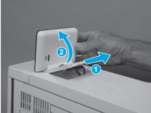
Figure 5-2534 Turn the control panel over
