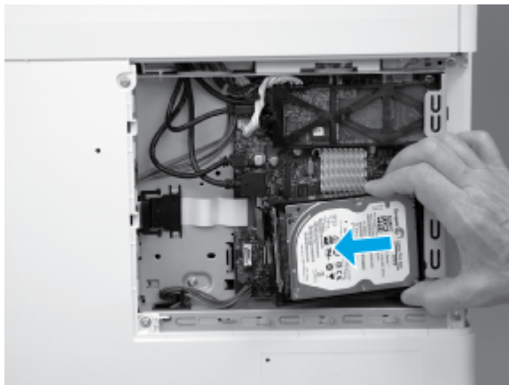
Figure 5-2428 Remove the HDD
