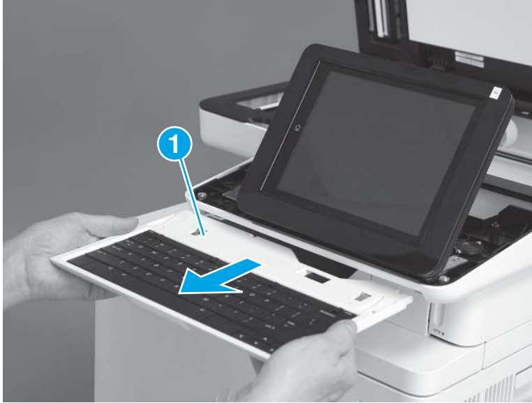
Figure 5-156 Remove the keyboard
