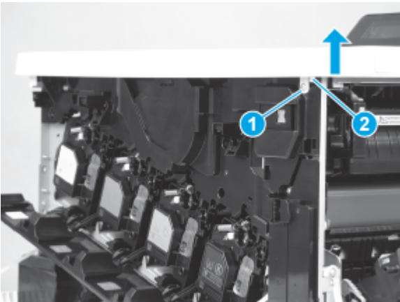
Figure 5-2023 Remove one screw and release one tab
