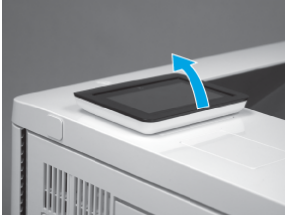
Figure 5-1578 Tilt the control panel up
