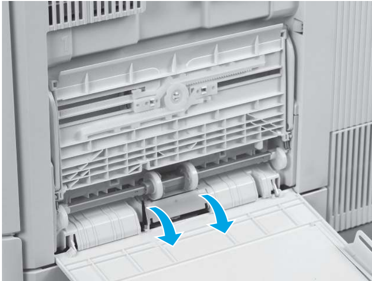
Figure 2-10 Open the roller cover
