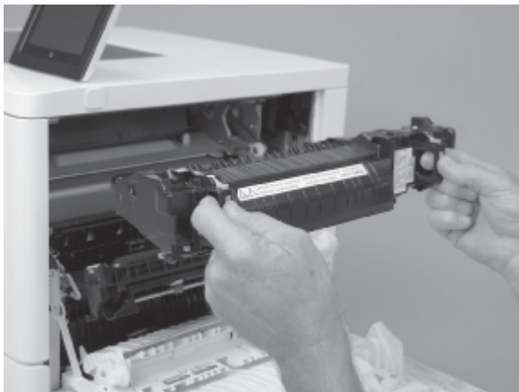
Figure 5-893 Remove the fuser
