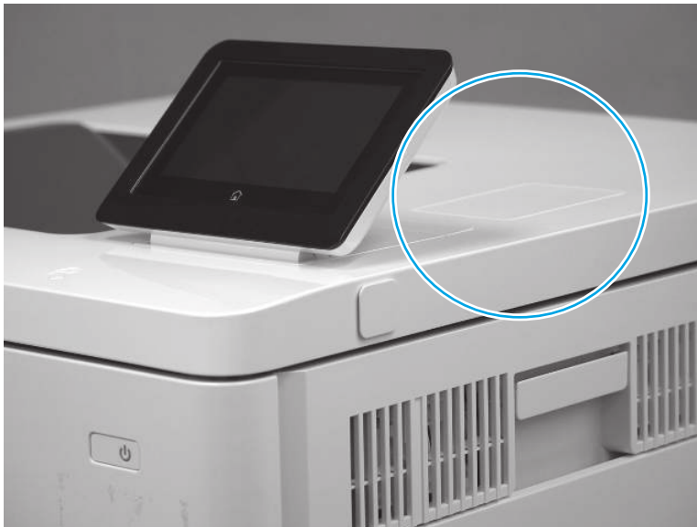
Figure 5-537 Locate the HIP cover
