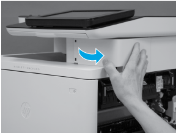
Figure 5-1989 Rotate the cover
