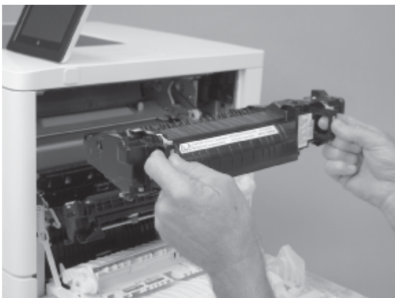
Figure 5-1839 Remove the fuser
