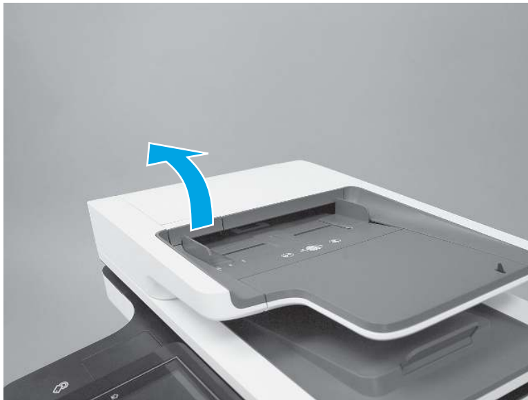
Figure 5-186 Open the document-feeder jam access door
