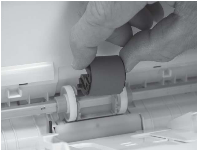
Figure 2-7 Remove the roller
