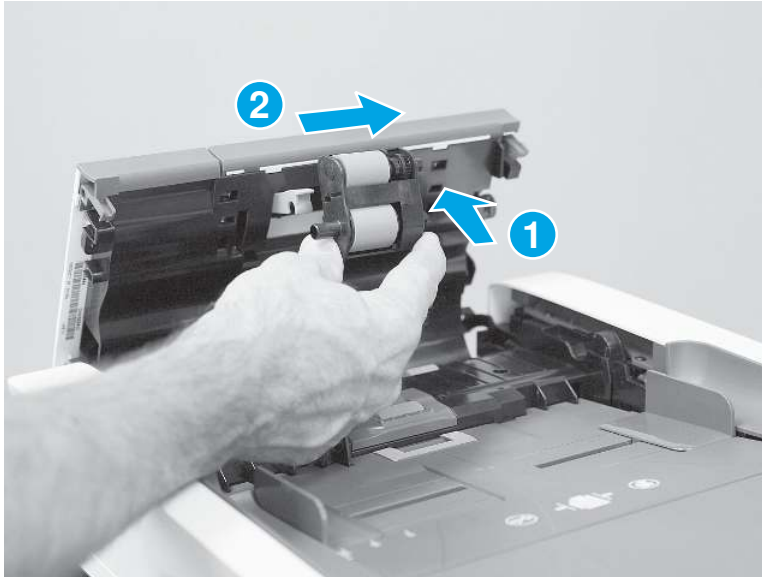
Figure 5-196 Install the roller assembly
