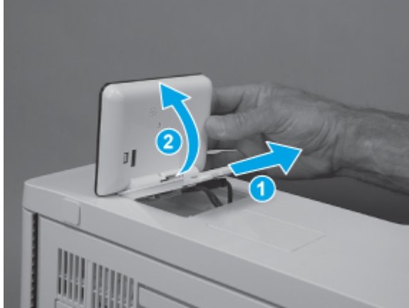
Figure 5-2296 Turn the control panel over
