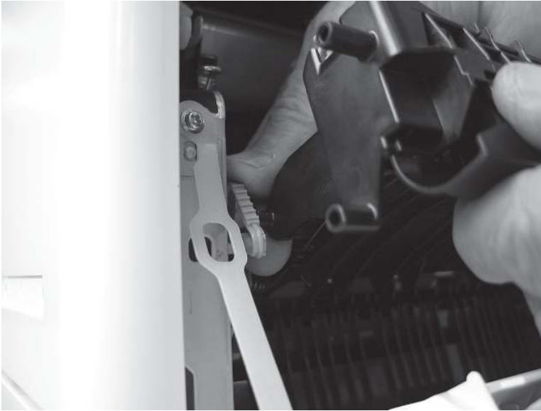
Figure 5-2398 Disengage the blue arm and pin
