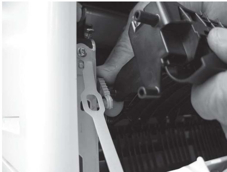
Figure 5-706 Disengage the blue arm and pin
