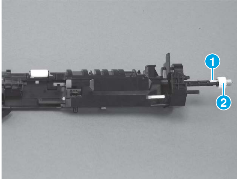
Figure 5-2394 Remove the gear
