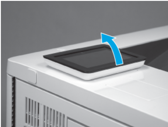
Figure 5-2291 Tilt the control panel up
