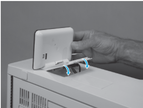
Figure 5-128 Rotate the control-panel base down
