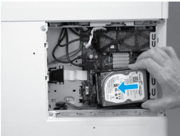
Figure 5-2079 Remove the HDD
