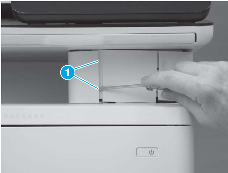
Figure 5-2208 Release two tabs
