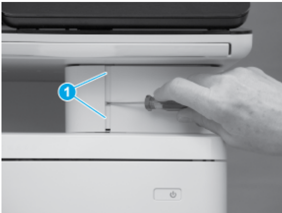
Figure 5-1195 Release two tabs
