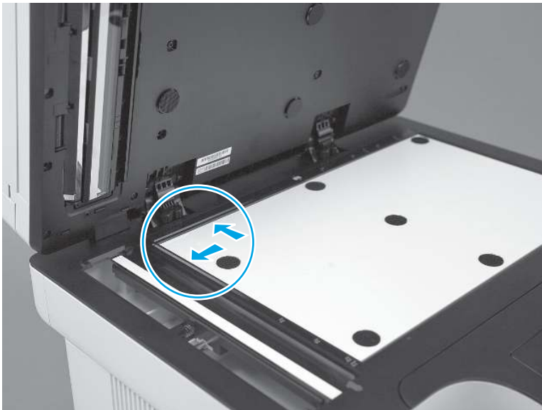
Figure 5-182 Install the white backing
