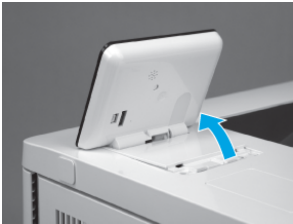
Figure 5-749 Rotate the control-panel base up
