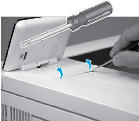
Figure 5-1841 Release the control-panel screws cover tabs
