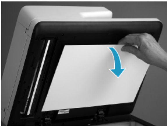
Figure 5-175 Remove the white backing
