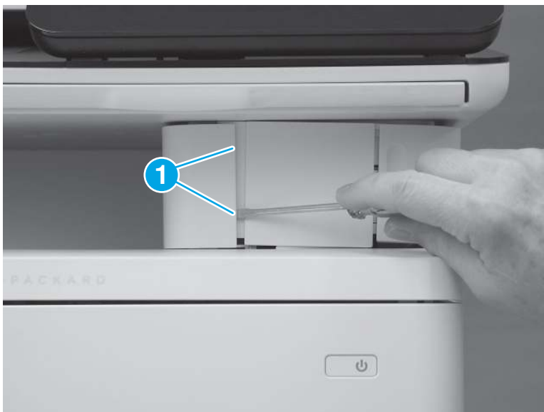
Figure 5-866 Release two tabs
