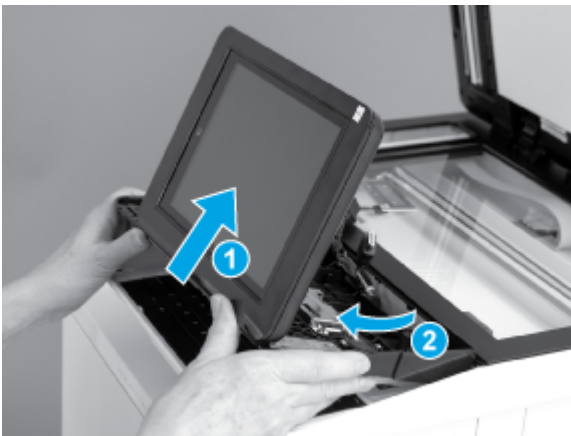
Figure 5-304 Remove the control panel
