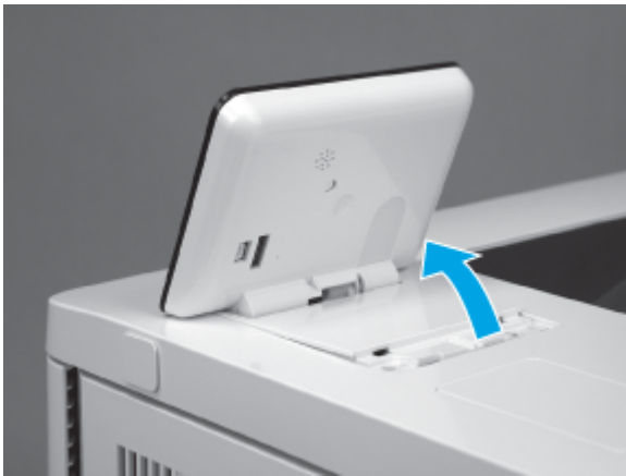
Figure 5-2179 Rotate the control-panel base up
