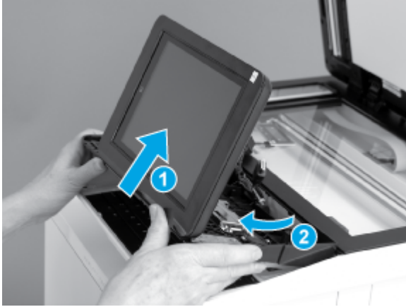
Figure 5-138 Remove the control panel
