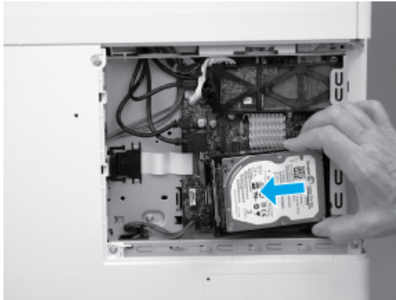
Figure 5-32 Remove the HDD
