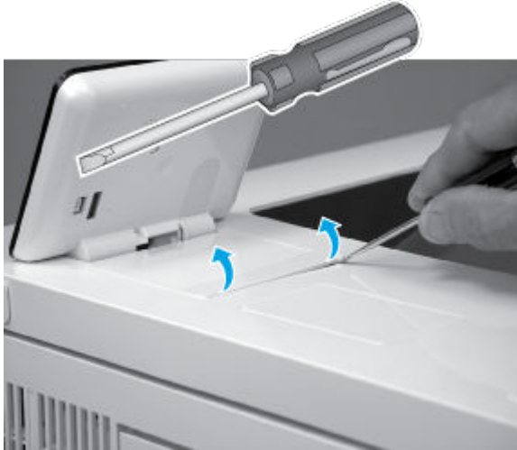
Figure 5-2176 Release the control-panel screws cover tabs
