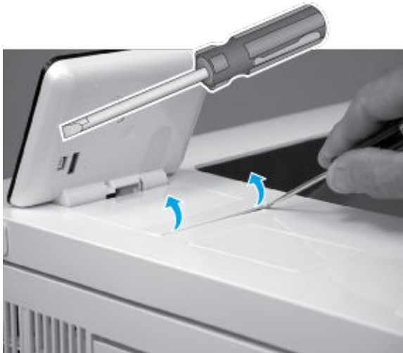
Figure 5-627 Release the control-panel screws cover tabs
