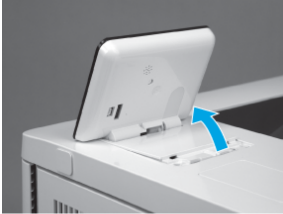
Figure 5-1501 Rotate the control-panel base up
