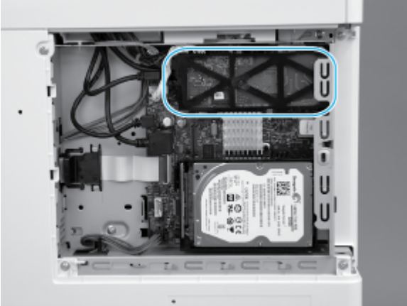
Figure 5-2302 Locate the fax PCA
