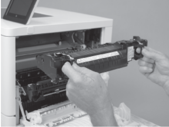
Figure 5-25 Remove the fuser
