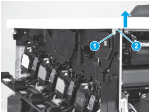
Figure 5-1191 Remove one screw and release one tab
