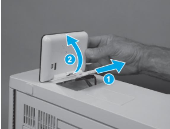
Figure 5-2180 Turn the control panel over
