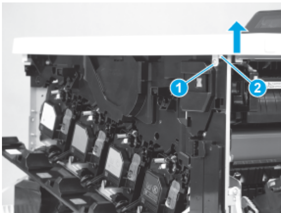
Figure 5-1721 Remove one screw and release one tab
