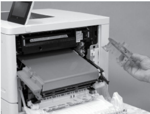
Figure 5-249 Remove the orange handle
