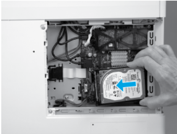
Figure 5-972 Remove the HDD
