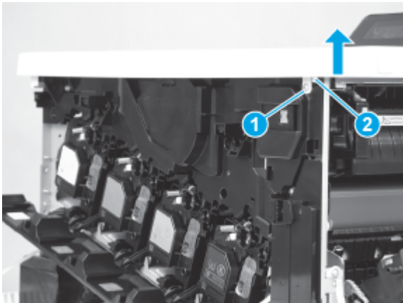
Figure 5-2226 Remove one screw and release one tab
