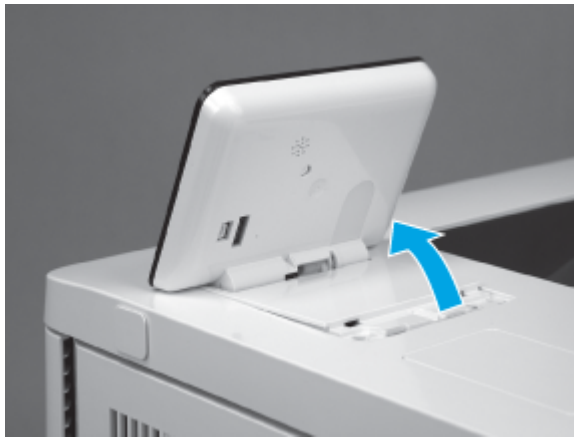
Figure 5-2533 Rotate the control-panel base up
