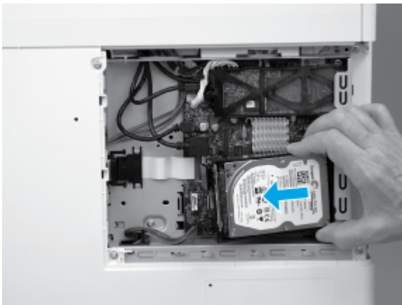
Figure 5-1968 Remove the HDD
