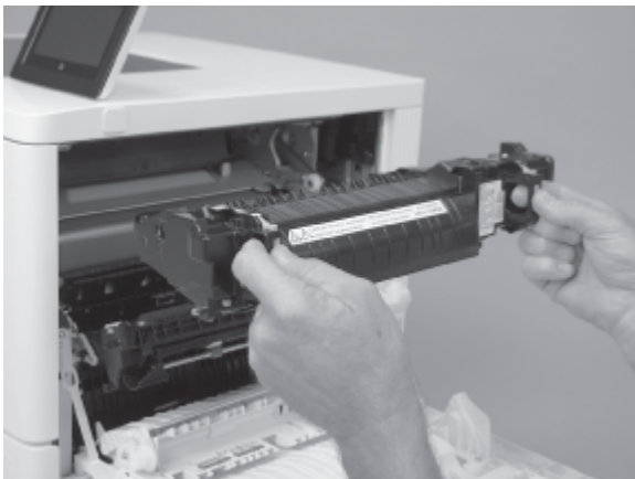
Figure 5-2519 Remove the fuser
