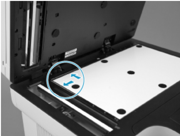
Figure 5-342 Install the white backing
