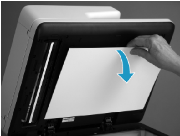
Figure 5-291 Remove the white backing
