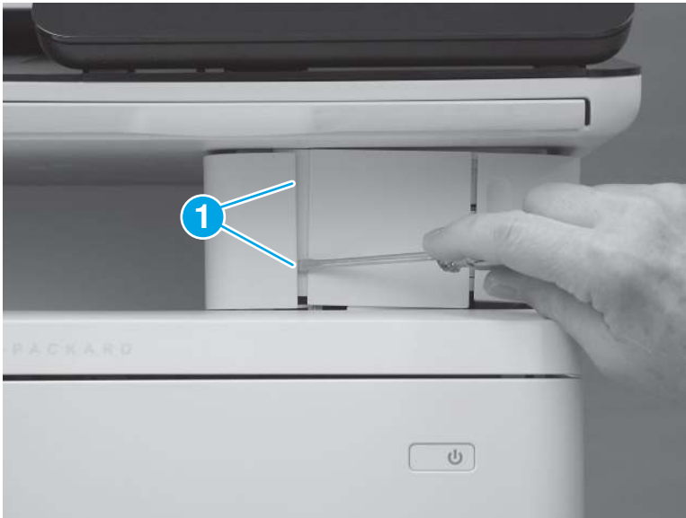
Figure 5-379 Release two tabs
