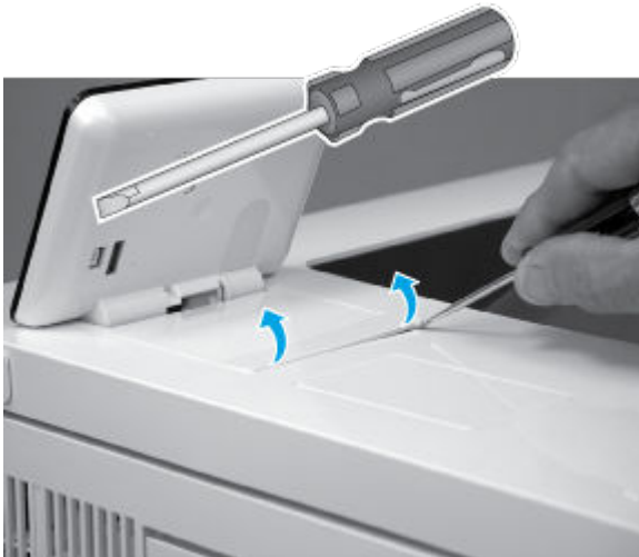
Figure 5-569 Release the control-panel screws cover tabs
