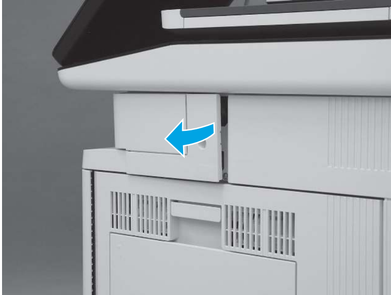
Figure 5-867 Release the back edge of the cover
