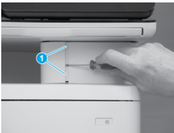
Figure 5-352 Release two tabs
