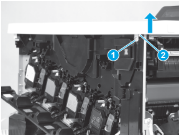
Figure 5-820 Remove one screw and release one tab
