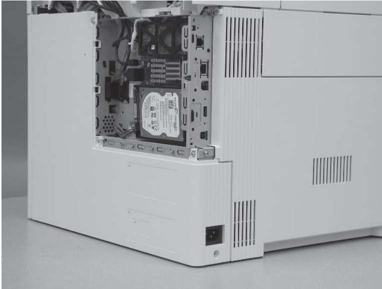
Figure 5-879 Remove four screws
