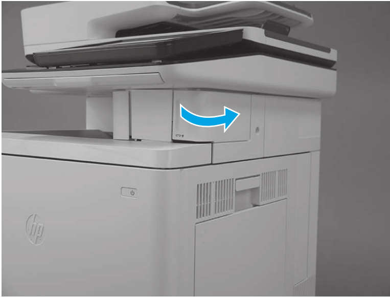
Figure 5-19 Open the stapler door
