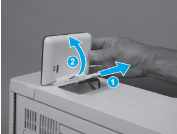
Figure 5-1956 Turn the control panel over
