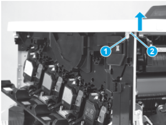
Figure 5-758 Remove one screw and release one tab
