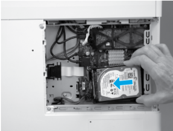
Figure 5-1210 Remove the HDD
