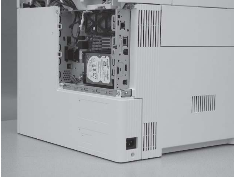
Figure 5-2560 Remove four screws
