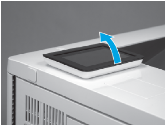
Figure 5-118 Tilt the control panel up
