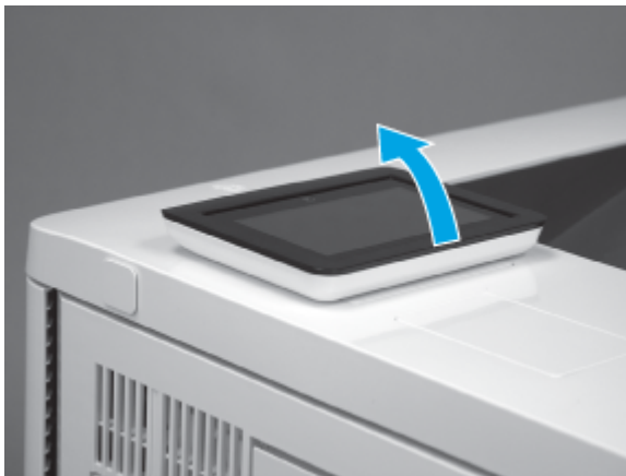
Figure 5-745 Tilt the control panel up
