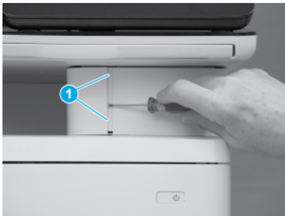
Figure 5-594 Release two tabs
