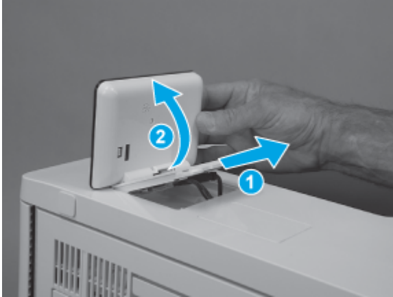
Figure 5-546 Turn the control panel over
