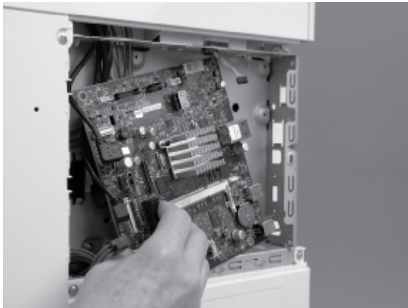
Figure 5-2553 Remove the formatter
