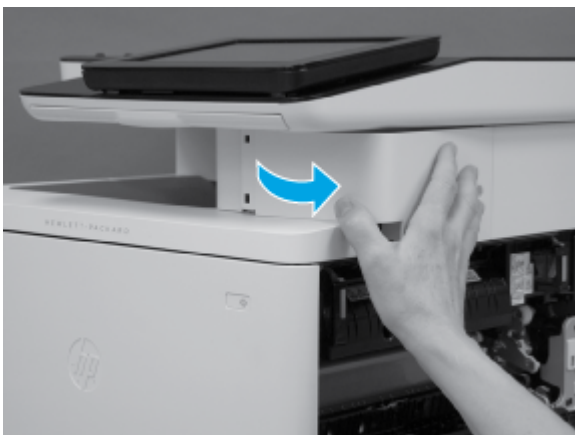
Figure 5-657 Rotate the cover
