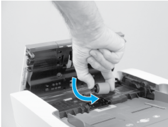
Figure 5-192 Install the roller
