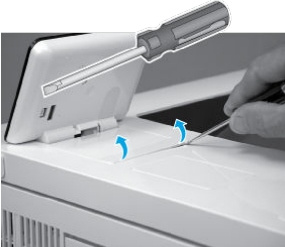
Figure 5-2530 Release the control-panel screws cover tabs
