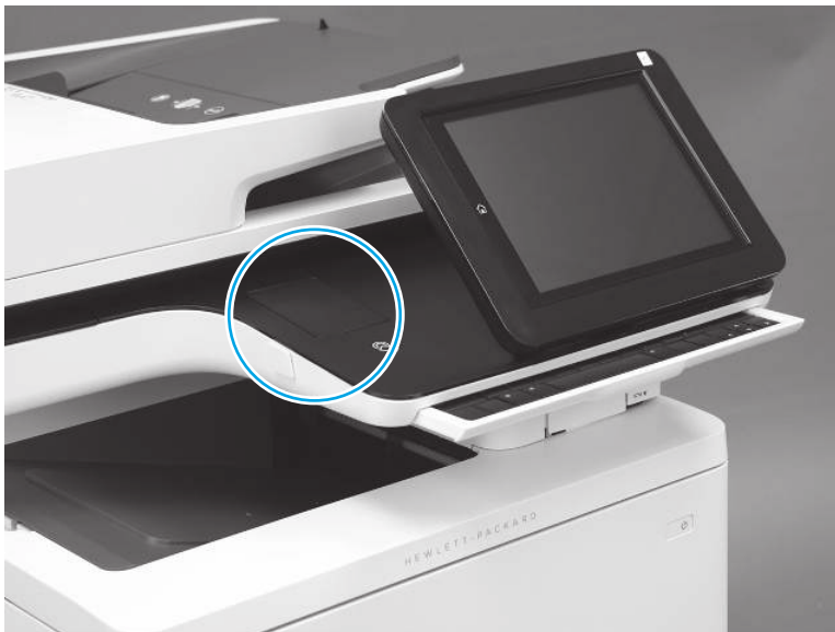
Figure 5-112 Locate the HIP cover
