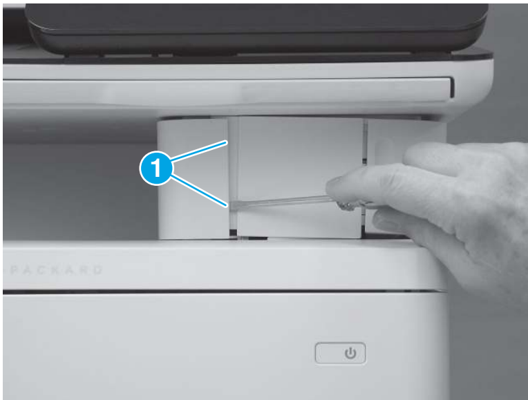
Figure 5-934 Release two tabs
