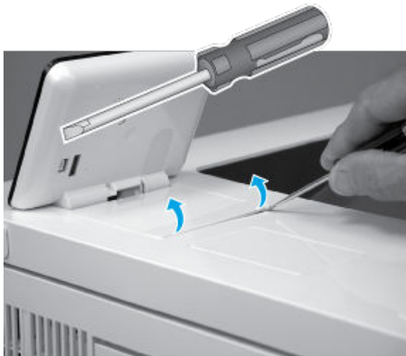
Figure 5-119 Release the control-panel screws cover tabs
