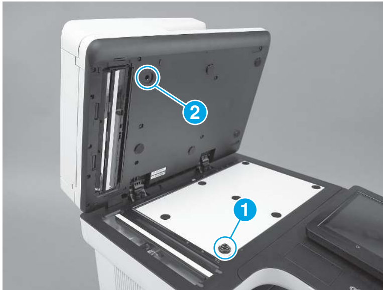
Figure 5-176 Check the retention clips
