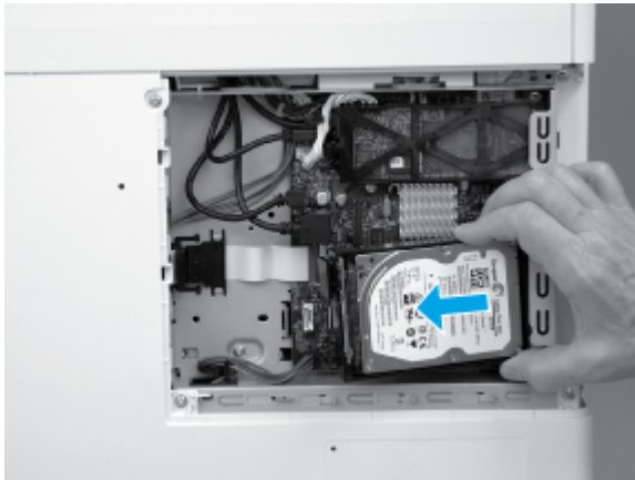
Figure 5-1759 Remove the HDD
