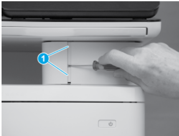
Figure 5-1697 Release two tabs
