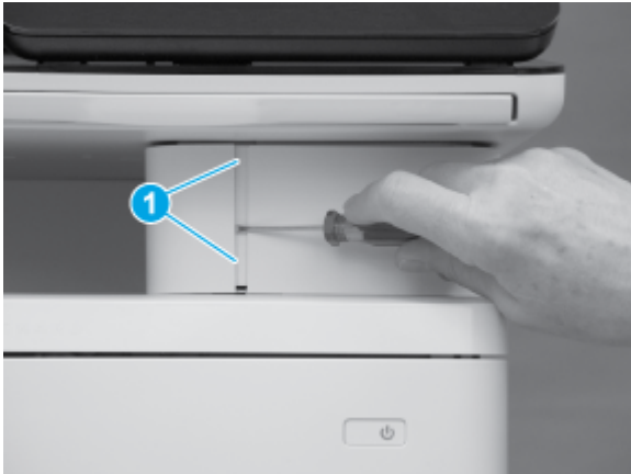
Figure 5-656 Release two tabs
