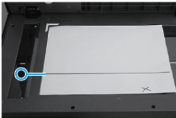
Figure 4-92 Place the copy on the flatbed
