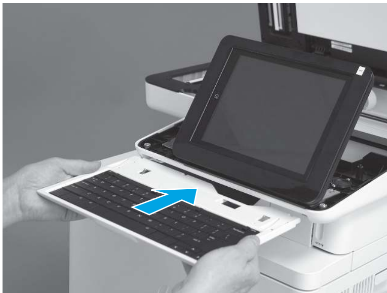
Figure 5-158 Slide the keyboard into the slot
