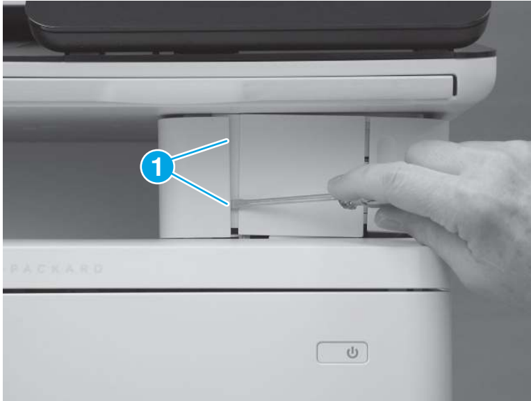
Figure 5-1880 Release two tabs
