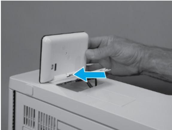
Figure 5-127 Turn the control panel over
