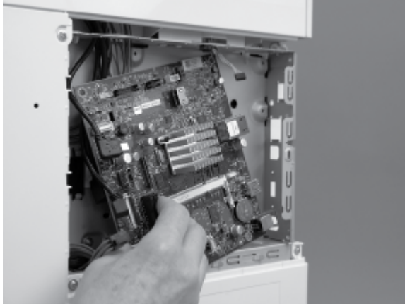
Figure 5-993 Remove the formatter
