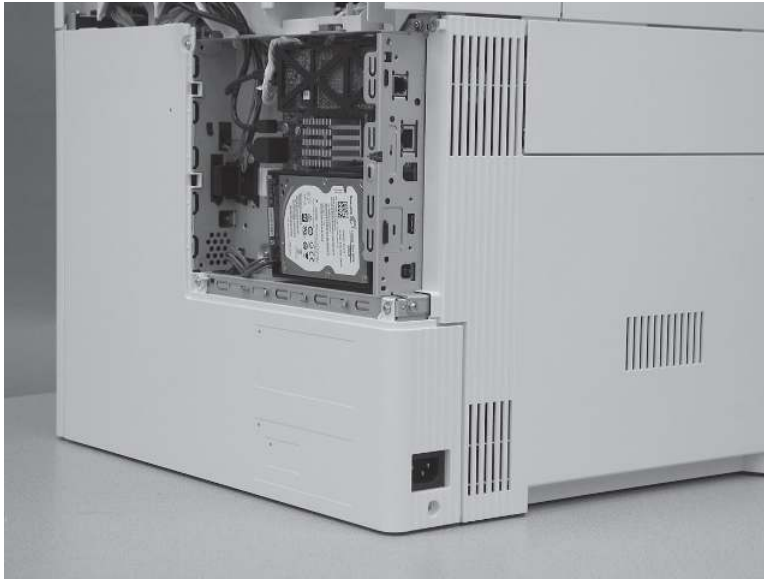
Figure 5-1152 Remove four screws
