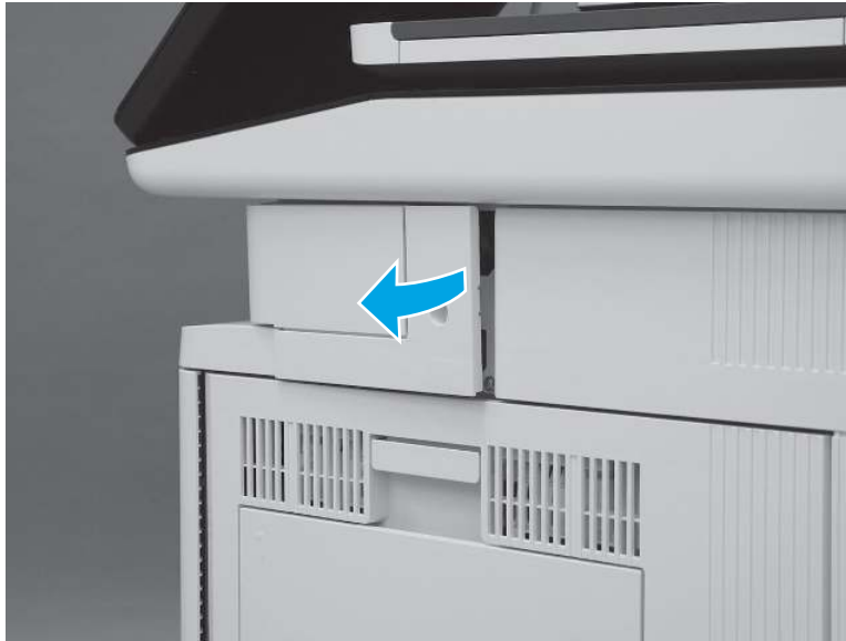
Figure 5-835 Release the back edge of the cover
