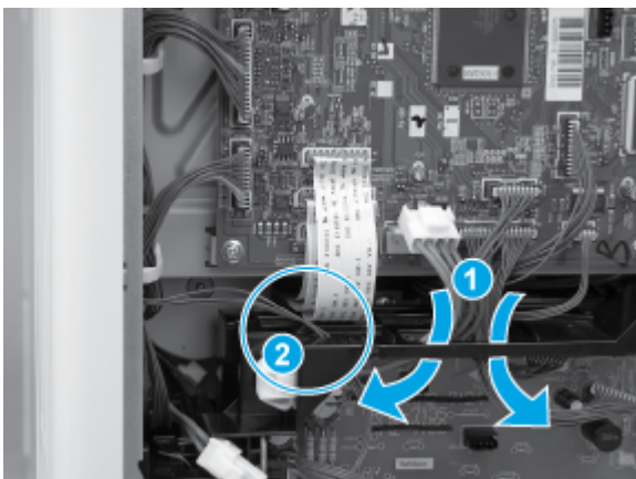
Figure 5-2356 Pass the wire harnesses through the opening
