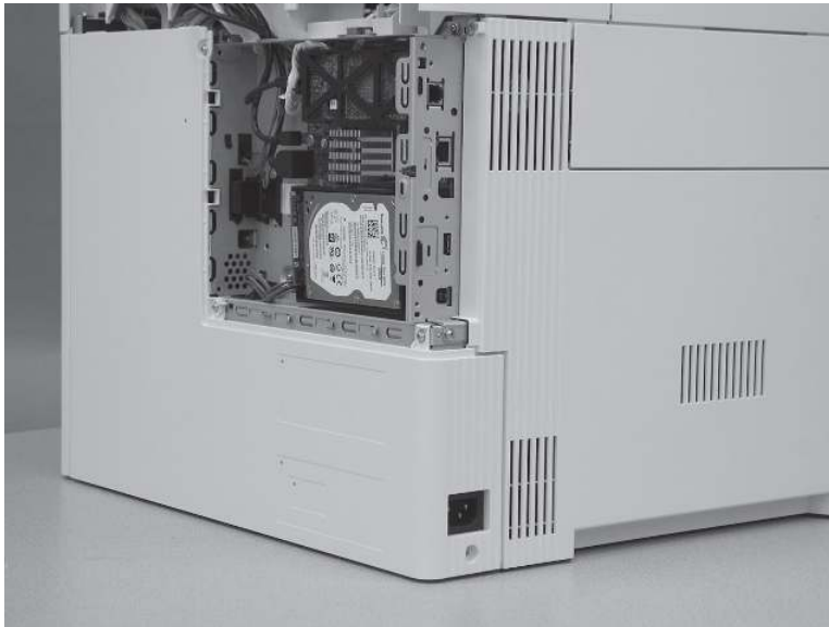
Figure 5-517 Remove four screws
