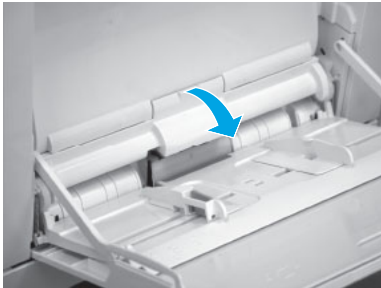
Figure 5-694 Open the roller cover
