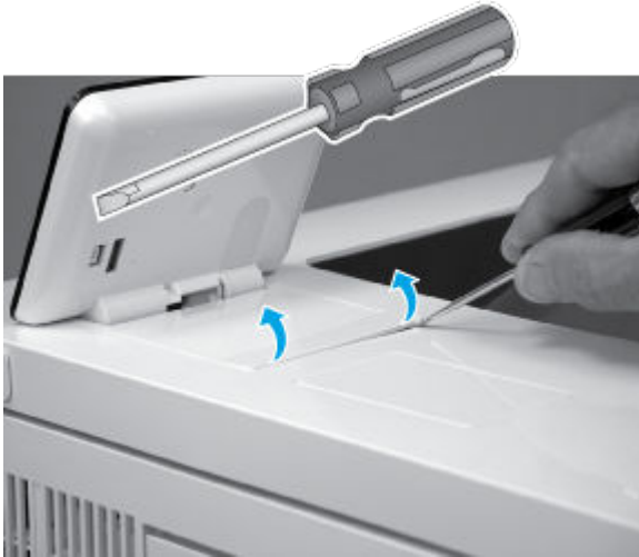
Figure 5-542 Release the control-panel screws cover tabs
