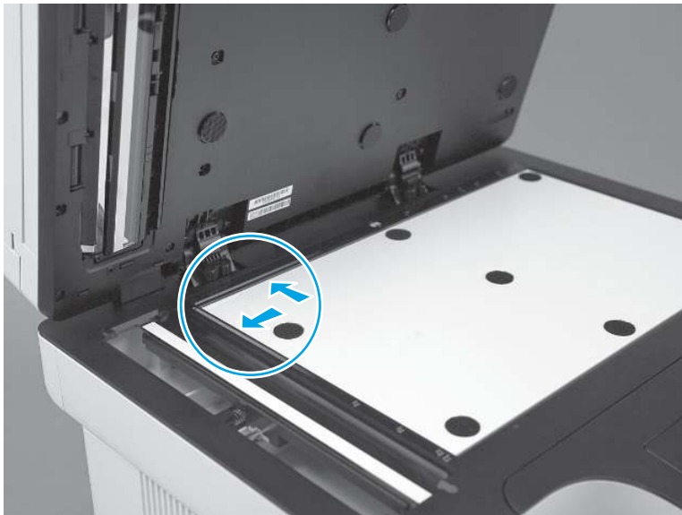
Figure 5-170 Install the white backing
