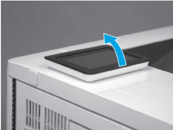
Figure 5-1660 Tilt the control panel up
