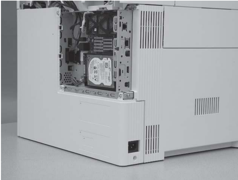
Figure 5-1071 Remove four screws
