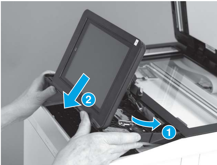
Figure 5-142 Install the control panel
