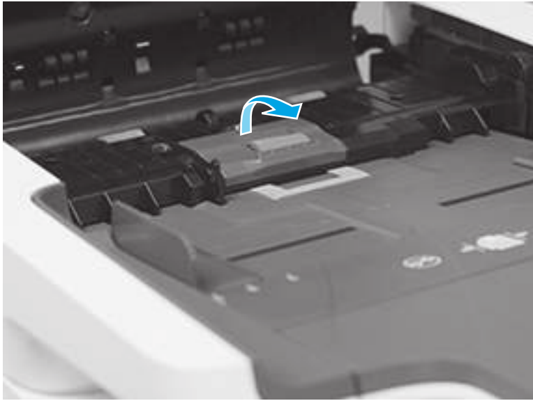
Figure 5-189 Release the separation roller cover
