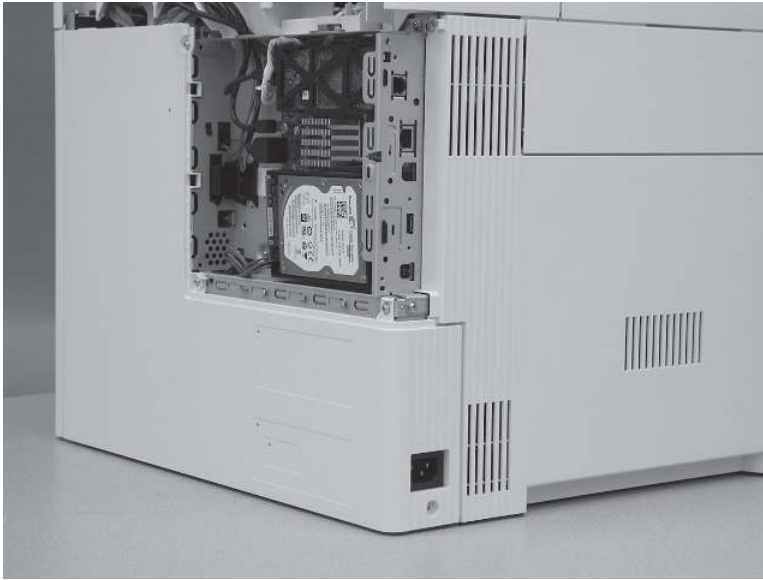
Figure 5-1185 Remove four screws
