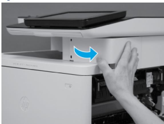
Figure 5-832 Rotate the cover
