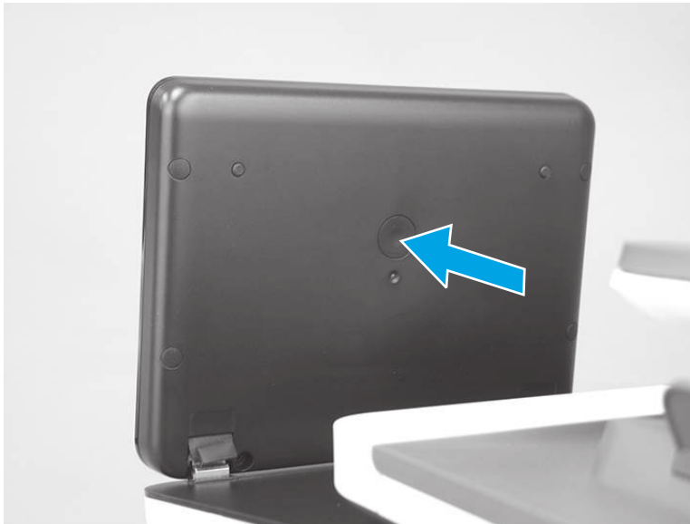
Figure 4-58 Press the diagnostics-access button
