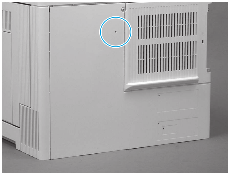
Figure 4-51 Engine test button
