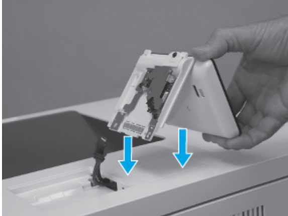
Figure 5-125 Place the control panel on the product
