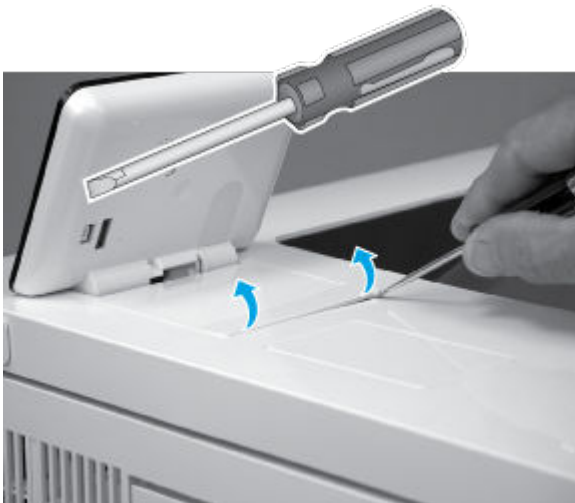
Figure 5-903 Release the control-panel screws cover tabs
