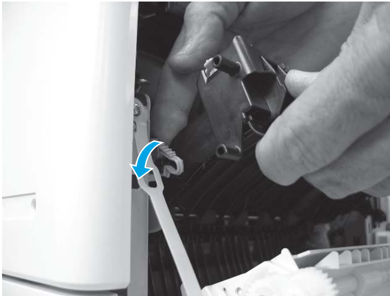
Figure 5-2154 Carefully flex the top portion of the blue arm
