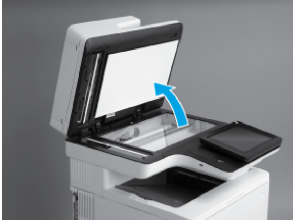
Figure 5-276 Check the white backing
