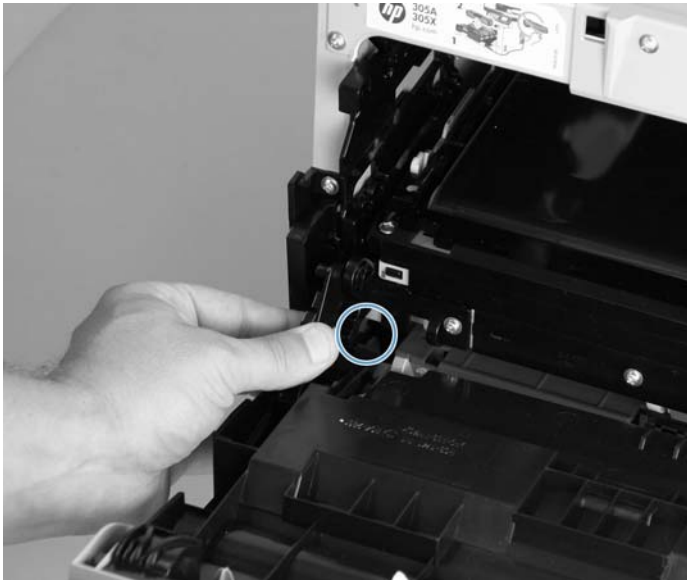
Figure 1-69 Remove the front-door assembly (9 of 10)
