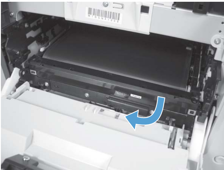
Figure 1-72 Remove the ITB (2 of 6)
