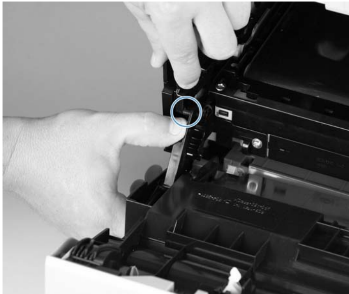
Figure 1-67 Remove the front-door assembly (7 of 10)
