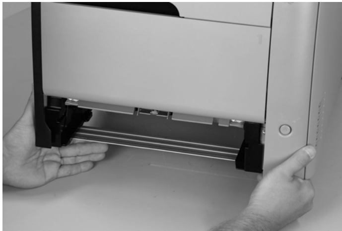
Figure 1-4 Remove the pickup roller (1 of 3)
