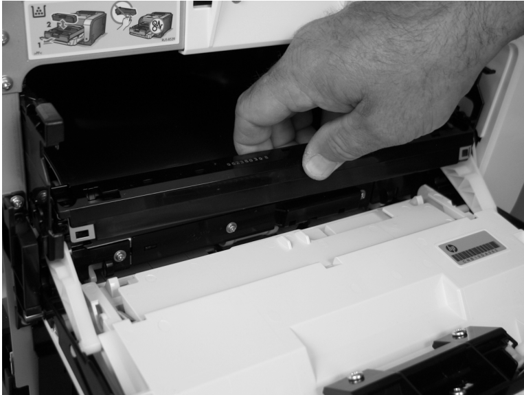
Figure 1-108 Remove the color-misregistration sensor assembly PCA (4 of 4)
