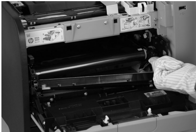
Figure 1-74 Remove the ITB (4 of 6)
