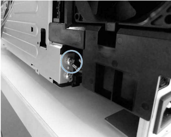
Figure 1-146 Remove the ground strap
