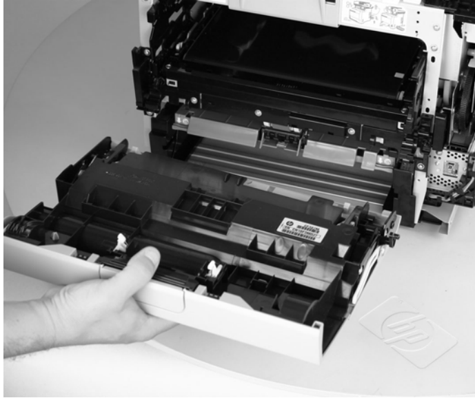
Figure 1-70 Remove the front-door assembly (10 of 10)
