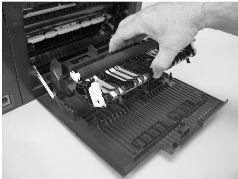
Figure 1-31 Remove the feed assembly (2 of 2)
