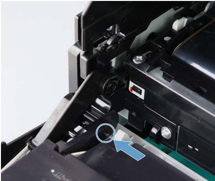
Figure 1-61 Remove the front-door assembly (1 of 10)
