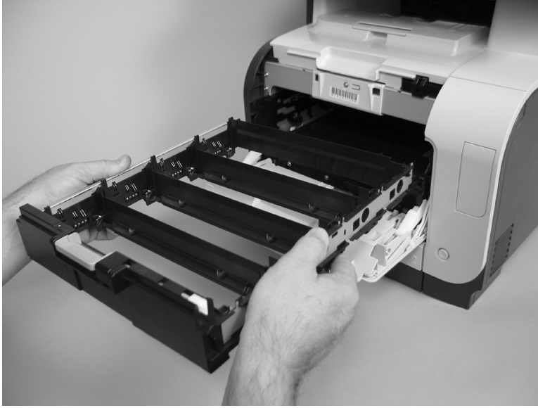
Figure 1-25 Remove the print-cartridge drawer (3 of 3)
