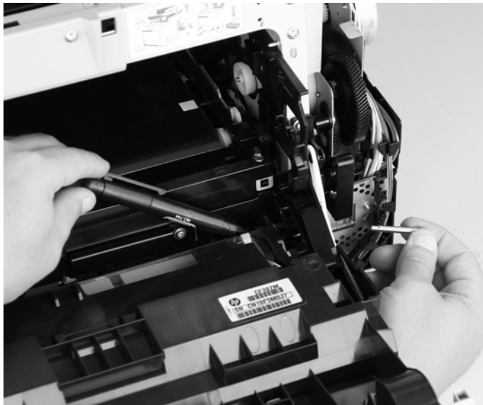
Figure 1-63 Remove the front-door assembly (3 of 10)
