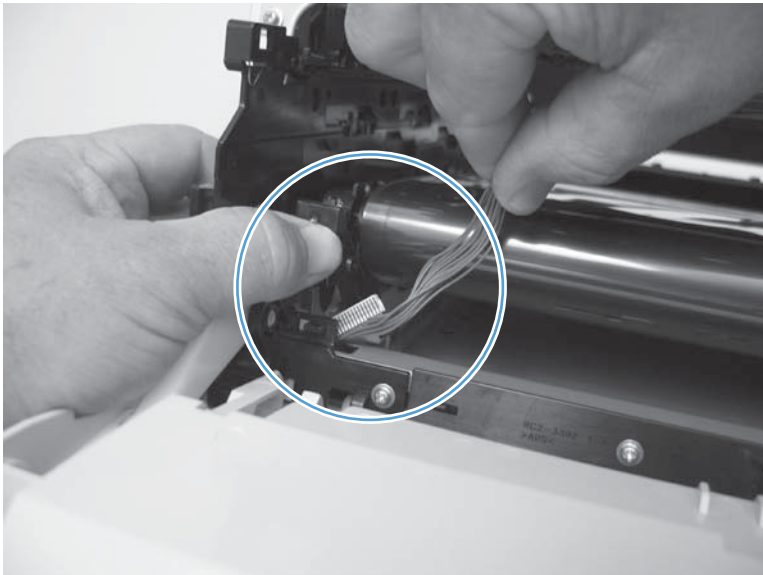
Figure 1-109 Reinstall the color-misregistration sensor assembly PCA (1 of 2)
