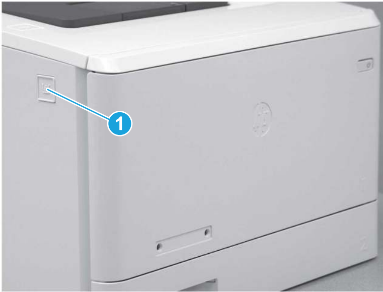
Figure 5-346 Release the front door
