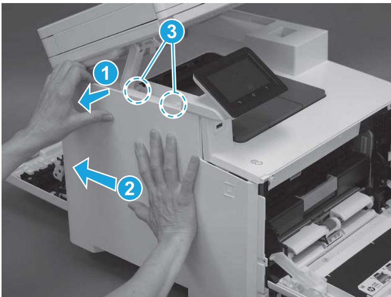
Figure 5-894 Release one tab and two hooks
