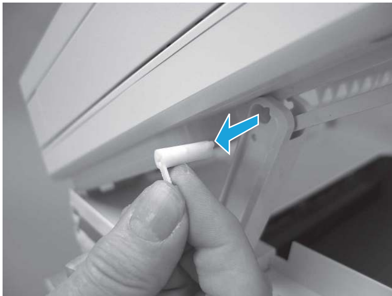
Figure 5-1447 Remove the pin
