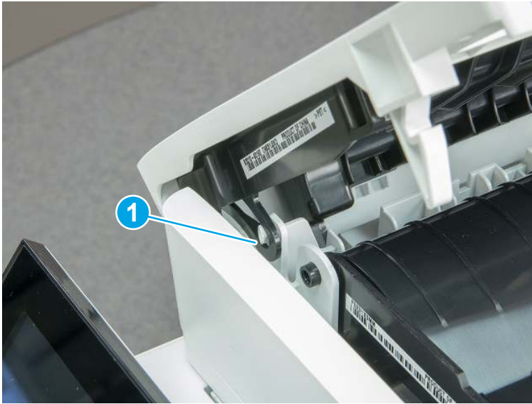
Figure 5-14 Release one hinge pin
