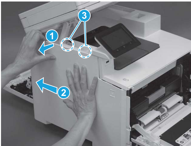
Figure 5-921 Release one tab and two hooks
