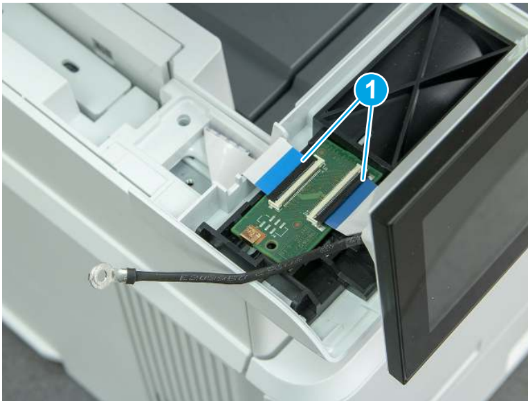
Figure 5-237 Disconnect two FFC
