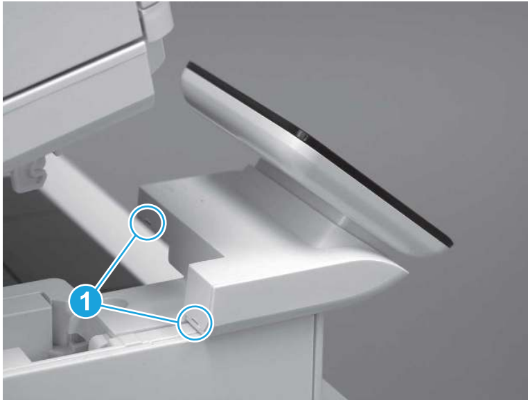
Figure 5-1637 Release two tabs
