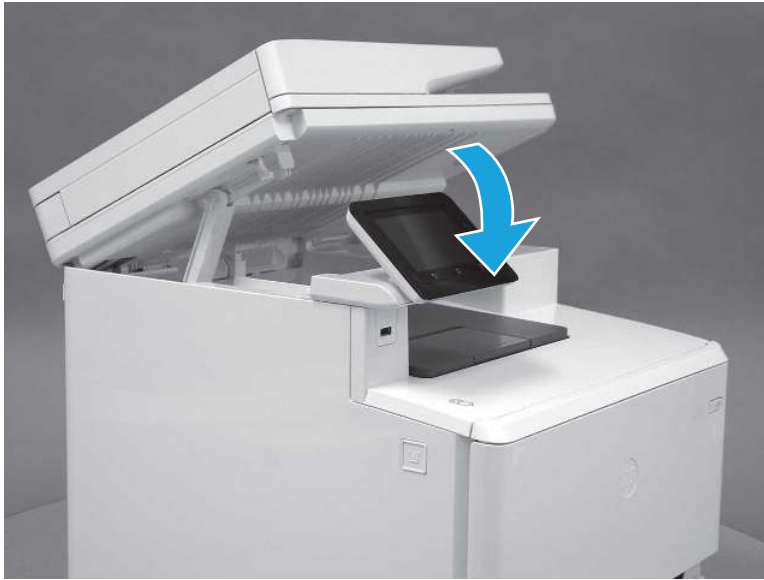
Figure 5-1994 Lower the scanner
