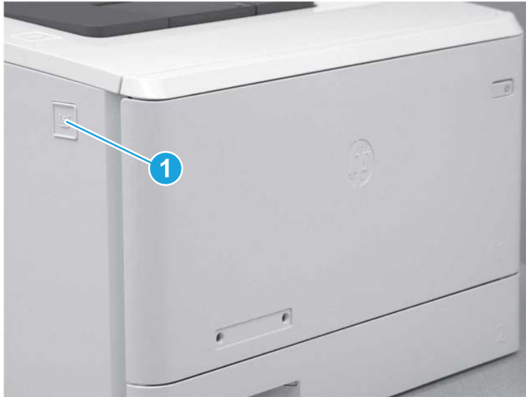
Figure 5-377 Release the front door
