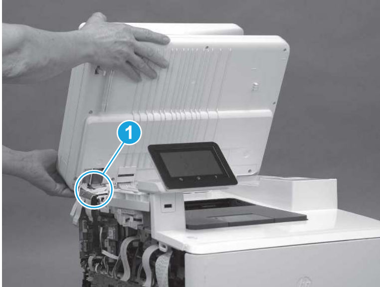
Figure 5-230 Release the cables
