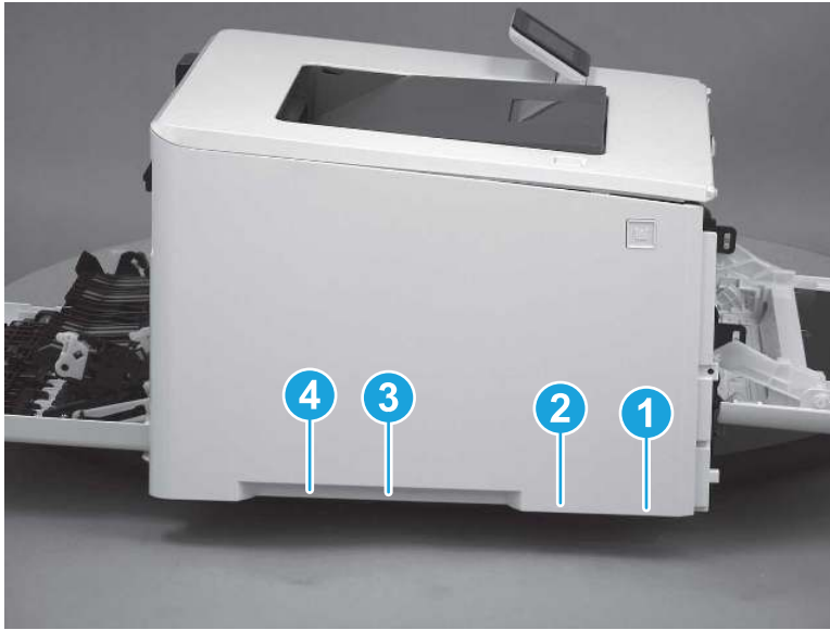
Figure 5-1029 Release bottom tabs
