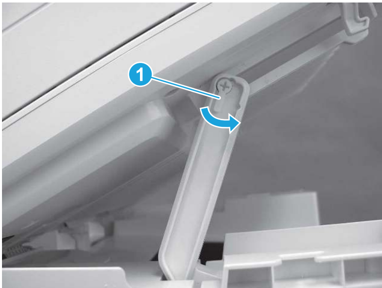
Figure 5-1646 Release scanner support arm pin
