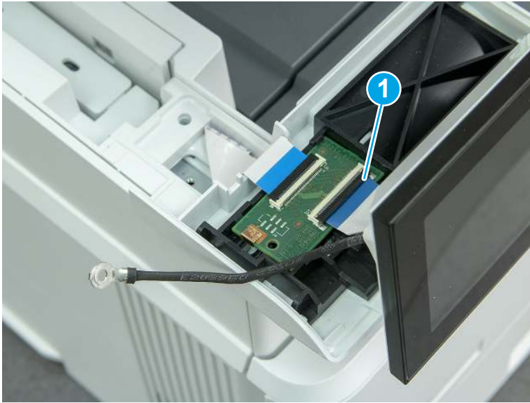
Figure 5-280 Disconnect one flat cable
