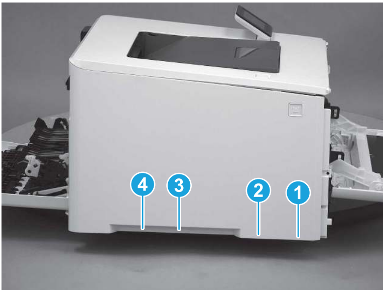
Figure 5-807 Release bottom tabs
