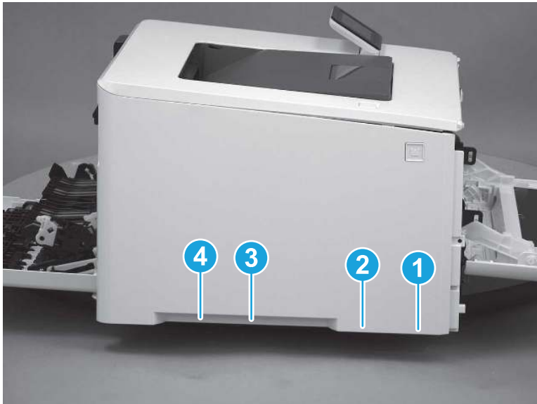
Figure 5-1970 Release bottom tabs
