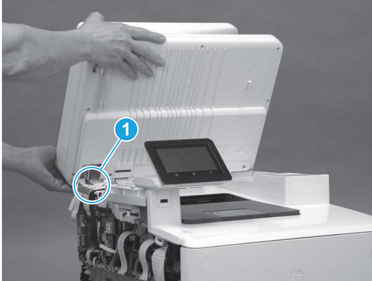
Figure 5-1450 Release the cables
