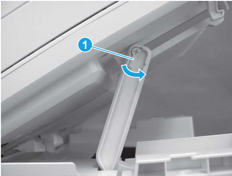
Figure 5-1947 Release scanner support arm pin
