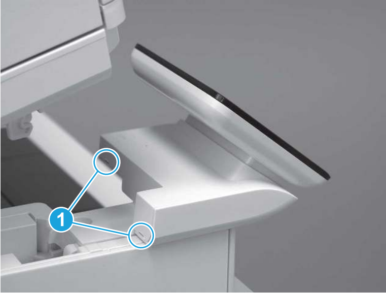
Figure 5-257 Release two tabs
