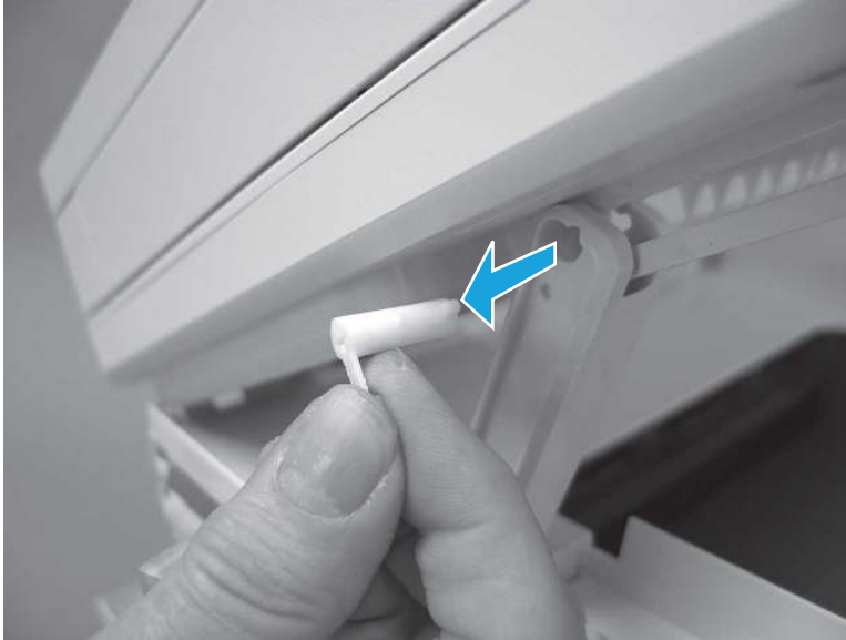
Figure 5-1647 Remove the pin
