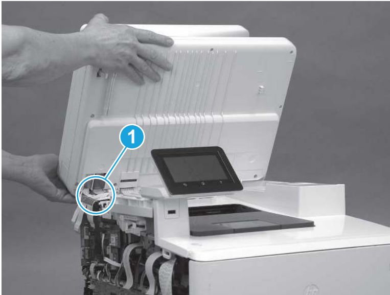
Figure 5-44 Release the cables
