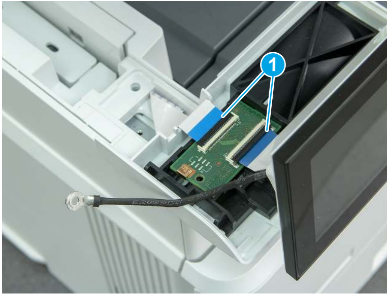
Figure 5-2010 Disconnect two FFC
