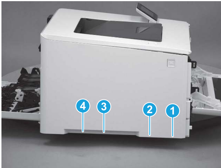
Figure 5-383 Release bottom tabs
