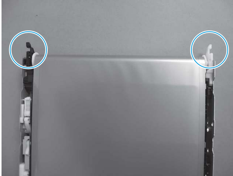
Figure 5-853 Check tabs on the end of the ITB
