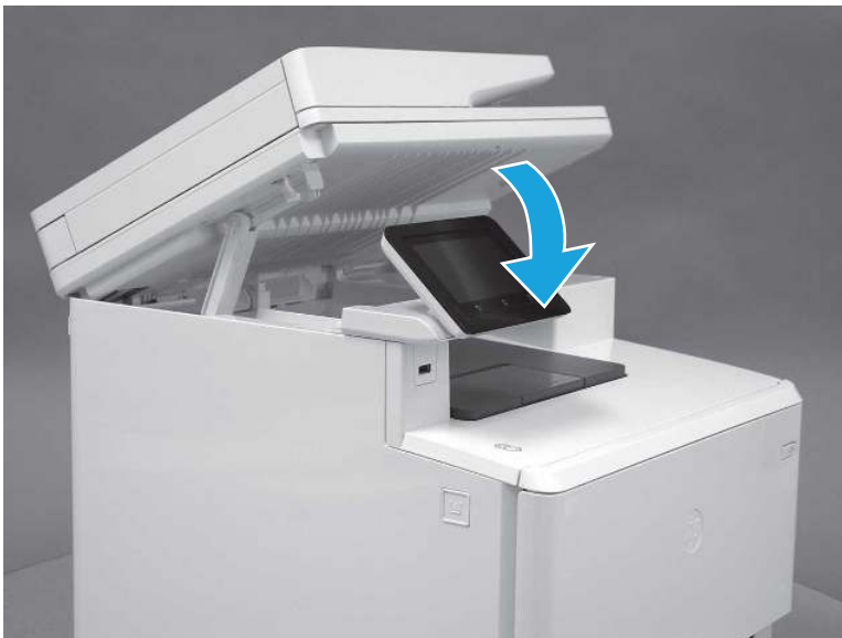
Figure 5-367 Lower the scanner
