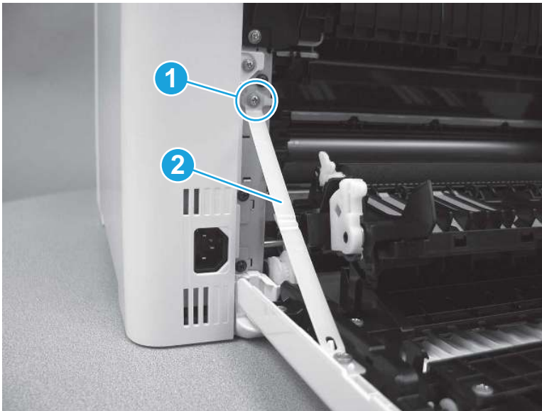
Figure 5-819 Remove one screw and release the arm
