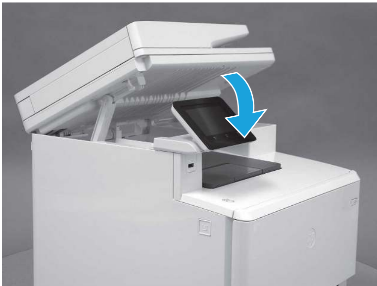
Figure 5-548 Lower the scanner
