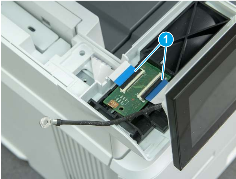
Figure 5-1546 Disconnect two FFC
