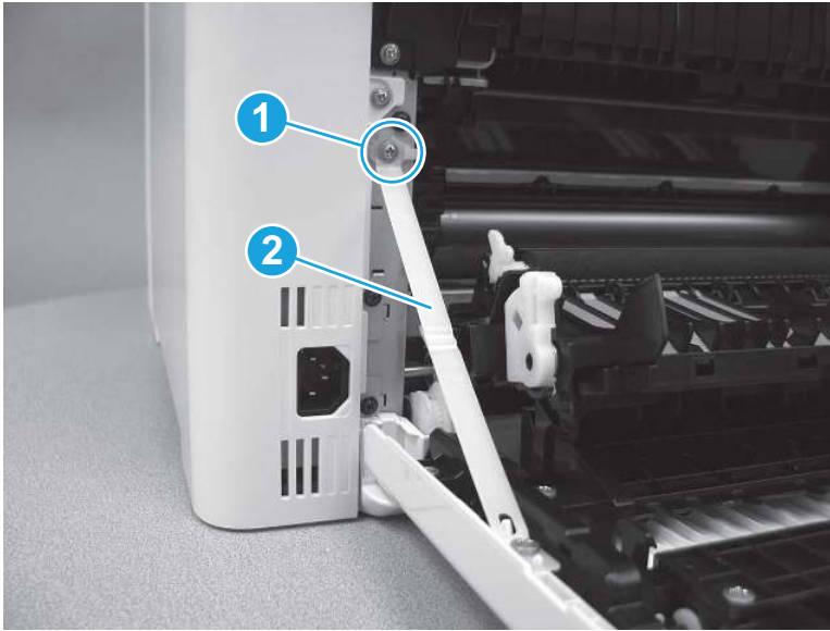
Figure 5-759 Remove one screw and release the arm
