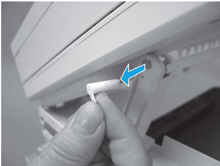
Figure 5-1760 Remove the pin
