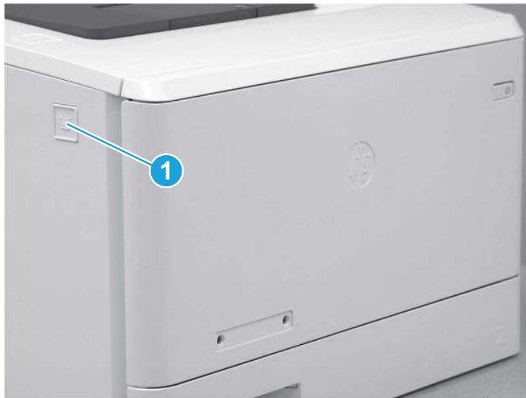
Figure 5-860 Release the front door
