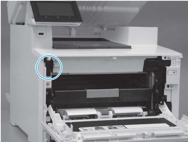
Figure 4-46 Defeat the front (cartridge) door interlock
