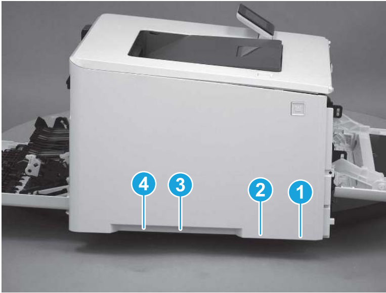
Figure 5-1221 Release bottom tabs
