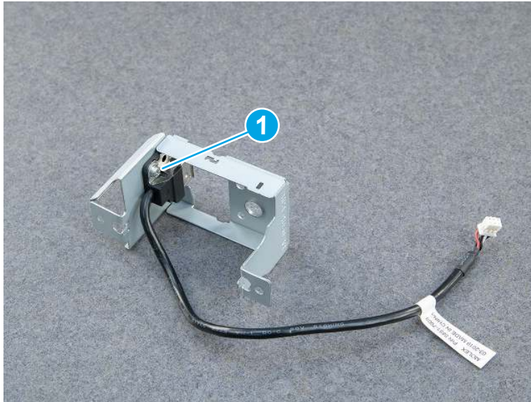
Figure 5-254 Remove one screw and remove the USB connector
