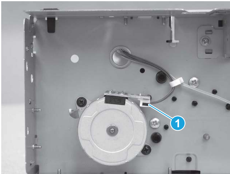
Figure 5-2237 Disconnect one connector
