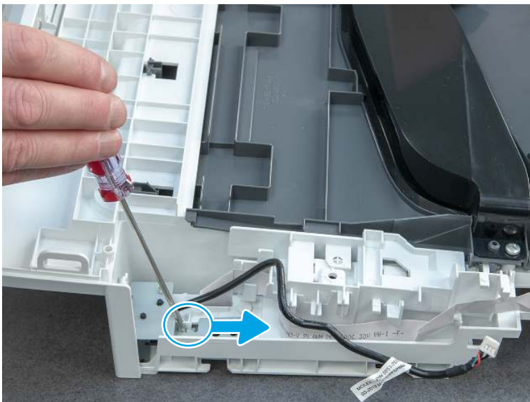
Figure 5-253 Release the metal tab and lift to remove the USB
