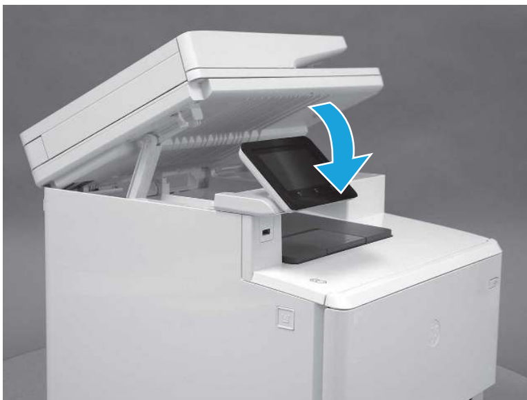
Figure 5-1115 Lower the scanner
