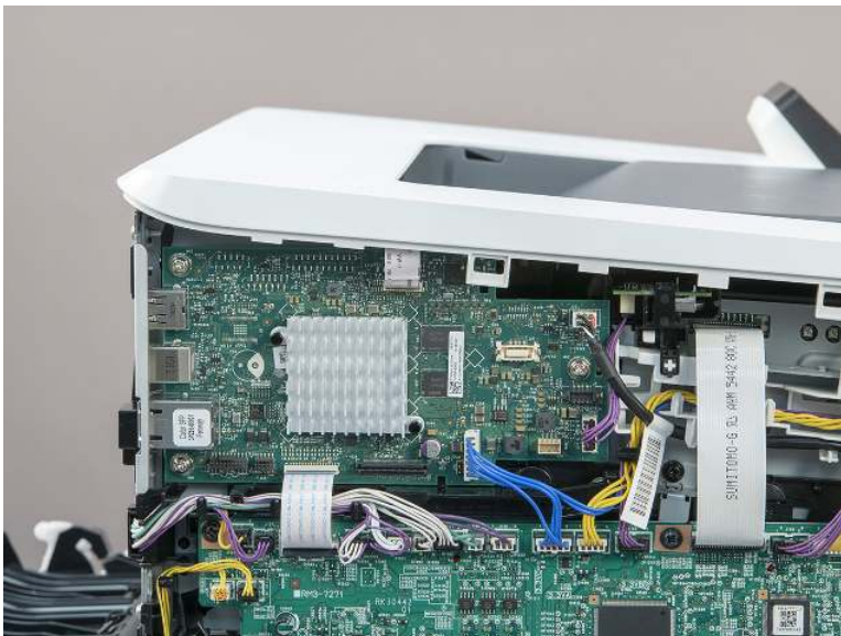
Figure 5-1856 Disconnect all of the connectors (SFP)
