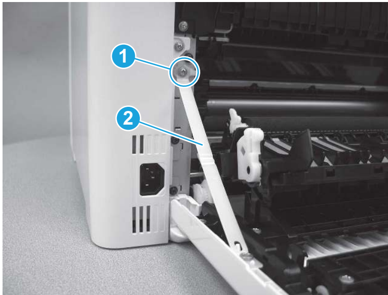
Figure 5-716 Remove one screw and release the arm
