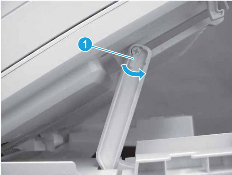
Figure 5-317 Release scanner support arm pin
