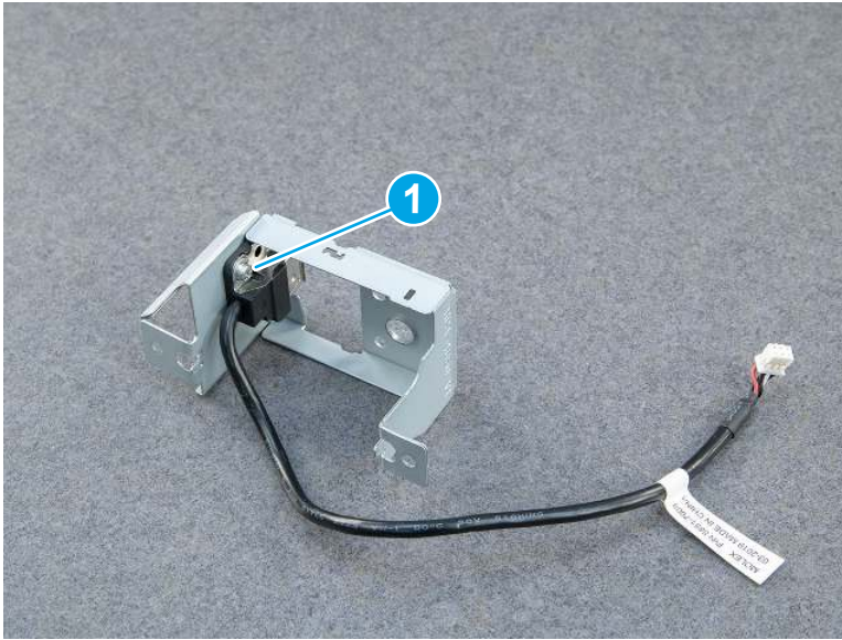
Figure 5-1979 Remove one screw and remove the USB connector
