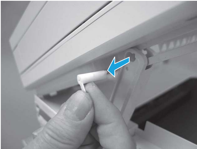
Figure 5-318 Remove the pin
