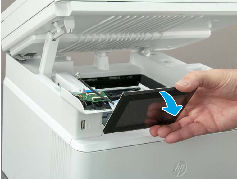
Figure 5-266 Remove the control-panel assembly
