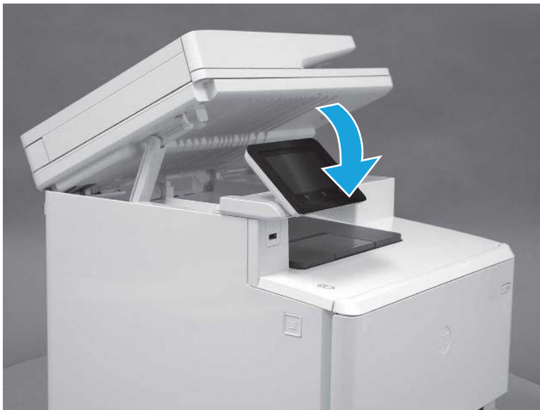
Figure 5-1732 Lower the scanner
