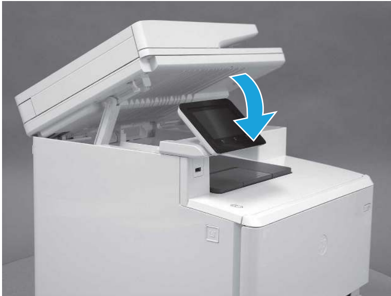
Figure 5-1702 Lower the scanner
