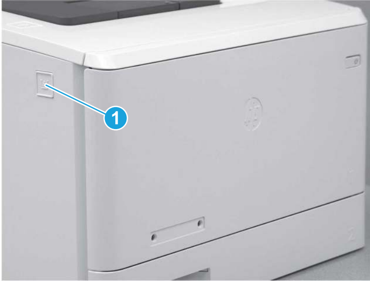
Figure 5-513 Release the front door
