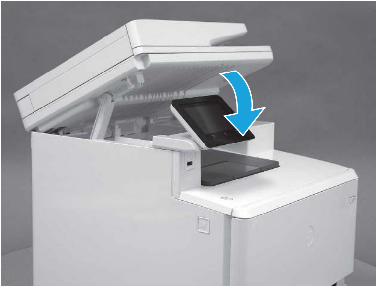
Figure 5-212 Lower the scanner
