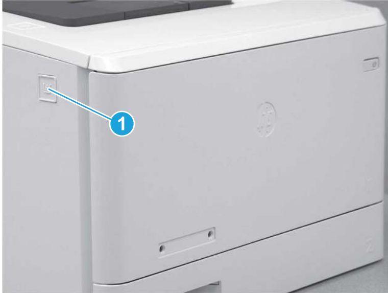
Figure 5-935 Release the front door
