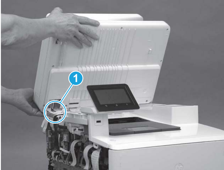
Figure 5-321 Release the cables
