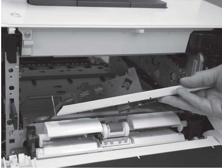
Figure 5-844 Remove the registration density sensor and guide
