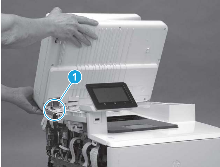
Figure 5-1763 Release the cables
