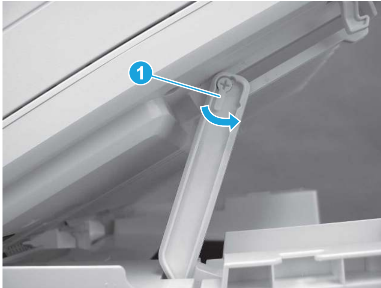
Figure 5-1446 Release scanner support arm pin
