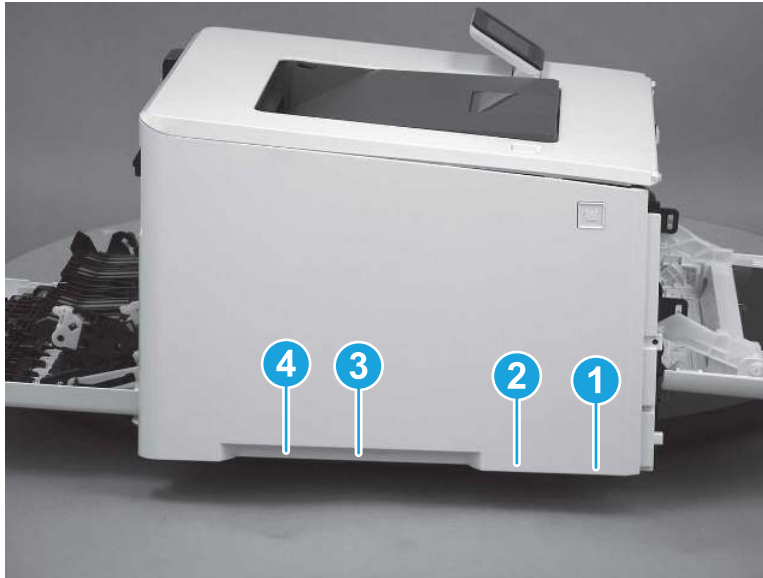
Figure 5-486 Release bottom tabs
