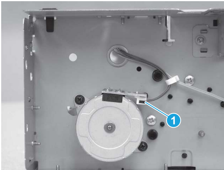
Figure 5-2154 Disconnect one connector
