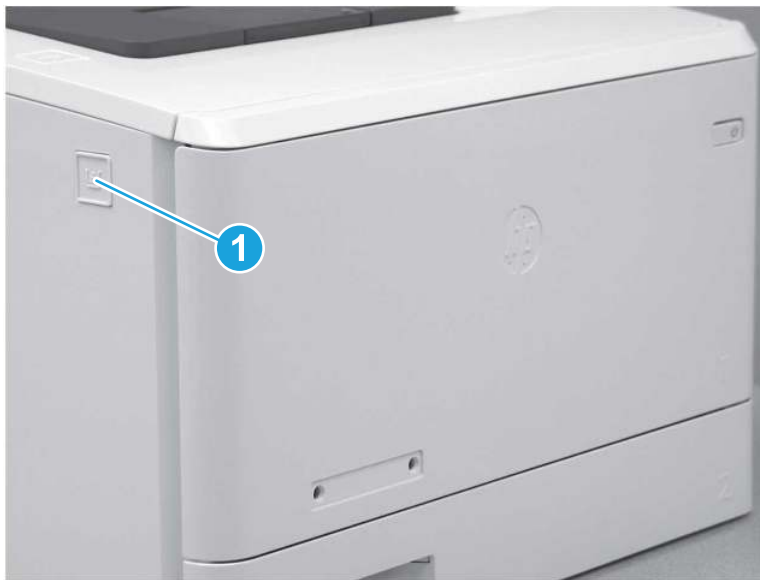
Figure 2-1 Release the front door
