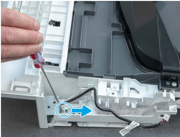
Figure 5-2035 Release the metal tab and lift to remove the USB
