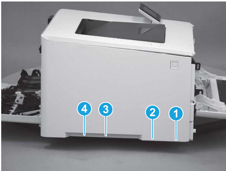
Figure 5-2044 Release bottom tabs
