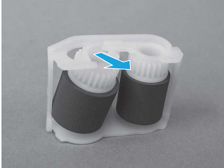
Figure 2-31 Remove the roller
