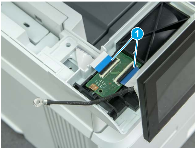
Figure 5-328 Disconnect two FFC
