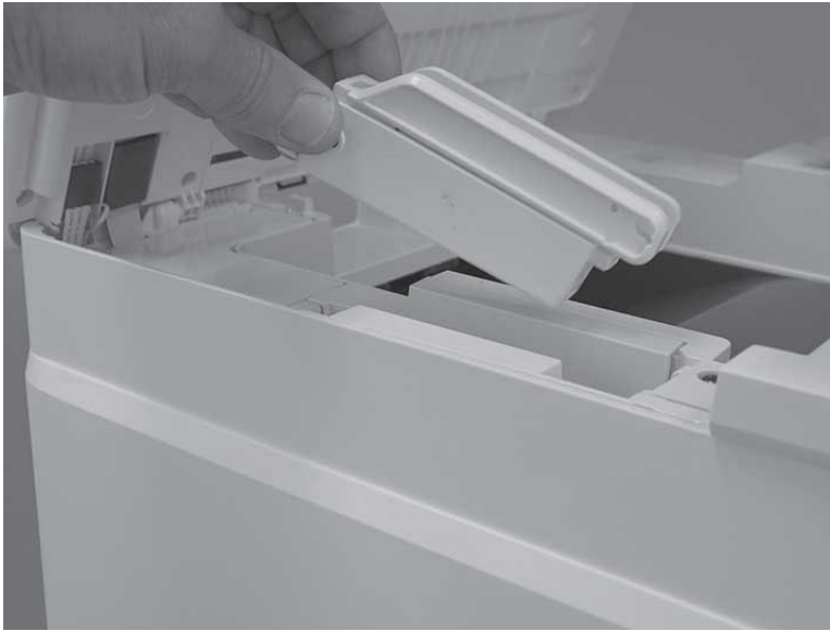
Figure 5-23 Remove the support arm
