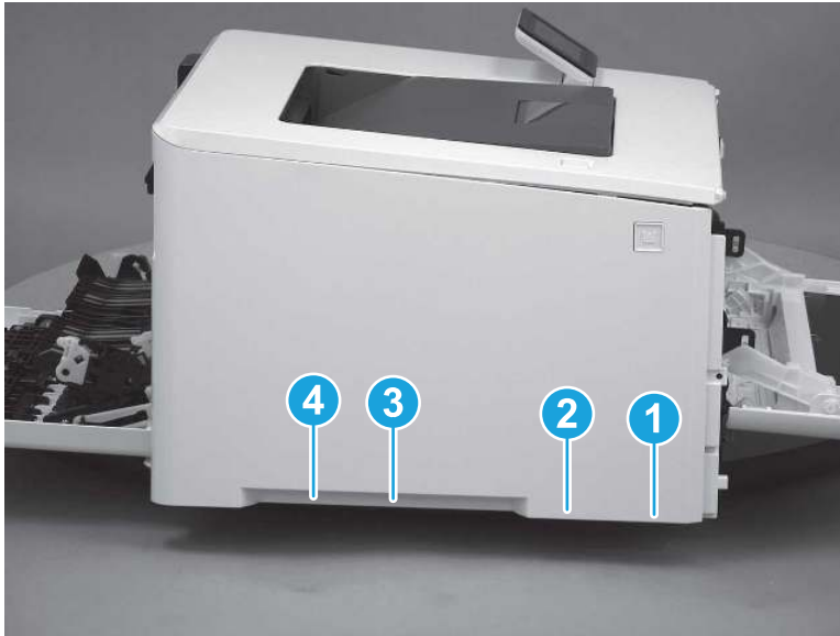
Figure 5-2064 Release bottom tabs
