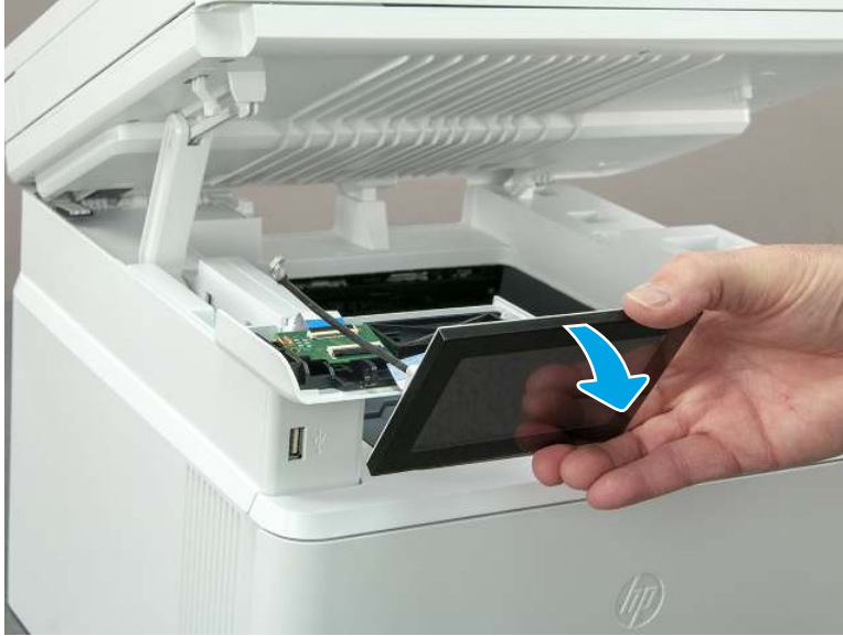
Figure 5-282 Remove the control-panel assembly
