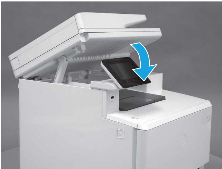
Figure 5-2003 Lower the scanner
