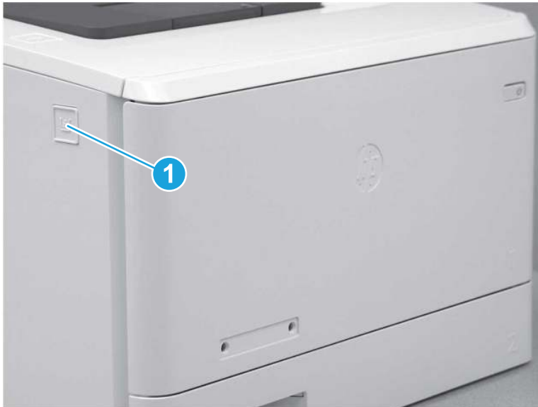
Figure 5-781 Release the front door
