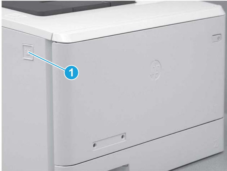
Figure 5-1094 Release the front door
