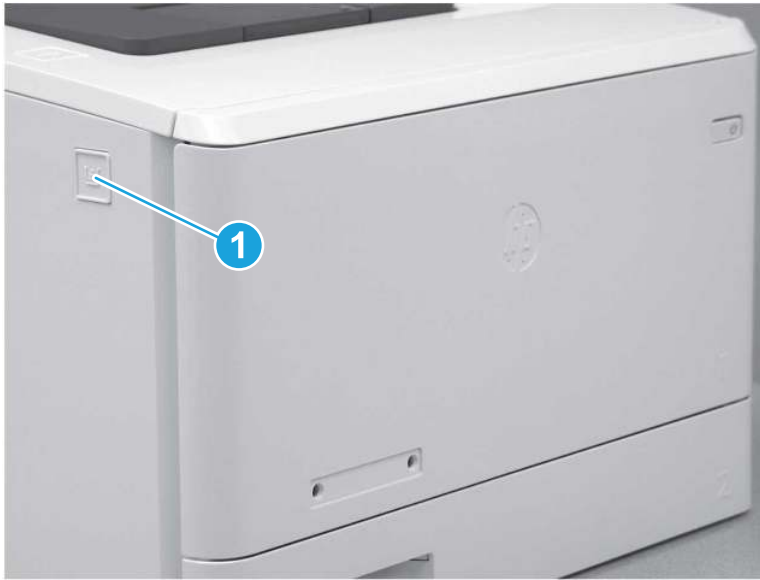
Figure 5-1398 Release the front door
