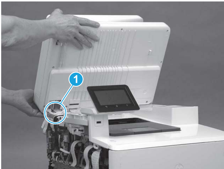
Figure 5-1650 Release the cables
