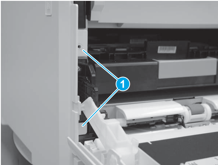
Figure 1-552 Release two tabs
