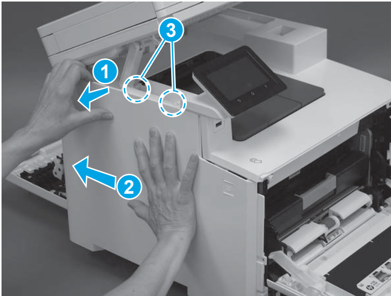
Figure 1-1794 Release one tab and two hooks
