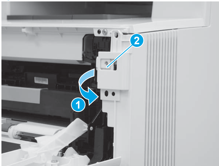
Figure 1-317 Rotate the front of the cover
