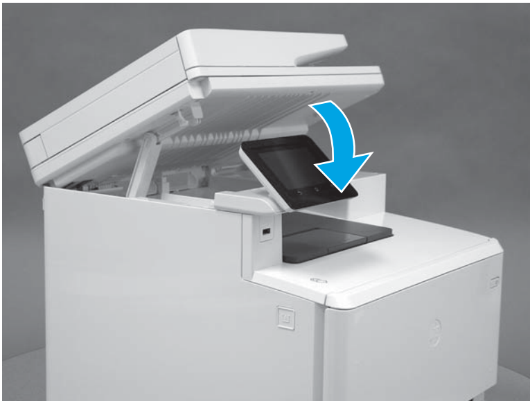
Figure 1-2053 Lower the scanner
