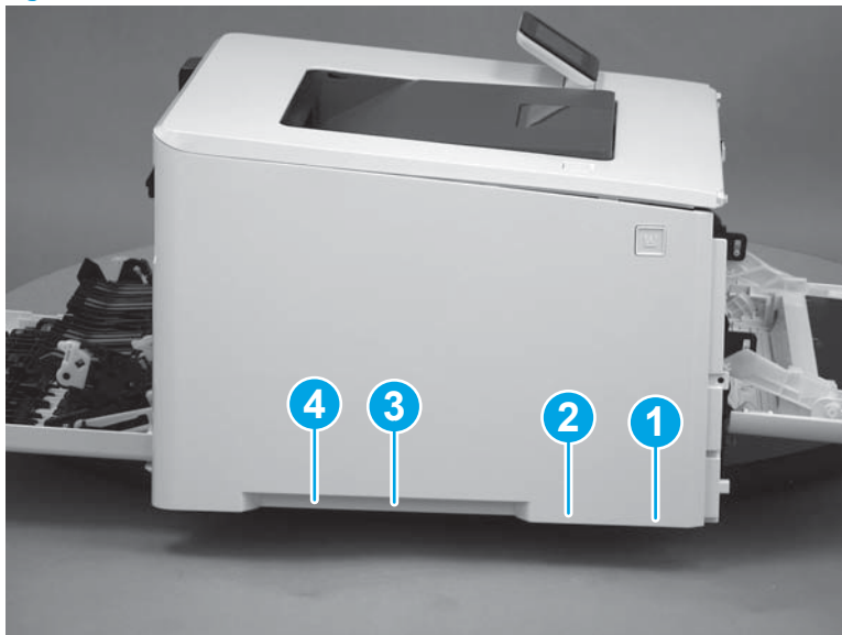
Figure 1-325 Release bottom tabs
