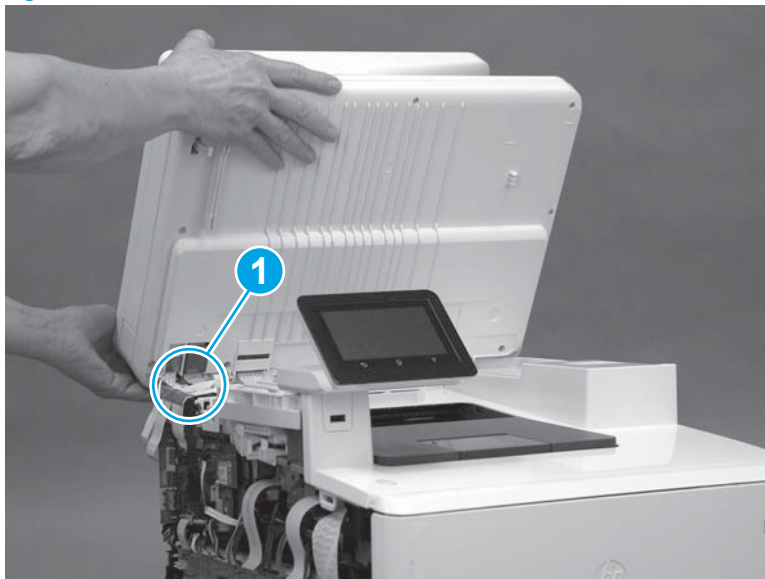
Figure 1-2225 Release the cables
