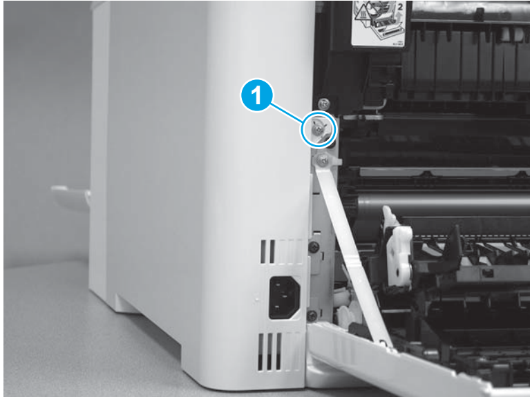
Figure 1-227 Remove one screw
