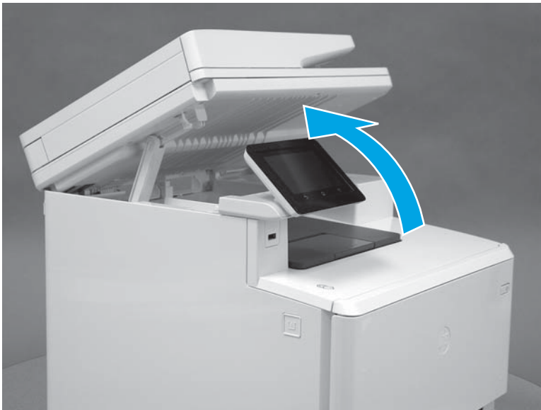
Figure 1-2195 Raise the scanner
