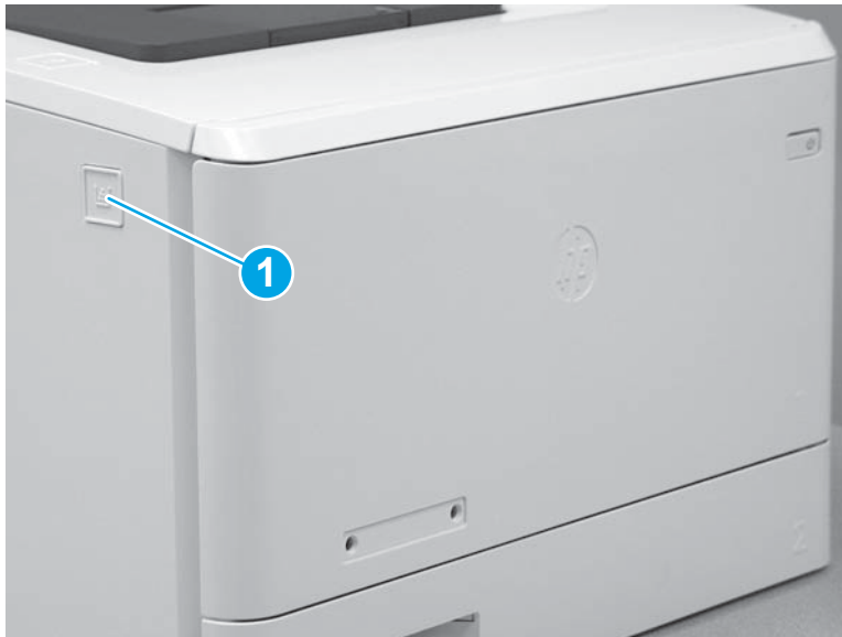
Figure 1-659 Release the front door
