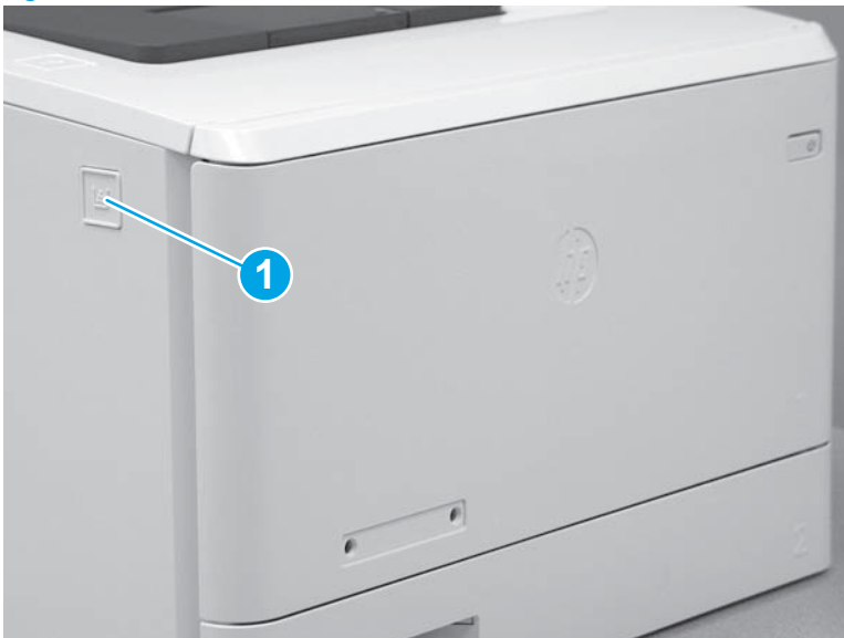
Figure 1-690 Release the front door
