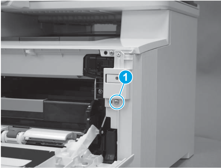
Figure 1-1049 Remove one screw
