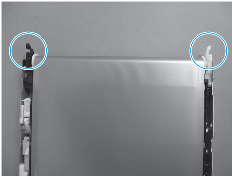
Figure 1-1030 Lower both tabs on each side of the ITB to the down position.
