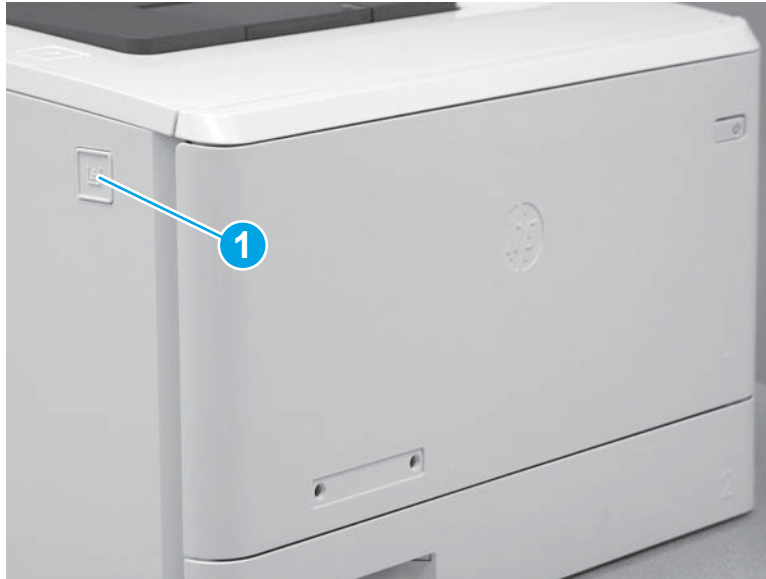
Figure 1-2301 Release the front door
