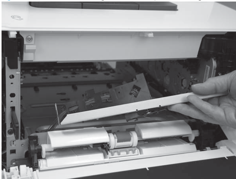
Figure 1-1104 Remove the registration density sensor and guide
