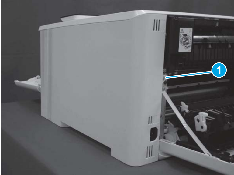
Figure 1-2400 Remove one screw
