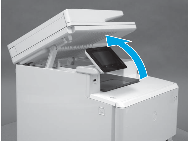
Figure 1-226 Raise the scanner
