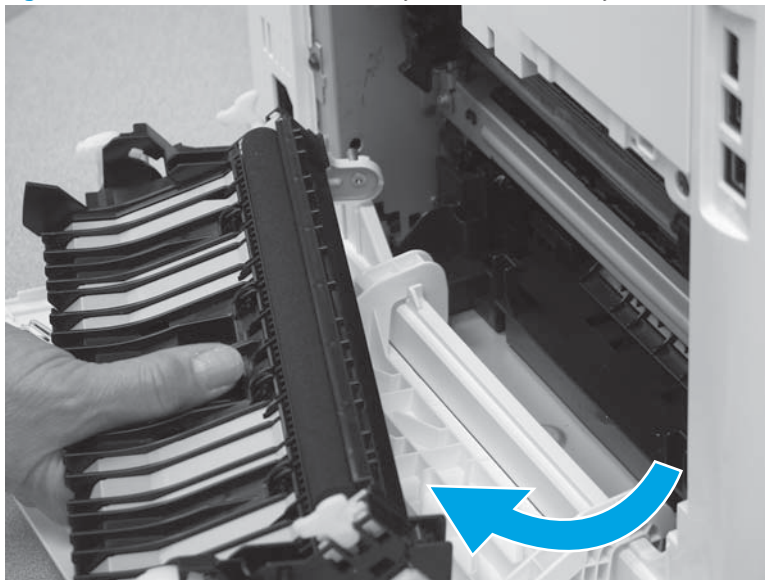
Figure 1-1076 Remove the secondary transfer assembly
