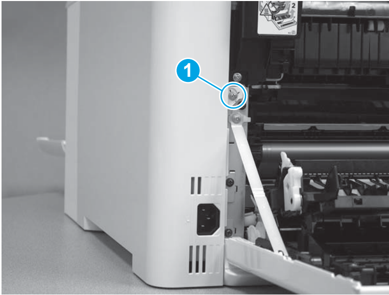
Figure 1-815 Remove one screw
