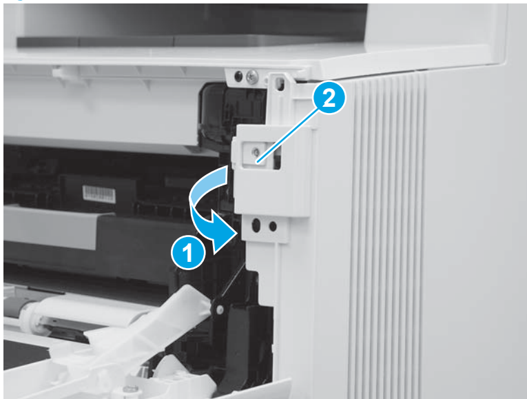
Figure 1-1212 Rotate the front of the cover
