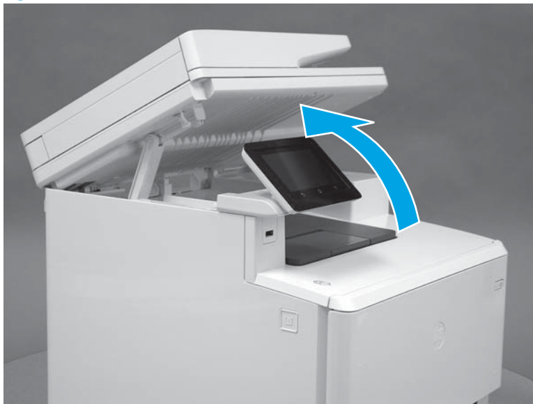
Figure 1-758 Raise the scanner
