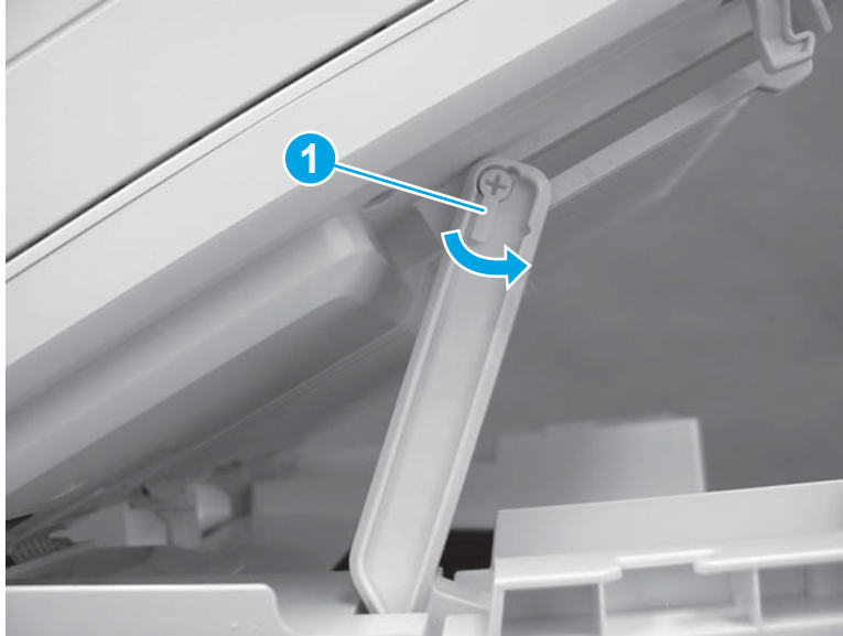
Figure 1-412 Release the scanner arm pin
