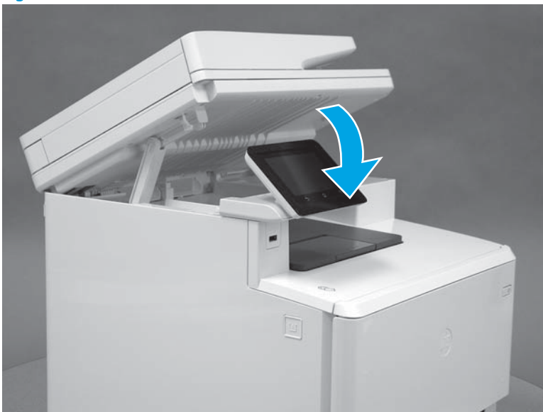
Figure 1-1298 Lower the scanner
