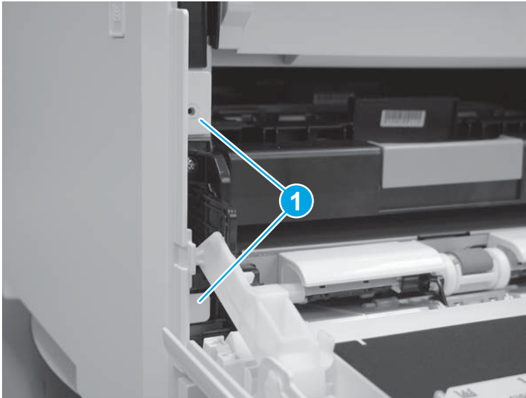
Figure 1-1000 Release two tabs
