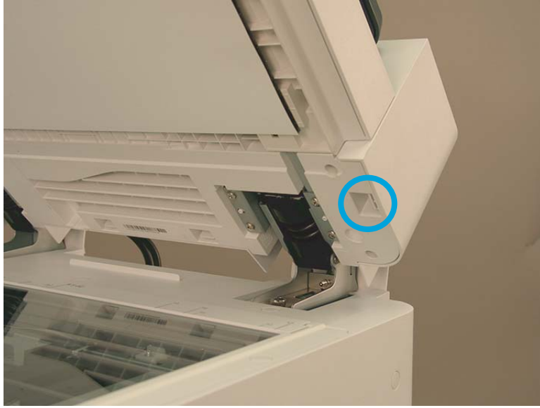
Figure 2-889 Release one tab on the right side of back cover.
