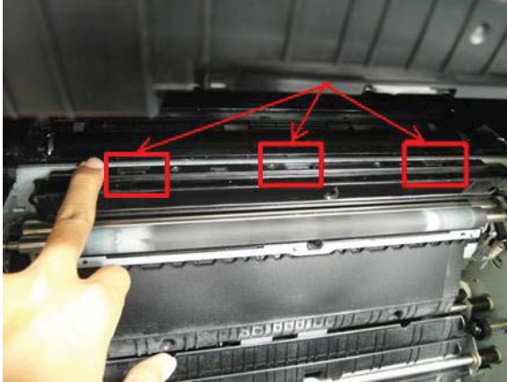
Figure 2-394 Clean the CPR sensors
