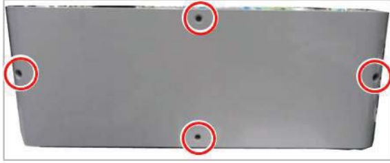
Figure 2-1075 Remove the DCF rear cover
