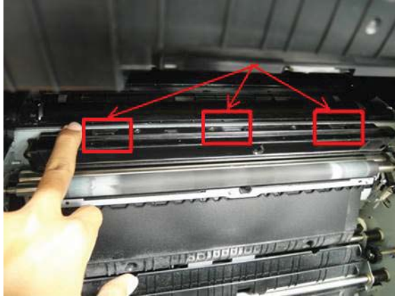
Figure 2-50 Clean the CPR sensors
