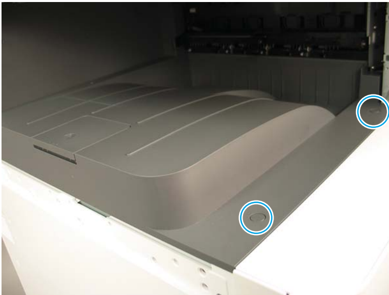
Figure 2-631 Remove the exit cover
