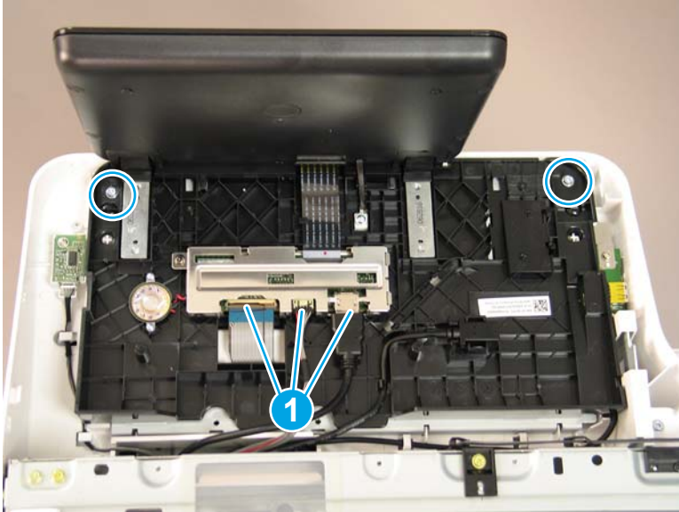
Figure 2-143 Remove the control panel screws and disconnect connectors
