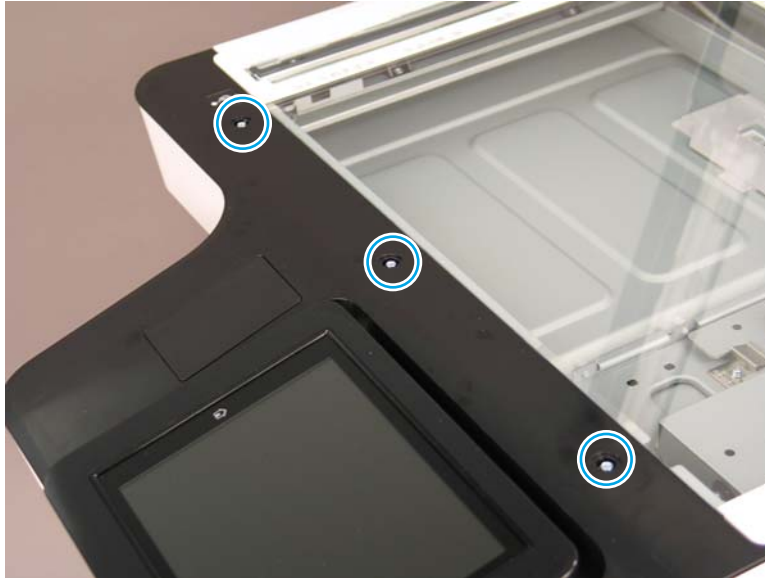
Figure 2-145 Remove the document feeder bezel
