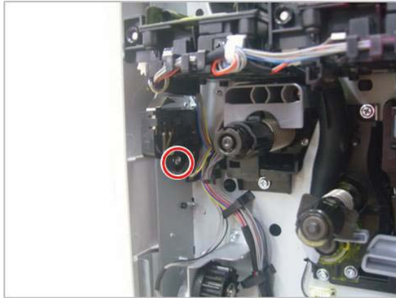
Figure 2-340 Remove one screw and the cover open sensor
