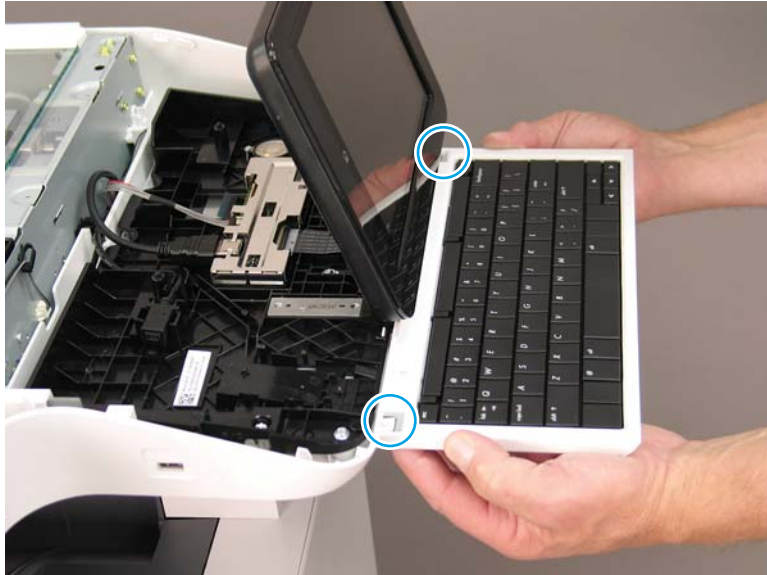
Figure 2-149 Remove the control-panel keyboard
