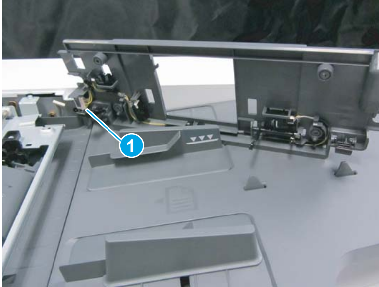
Figure 2-866 Turn the cover over and disconnect connector
