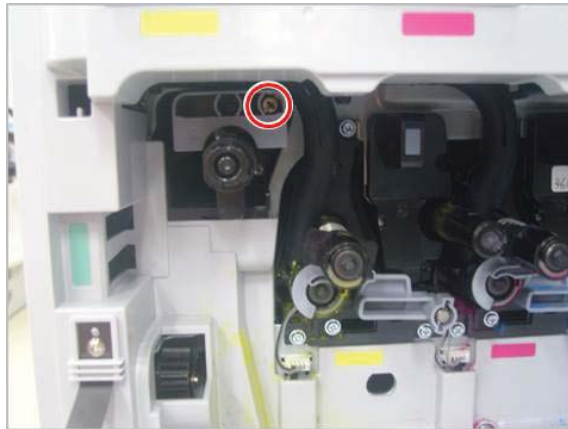
Figure 2-389 ITB screw location
