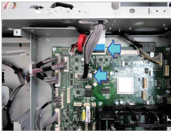
Figure 2-73 Disconnect scan cables
