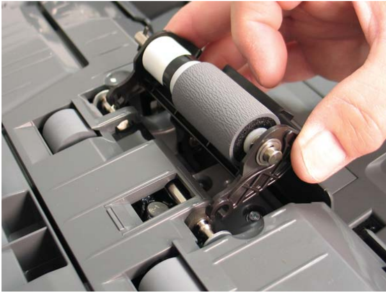
Figure 2-964 Remove the separation roller
