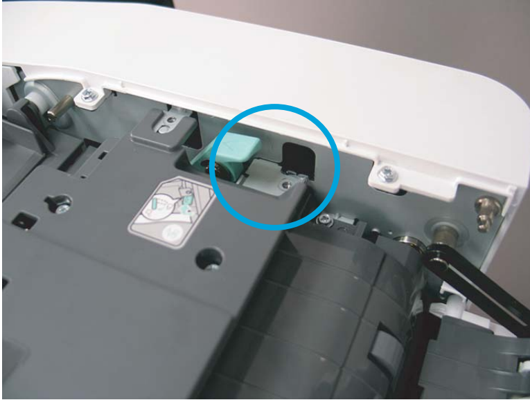
Figure 2-955 Rotate pick/feed roller assembly to release sheet metal tab from ADF frame.
