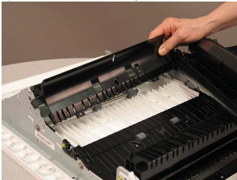
Figure 2-681 Remove the duplex lower guide
