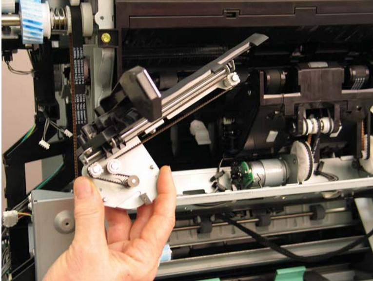
Figure 5-442 Remove the rear tamper
