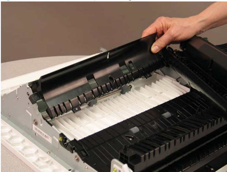
Figure 2-712 Remove the duplex lower guide
