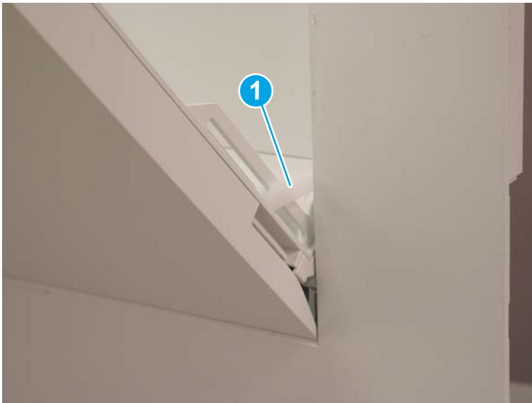
Figure 2-732 Release the hinge arm
