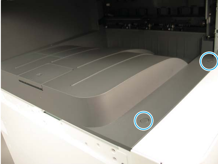
Figure 2-350 Remove the exit cover
