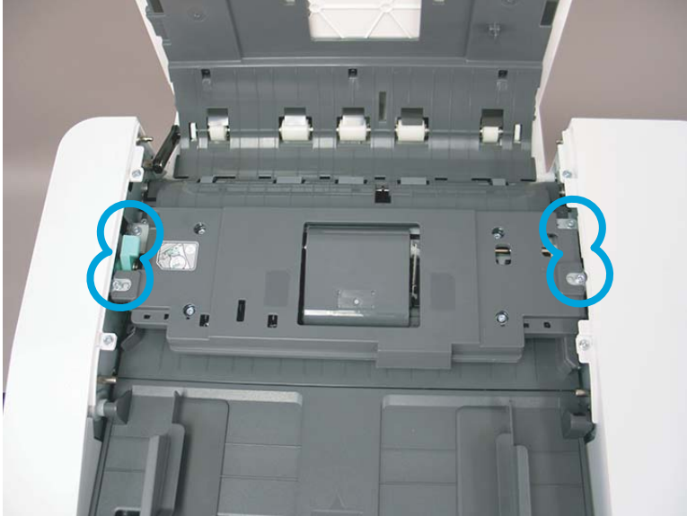
Figure 2-951 Remove four screws.
