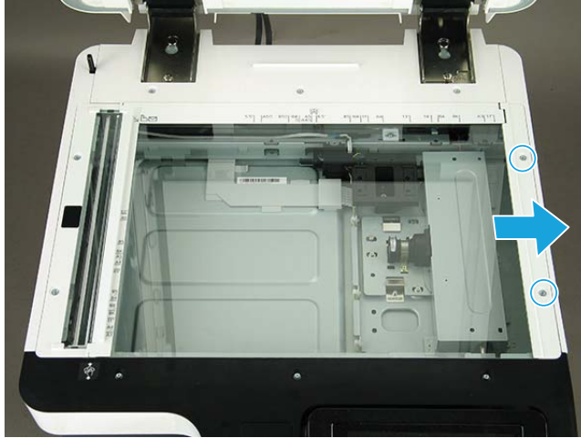
Figure 2-1034 Remove scanner glass
