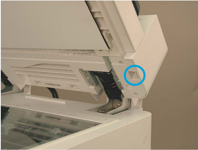
Figure 2-1012 Release one tab on the right side of back cover.
