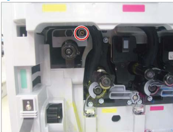
Figure 2-45 ITB screw location
