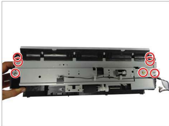
Figure 2-813 Remove seven screws
