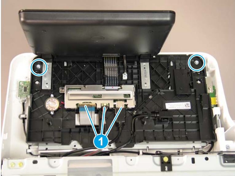
Figure 2-146 Remove the control panel screws and disconnect connectors
