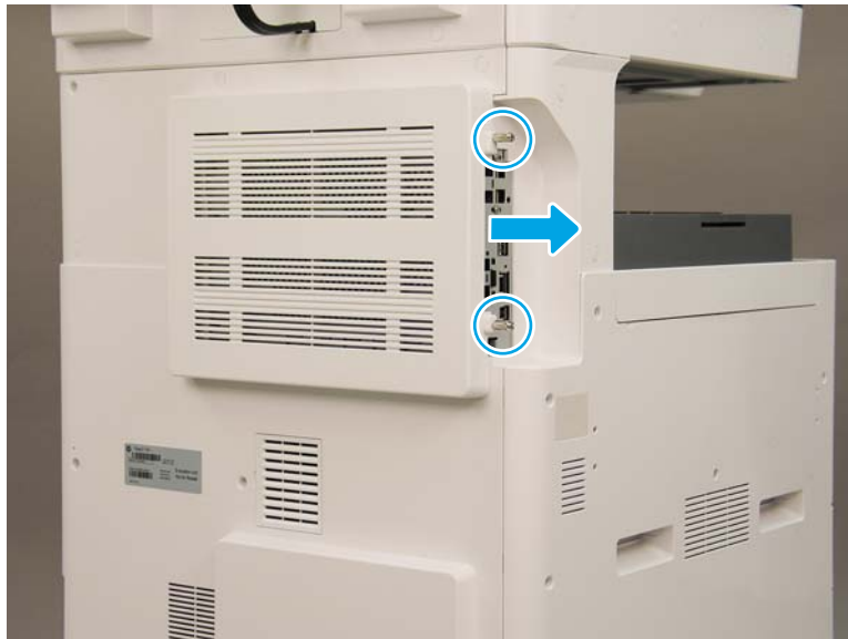
Figure 2-550 Remove the formatter cover
