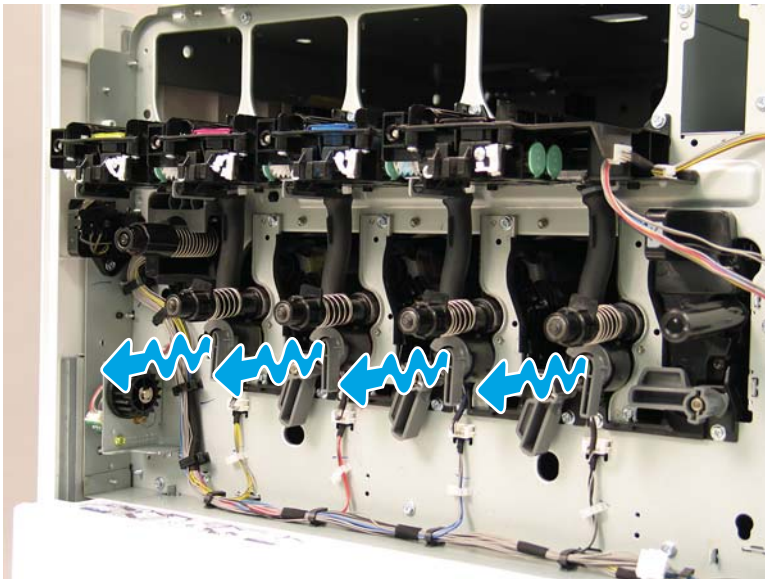
Figure 2-411 Release the toner supply pipes
