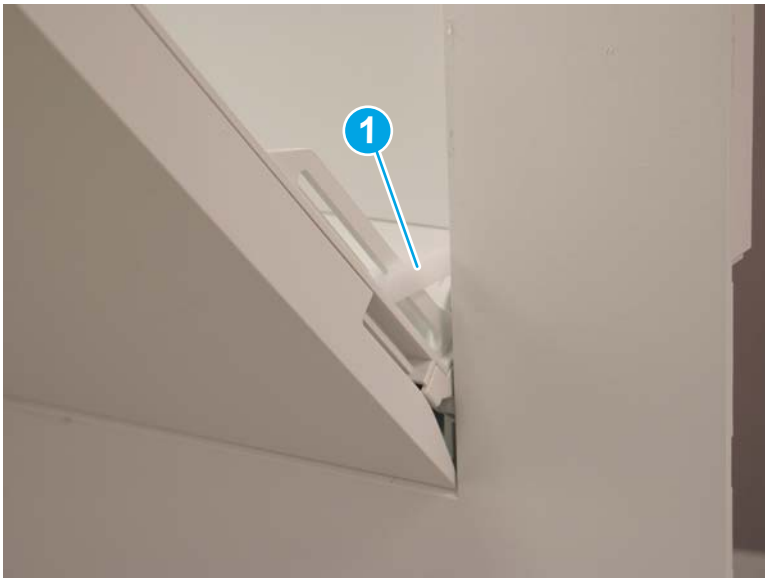
Figure 2-700 Release the hinge arm
