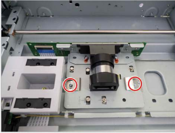
Figure 2-1052 Remove screws and release scanner imaging unit
