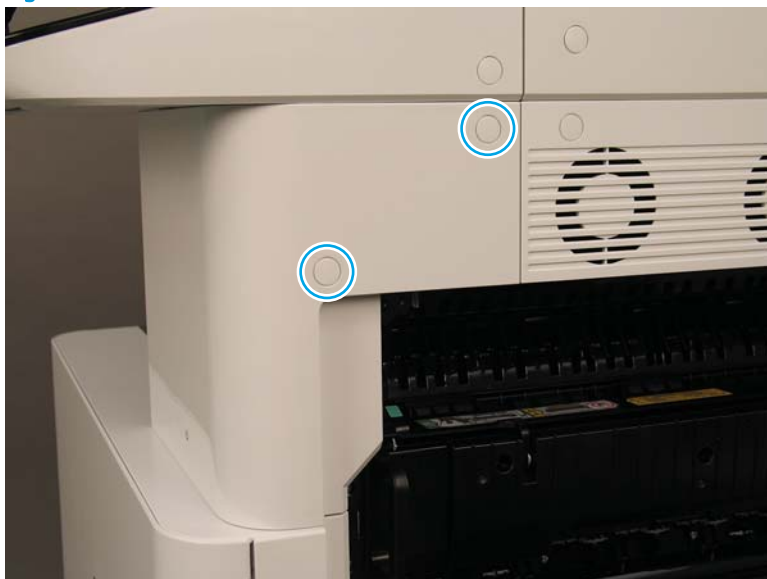
Figure 2-162 Remove two screws and rotate the cover
