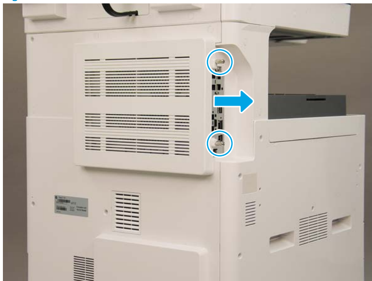
Figure 2-1035 Remove the formatter cover
