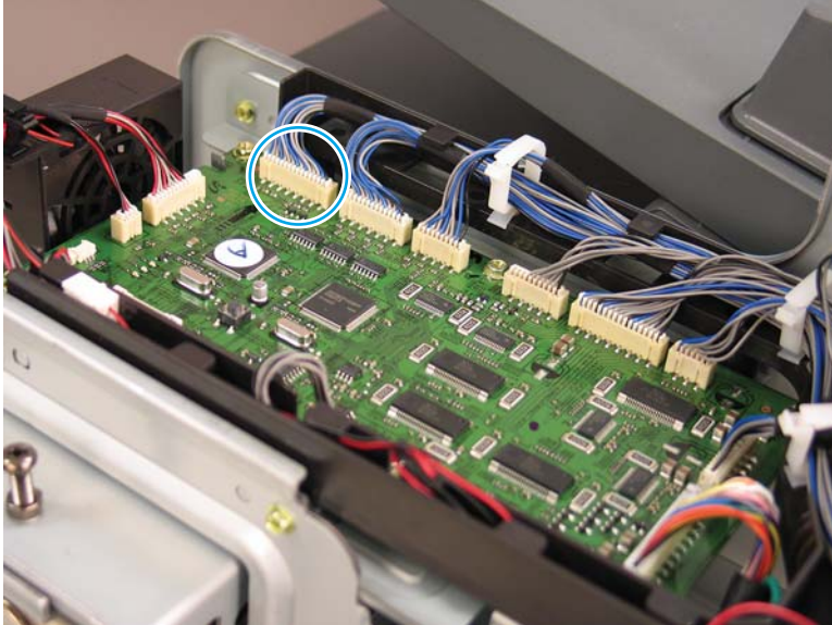
Figure 2-959 Disconnect the document feeder PCA connector
