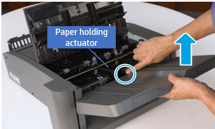
Figure 6-721 Remove the output tray
