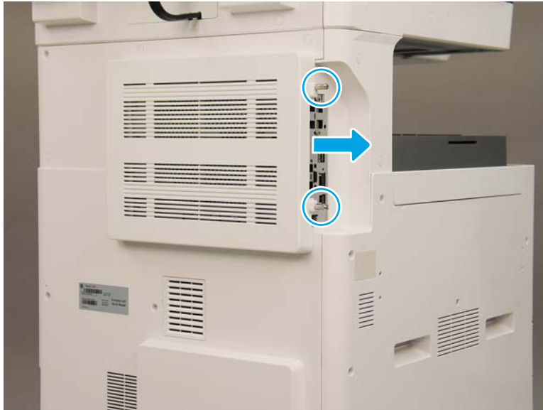
Figure 2-896 Remove the formatter cover and the upper rear cover
