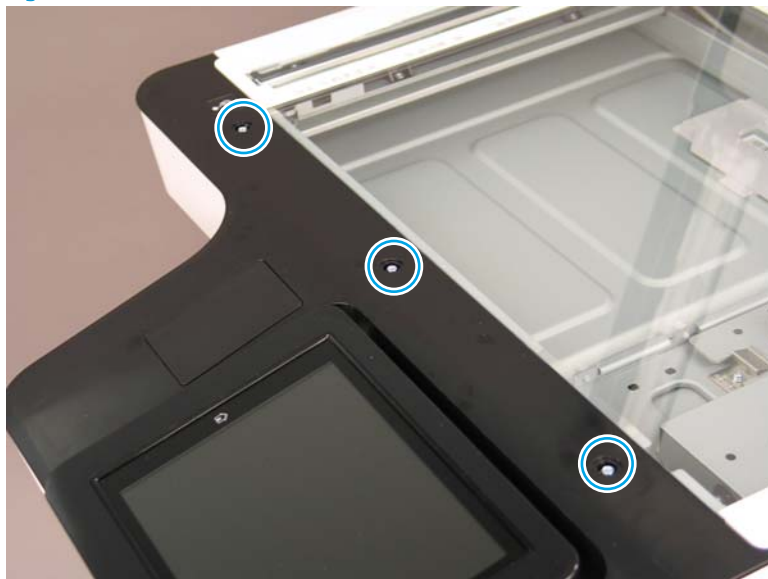
Figure 2-142 Remove the document feeder bezel
