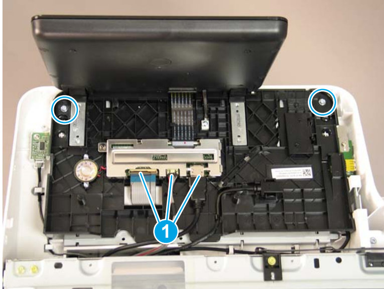
Figure 2-66 Remove the control panel screws and disconnect connectors
