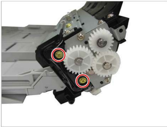
Figure 2-811 Remove two screws and three gears
