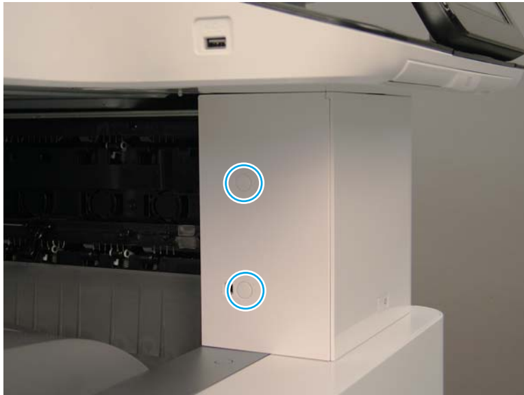
Figure 2-91 Remove the front top inner cover
