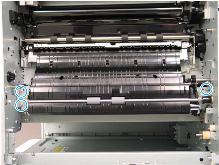
Figure 2-575 Remove three screws
