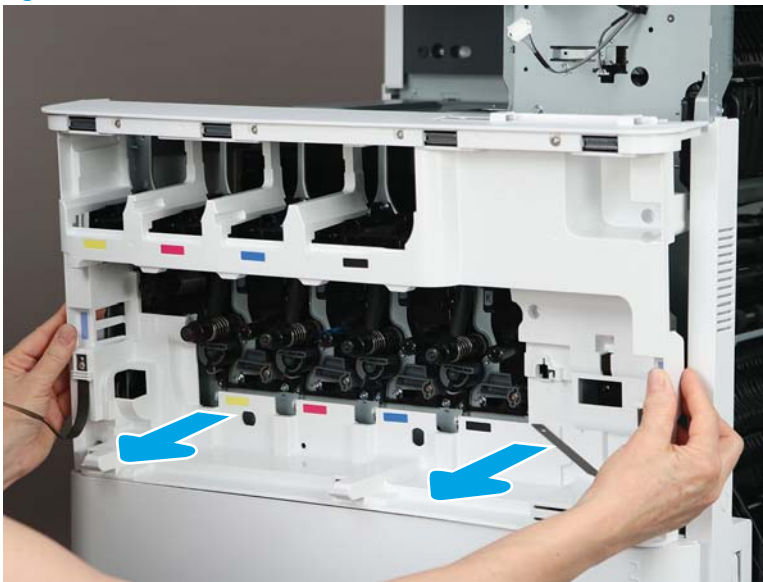
Figure 2-548 Remove the inner cover
