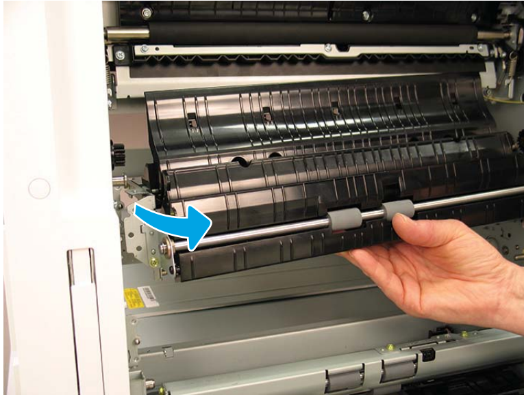
Figure 2-591 Rotate pickup unit 1
