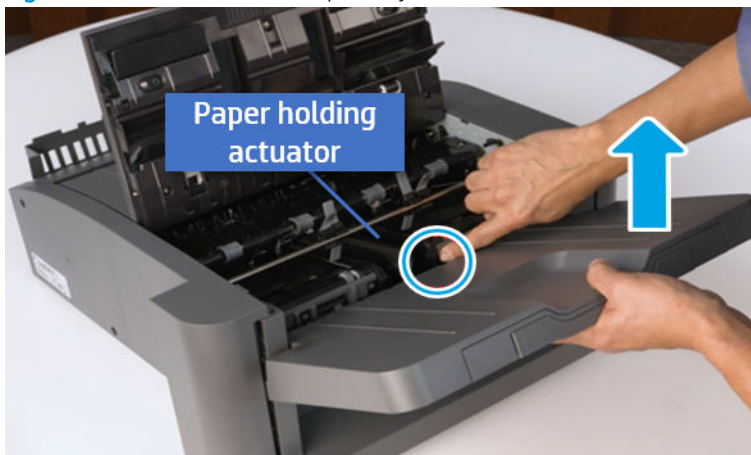
Figure 6-495 Remove the output tray
