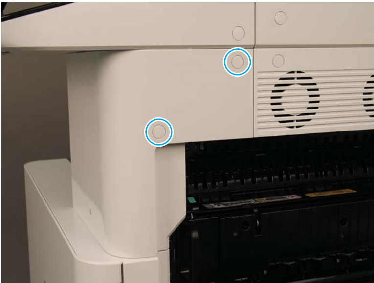
Figure 2-335 Remove two screws and rotate the cover
