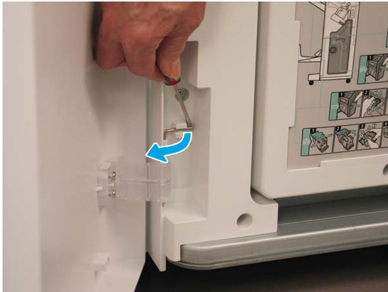
Figure 5-127 Release the lower hinge pin
