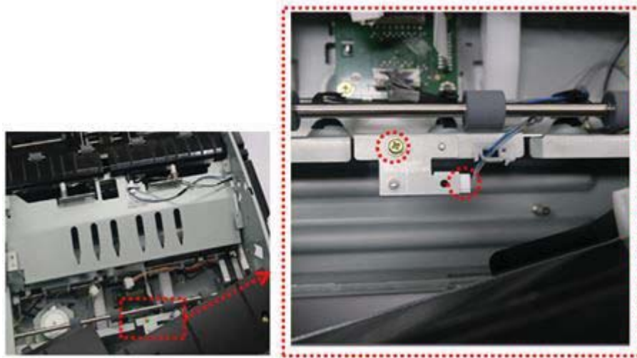
Figure 6-897 Remove the punch dust full sensor sub-assembly
