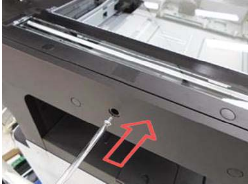
Figure 1-48 Tighten scan locking screw
