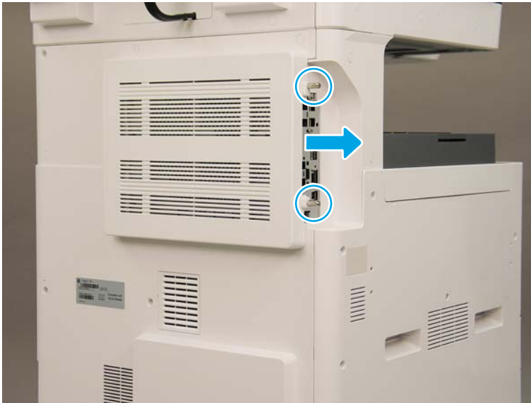
Figure 2-640 Remove the formatter cover
