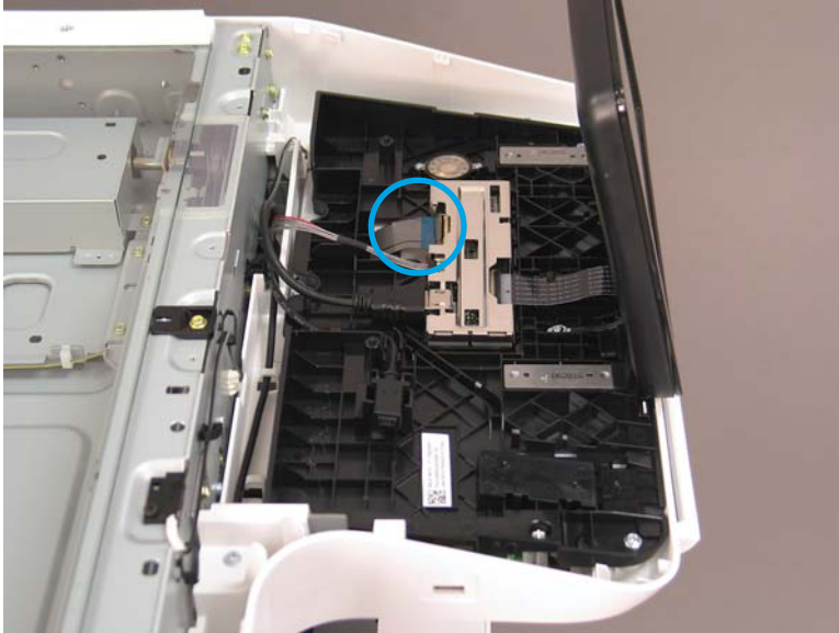
Figure 2-68 Disconnect one FFC
