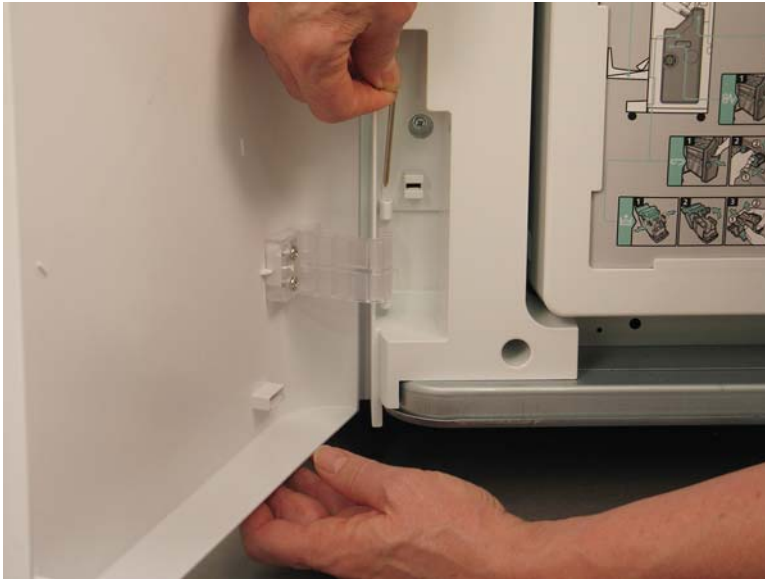
Figure 5-193 Remove the lower hinge pin
