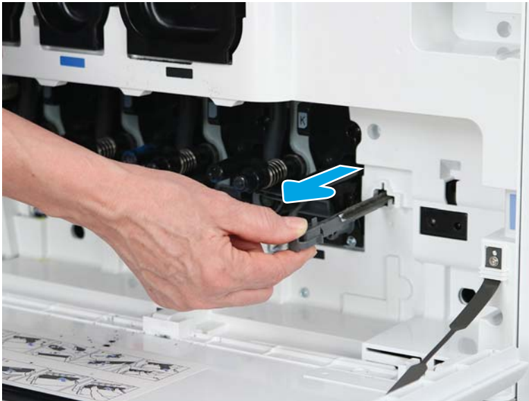
Figure 2-403 Remove the paper dust brush
