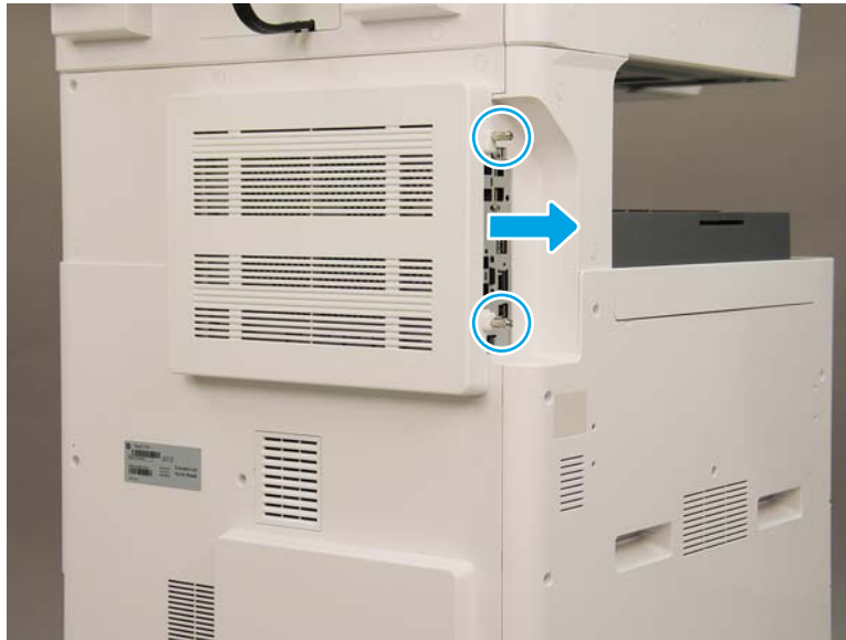
Figure 2-137 Remove the formatter cover
