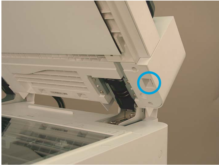
Figure 2-930 Release one tab on the right side of back cover.
