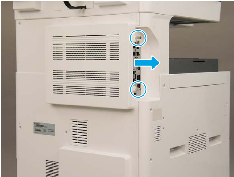
Figure 2-488 Remove the formatter cover
