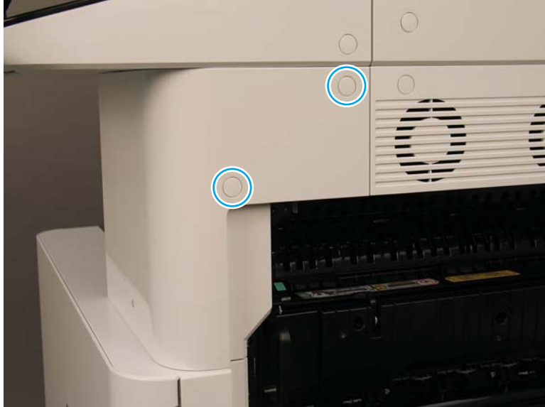
Figure 2-459 Remove two screws and rotate the cover
