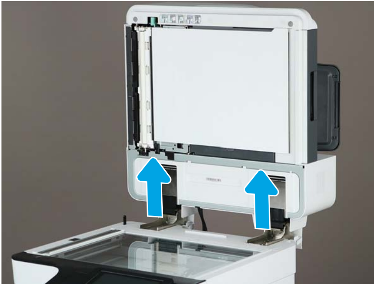
Figure 2-1027 Remove two screw and lift up to remove ADF
