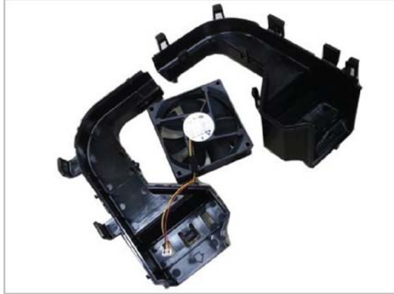
Figure 2-118 Remove the fuser fan
