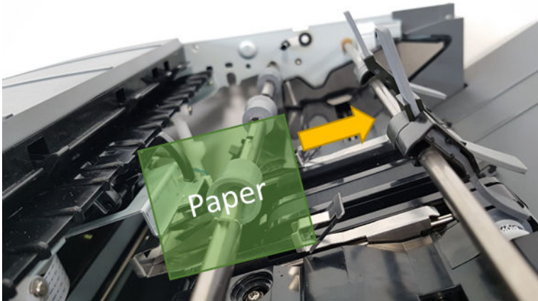
Figure 6-57 Inner finisher - ejector operation 1
