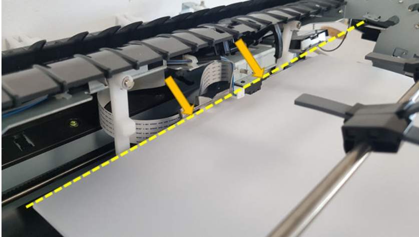
Figure 6-45 Inner finisher - end fence operation 1
