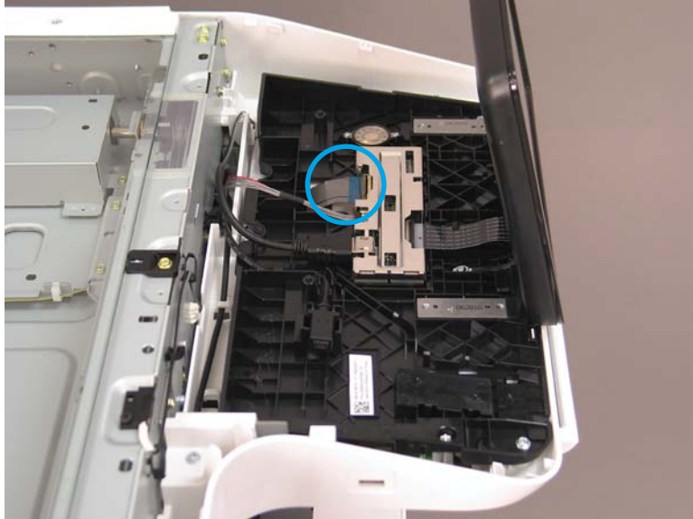
Figure 2-148 Disconnect one FFC
