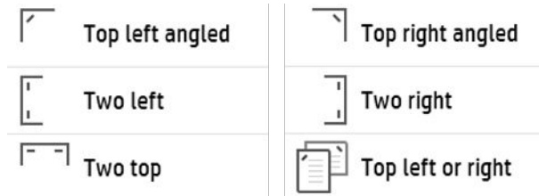
Figure 6-47 Inner finisher system - stapling options
