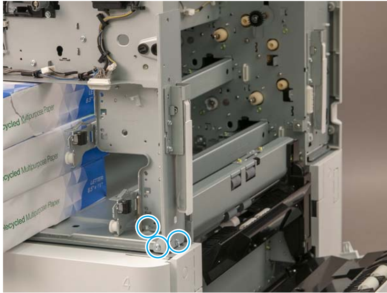
Figure 2-376 Remove three screws
