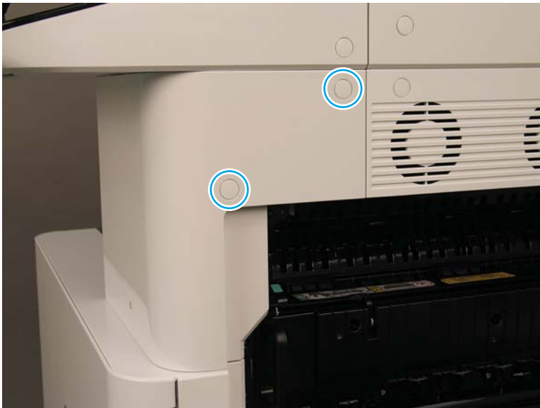
Figure 2-635 Remove two screws and rotate the cover
