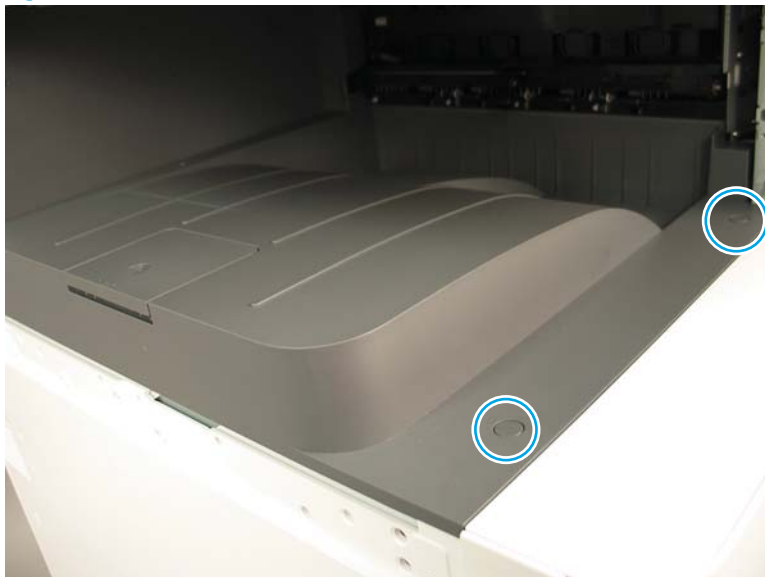
Figure 2-639 Remove the exit cover
