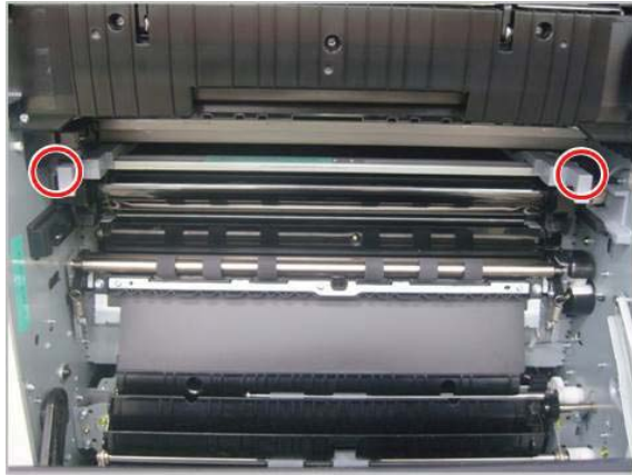
Figure 2-392 Remove two screws
