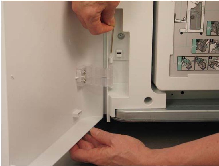
Figure 5-72 Remove the lower hinge pin
