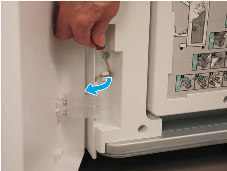
Figure 5-40 Release the lower hinge pin
