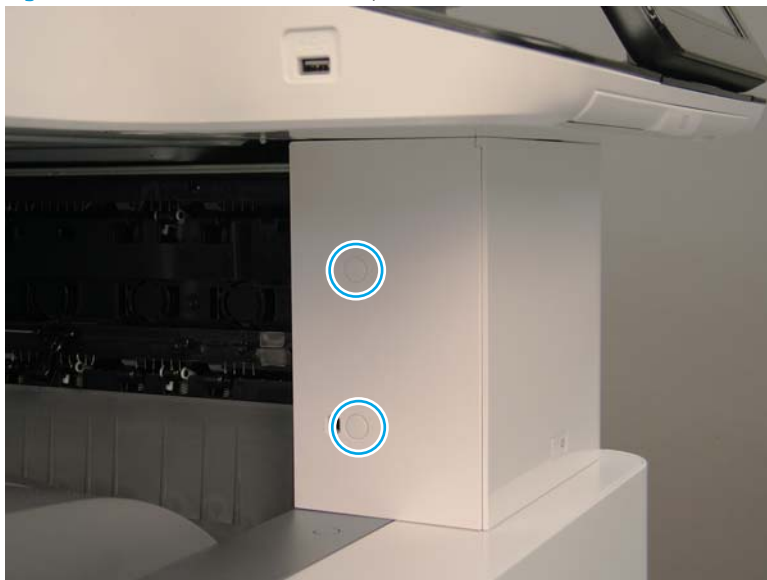
Figure 2-161 Remove the front top inner cover
