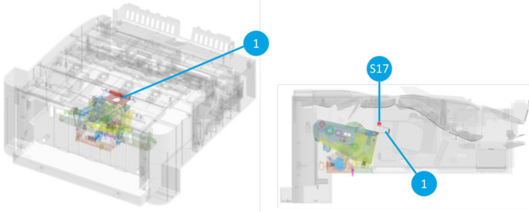
Figure 6-44 Inner finisher system - end fence unit detail view
