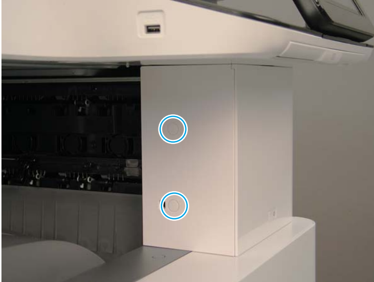
Figure 2-634 Remove the front top inner cover
