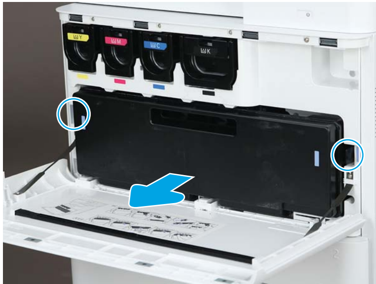
Figure 2-455 Remove the TCU
