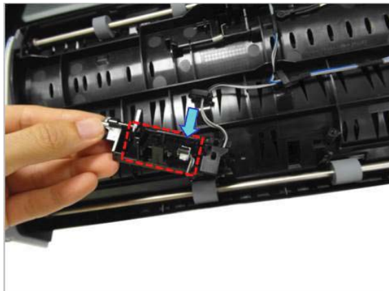
Figure 2-248 Remove the duplex 1 sensor
