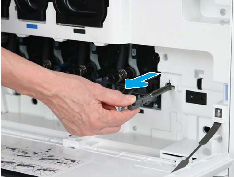
Figure 2-456 Remove the paper dust brush
