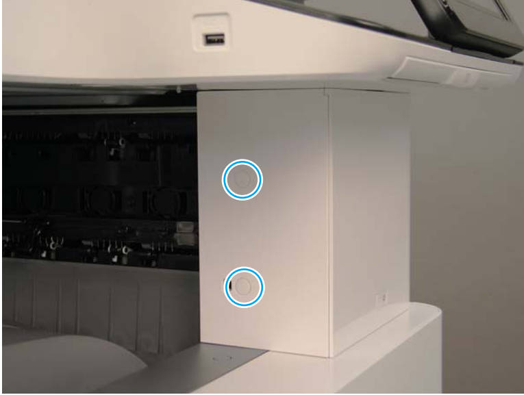
Figure 2-384 Remove the front top inner cover
