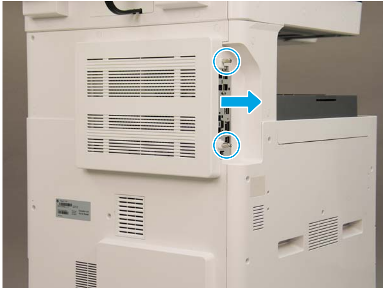
Figure 2-139 Remove the formatter cover
