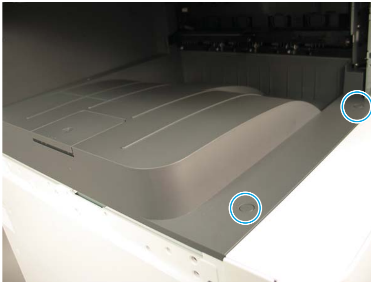
Figure 2-216 Remove the exit cover
