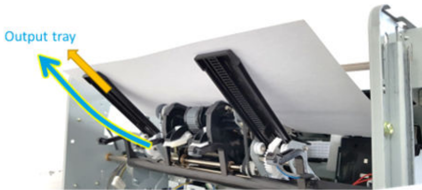
Figure 6-30 Inner finisher - paper support operation
