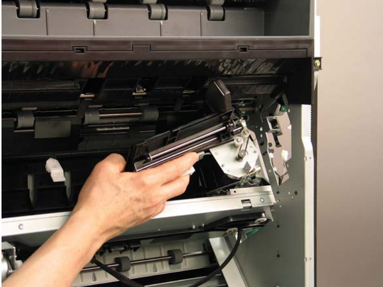
Figure 5-276 Remove the front tamper
