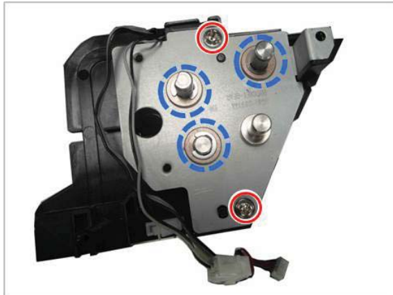
Figure 2-812 Remove the bracket-rear
