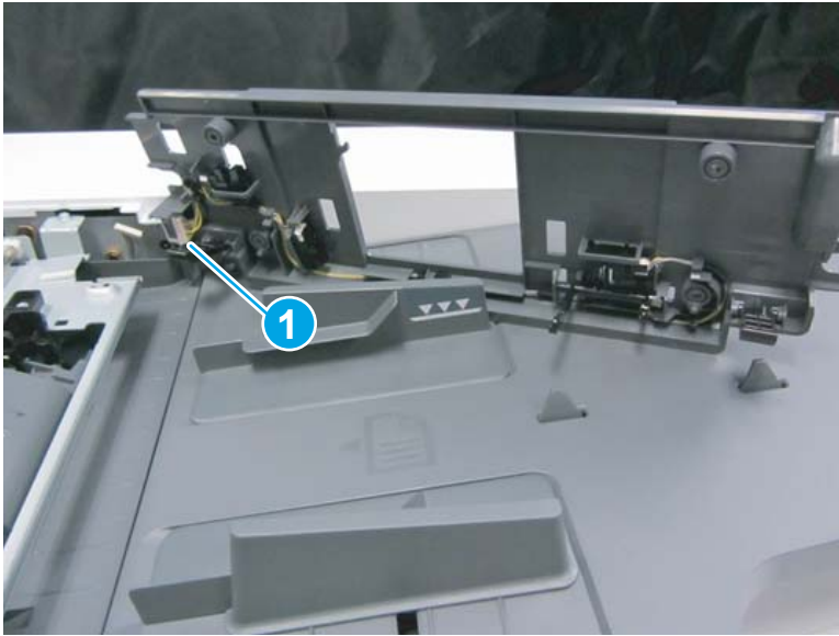
Figure 2-879 Turn the cover over and disconnect connector
