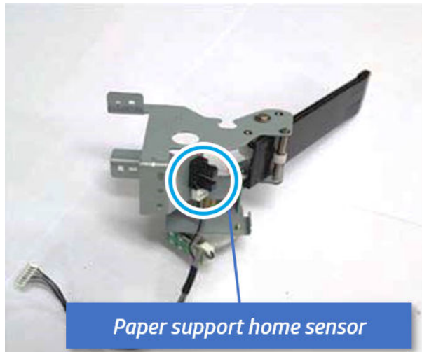
Figure 6-272 Remove the paper support home sensor
