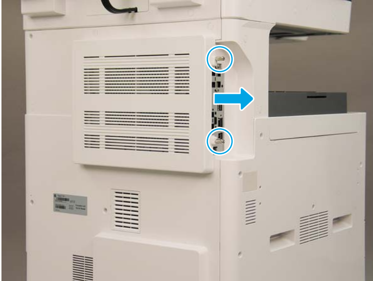
Figure 2-138 Remove the formatter cover
