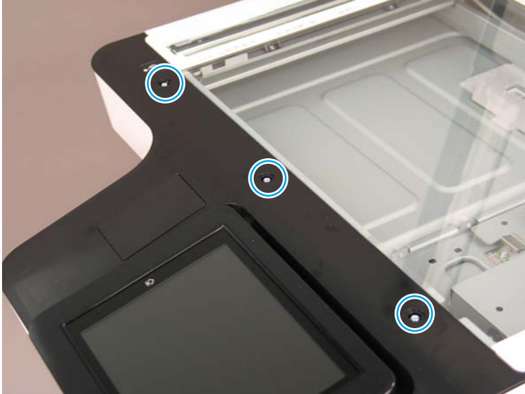
Figure 2-65 Remove the document feeder bezel
