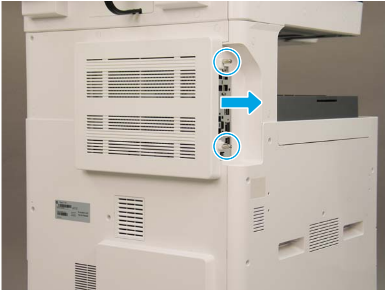
Figure 2-534 Remove the formatter cover
