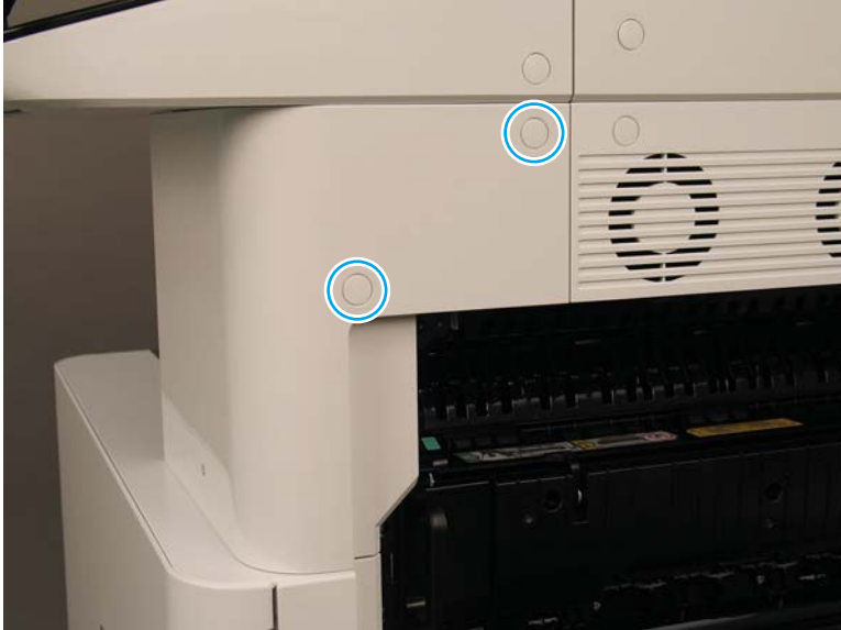
Figure 2-629 Remove two screws and rotate the cover
