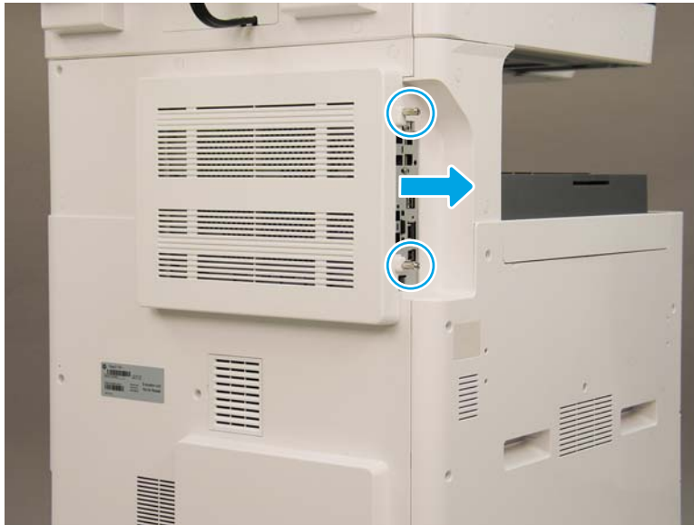
Figure 2-169 Remove the formatter cover
