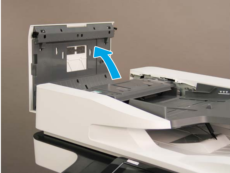
Figure 2-864 Open the document feeder cover
