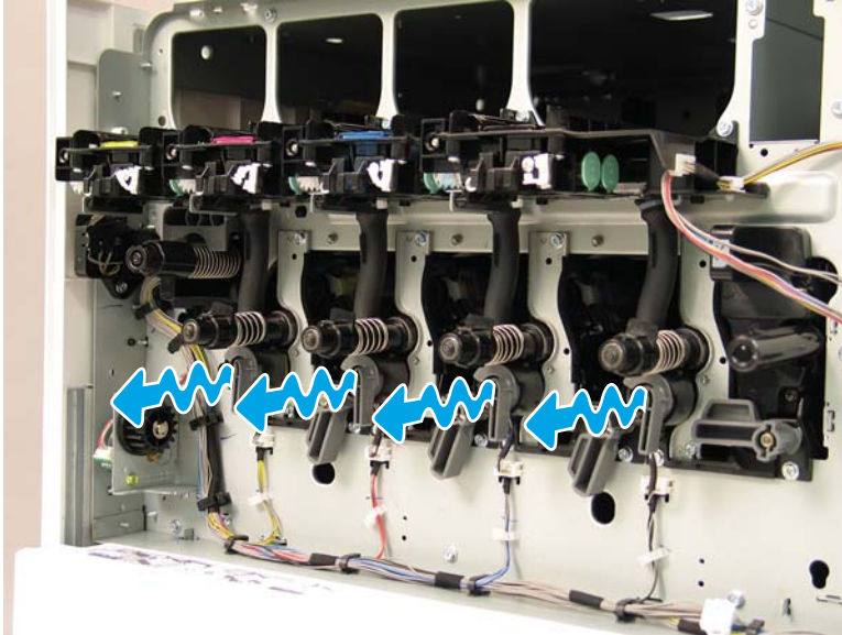
Figure 2-468 Release the toner supply pipes
