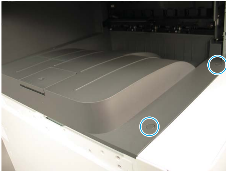
Figure 2-337 Remove the exit cover
