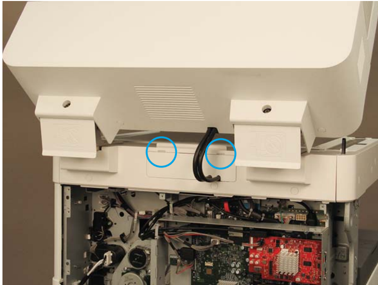
Figure 2-59 Remove document feeder connector cover
