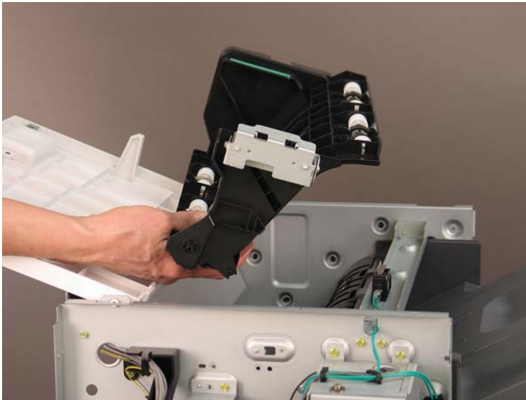
Figure 5-163 Remove the top jam access cover
