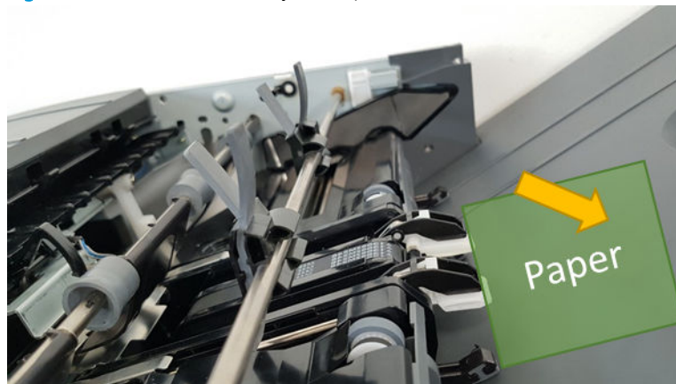
Figure 6-59 Inner finisher - ejector operation 3
