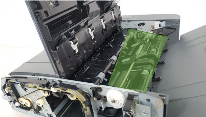
Figure 6-41 Inner finisher - tamper operation 1
