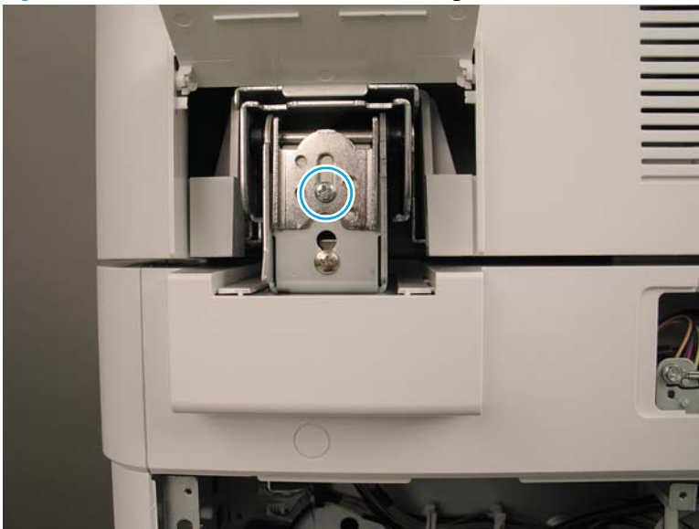
Figure 2-57 Release the document feeder hinge screws
