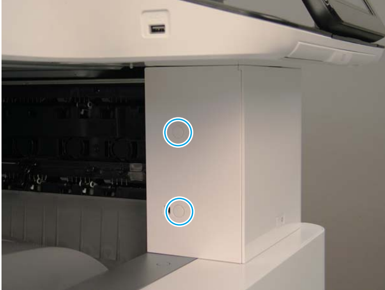
Figure 2-628 Remove the front top inner cover
