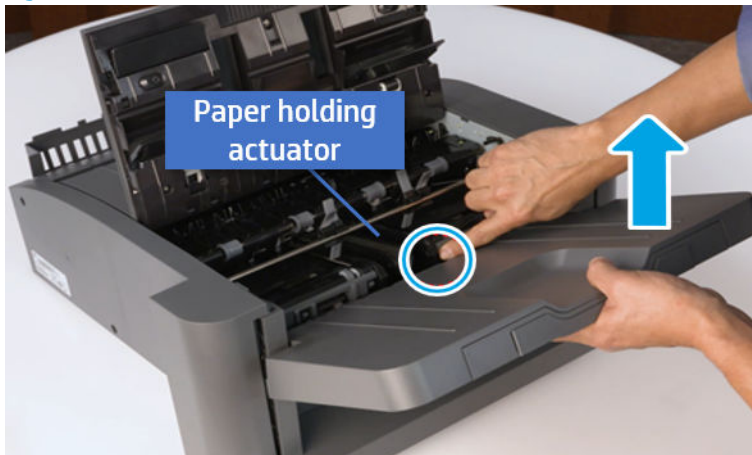
Figure 6-400 Remove the output tray
