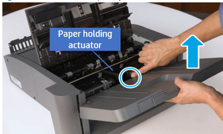
Figure 6-789 Remove the output tray
