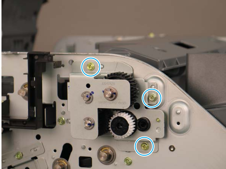
Figure 2-950 Remove the document feeder damping unit
