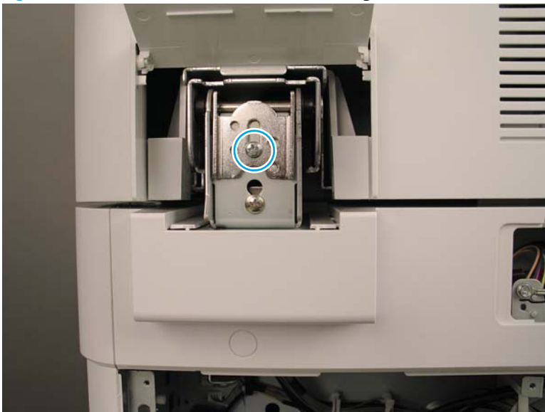
Figure 2-899 Release the document feeder hinge screws
