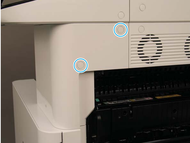
Figure 2-240 Remove two screws and rotate the cover
