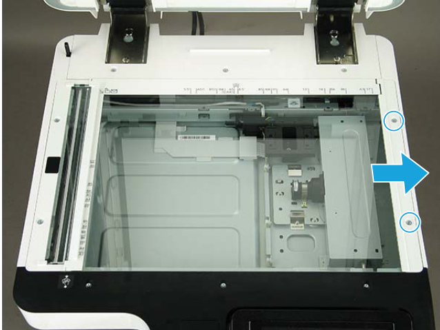
Figure 2-1044 Remove scanner glass
