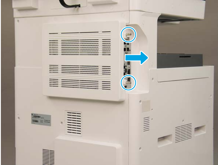
Figure 2-174 Remove the formatter cover
