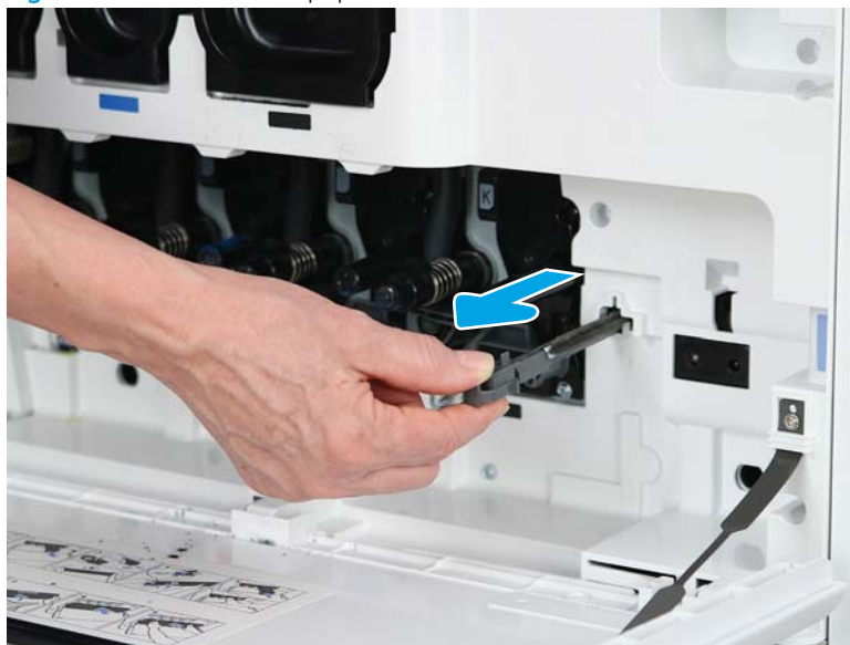
Figure 2-40 Remove the paper dust brush
