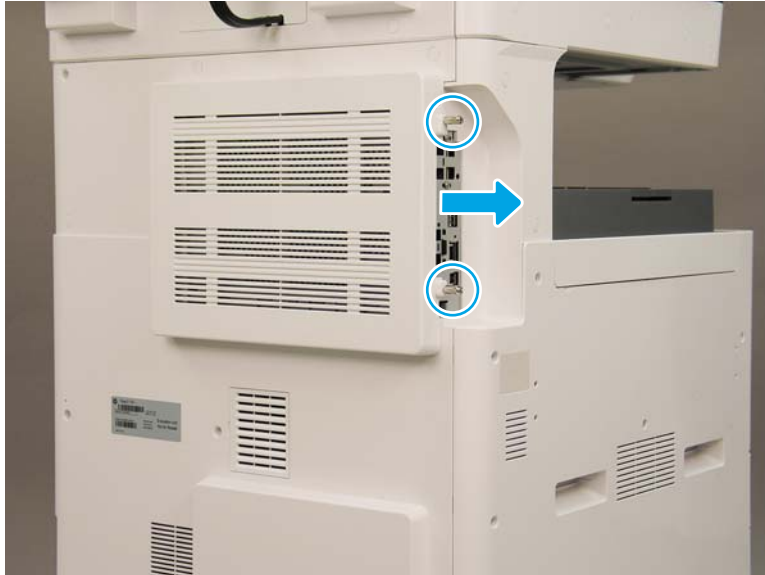
Figure 2-54 Remove the formatter cover and the upper rear cover
