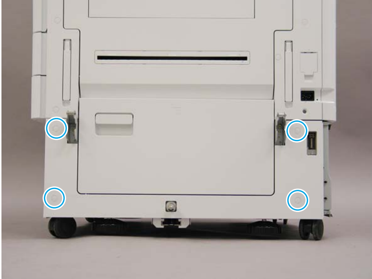
Figure 2-1072 Remove the lower right cover
