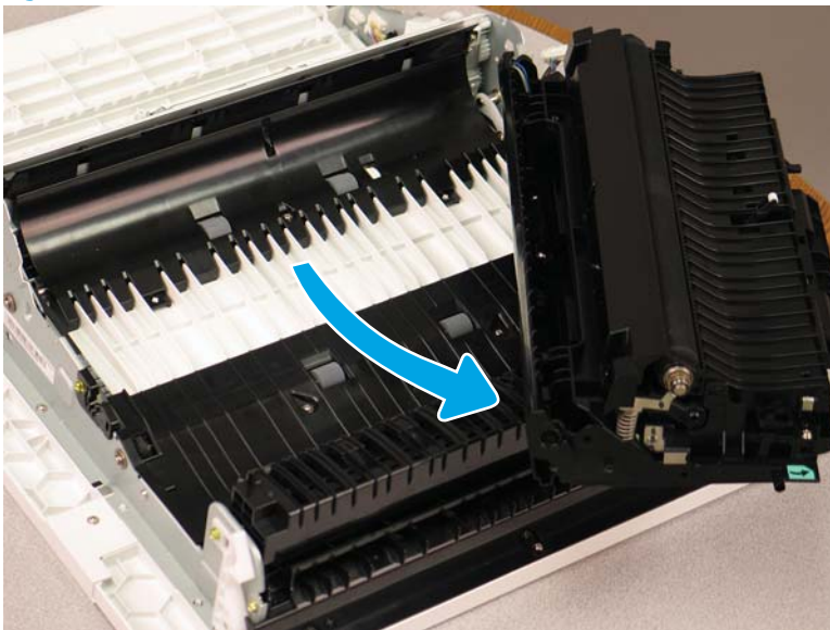
Figure 2-679 Rotate the feed roller assembly
