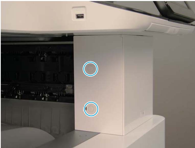
Figure 2-347 Remove the front top inner cover
