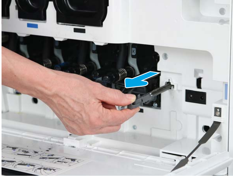
Figure 2-332 Remove the paper dust brush
