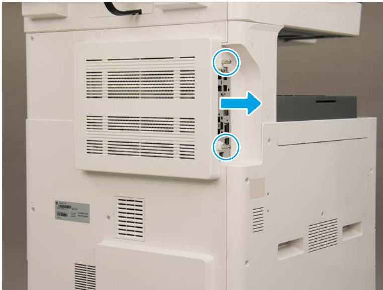
Figure 2-500 Remove the formatter cover
