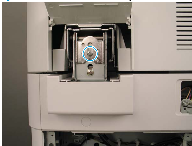
Figure 2-822 Release the document feeder hinge screws
