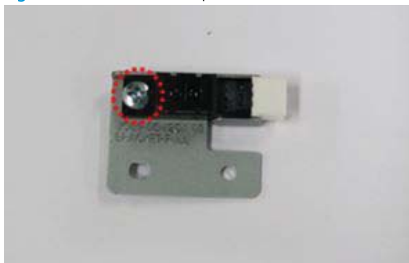
Figure 6-898 Remove the punch dust full sensor
