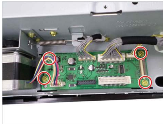
Figure 2-905 Remove screws and release scanner PCA
