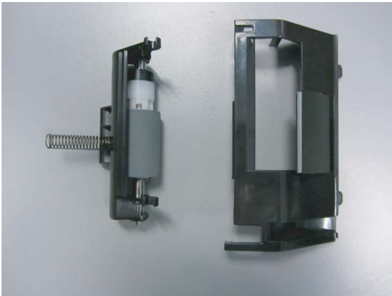
Figure 2-884 Document feeder separation roller cover and roller assembly
