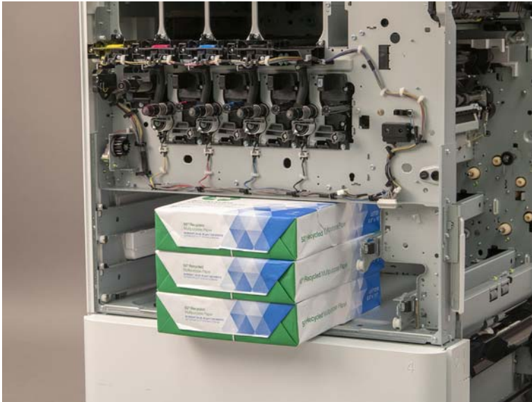
Figure 2-374 Support the chassis
