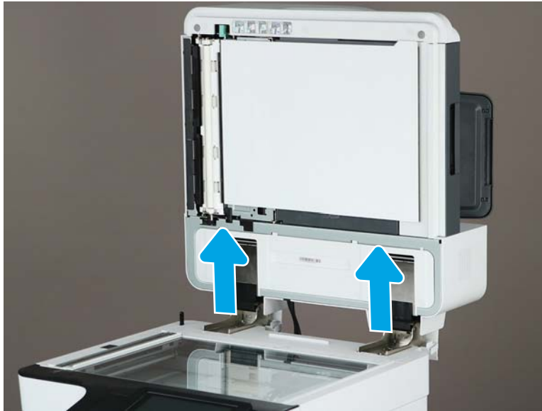
Figure 2-1059 Remove two screw and lift up to remove ADF
