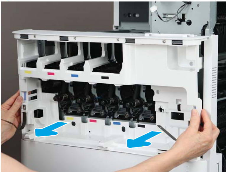
Figure 2-339 Remove the inner cover
