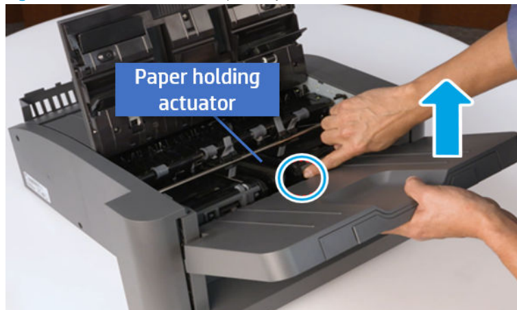
Figure 6-710 Remove the output tray
