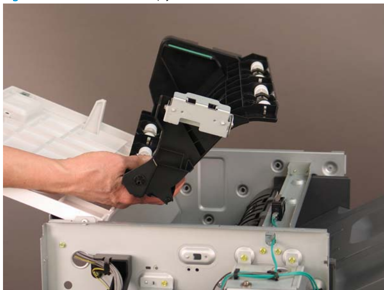
Figure 5-180 Remove the top jam access cover
