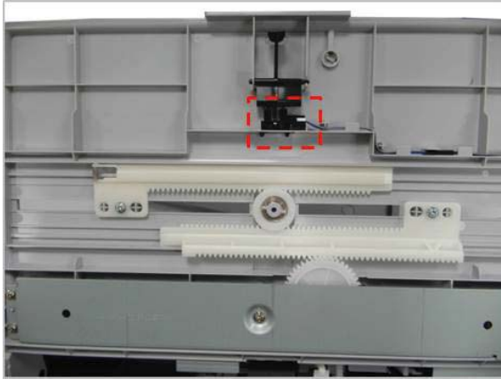
Figure 2-751 Remove the Tray 1 paper length sensor
