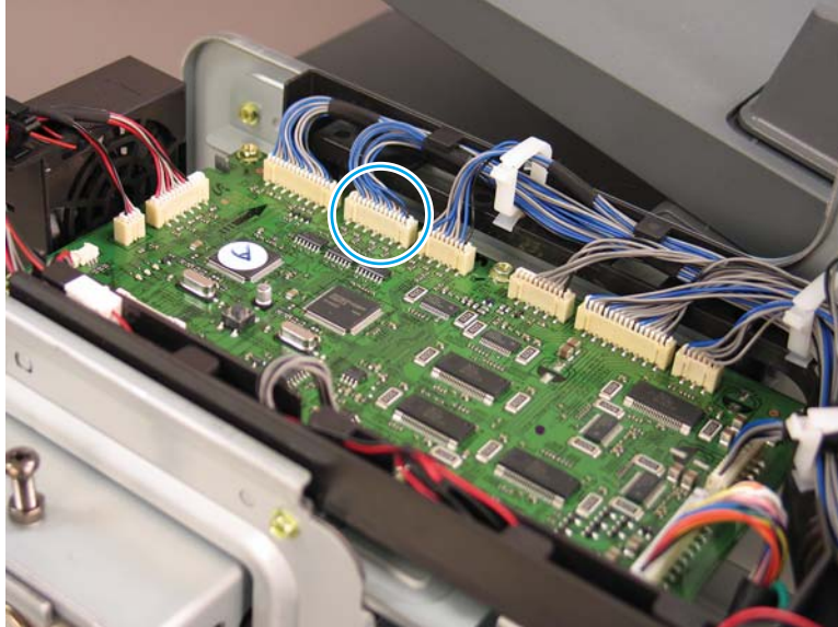
Figure 2-933 Disconnect one connector
