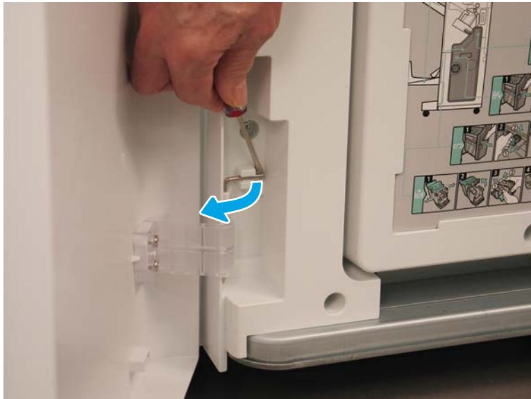
Figure 5-93 Release the lower hinge pin
