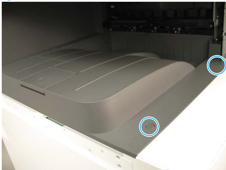
Figure 2-120 Remove the exit cover
