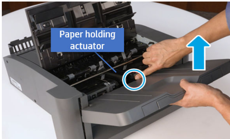
Figure 6-368 Remove the output tray
