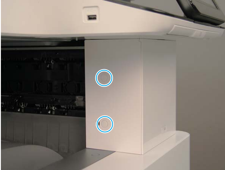
Figure 2-543 Remove the front top inner cover
