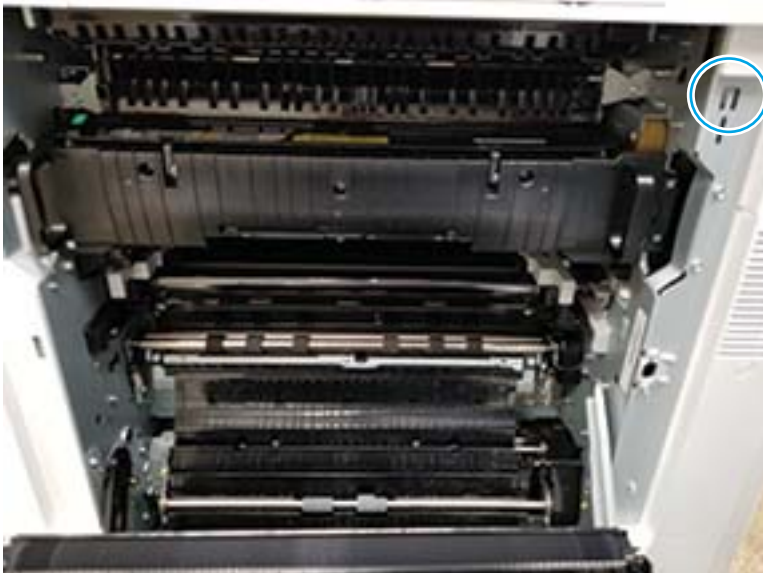
Figure 3-8 Defeat the toner cartridge door interlock
