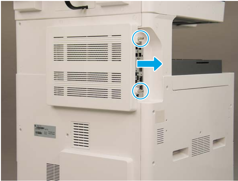
Figure 2-136 Remove the formatter cover
