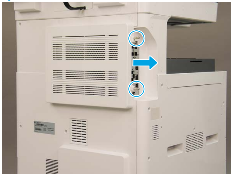
Figure 2-123 Remove the formatter cover
