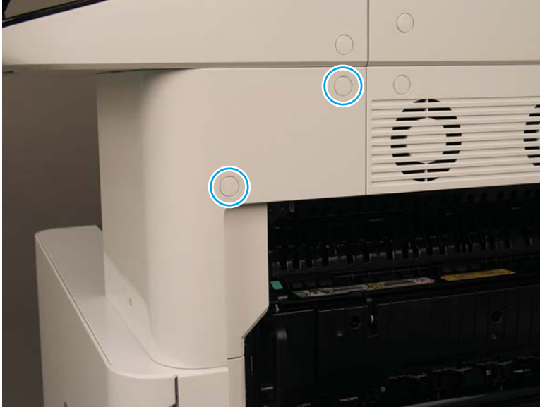
Figure 2-321 Remove two screws and rotate the cover
