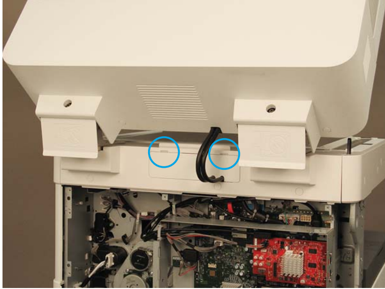
Figure 2-907 Remove document feeder connector cover
