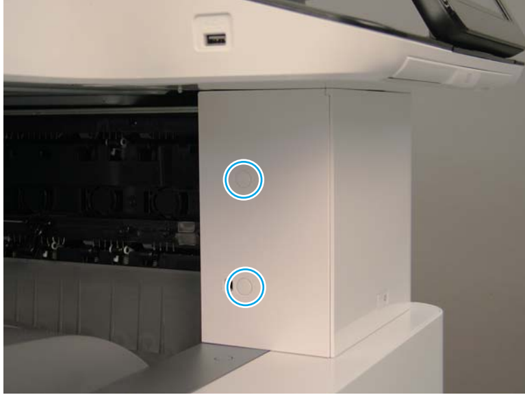
Figure 2-458 Remove the front top inner cover
