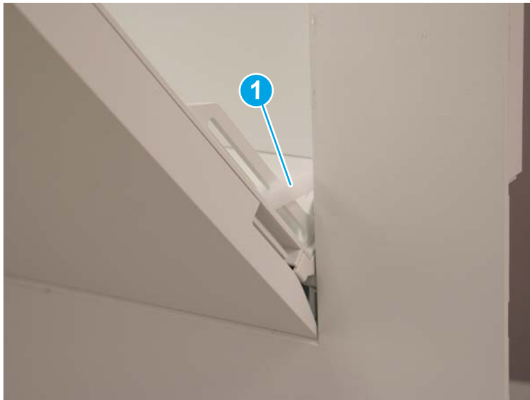
Figure 2-669 Release the hinge arm
