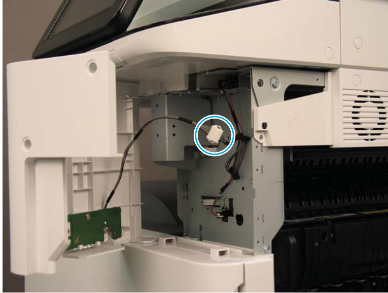
Figure 2-636 Remove the front power cover
