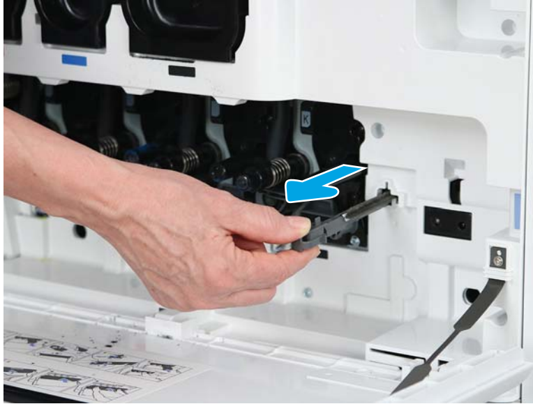
Figure 2-436 Remove the paper dust brush
