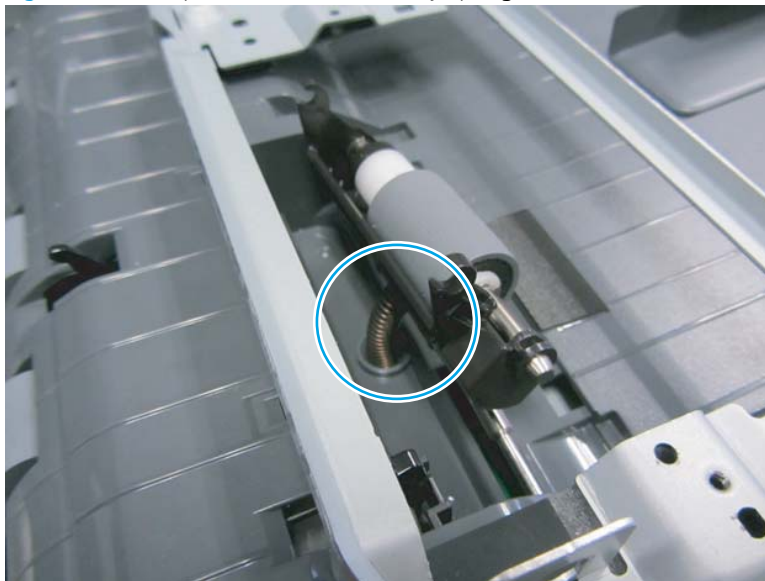
Figure 2-886 Separation roller assembly spring
