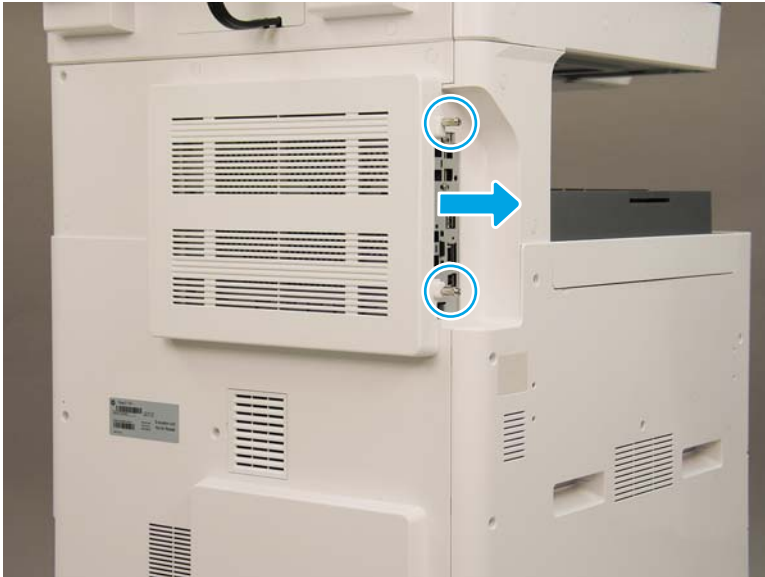
Figure 2-819 Remove the formatter cover and the upper rear cover
