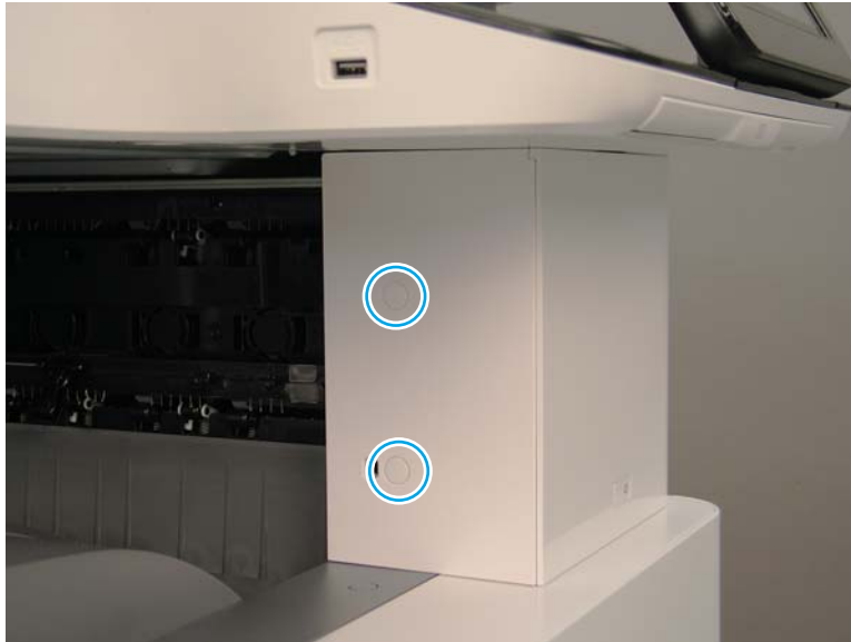
Figure 2-638 Remove the front top inner cover
