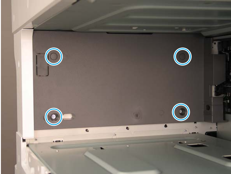
Figure 2-121 Remove the HDD cover
