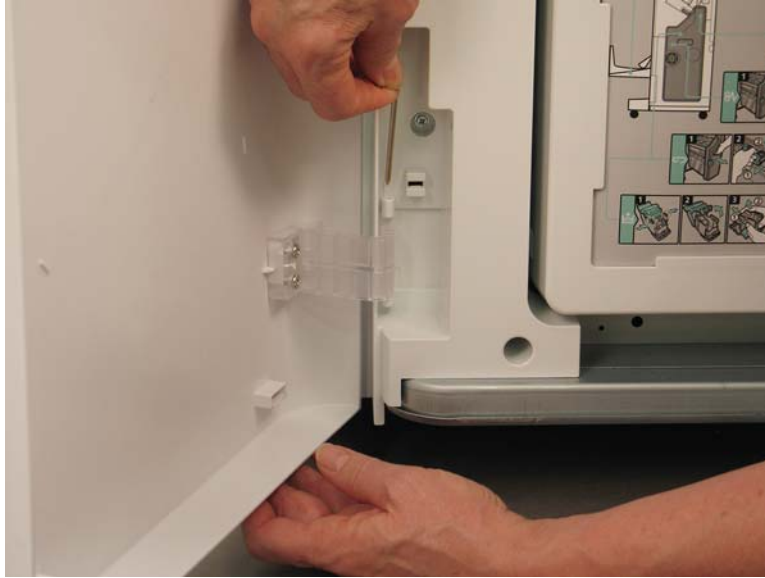
Figure 5-356 Remove the lower hinge pin
