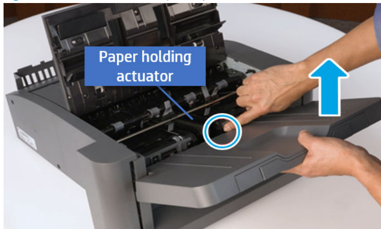
Figure 6-754 Remove the output tray
