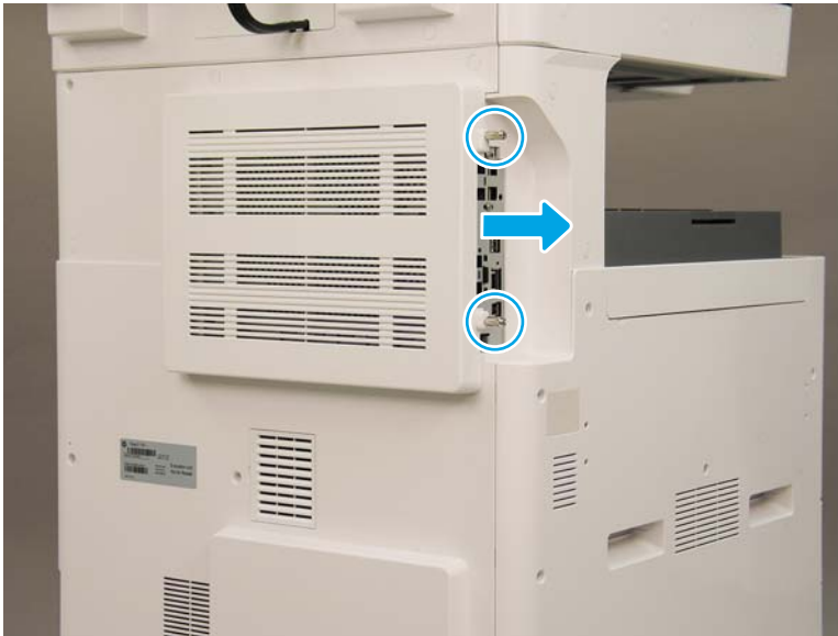
Figure 2-101 Remove the formatter cover
