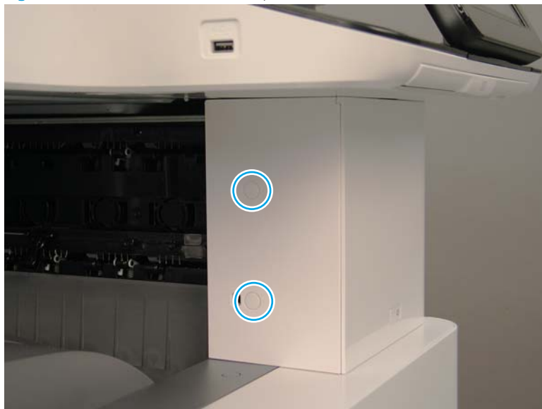
Figure 2-119 Remove the front top inner cover
