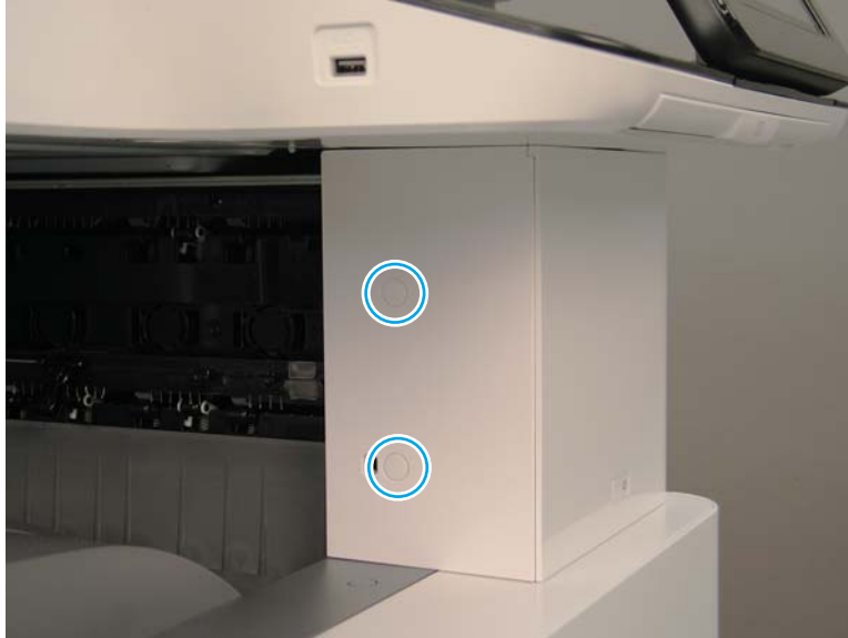
Figure 2-637 Remove the front top inner cover
