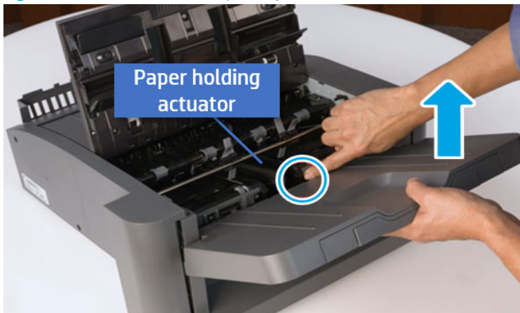
Figure 6-826 Remove the output tray
