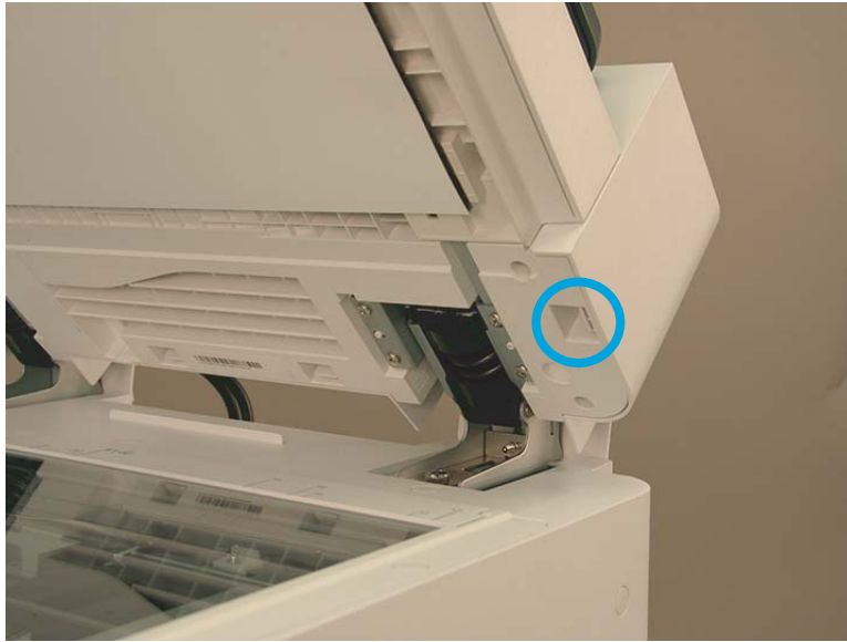
Figure 2-843 Release one tab on the right side of back cover.
