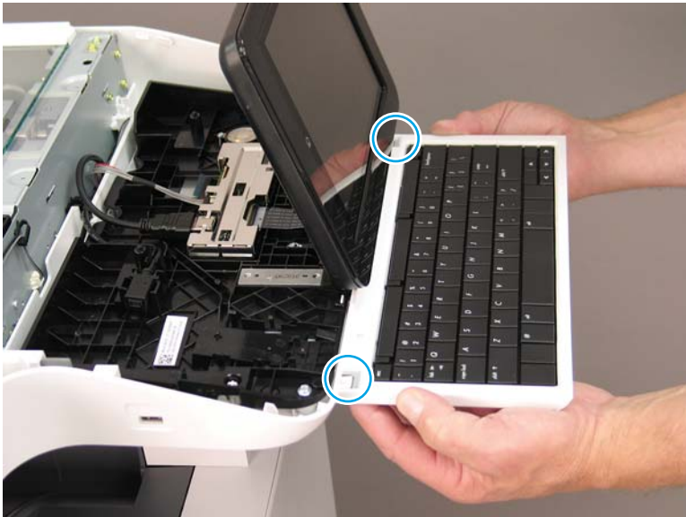
Figure 2-69 Remove the control-panel keyboard
