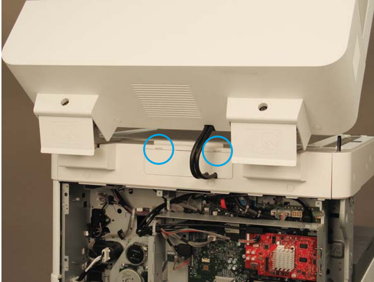
Figure 2-1053 Remove document feeder connector cover
