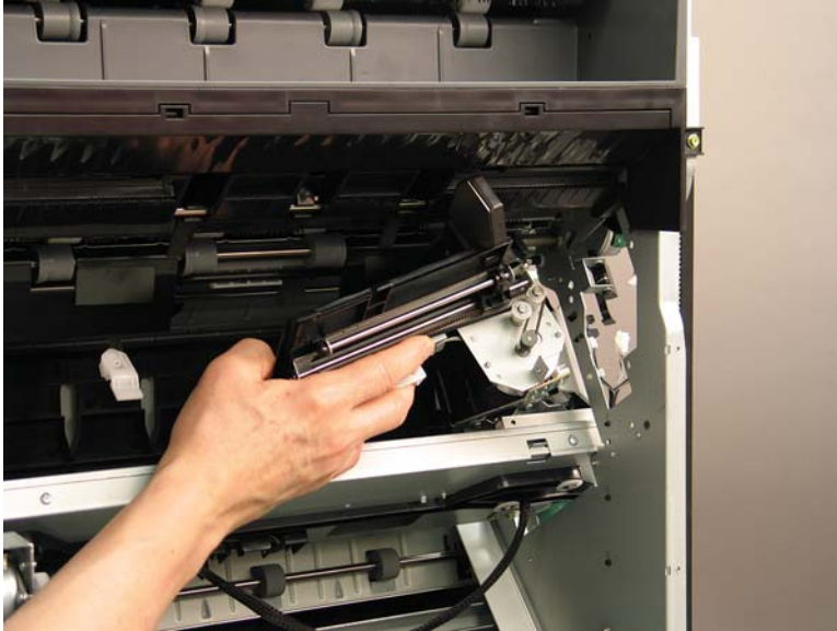
Figure 5-394 Remove the front tamper
