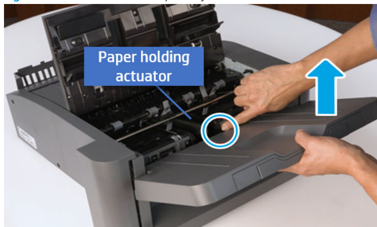
Figure 6-277 Remove the output tray
