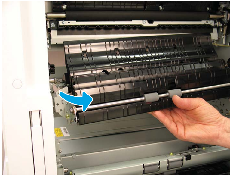
Figure 2-368 Rotate pickup unit 1
