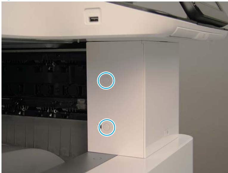
Figure 2-320 Remove the front top inner cover
