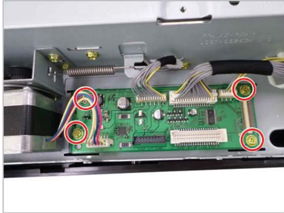
Figure 2-1032 Remove screws and release scanner PCA
