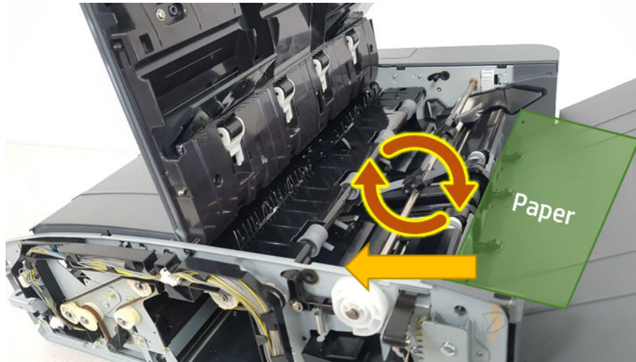
Figure 6-35 Inner finisher - paddle operation 1
