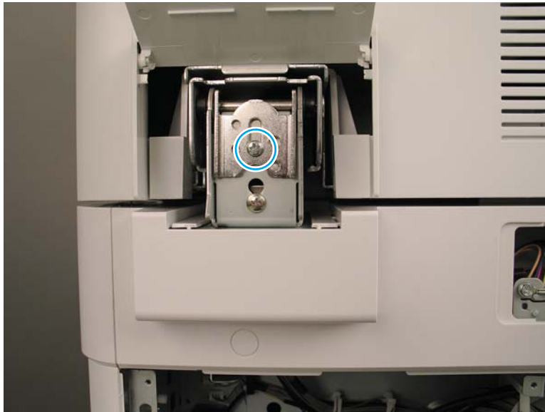
Figure 3-53 Adjust ADF hinge
