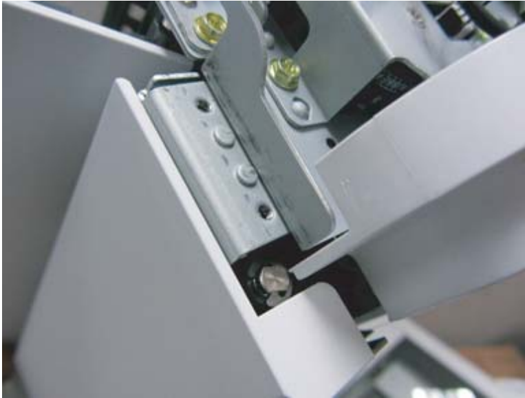
Figure 2-1018 Pry the scan in lower assembly away from the ADF
