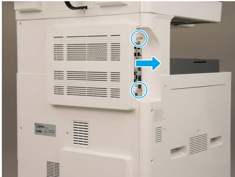
Figure 2-220 Remove the formatter cover
