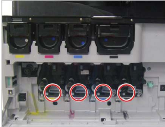
Figure 2-4 Laser scanner assembly color entrances
