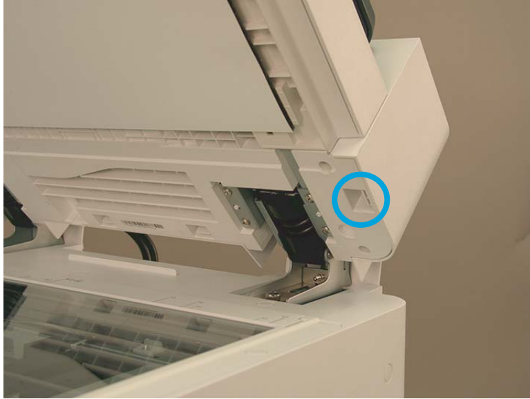
Figure 2-992 Release one tab on the right side of back cover.
