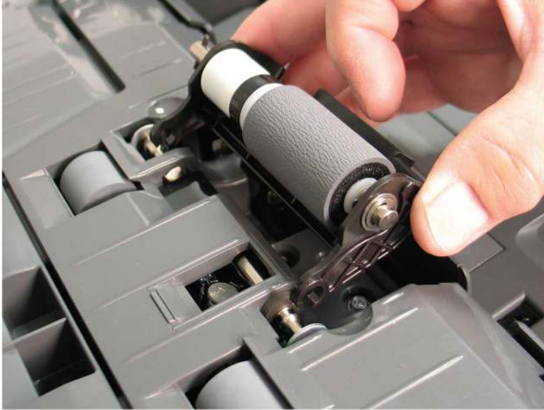
Figure 2-464 Release the separation roller
