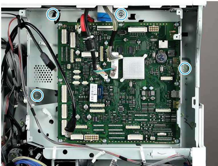
Figure 2-169 Remove the main board cage screws
