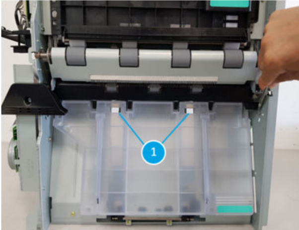
Figure 5-1618 Remove two screws at the left of the booklet maker
