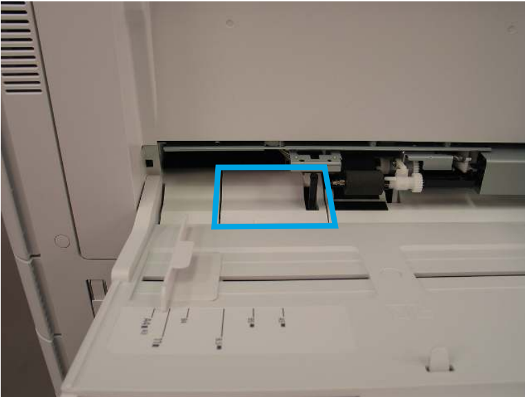
Figure 2-348 Remove MP-cover base
