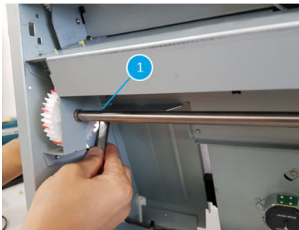
Figure 5-1490 Use a tweezer to remove the Booklet paddle home sensor
