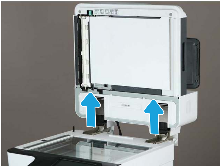
Figure 2-38 Release the document feeder
