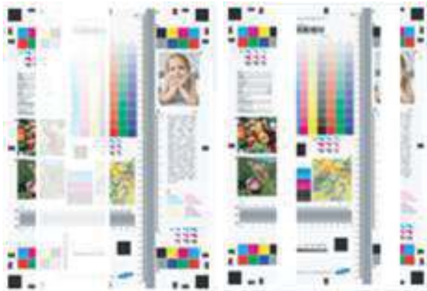
Figure 3-43 Typical faulty images
