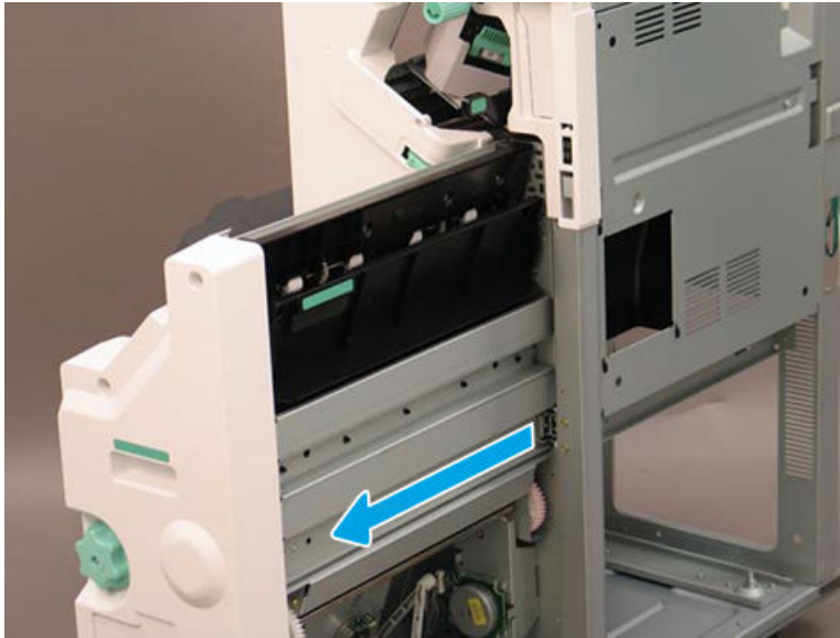
Figure 5-1680 Extend the right rail
