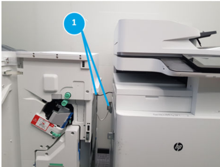
Figure 5-134 Separate the finisher from the printer and disconnect the two connectors
