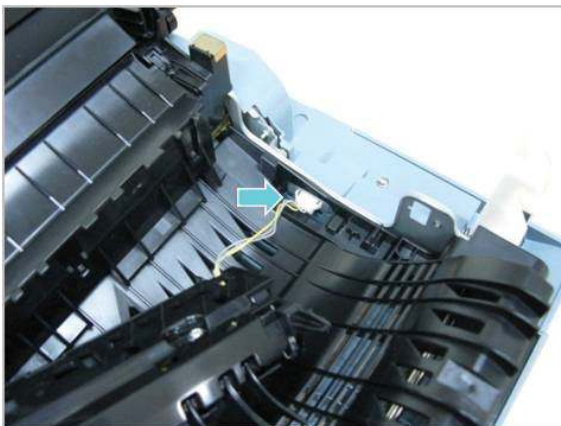
Figure 2-213 Remove right-door exit
