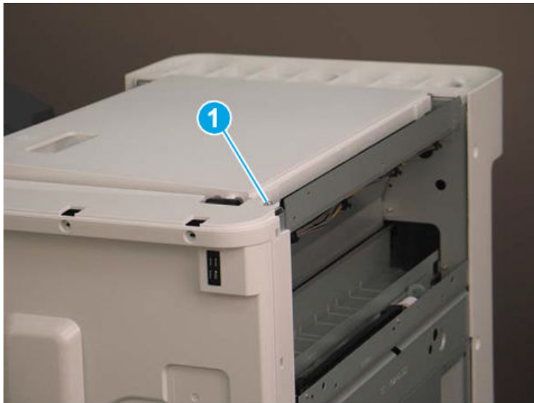
Figure 5-584 Remove one screw
