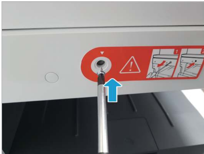
Figure 1-51 Tighten scan locking screw
