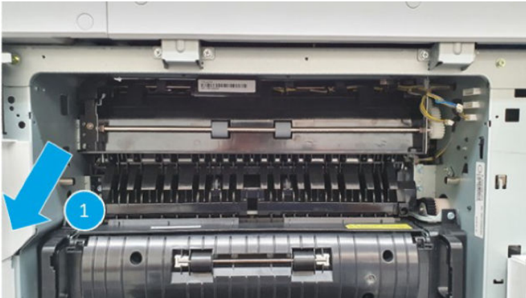
Figure 2-524 Remove the second exit unit
