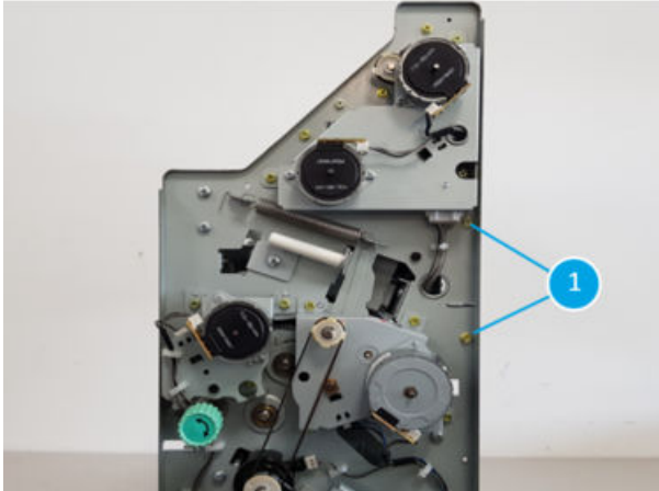
Figure 5-1613 Remove two screws at the front of the booklet maker
