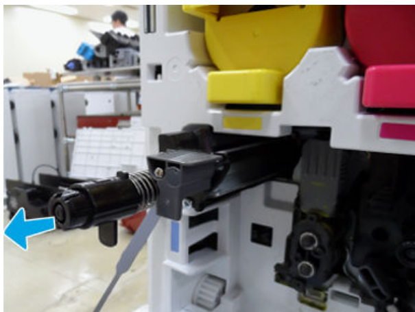
Figure 2-58 Release ITB cleaner
