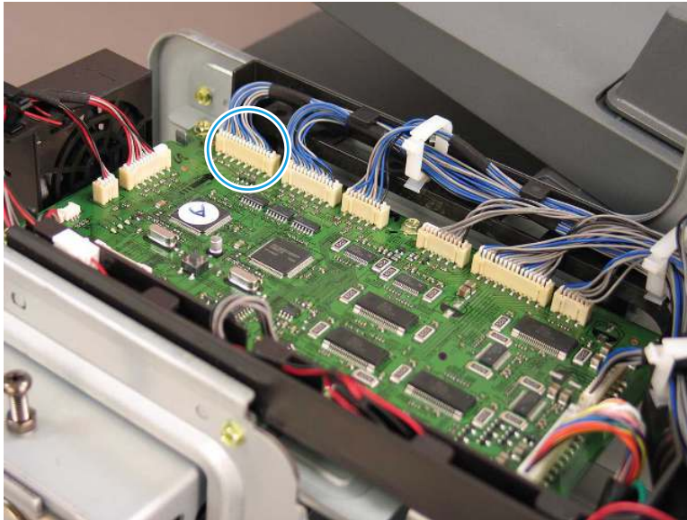
Figure 2-429 Disconnect the document feeder PCA connector
