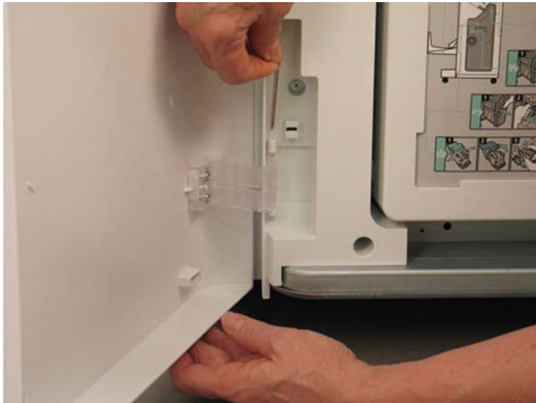
Figure 5-1247 Remove the lower hinge pin
