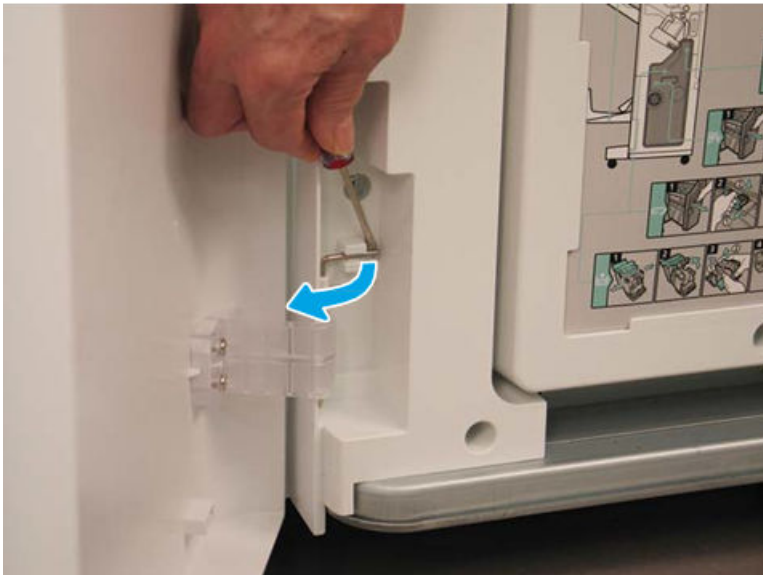
Figure 5-925 Release the lower hinge pin
