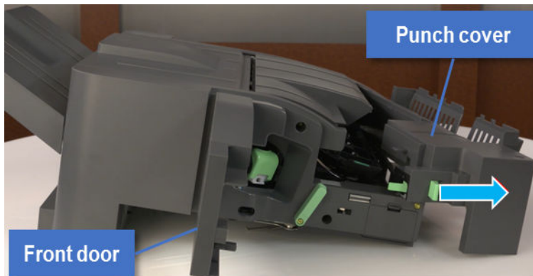
Figure 6-63 Open the front door and punch cover
