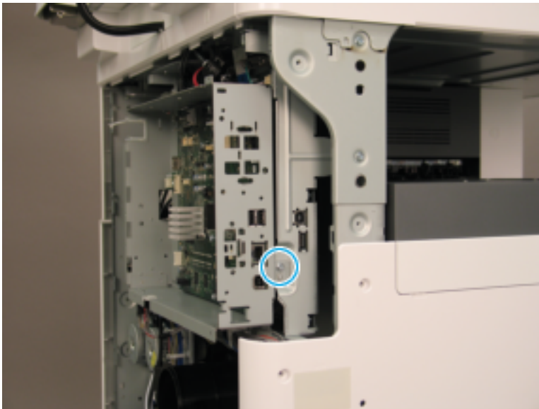
Figure 2-95 Remove the formatter cage side screw
