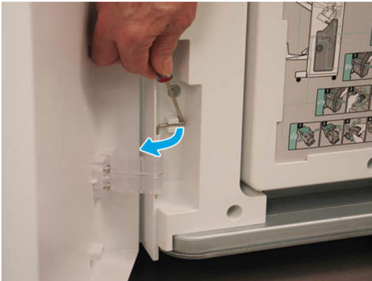
Figure 5-424 Release the lower hinge pin
