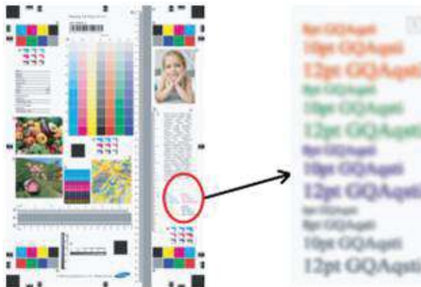
Figure 3-48 Typical faulty images
