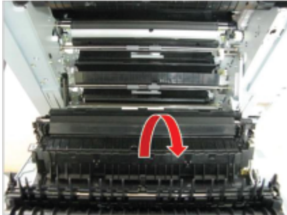
Figure 2-209 Remove right door
