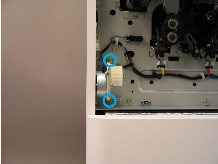
Figure 2-161 Remove screws and toner collection unit drive unit
