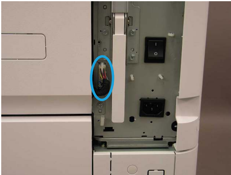
Figure 2-226 Disconnect right door connector
