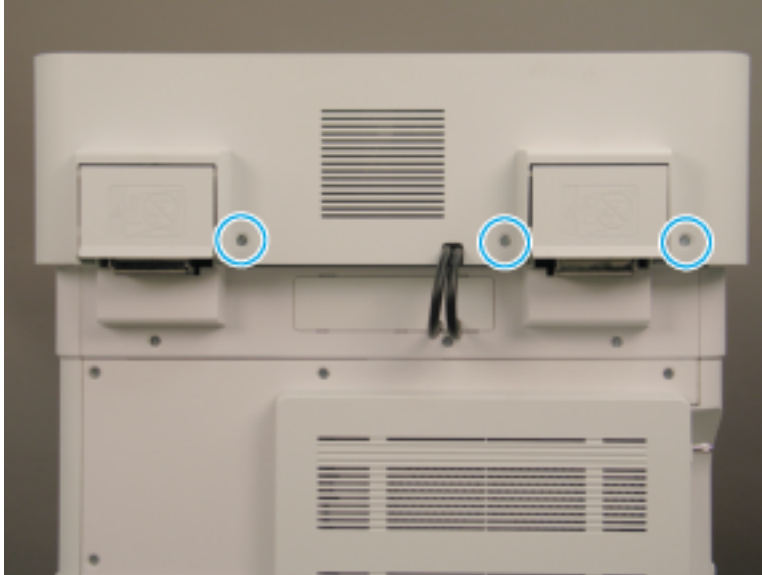
Figure 2-425 Remove the document feeder back cover bottom screws
