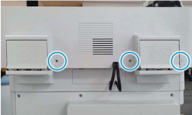
Figure 2-395 Remove 3 caps and 3 screws.
