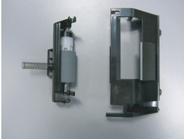
Figure 2-412 Document feeder separation roller cover and roller assembly
