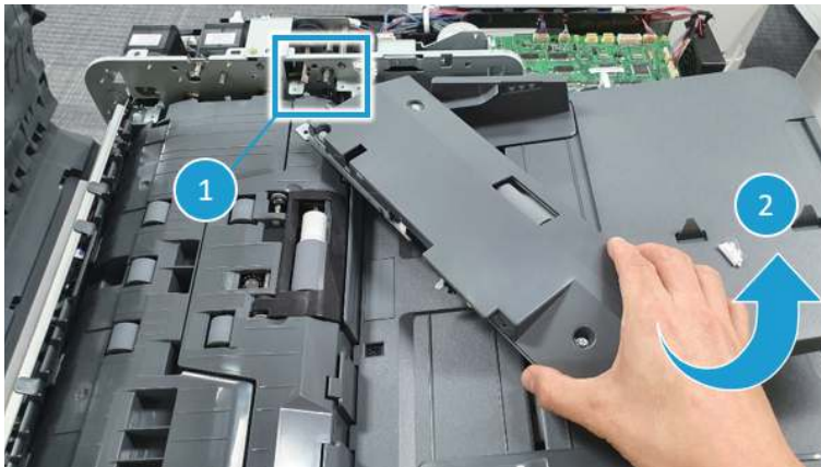
Figure 2-457 Remove the pickup roller assembly
