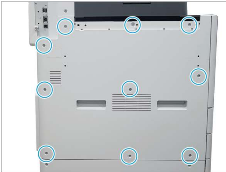
Figure 2-259 Remove the left cover
