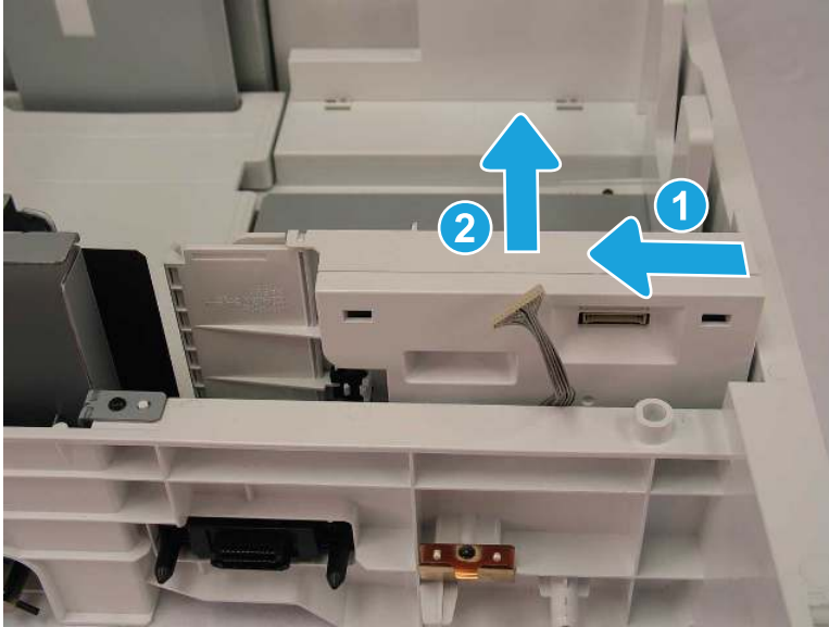
Figure 2-641 Release the sub-paper side right assembly
