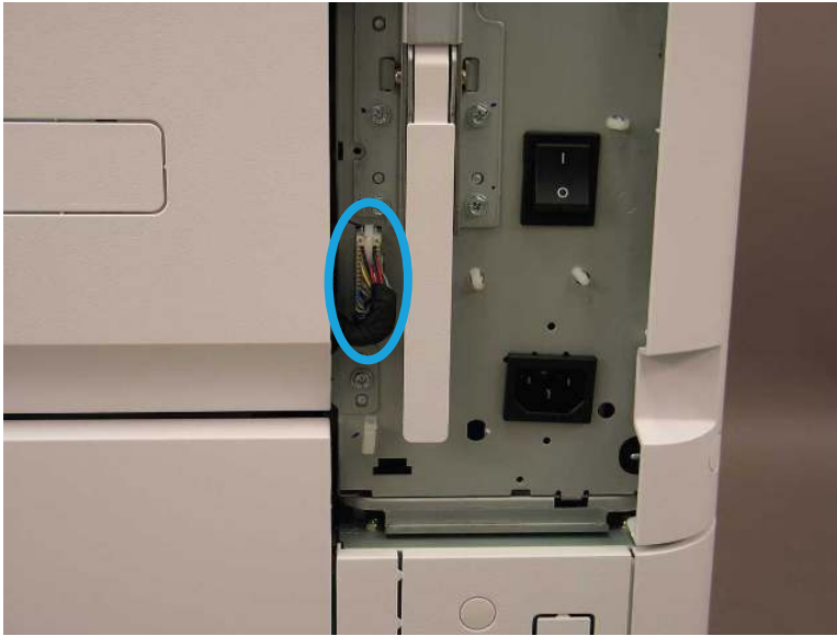
Figure 2-53 Disconnect right door connector
