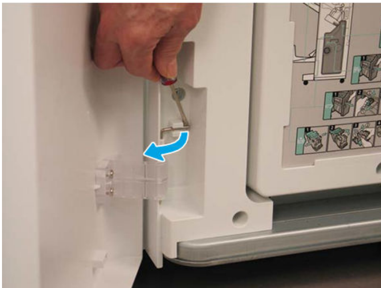
Figure 5-365 Release the lower hinge pin
