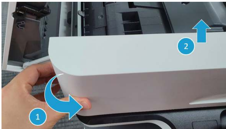
Figure 2-490 Remove the document feeder front cover
