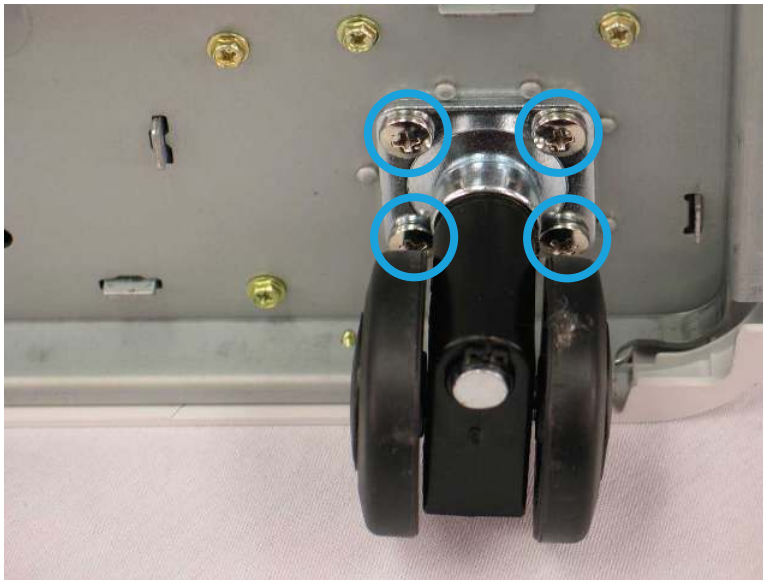
Figure 2-596 Remove the HCI caster wheel
