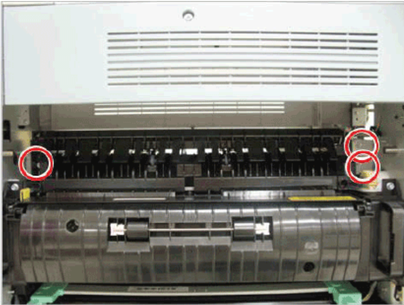
Figure 2-50 Remove screws and exit unit
