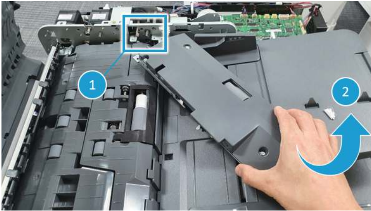
Figure 2-451 Remove the pickup roller assembly
