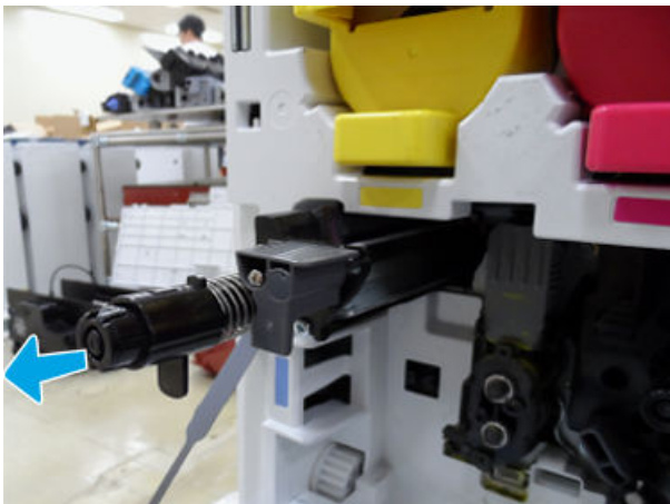
Figure 2-277 Release ITB cleaner
