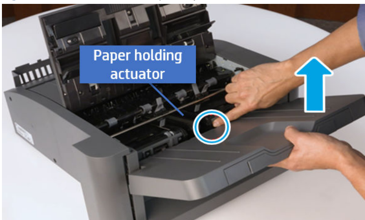
Figure 6-136 Remove the output tray.
