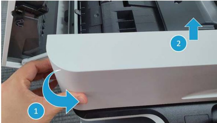
Figure 2-372 Remove the document feeder front cover
