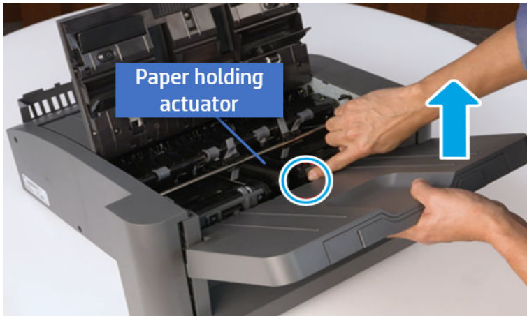
Figure 6-324 Remove the output tray.
