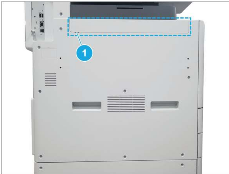
Figure 2-271 Remove the left trim cover
