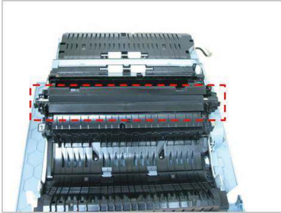
Figure 2-216 Remove transfer roller assembly
