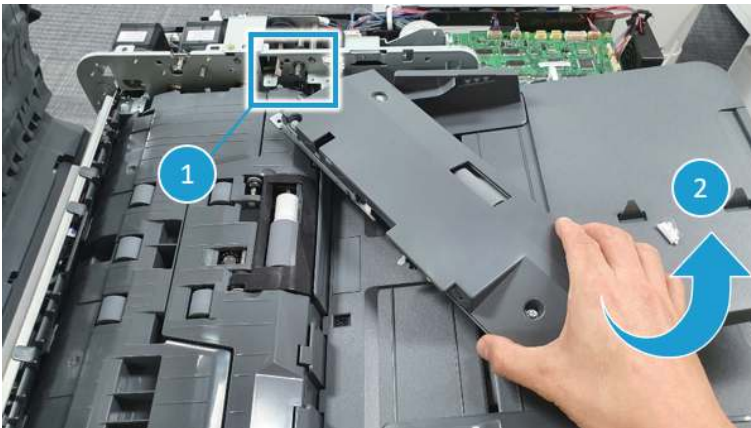
Figure 2-494 Remove the pickup roller assembly
