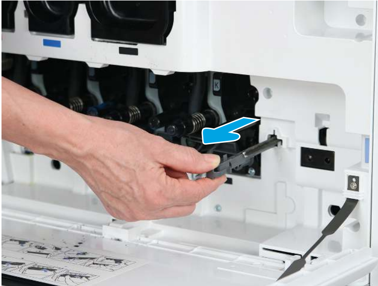
Figure 2-296 Remove the paper dust brush
