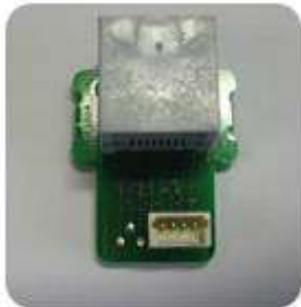
Figure 1-89 Toner CRUM joint PCA
