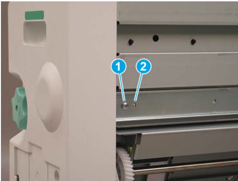
Figure 5-1925 Remove one screw
