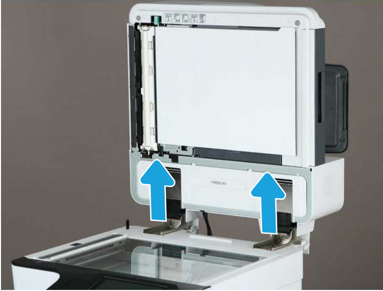
Figure 2-32 Release the document feeder
