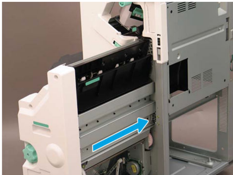
Figure 5-1637 Slide the right rail
