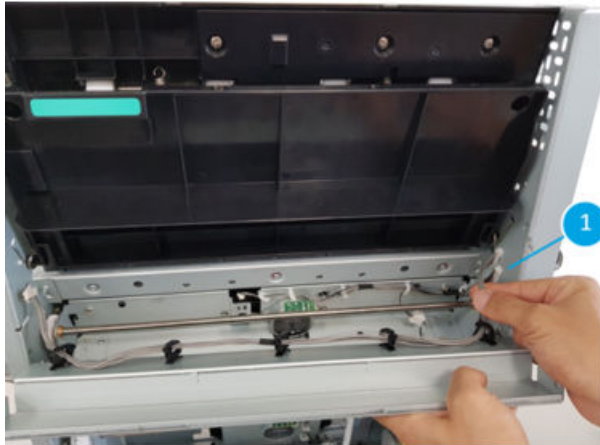
Figure 5-1654 Disconnect one connector
