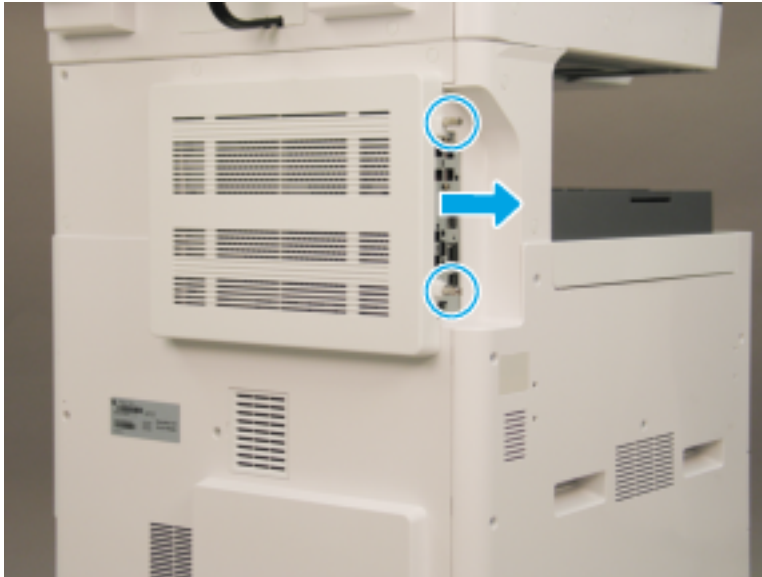
Figure 2-83 Remove the formatter cover
