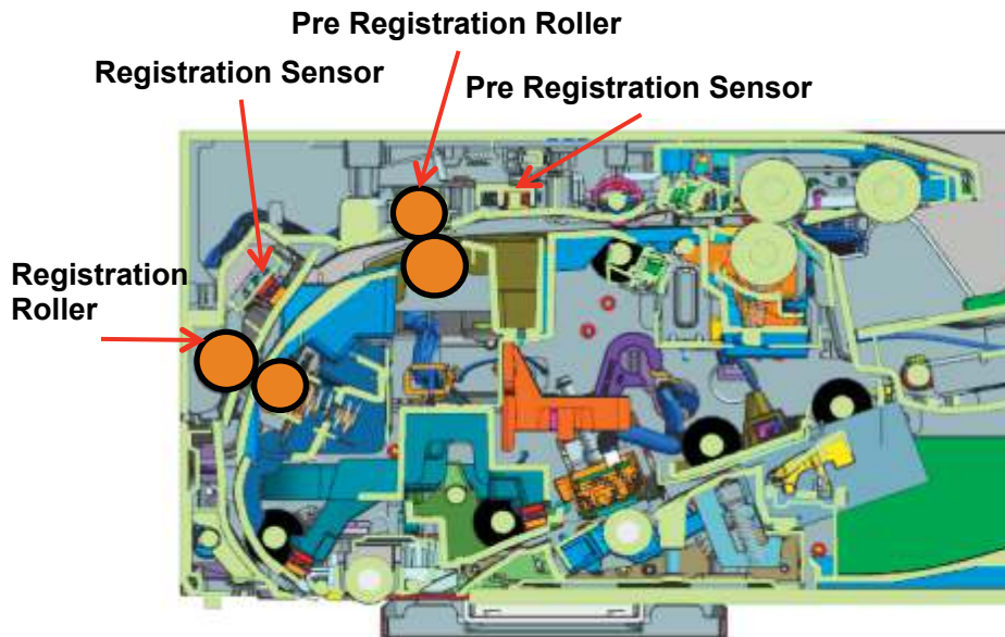
Figure 1-65 Flow document feeder registration
