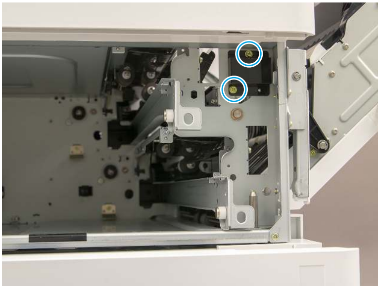
Figure 2-268 Remove the dampener cover
