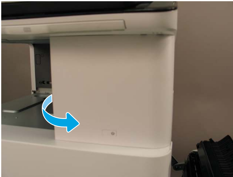
Figure 2-302 Remove the front top cover
