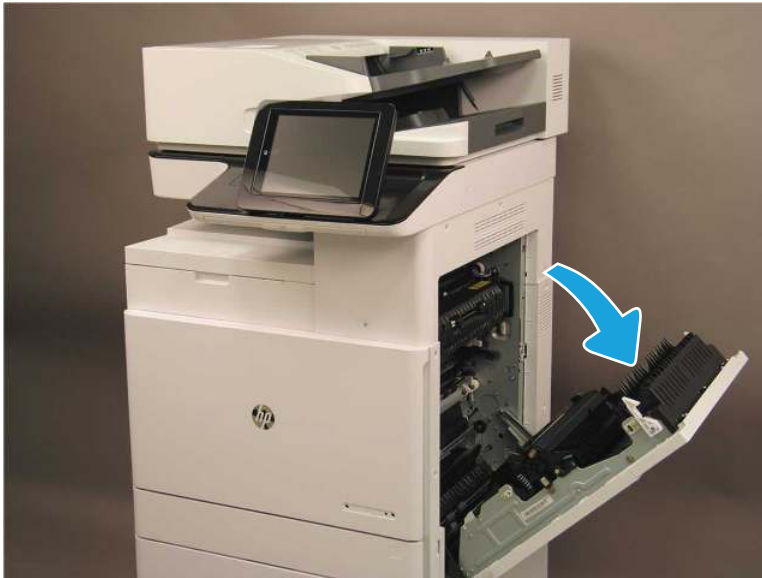
Figure 2-11 Open the right door
