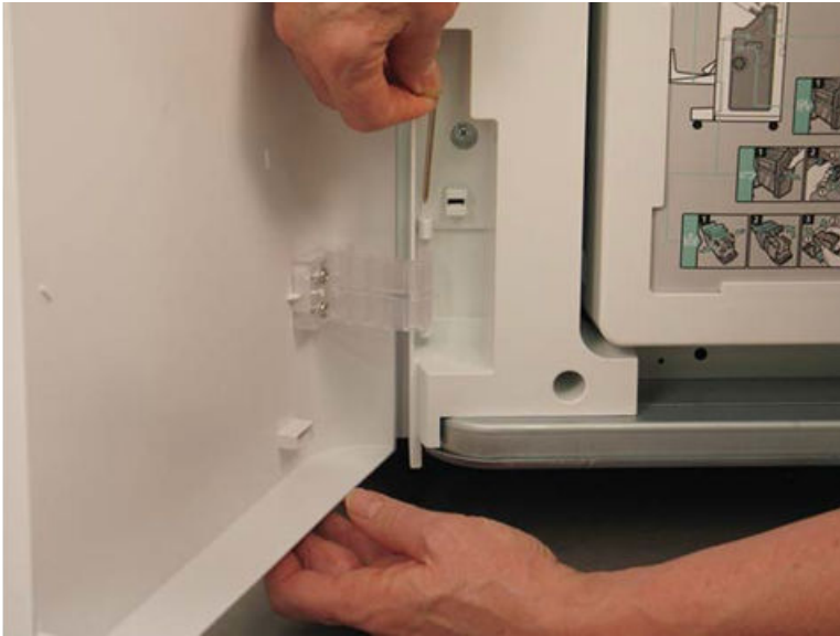
Figure 5-319 Remove the lower hinge pin
