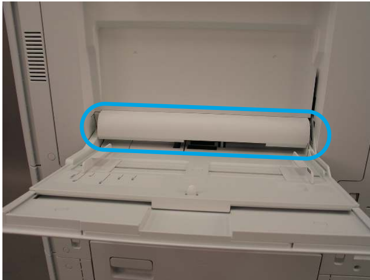
Figure 2-326 Remove the cover
