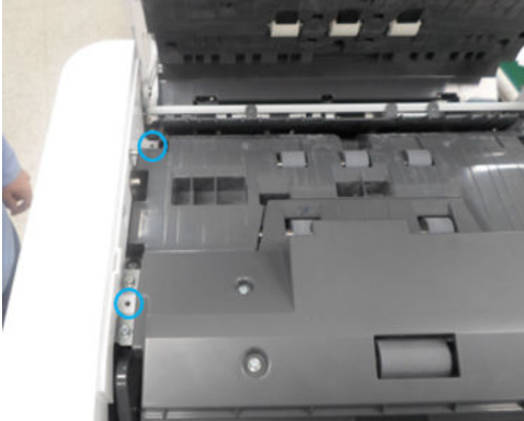
Figure 2-488 Remove the document feeder front cover top screws
