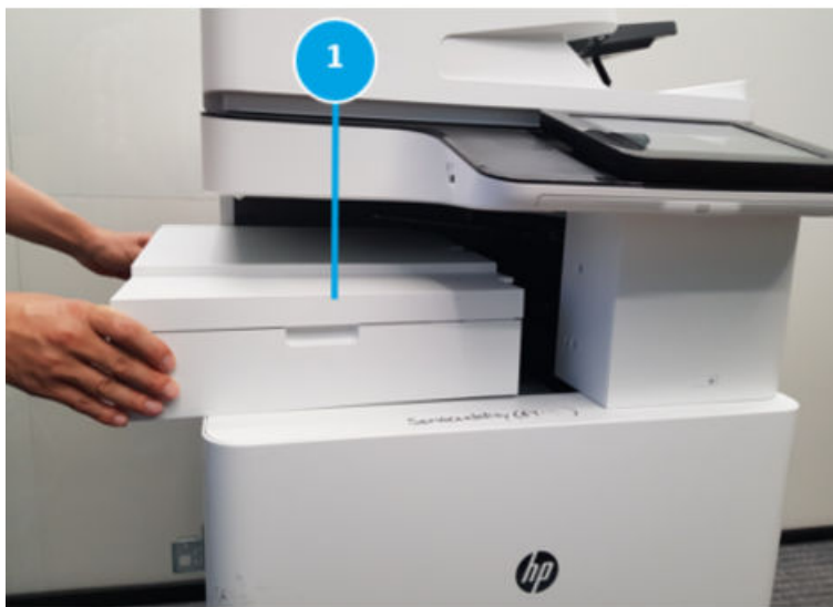
Figure 5-135 Pull out the bridge unit
