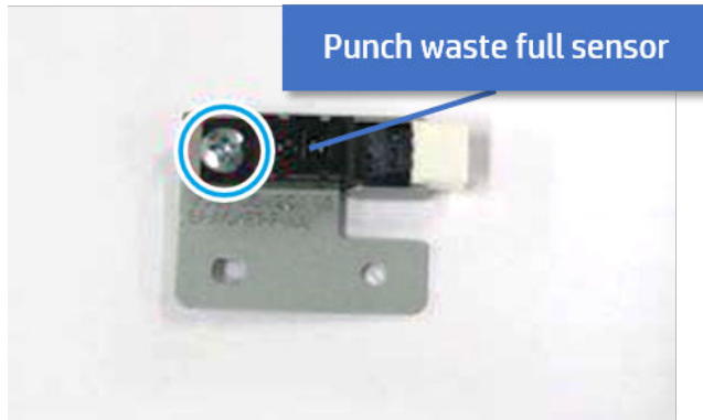
Figure 6-788 Remove the punch waste full sensor
