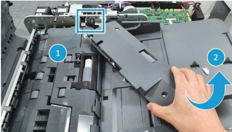
Figure 2-436 Remove the pickup roller assembly
