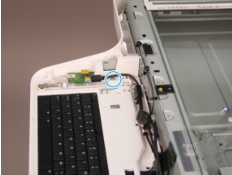
Figure 2-41 Remove USB interconnect cable
