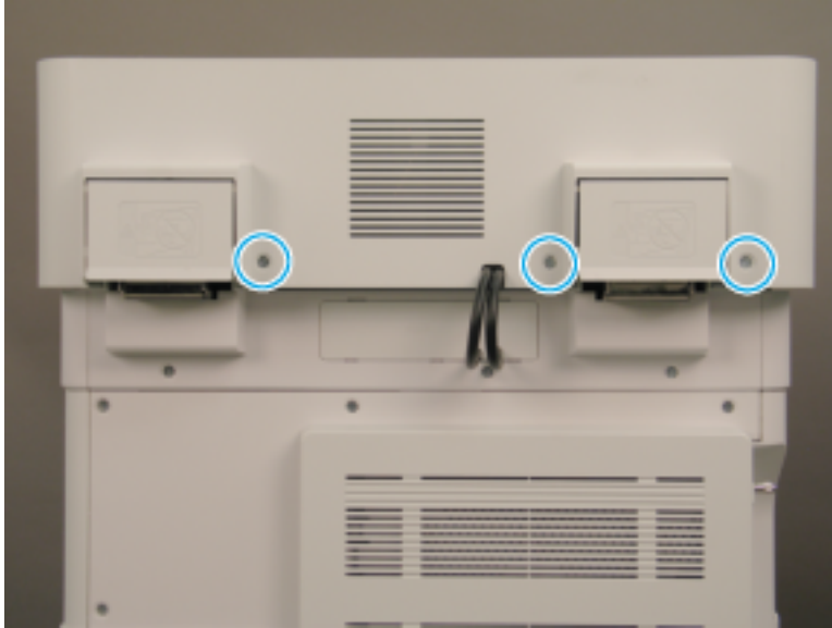
Figure 2-483 Remove the document feeder back cover bottom screws
