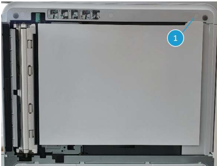
Figure 2-442 Open the document feeder
