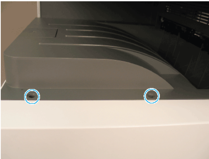
Figure 2-128 Remove screw-caps and screws
