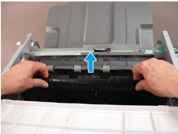
Figure 5-332 Remove the top lower feed assembly
