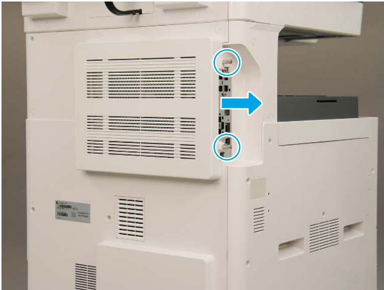
Figure 2-25 Remove the formatter cover
