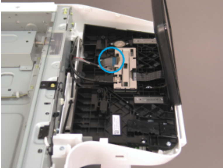
Figure 2-136 Disconnect one FFC
