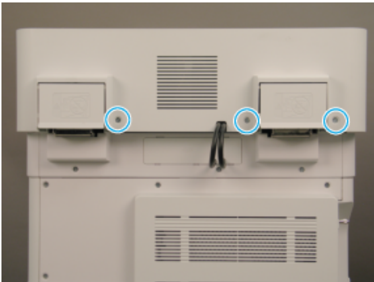
Figure 2-492 Remove the document feeder back cover bottom screws
