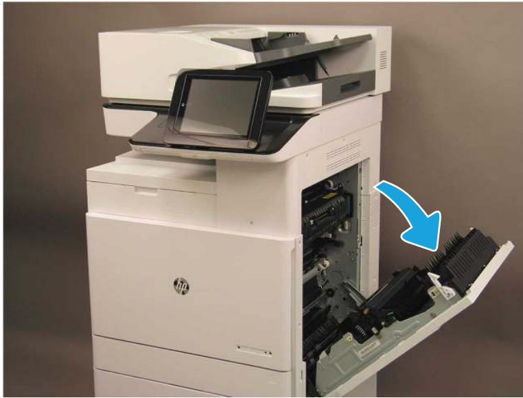
Figure 2-13 Open the right door
