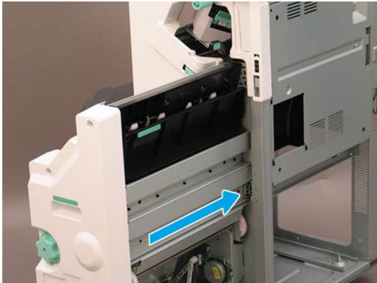
Figure 5-1437 Slide the right rail
