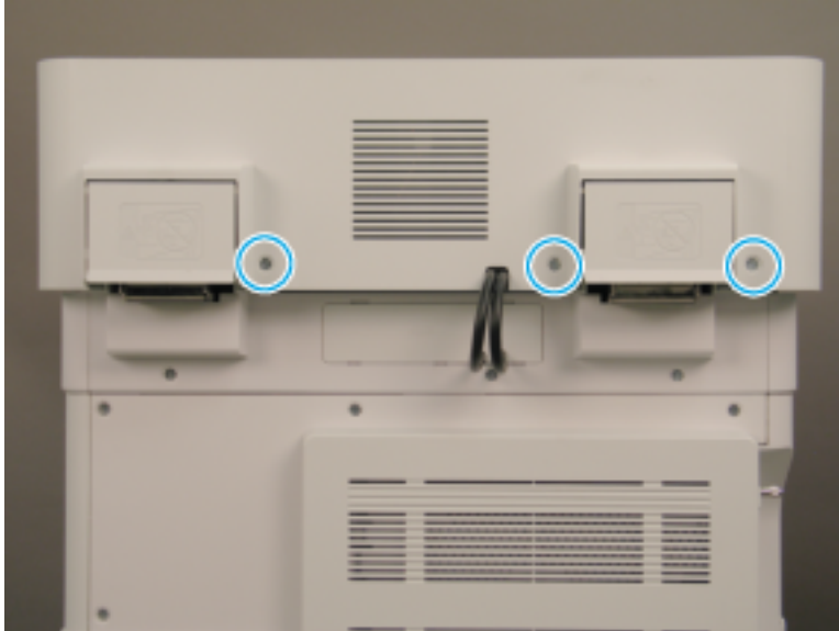
Figure 2-445 Remove the document feeder back cover bottom screws
