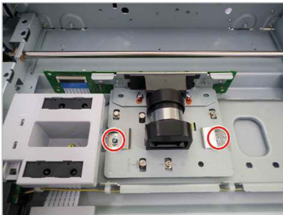
Figure 2-513 Remove screws and release scanner imaging unit
