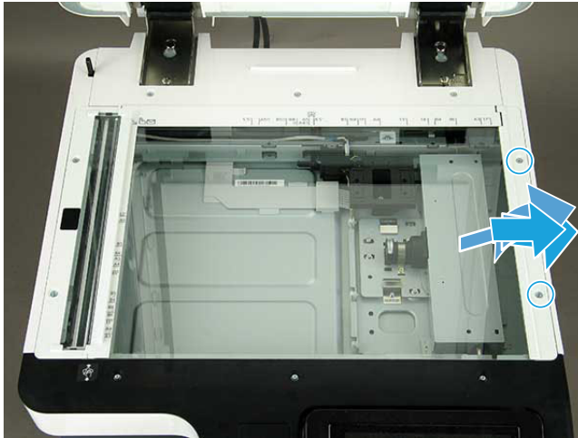
Figure 2-504 Remove scanner glass
