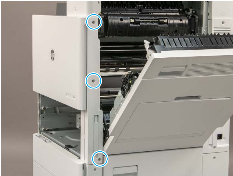
Figure 2-266 Remove the right front cover
