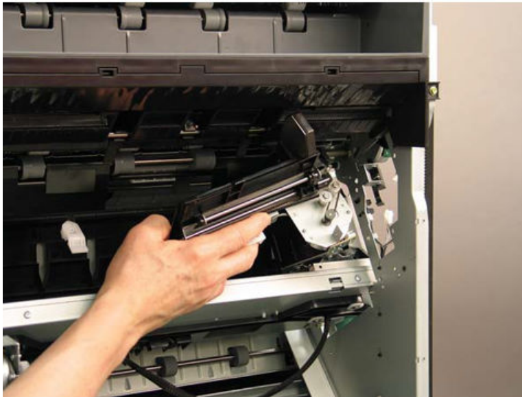
Figure 5-514 Remove the front tamper
