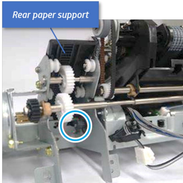
Figure 6-235 Remove the rear paper support
