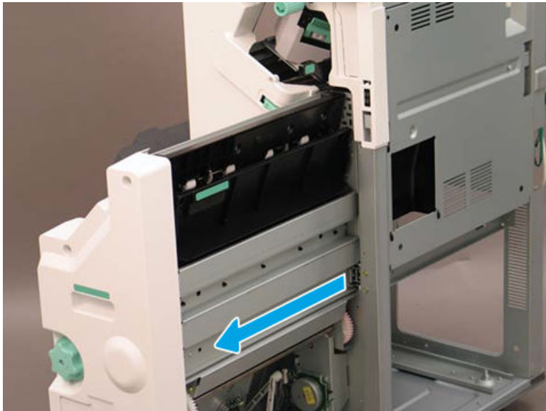
Figure 5-1443 Extend the right rail
