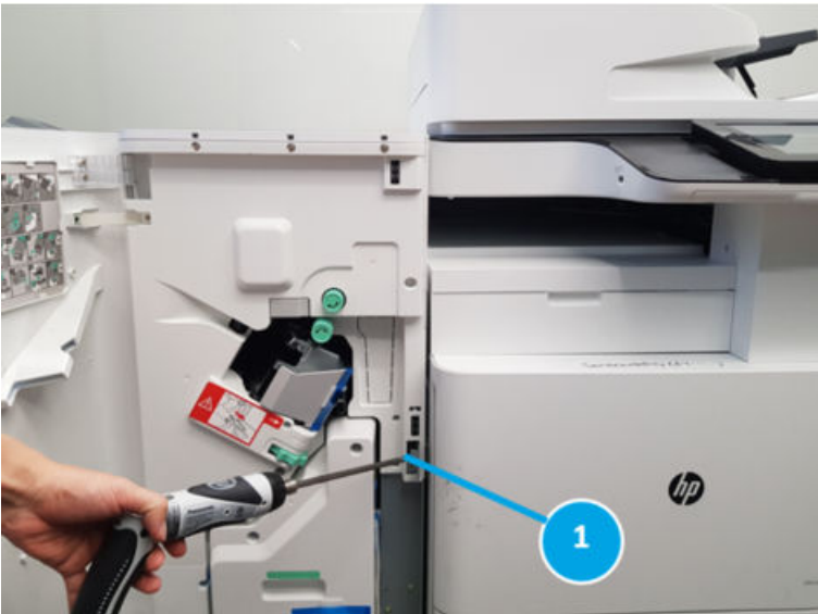
Figure 5-142 Pull the locker out
