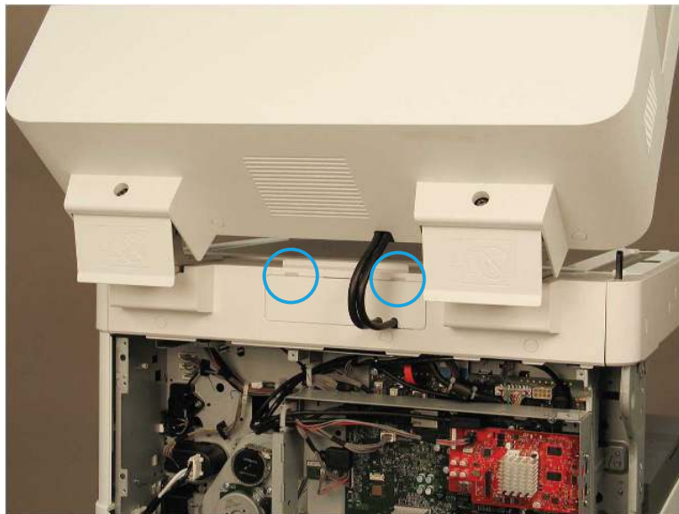
Figure 2-27 Remove document feeder connector cover
