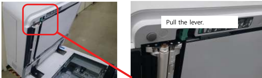
Figure 1-69 Flow document feeder dual sensor cleaning method (1 of 2)
