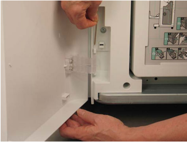
Figure 5-811 Remove the lower hinge pin
