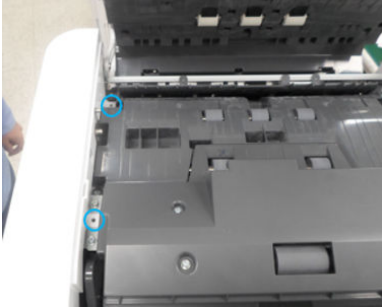
Figure 2-441 Remove the document feeder front cover top screws
