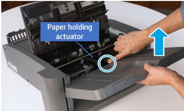
Figure 6-666 Remove the output tray.
