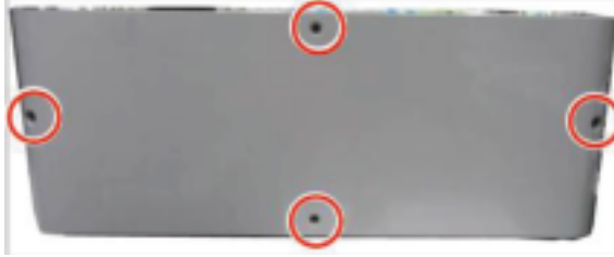
Figure 2-537 Remove the DCF rear cover
