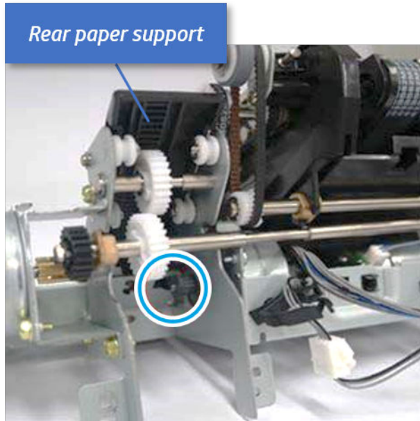
Figure 6-200 Remove the rear paper support
