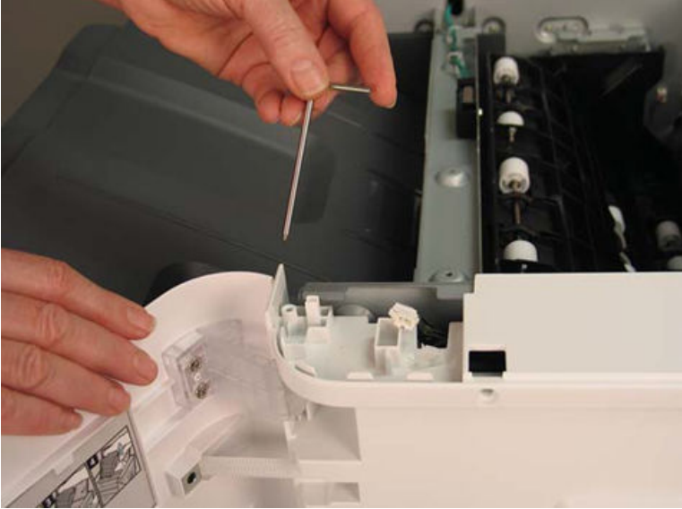
Figure 5-1034 Remove the top hinge pin
