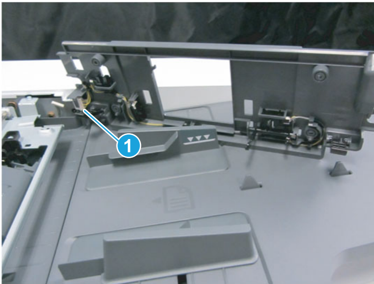
Figure 2-407 Turn the cover over and disconnect connector
