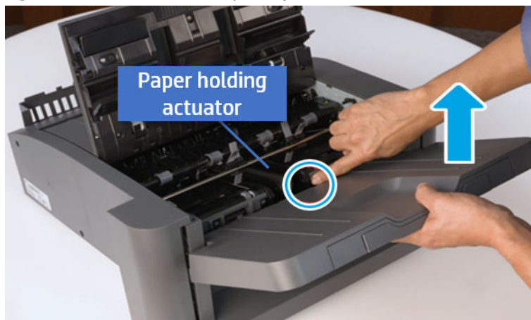
Figure 6-435 Remove the output tray.
