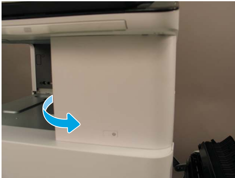
Figure 2-122 Remove the front top cover
