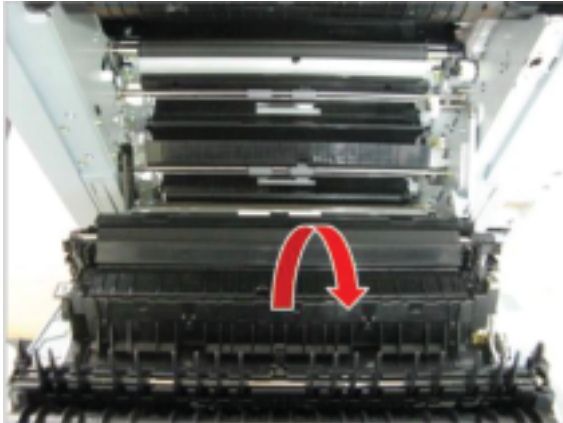
Figure 2-237 Remove right door
