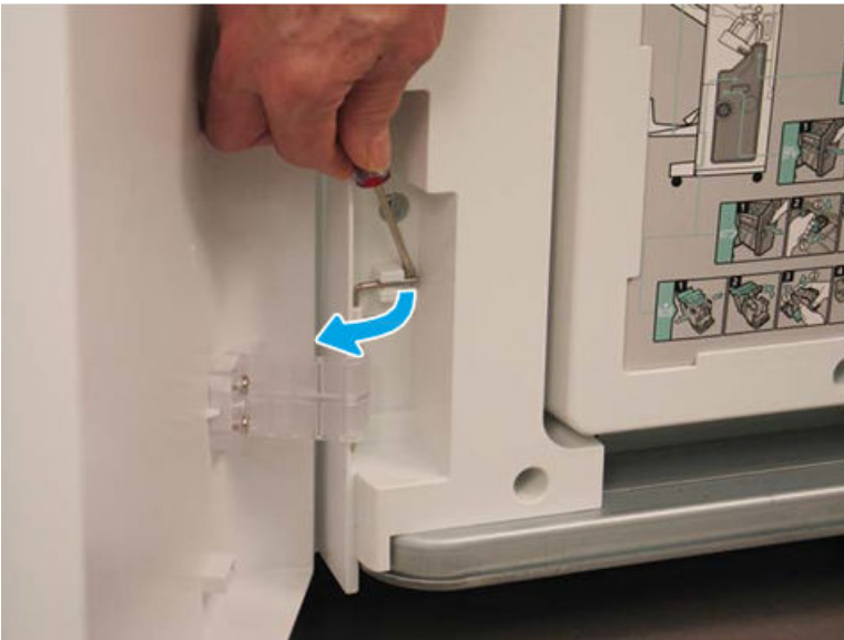
Figure 5-1035 Release the lower hinge pin
