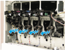
Figure 2-308 Release the toner supply pipes
