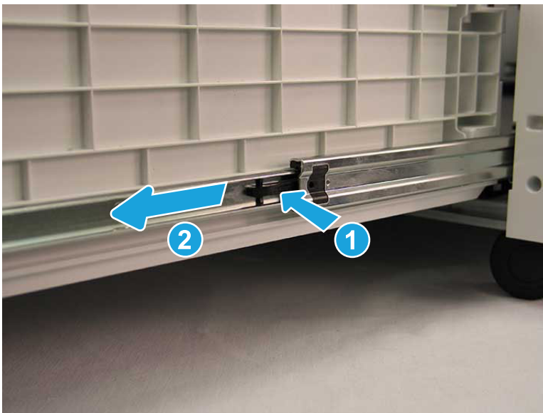
Figure 2-638 Release the tray right-side slide lock
