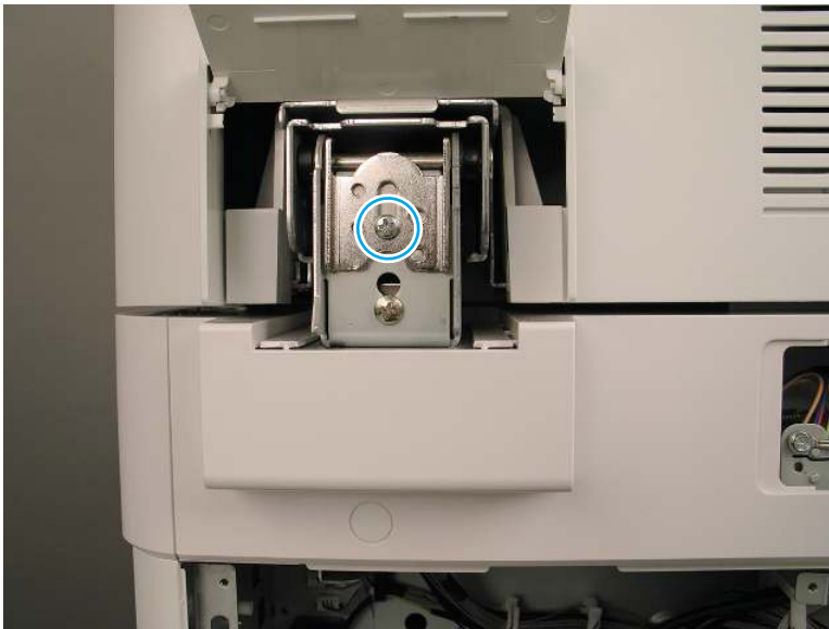
Figure 3-58 Adjust ADF hinge
