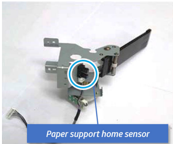
Figure 6-236 Remove the paper support home sensor
