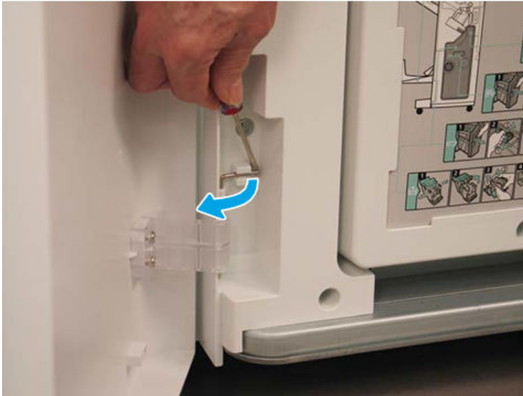
Figure 5-912 Release the lower hinge pin
