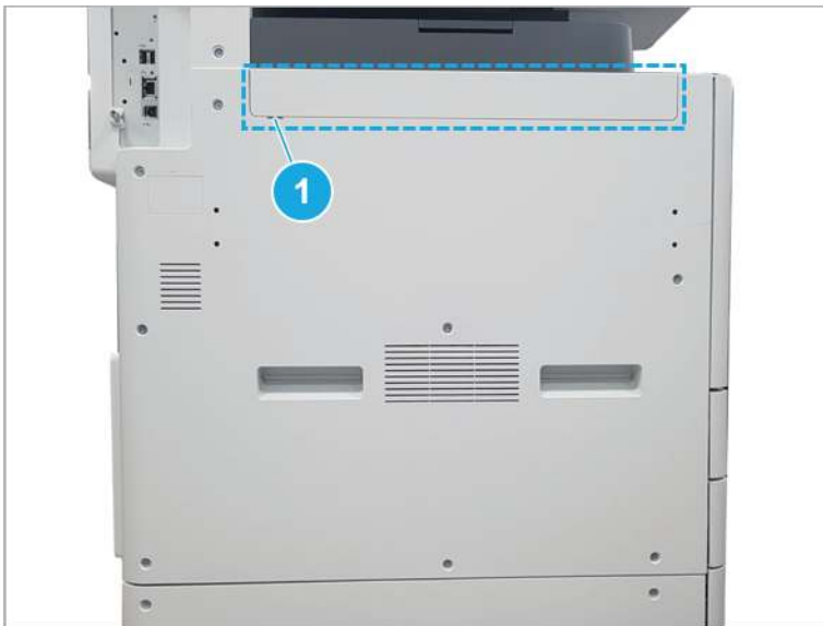
Figure 2-254 Remove the left trim cover
