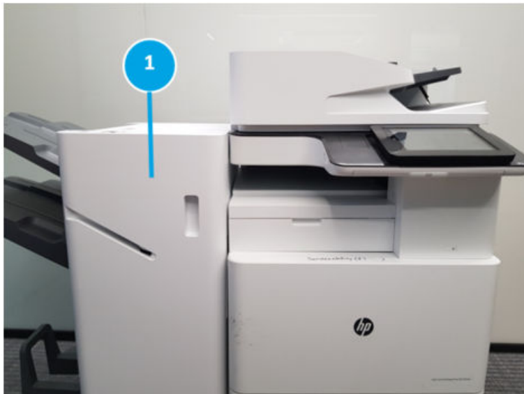
Figure 5-122 Open the front door
