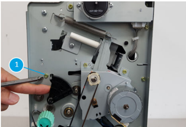
Figure 5-1800 Remove one screw at the front of the booklet maker
