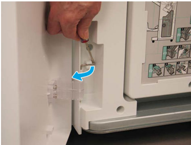
Figure 5-301 Release the lower hinge pin
