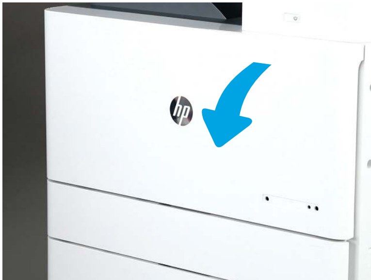
Figure 2-287 Open the front cover
