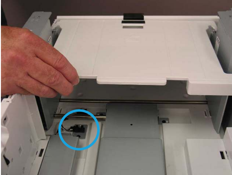
Figure 2-650 Remove the HCI photo interrupter and sensor bracket
