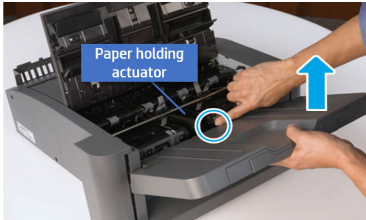
Figure 6-693 Remove the output tray.
