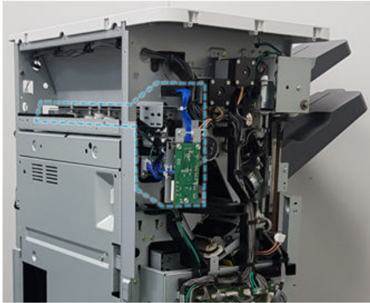
Figure 5-25 Punch unit detail view
