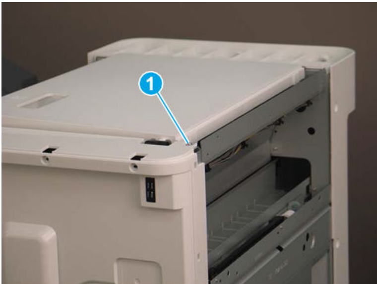
Figure 5-1176 Remove one screw
