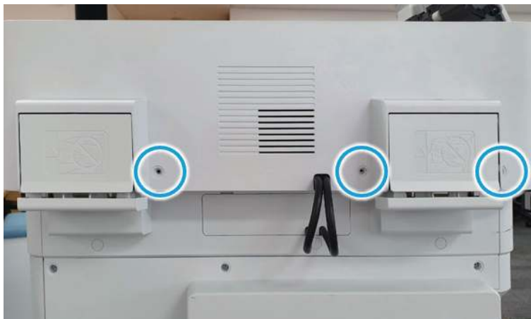
Figure 2-359 Remove 3 caps and 3 screws.
