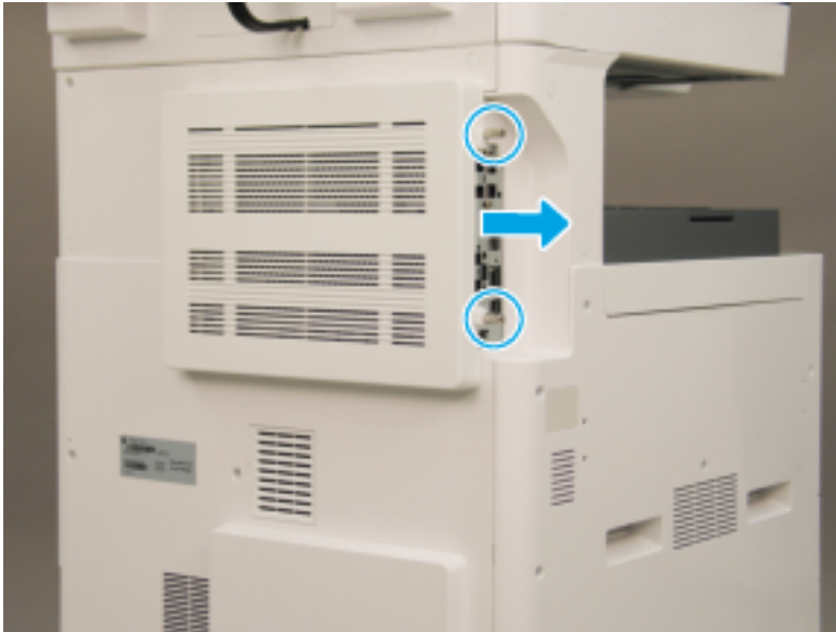
Figure 2-75 Remove the formatter cover
