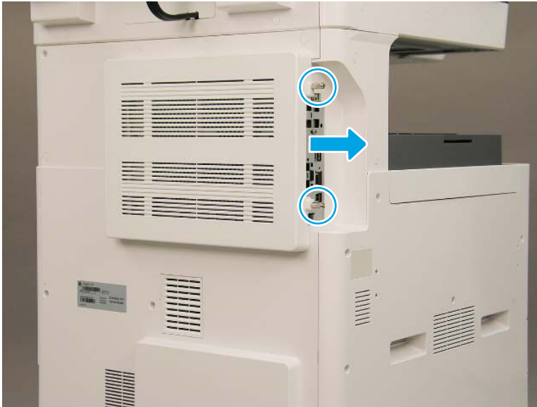
Figure 2-19 Remove the formatter cover
