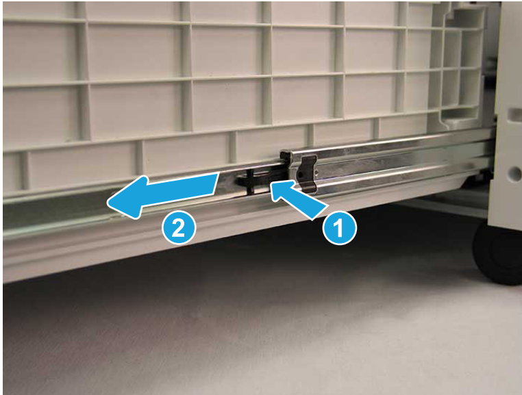
Figure 2-648 Release the tray right-side slide lock
