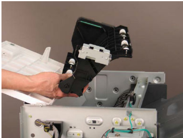
Figure 5-394 Remove the top jam access cover
