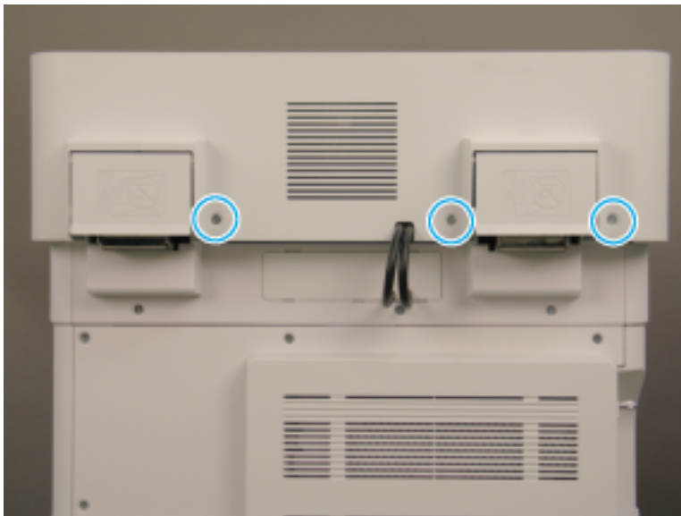
Figure 2-473 Remove the document feeder back cover bottom screws
