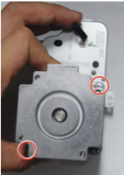
Figure 2-542 Remove the feed motor
