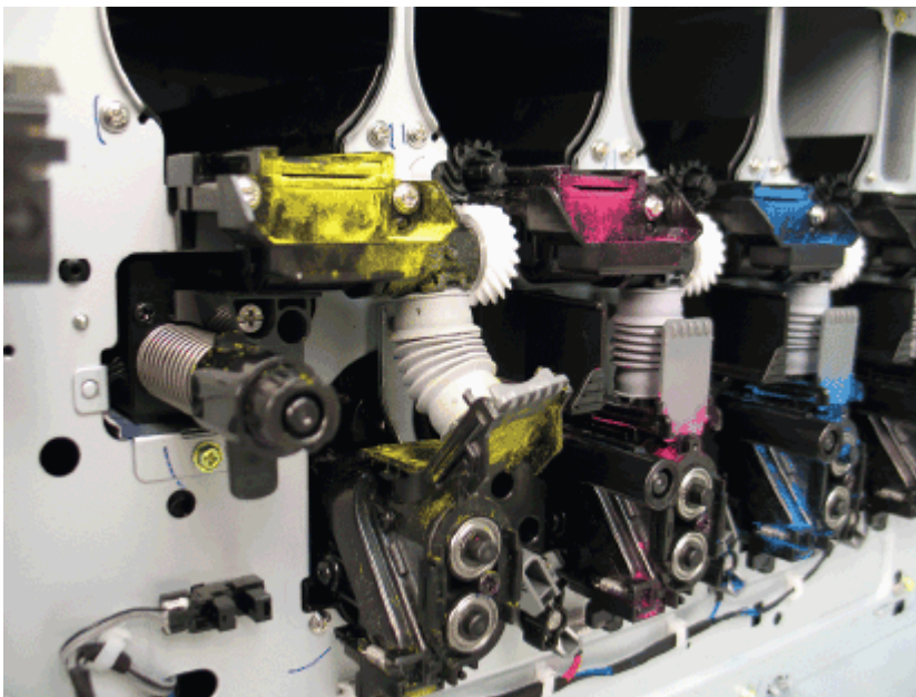
Figure 2-177 Remove the developer unit shutter duct
