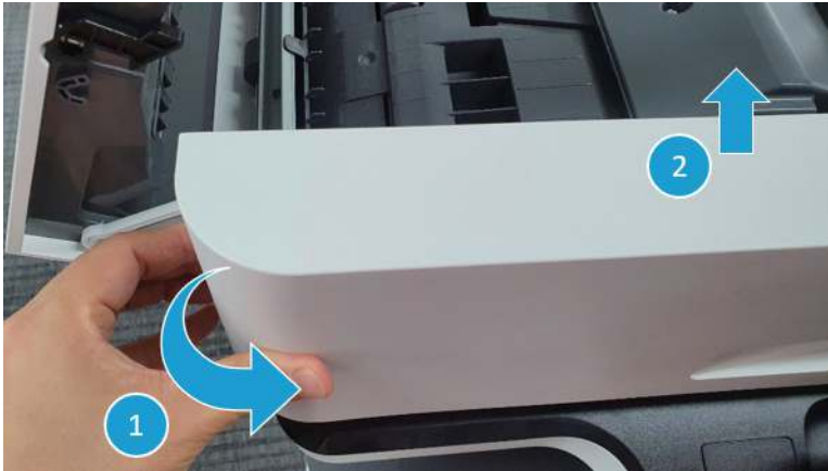
Figure 2-432 Remove the document feeder front cover
