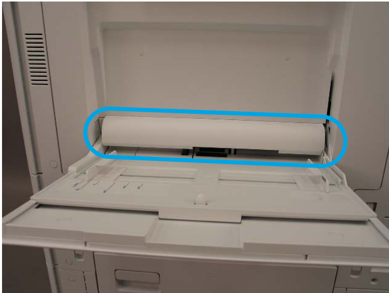
Figure 2-334 Remove MP front cover
