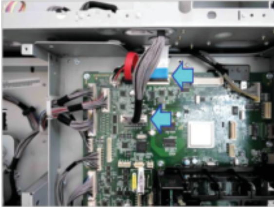
Figure 2-47 Disconnect scan cables
