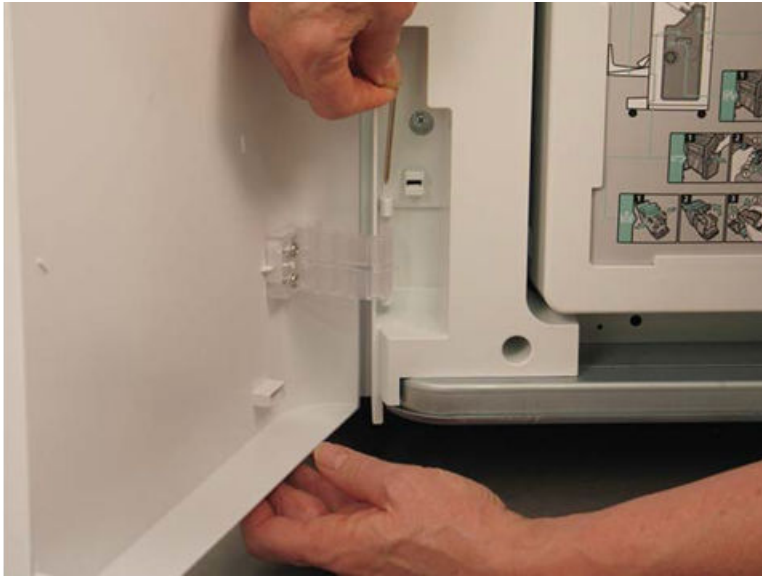
Figure 5-926 Remove the lower hinge pin
