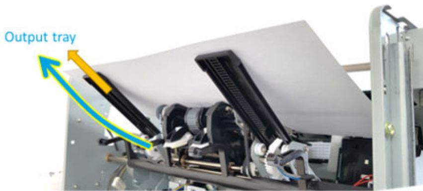
Figure 6-25 Inner finisher system - paper support unit operation
