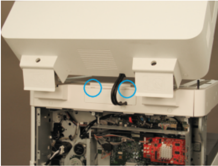
Figure 2-33 Remove document feeder connector cover
