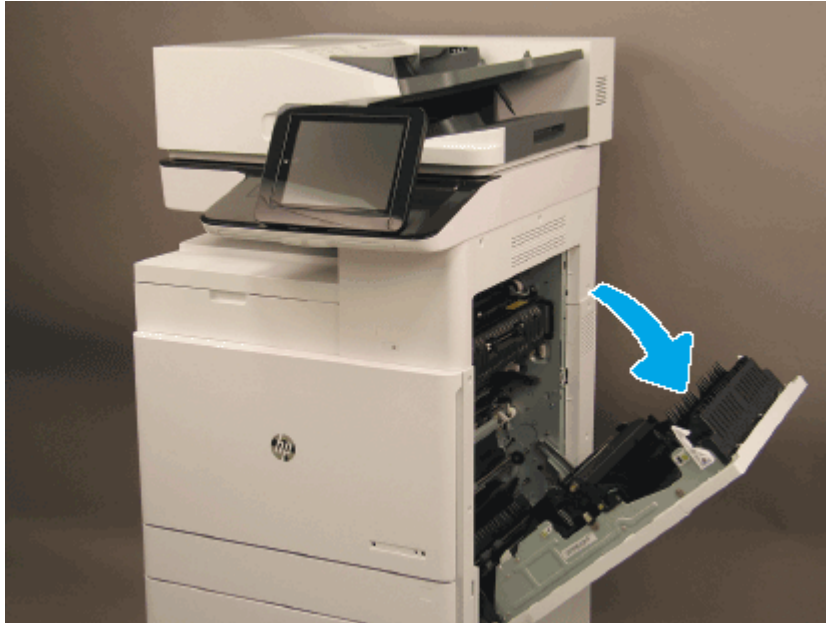
Figure 2-297 Open right door
