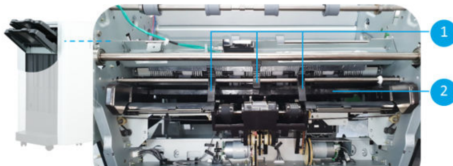
Figure 5-37 Paddle unit detail view - left
