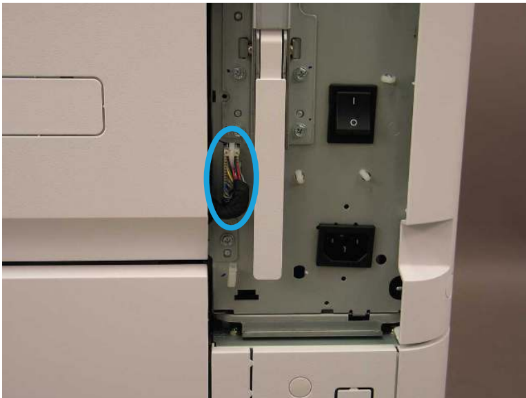
Figure 2-60 Disconnect right door connector
