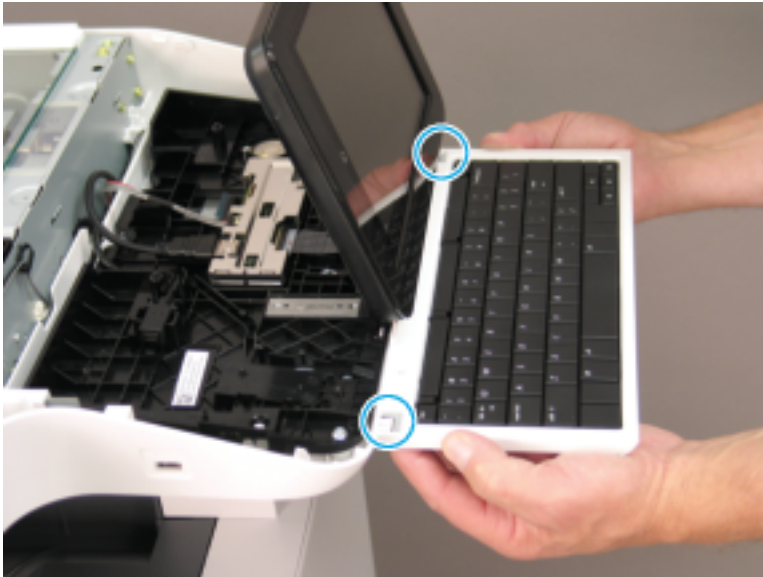
Figure 2-42 Remove the keyboard
