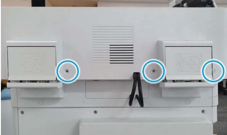
Figure 2-374 Remove 3 caps and 3 screws.
