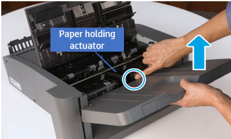
Figure 6-576 Remove the output tray.
