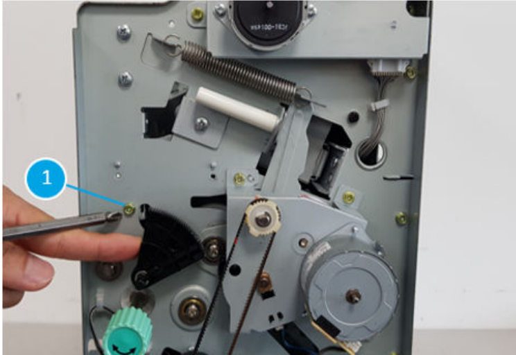
Figure 5-1857 Remove one screw at the front of the booklet maker
