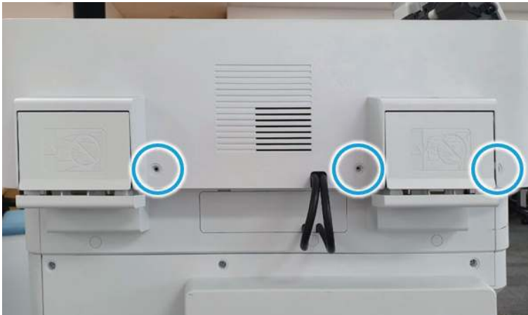
Figure 2-416 Remove 3 caps and 3 screws.
