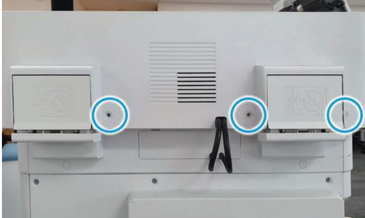
Figure 2-367 Remove 3 caps and 3 screws.
