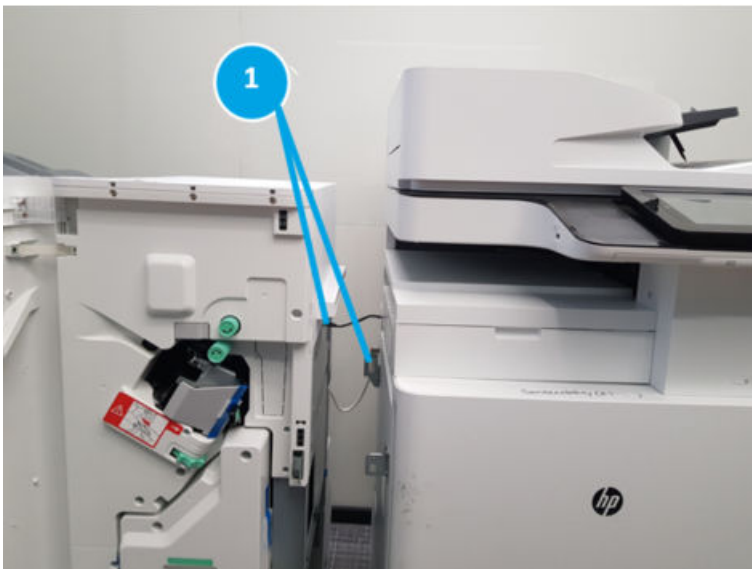
Figure 5-124 Separate the finisher from the printer and disconnect the two connectors
