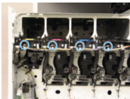
Figure 2-305 Disconnect four connectors
