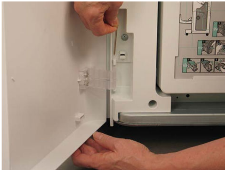
Figure 5-990 Remove the lower hinge pin
