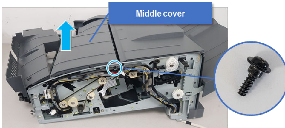
Figure 6-615 Remove the middle cover
