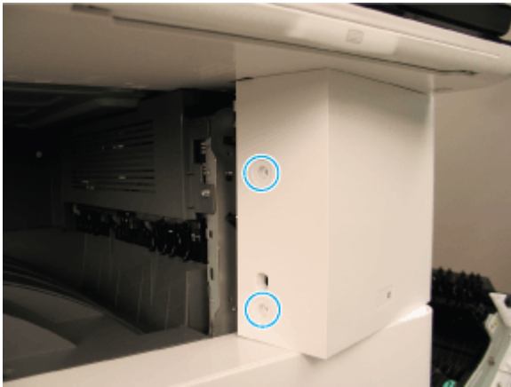
Figure 2-127 Remove the power-switch cover
