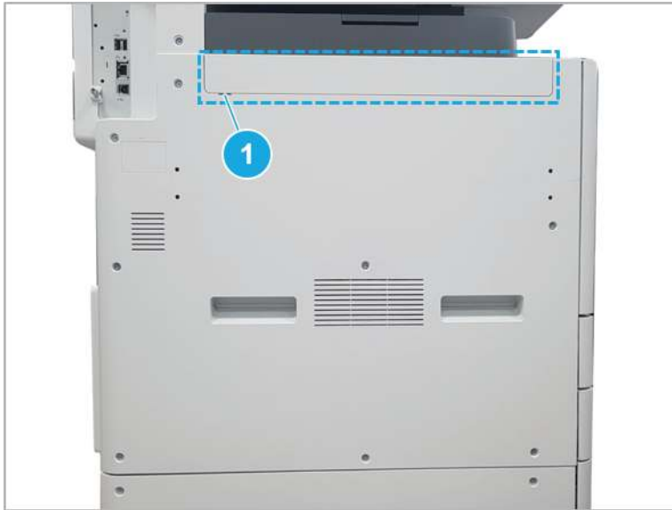
Figure 2-322 Remove the left trim cover
