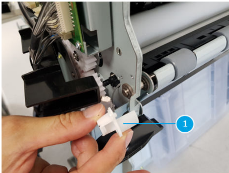
Figure 5-1900 Remove the white bush
