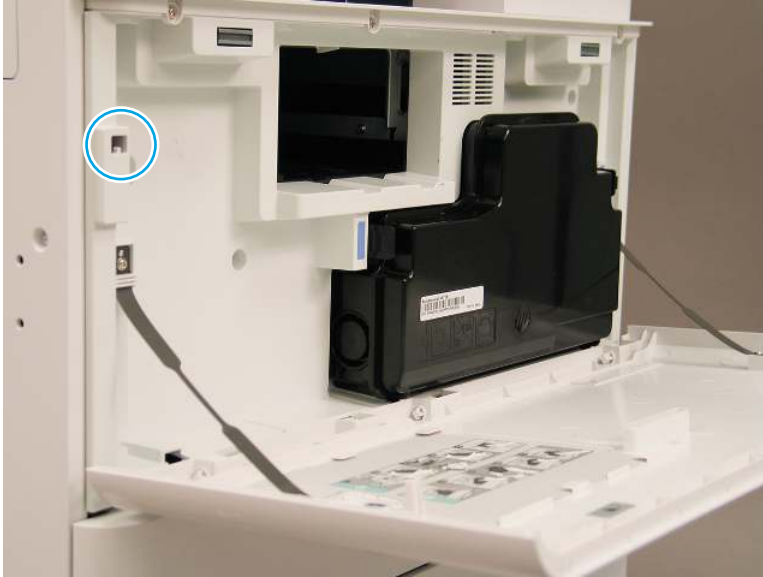
Figure 3-12 Defeat the toner cartridge door interlock
