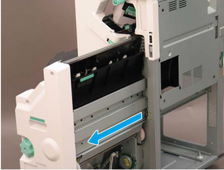
Figure 5-1820 Extend the right rail
