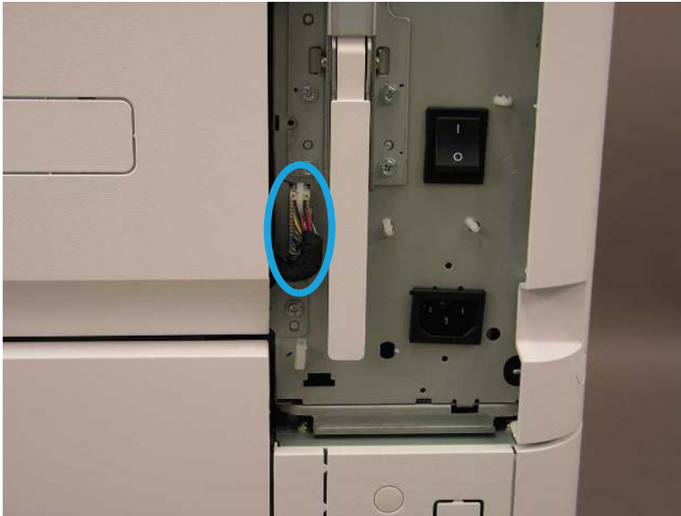
Figure 2-191 Disconnect right door connector
