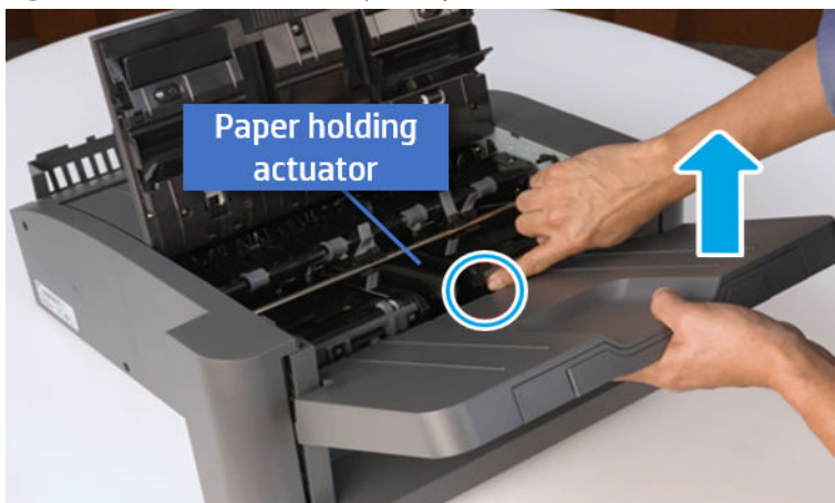
Figure 6-539 Remove the output tray.
