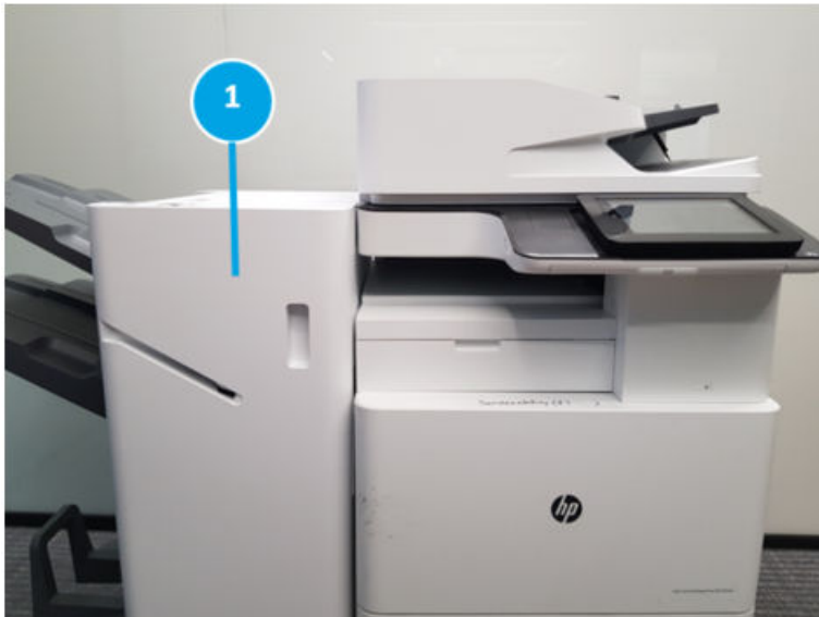
Figure 5-132 Open the front door
