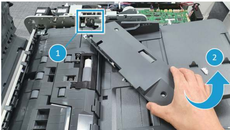
Figure 2-428 Remove the pickup roller assembly
