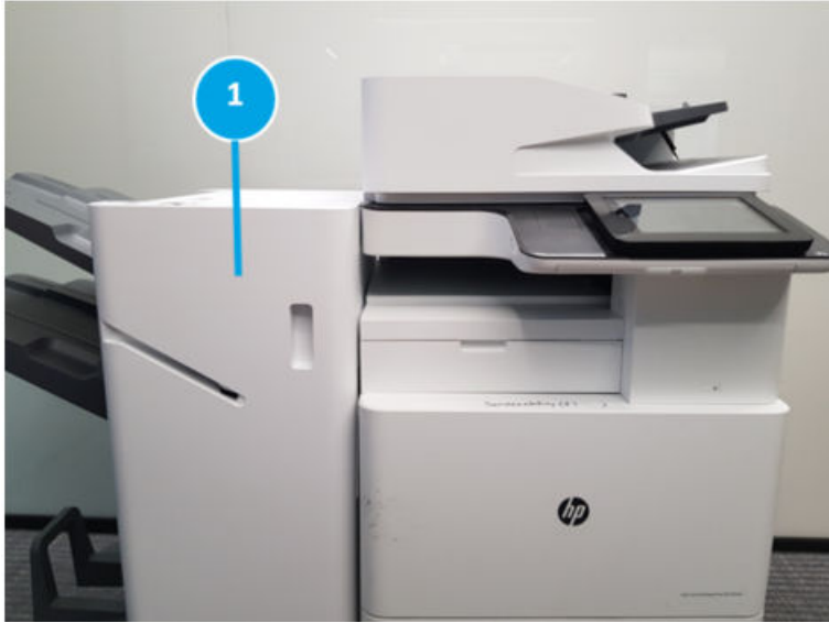
Figure 5-141 Open the front door
