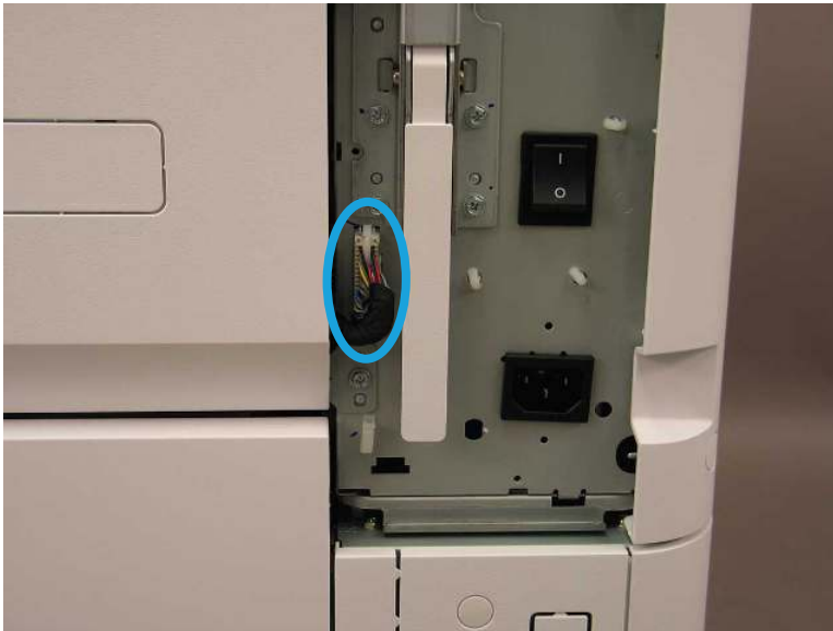
Figure 2-242 Disconnect right door connector
