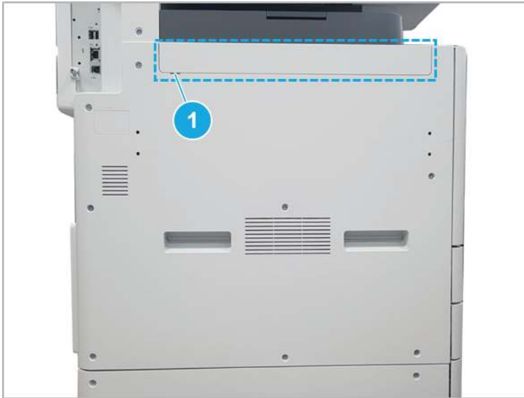
Figure 2-258 Remove the left trim cover
