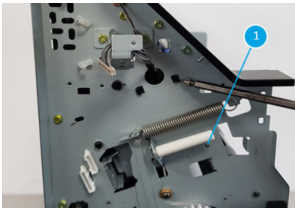
Figure 5-1695 Remove one screw
