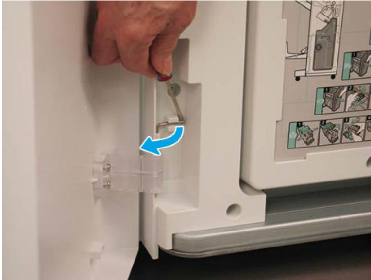
Figure 5-989 Release the lower hinge pin
