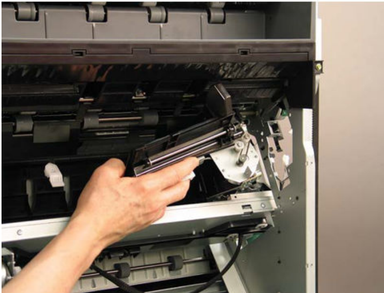
Figure 5-664 Remove the front tamper
