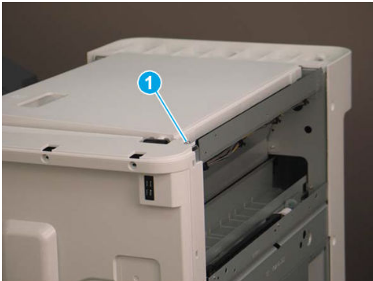
Figure 5-305 Remove one screw
