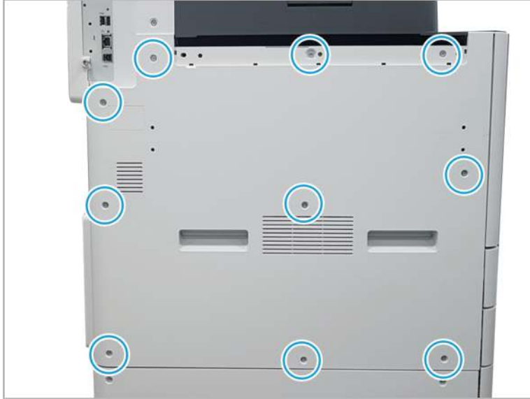
Figure 2-255 Remove the left cover
