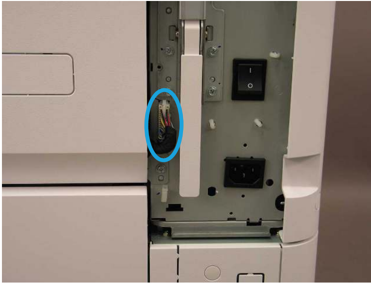
Figure 2-234 Disconnect right door connector
