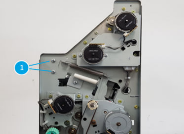
Figure 5-1687 Remove two screws
