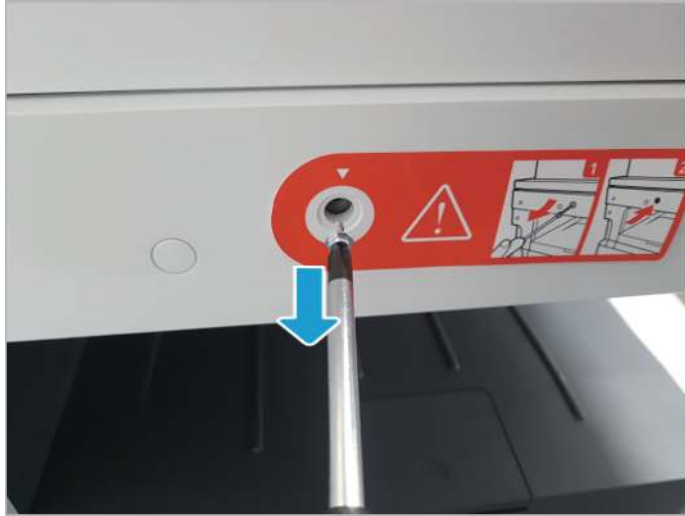
Figure 1-50 Remove scan locking screw
