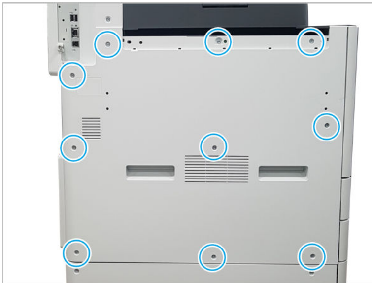
Figure 2-50 Remove the left cover
