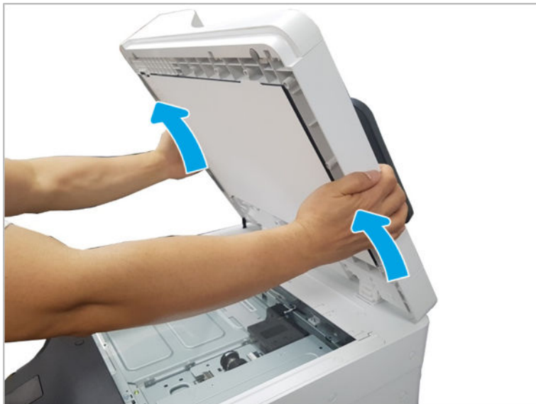
Figure 2-295 Release the ADF
