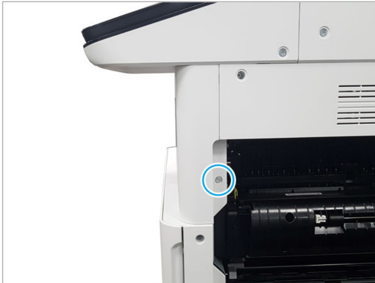
Figure 2-125 Remove one screw
