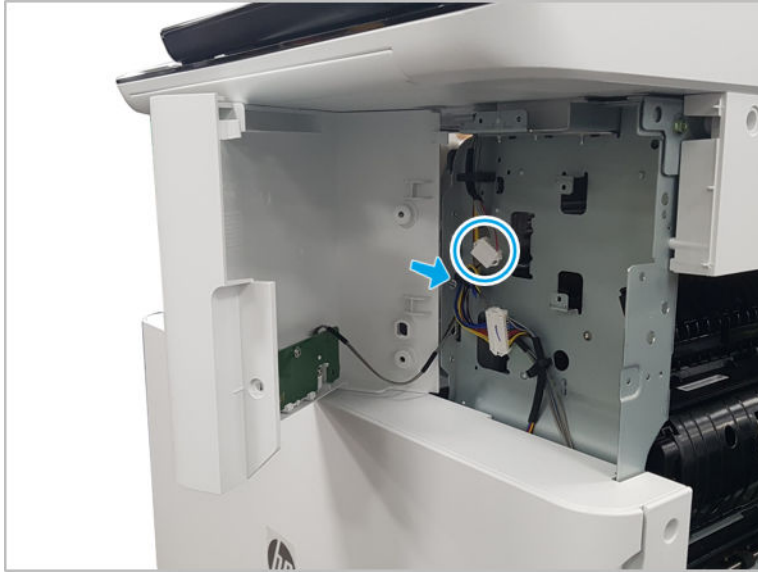
Figure 2-115 Remove the middle right cover
