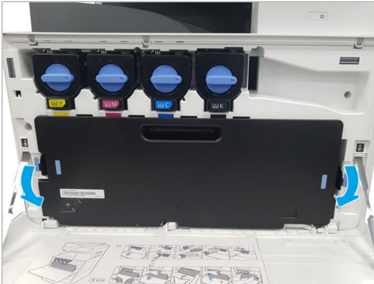
Figure 2-3 Remove toner collection unit
