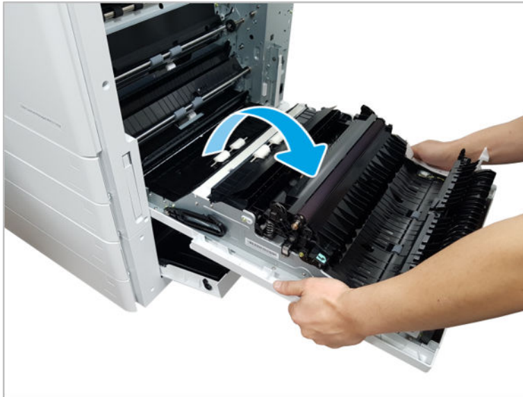
Figure 2-164 Remove right door
