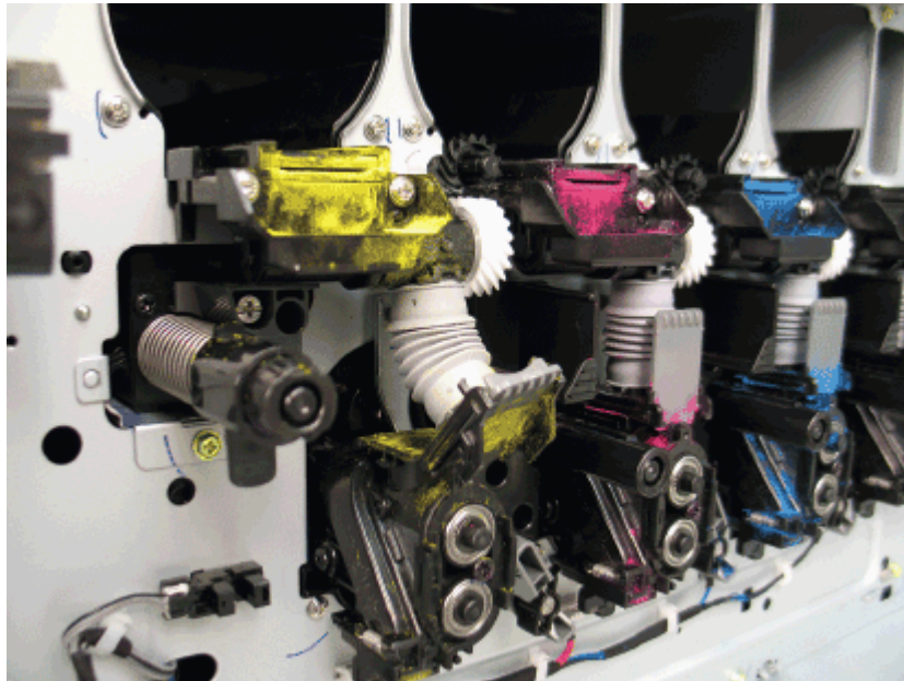
Figure 2-131 Remove the developer unit shutter duct
