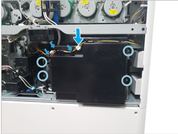
Figure 2-38 Remove the LVPS cover
