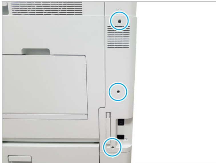
Figure 2-277 Remove the right-rear cover
