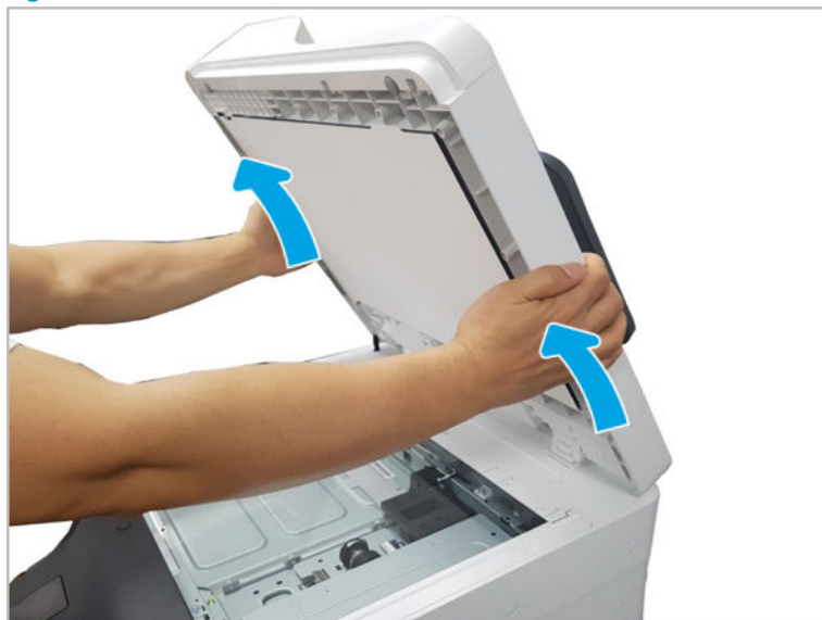
Figure 2-317 Release the document feeder
