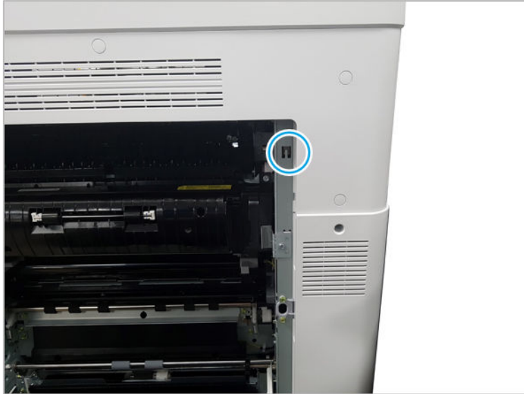
Figure 3-13 Defeat the front door interlock
