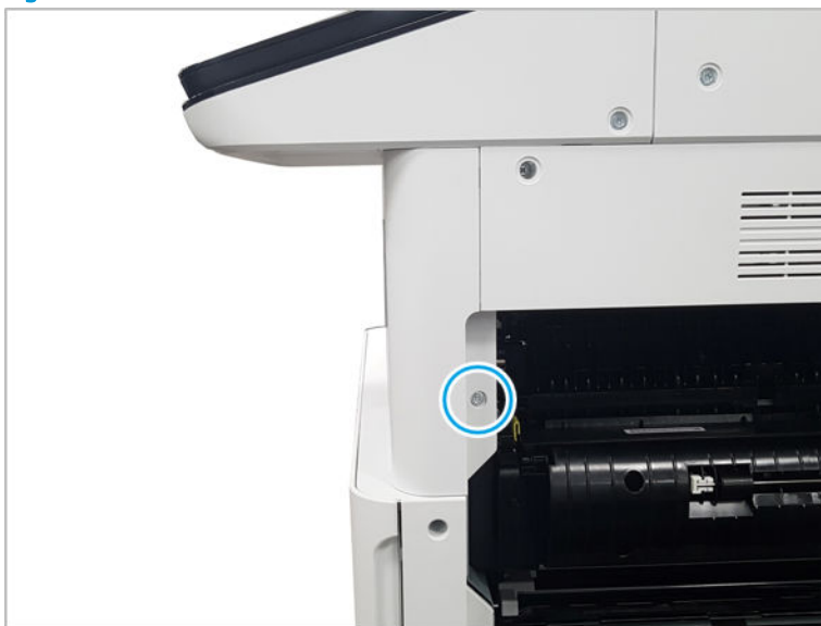
Figure 2-172 Remove one screw
