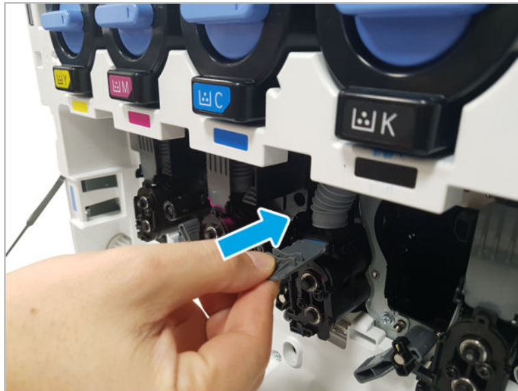
Figure 2-68 Close the shutter
