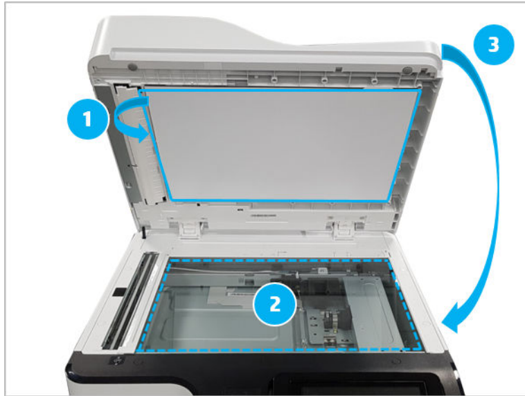
Figure 3-60 Detach and attach the sponge sheet
