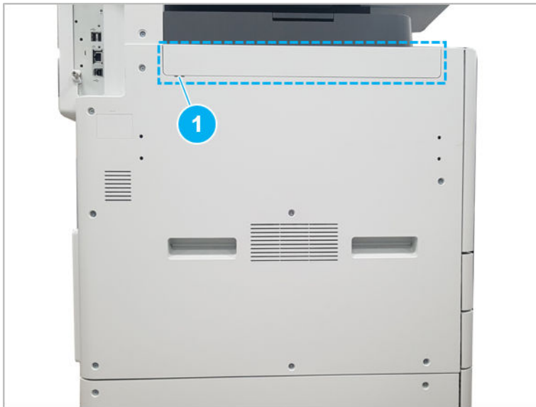
Figure 2-101 Remove the left trim cover
