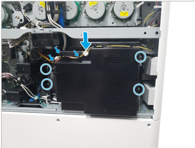
Figure 2-42 Remove the LVPS cover
