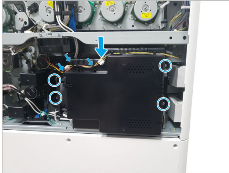
Figure 2-46 Remove the LVPS cover
