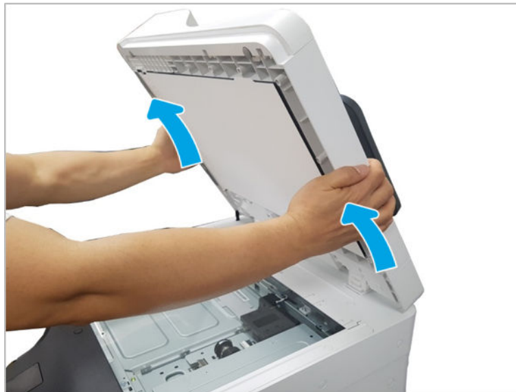
Figure 2-345 Release the document feeder
