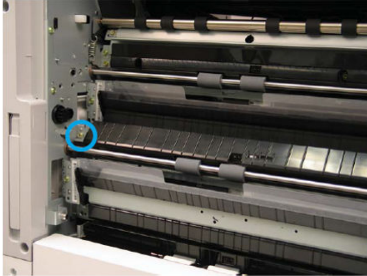
Figure 2-165 Remove one screw
