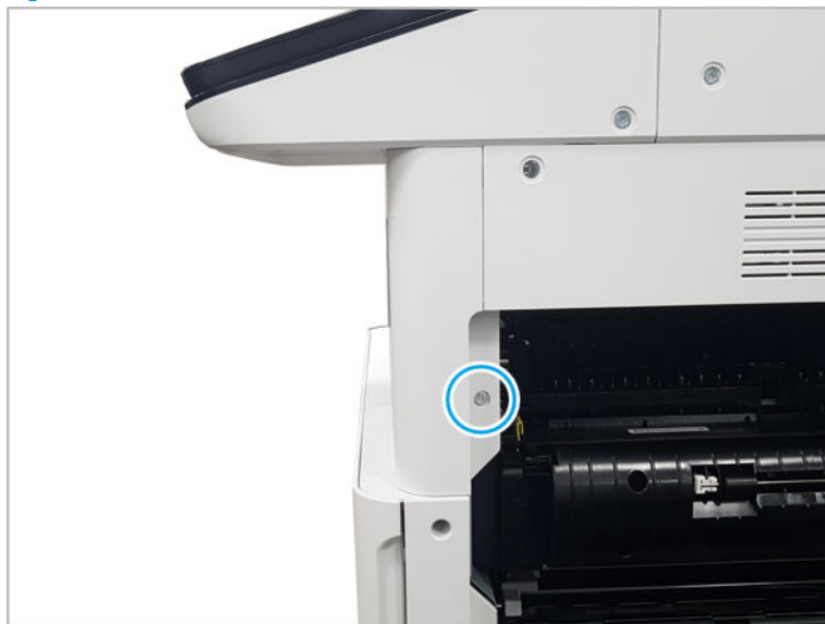
Figure 2-193 Remove one screw
