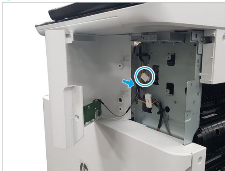
Figure 2-188 Remove the middle right cover
