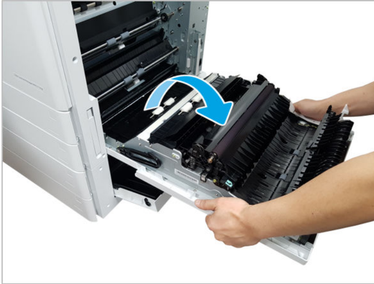
Figure 2-270 Remove right door
