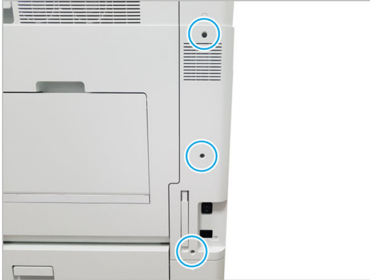
Figure 2-149 Remove the right-rear cover.
