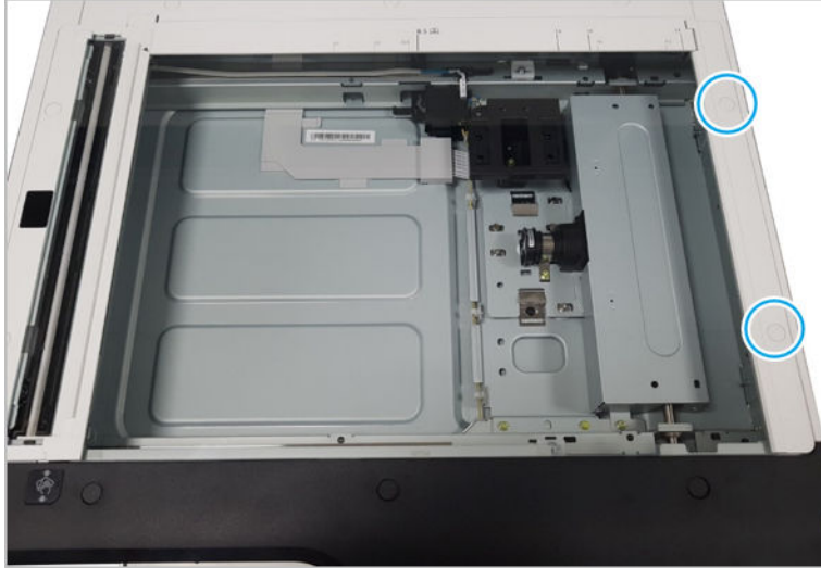
Figure 2-336 Remove screws and scanner glass right cover
