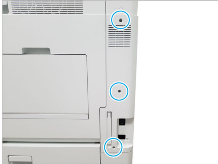
Figure 2-142 Remove the right-rear cover
