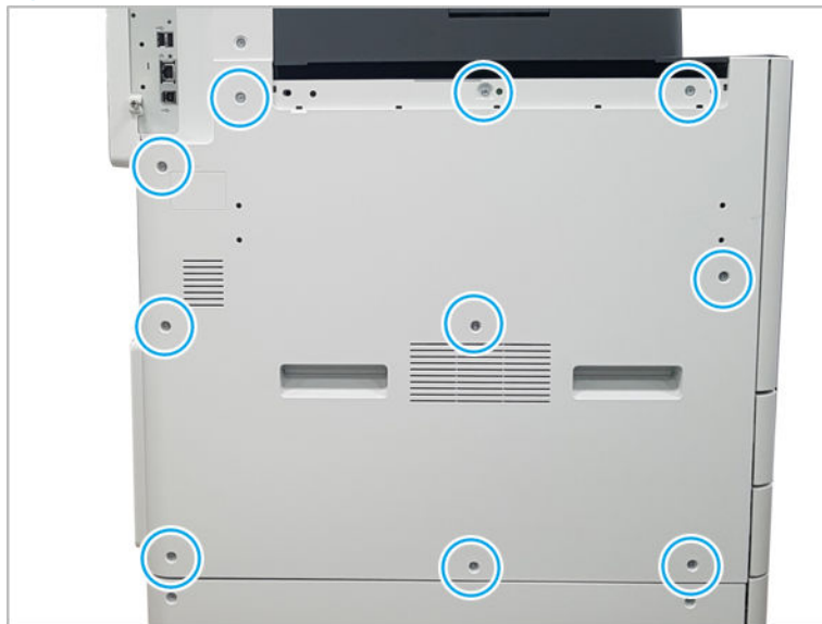
Figure 2-57 Remove the left cover
