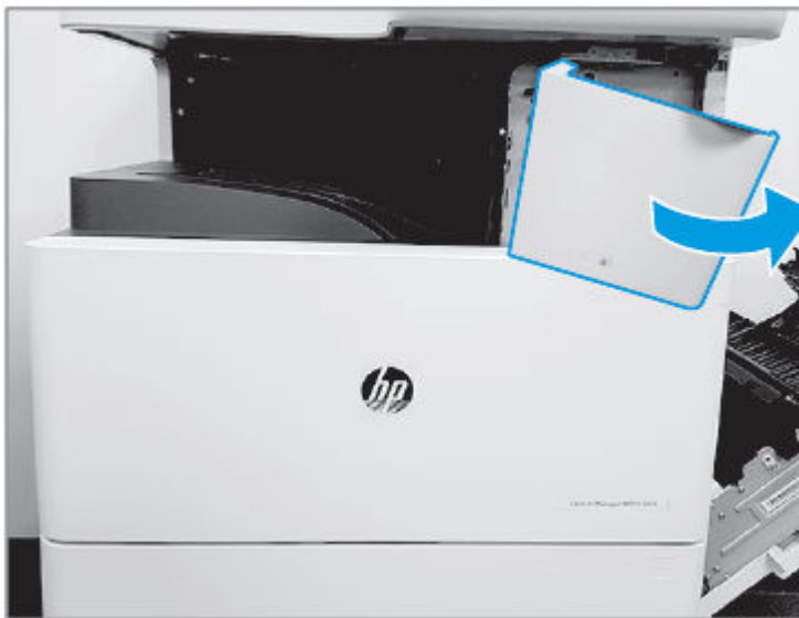
Figure 2-387 Remove the middle right cover
