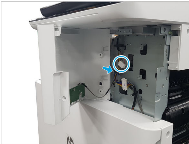
Figure 2-195 Remove the middle right cover
