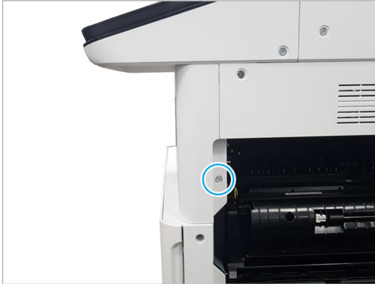
Figure 2-113 Remove one screw
