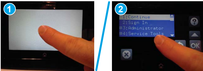
Figure 3-14 Open the Pre-boot menu
