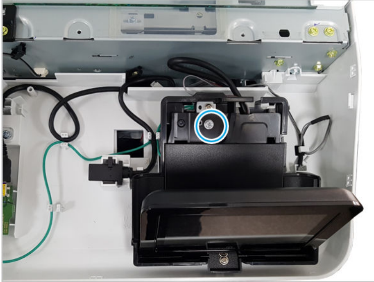
Figure 2-297 Remove one screw
