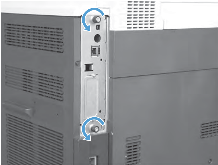
Figure 2-10 Remove the formatter
