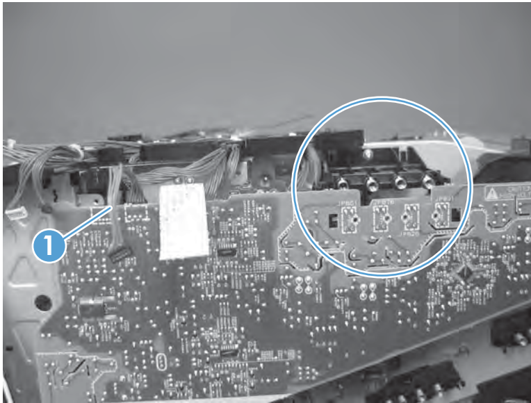
Figure 2-192 Reinstall the high-voltage power supply upper
