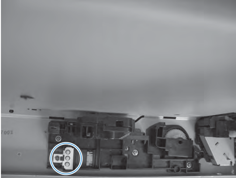
Figure 3-22 Test the Tray 2 paper size switches
