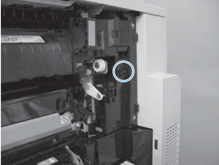
Figure 3-18 Test the right door switch
