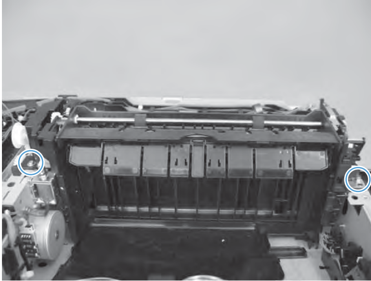
Figure 2-116 Remove the delivery assembly (4 of 7)
