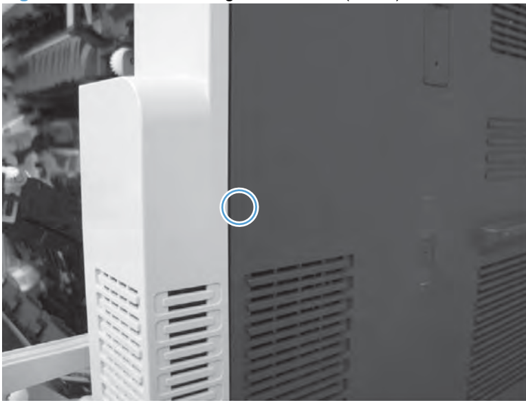
Figure 2-57 Remove the right-rear cover (1 of 2)
