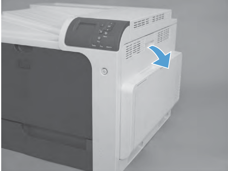
Figure 2-71 Remove the secondary transfer assembly (1 of 3)
