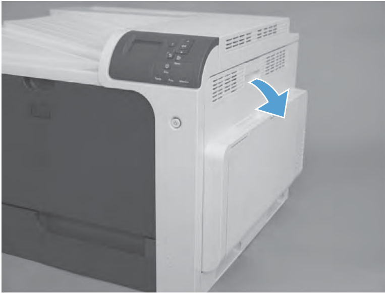
Figure 2-69 Remove the cassette feed guide (1 of 2)
