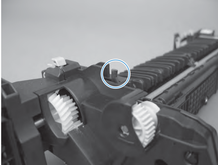
Figure 3-7 Test the fuser delivery sensor (1 of 2)
