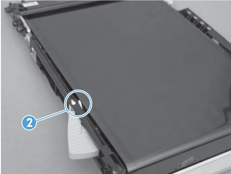
Figure 3-13 Test the primary transfer-roller-disengagement sensor (2 of 4)
