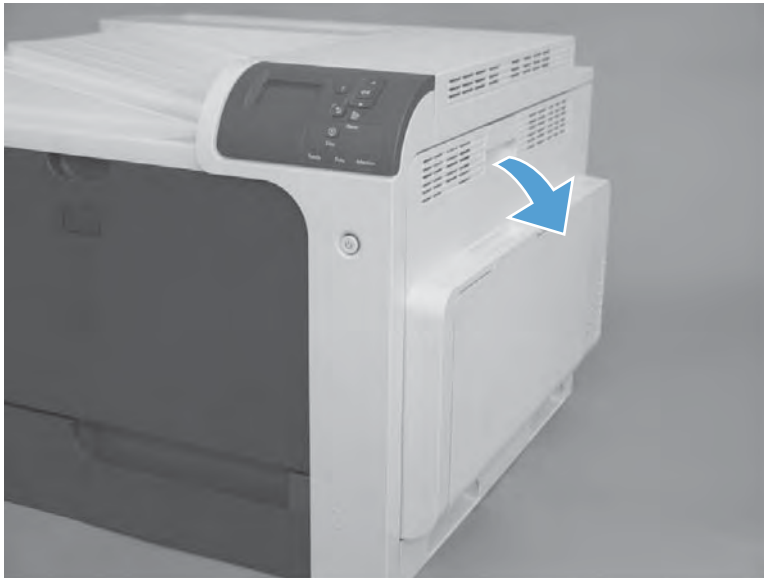
Figure 2-18 Remove the fuser (1 of 2)
