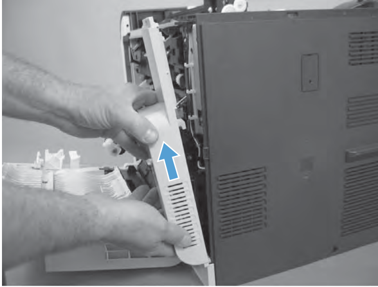
Figure 2-58 Remove the right-rear cover (2 of 2)
