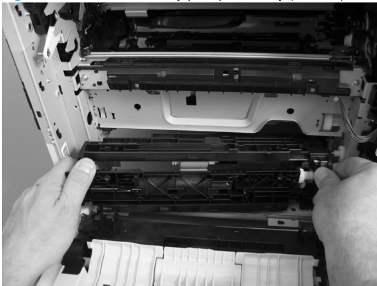
Figure 2-174 Remove the tray-pickup assembly (11 of 11)
