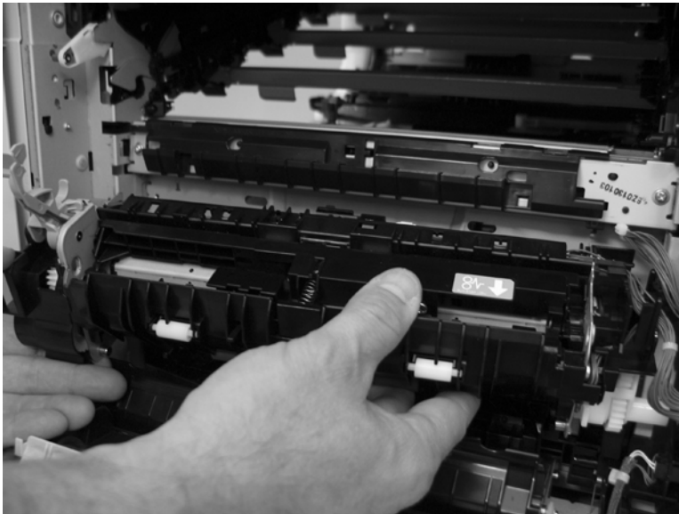
Figure 2-95 Remove the registration assembly (8 of 8)
