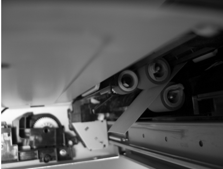
Figure 3-23 Test the Tray 3 feed sensor
