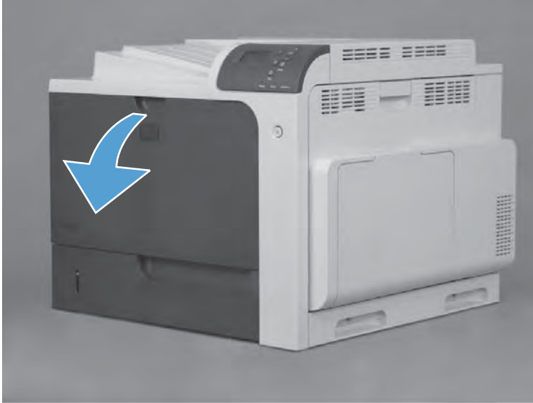
Figure 2-35 Remove the upper-left cover (1 of 3)
