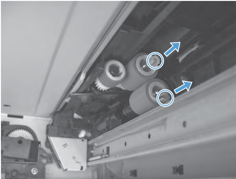
Figure 2-20 Remove the Pickup and feed rollers (Trays 2-5)
