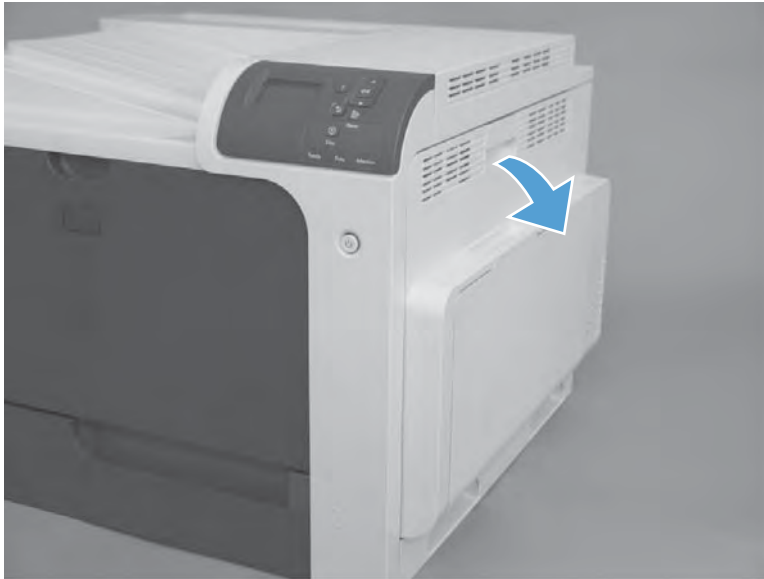
Figure 2-60 Remove the right-door assembly (1 of 9)
