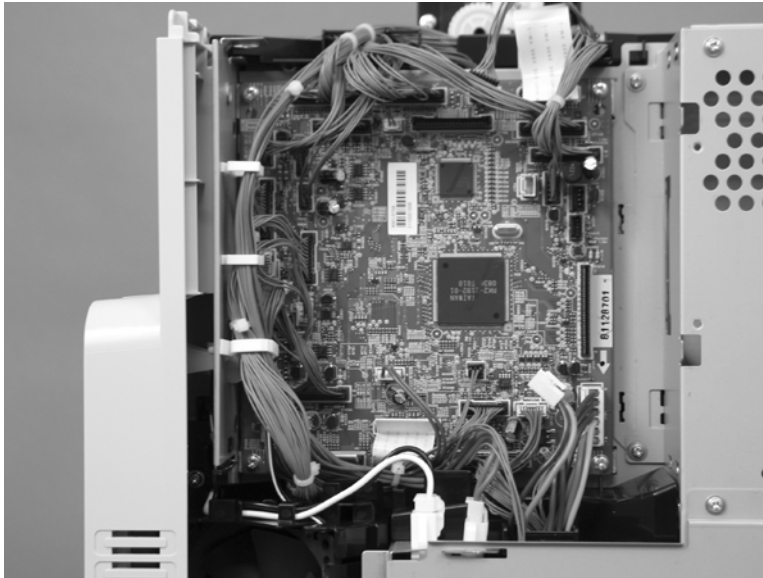
Figure 2-137 Remove the DC controller PCA and tray (1 of 3)
