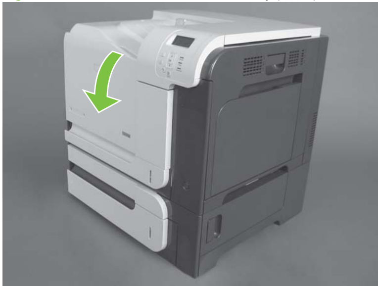
Figure 6-42 Remove the front-door assembly (1 of 2)
