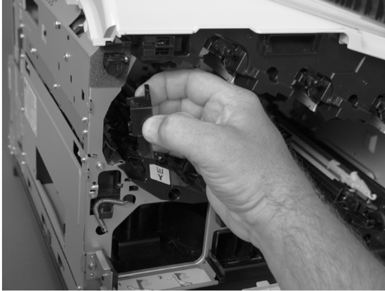
Figure 6-94 Remove the residual-toner-feed motor (2 of 7)
