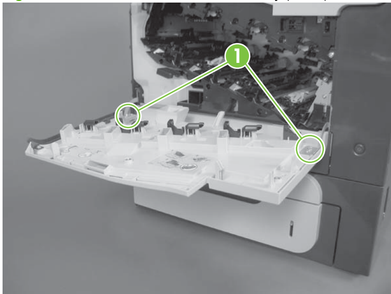
Figure 6-43 Remove the front-door assembly (2 of 2)
