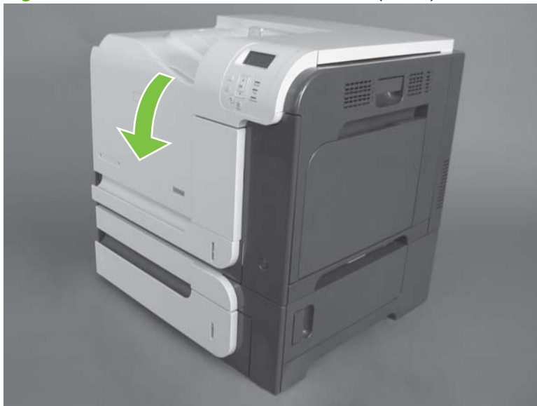
Figure 6-9 Remove the toner-collection unit (1 of 4)
