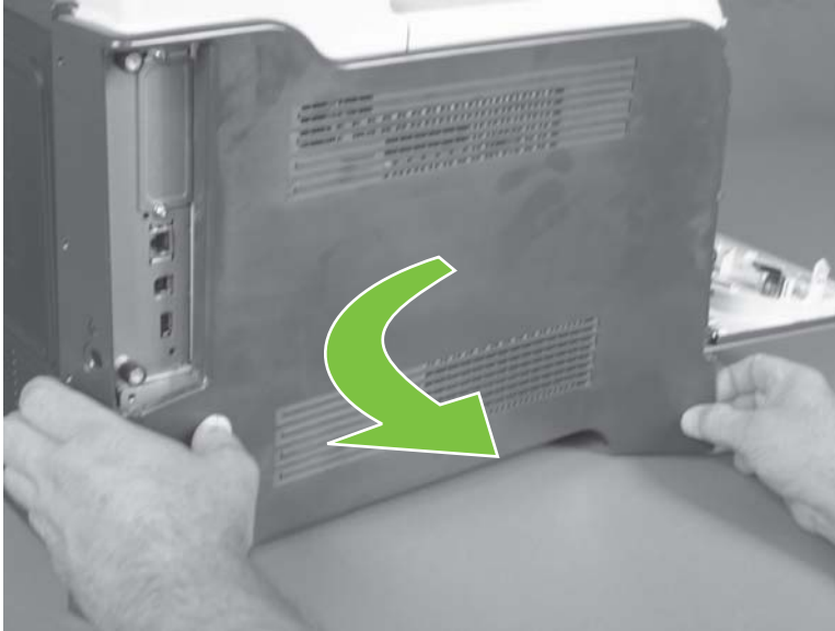
Figure 6-59 Remove the left cover (5 of 5)
