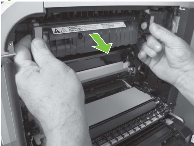
Figure 6-19 Remove the fuser (2 of 2)
