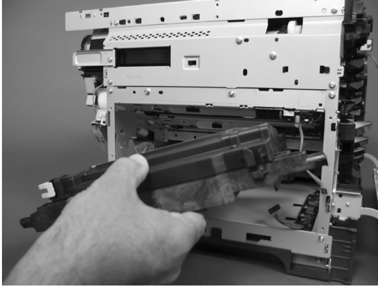
Figure 6-171 Remove the laser/scanner assembly (Y/M) (12 of 12)
