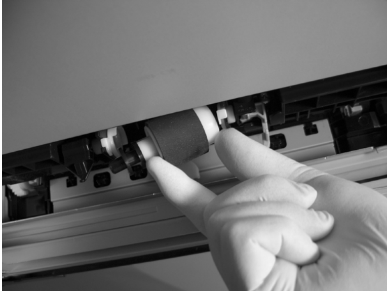
Figure 6-22 Remove the pickup roller (Tray 2) (3 of 4)
