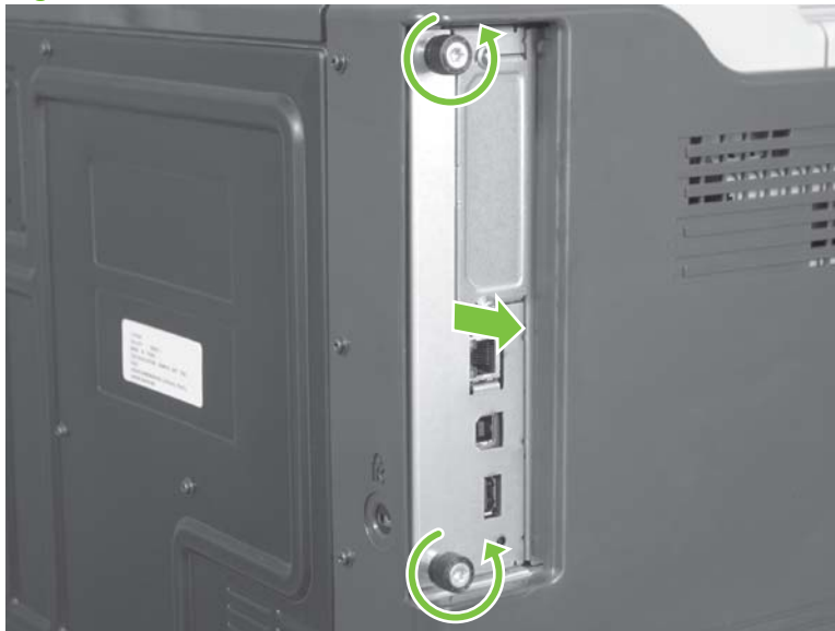
Figure 6-13 Remove the formatter
