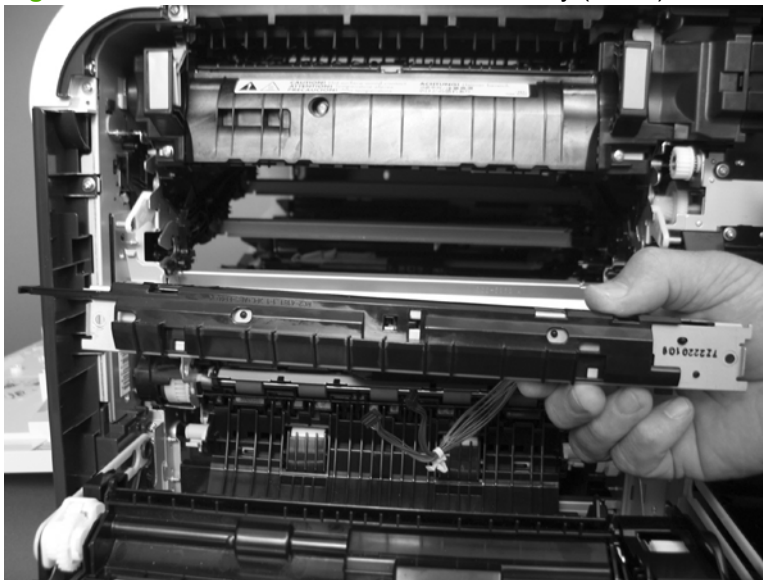
Figure 6-106 Remove the RD sensor assembly (6 of 6)
