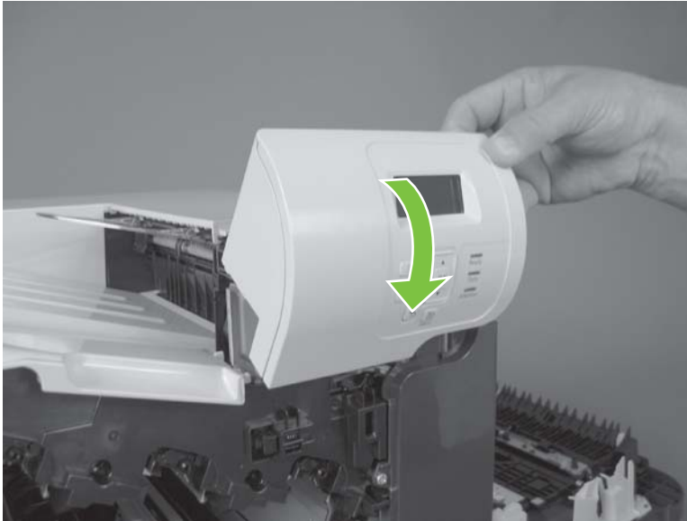
Figure 6-62 Remove the control-panel assembly (3 of 4)
