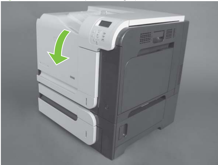
Figure 6-5 Remove the print cartridge (1 of 2)
