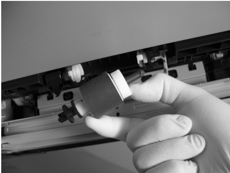
Figure 6-23 Remove the pickup roller (Tray 2) (4 of 4)
