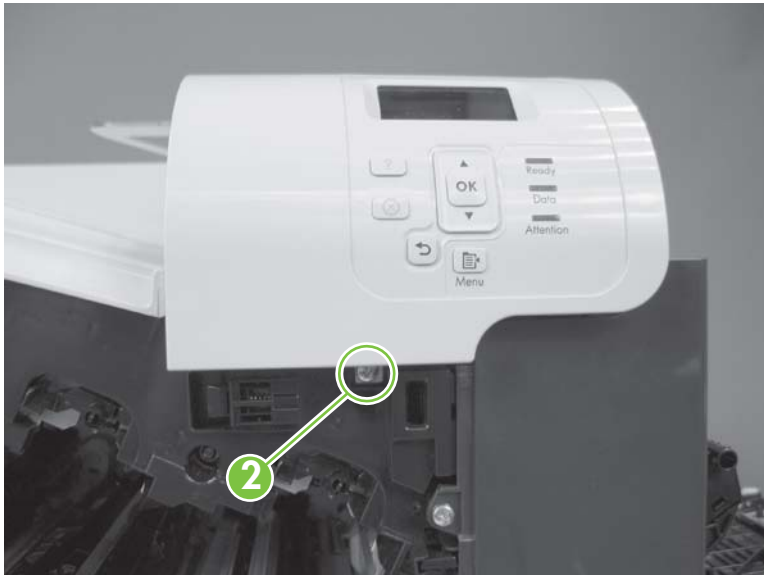
Figure 6-61 Remove the control-panel assembly (2 of 4)
