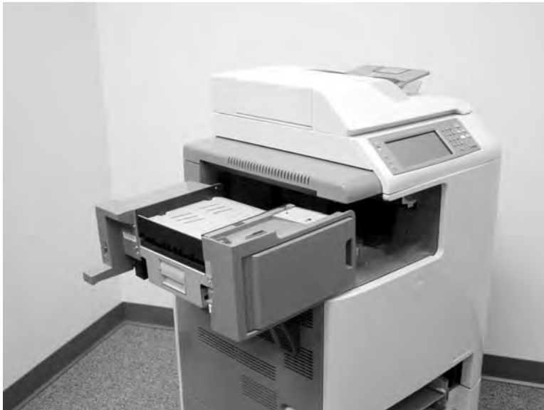
Figure 5-9 Remove the IPTU (2 of 3)
