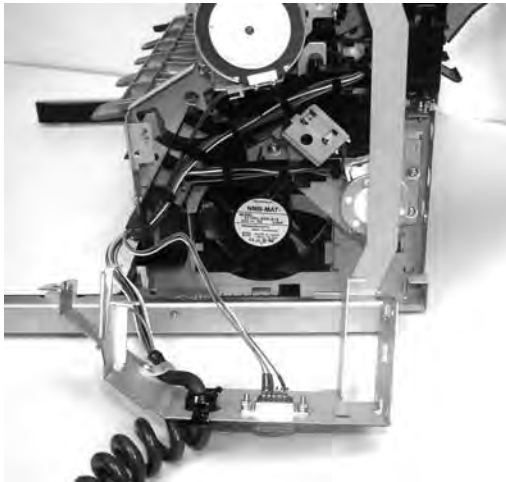
Figure 5-384 Remove the jogger unit (3 of 7)
