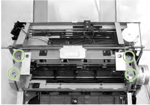
Figure 5-387 Remove the jogger unit (6 of 7)
