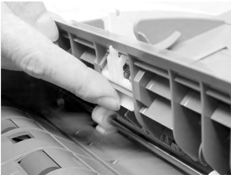
Figure 5-37 Remove the ADF separation pad (4 of 4)
