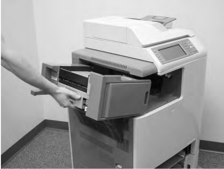
Figure 5-10 Remove the IPTU (3 of 3)
