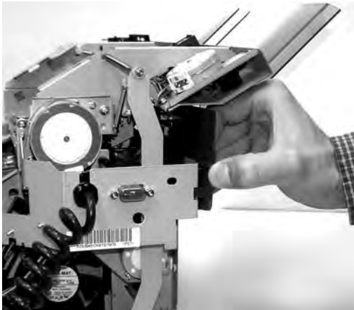
Figure 5-382 Remove the jogger unit (1 of 7)
