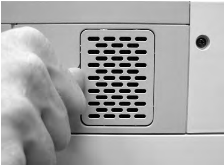
Figure 5-57 Remove the scanner filter (1 of 2)
