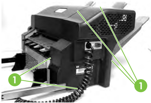
Figure 5-374 Claw locations on rear cover
