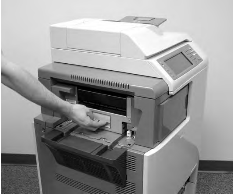
Figure 5-8 Remove the IPTU (1 of 3)
