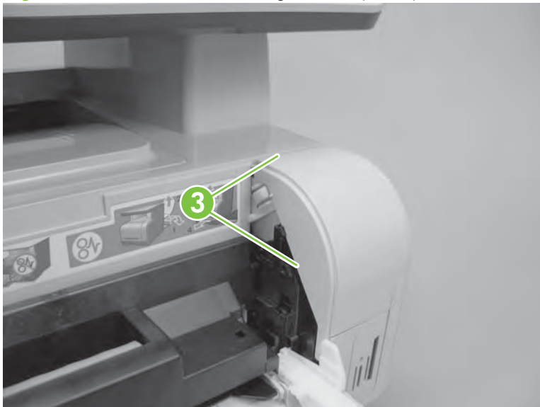
Figure 6-45 Remove the front-right cover (2 of 3)
