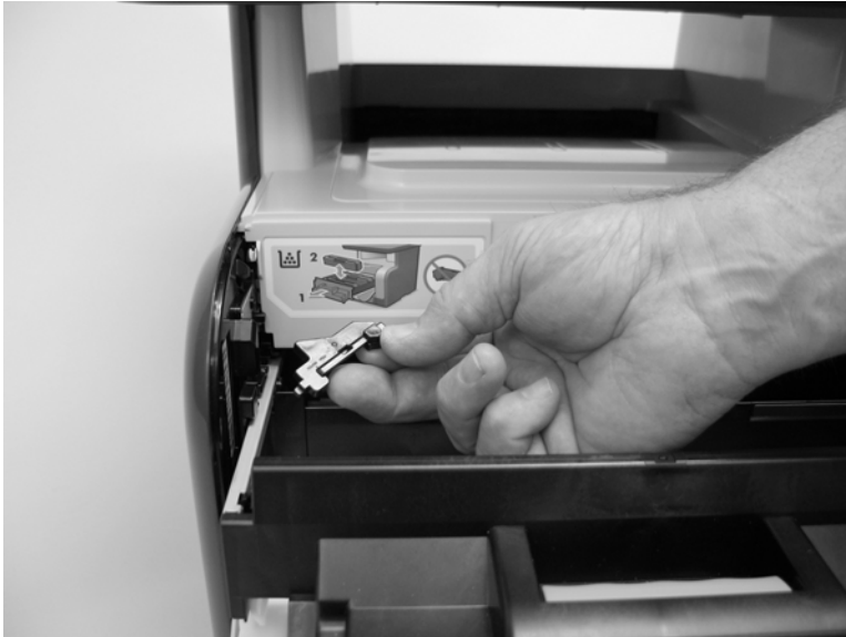
Figure 6-25 Remove the front door and front-lower cover (4 of 13)
