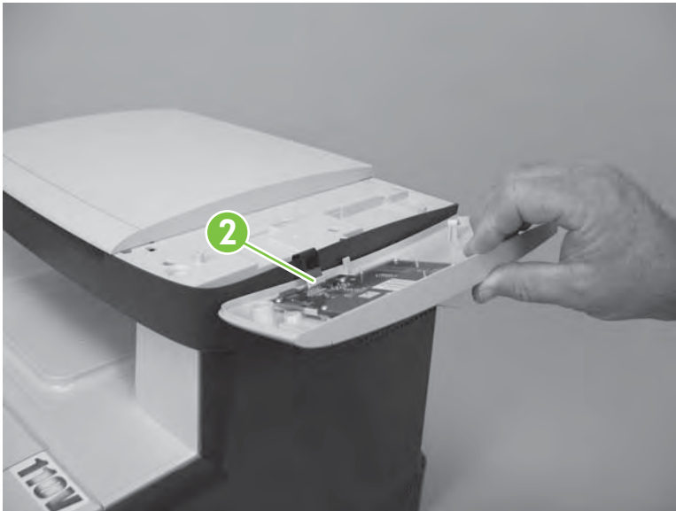
Figure 6-7 Remove the control-panel (3 of 3; base model)
