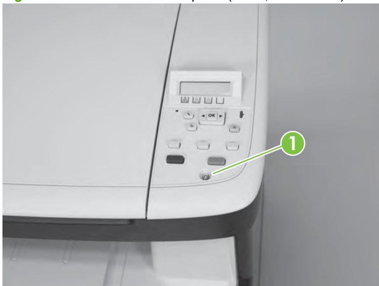
Figure 6-5 Remove the control-panel (1 of 3; base model)
