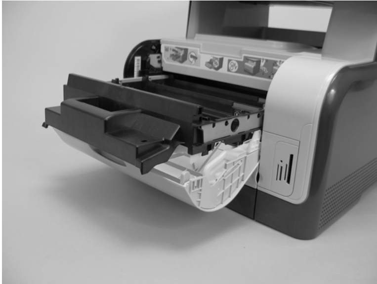
Figure 6-66 Remove the print-cartridge drawer (1 of 5)
