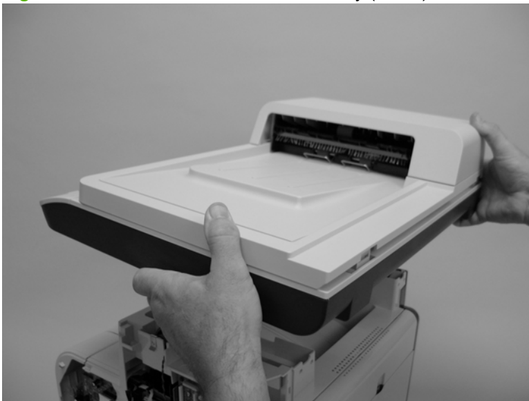
Figure 6-62 Remove the scanner assembly (4 of 4)
