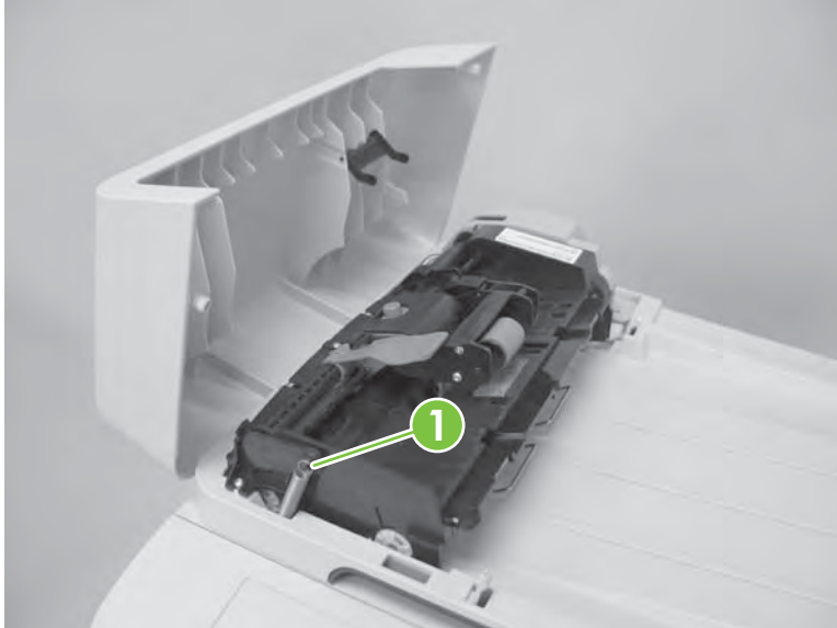
Figure 6-13 Remove the ADF pickup roller assembly (1 of 2)
