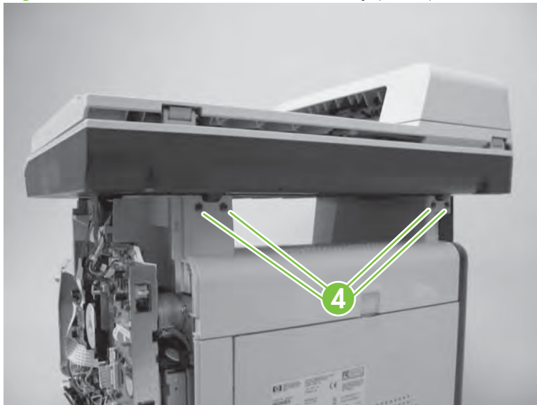
Figure 6-60 Remove the scanner assembly (2 of 4)
