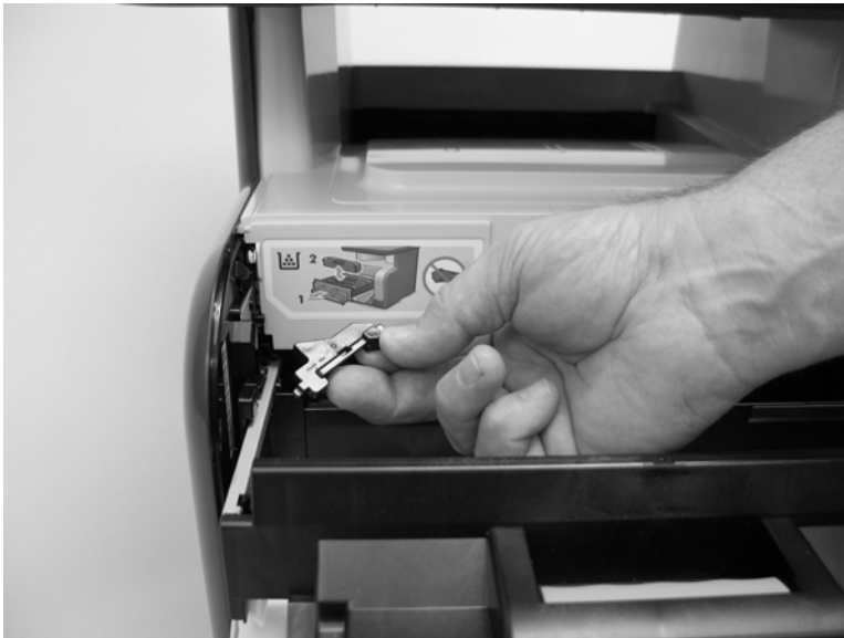
Figure 6-69 Remove the print-cartridge drawer (4 of 5)
