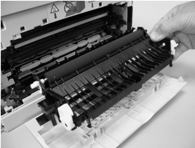
Figure 6-21 Remove the paper-guide assembly (2 of 2)
