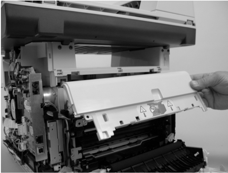
Figure 6-54 Remove the rear-upper cover (2 of 2)
