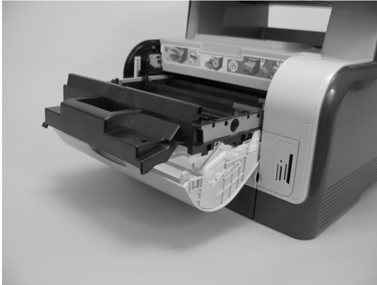
Figure 6-22 Remove the front door and front-lower cover (1 of 13)
