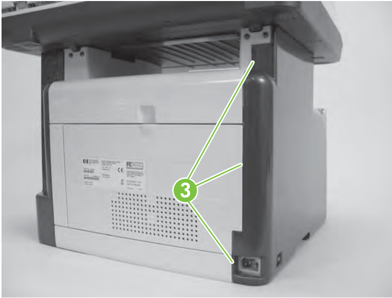
Figure 6-42 Remove the left cover (3 of 4)
