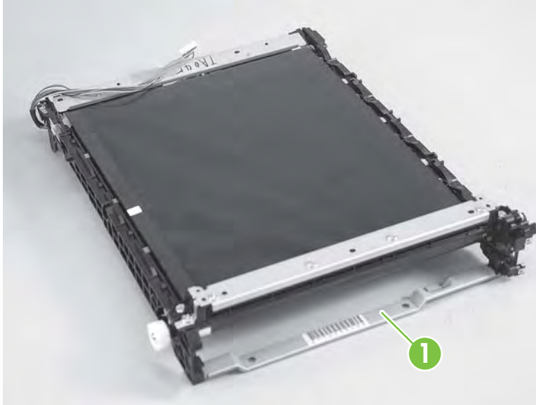
Figure 6-80 Reinstall the ITB (1 of 2)
