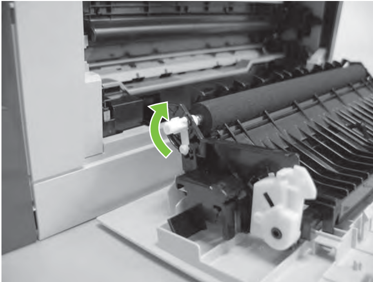
Figure 6-17 Remove the transfer roller (1 of 3)
