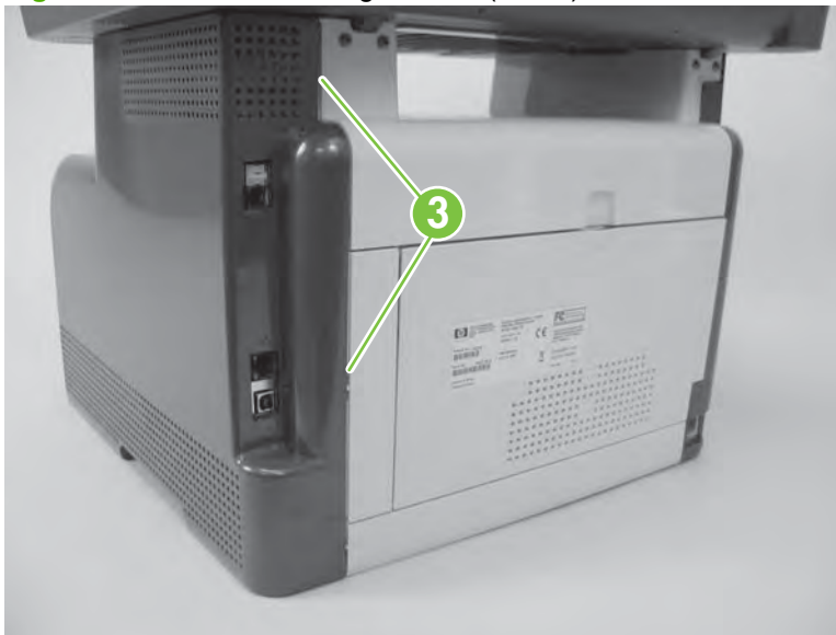
Figure 6-38 Remove the right cover (4 of 5)
