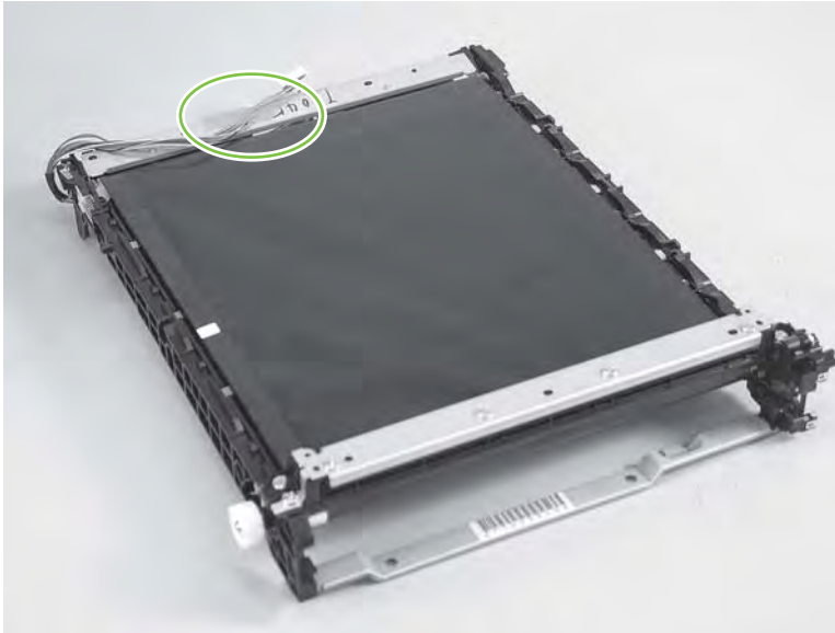
Figure 6-81 Reinstall the ITB (2 of 2)
