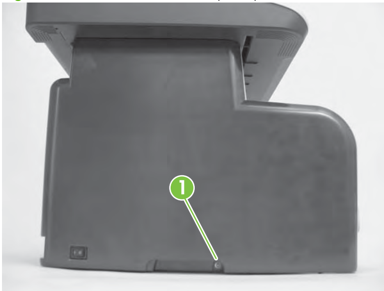
Figure 6-40 Remove the left cover (1 of 4)
