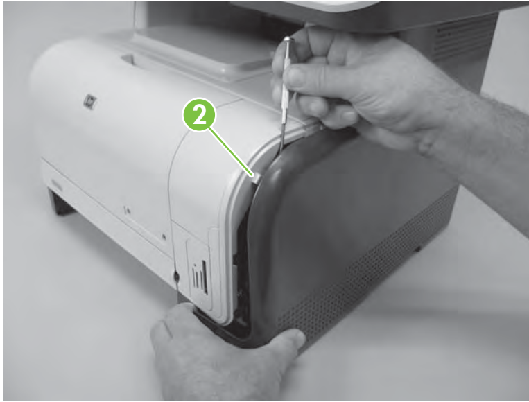
Figure 6-37 Remove the right cover (3 of 5)
