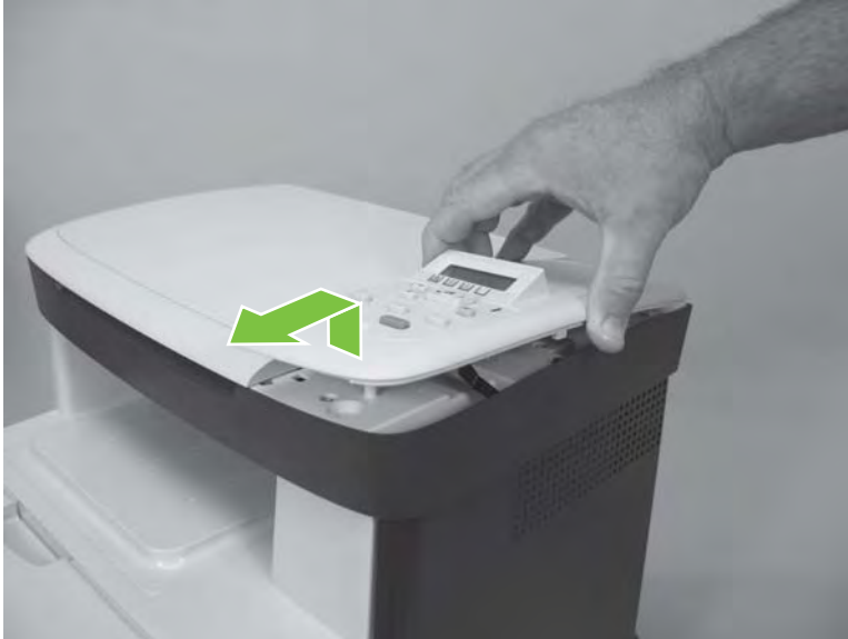
Figure 6-6 Remove the control-panel (2 of 3; base model)
