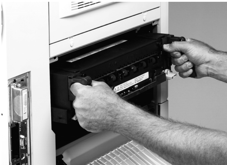
Figure 162. Remove the fuser
