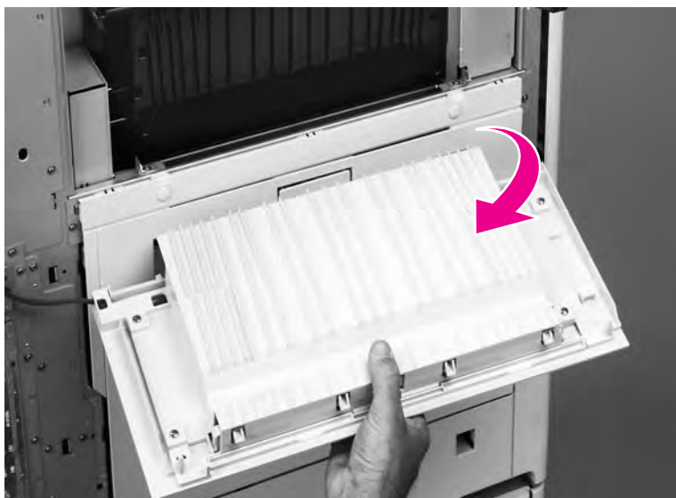
Figure 153. Remove the paper path access door
