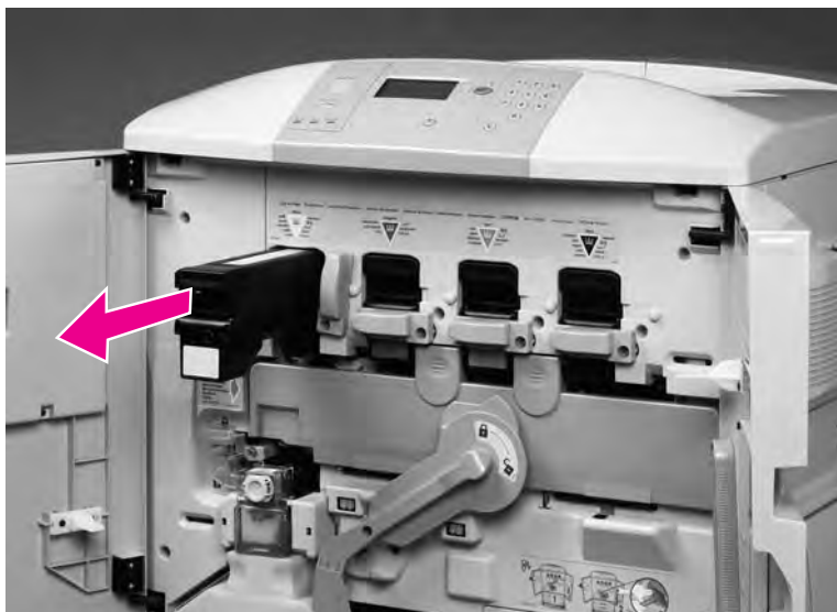
Figure 76. Remove the toner cartridge
