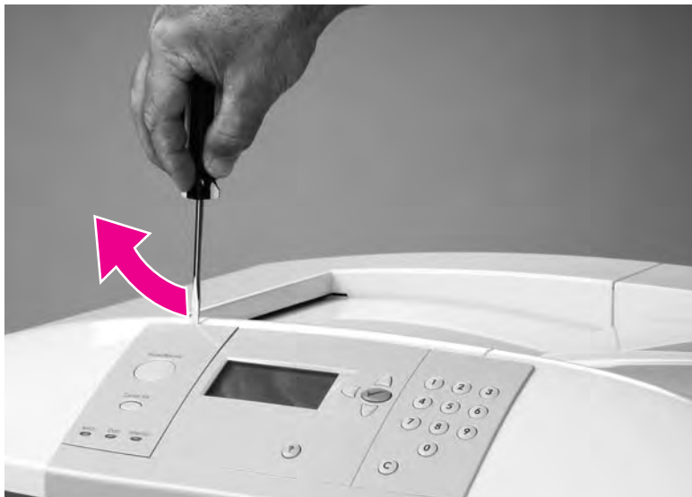
Figure 86. Remove the control panel overlay
