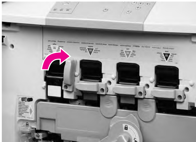
Figure 75. Rotate the toner cartridge lever
