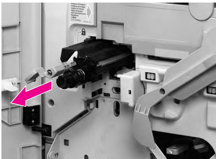
Figure 83. Remove the transfer cleaner
