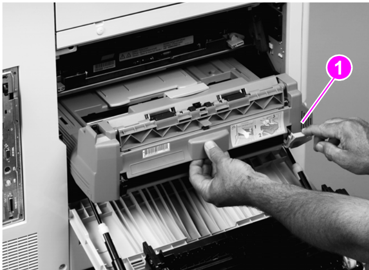
Figure 160. Remove the duplexer
