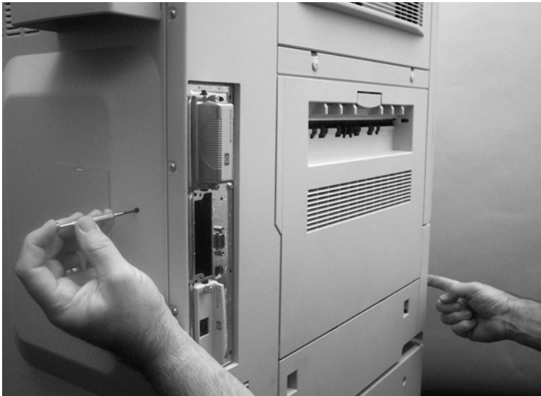
Figure 126. Prepare to print a laser/scanner adjustment page
