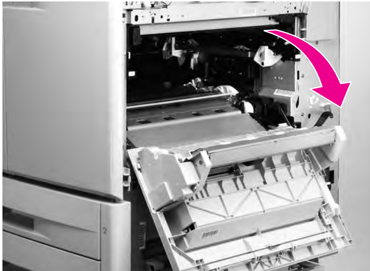
Figure 107. Open the ITB door
