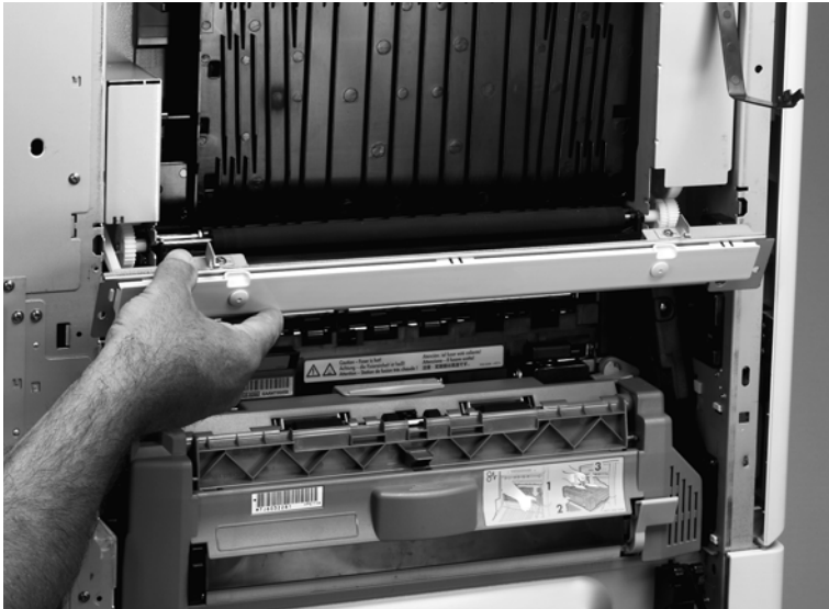
Figure 156. Remove the left side middle cover mounting bracket
