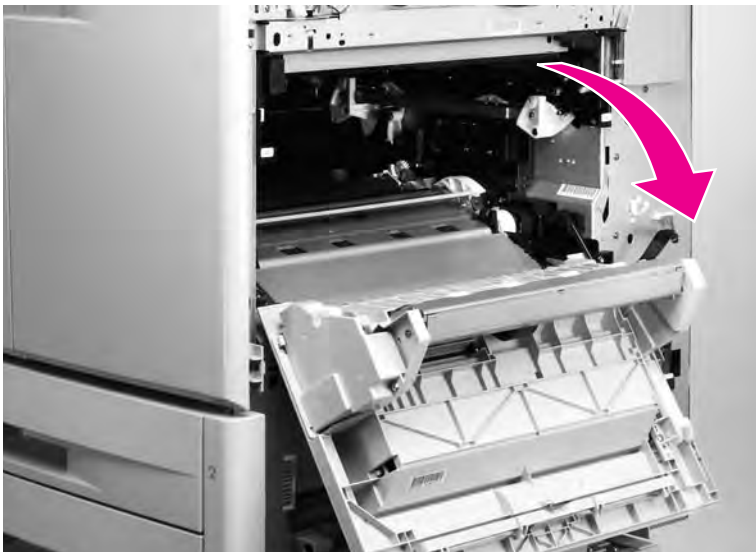
Figure 186. Open the ITB door
