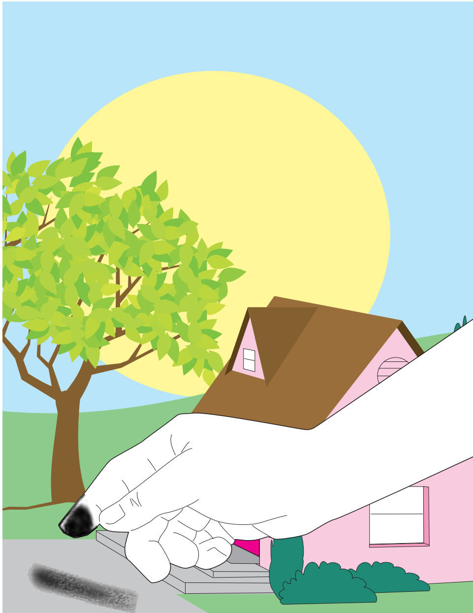
Figure 300. Poorly fused image (2 of 2)
