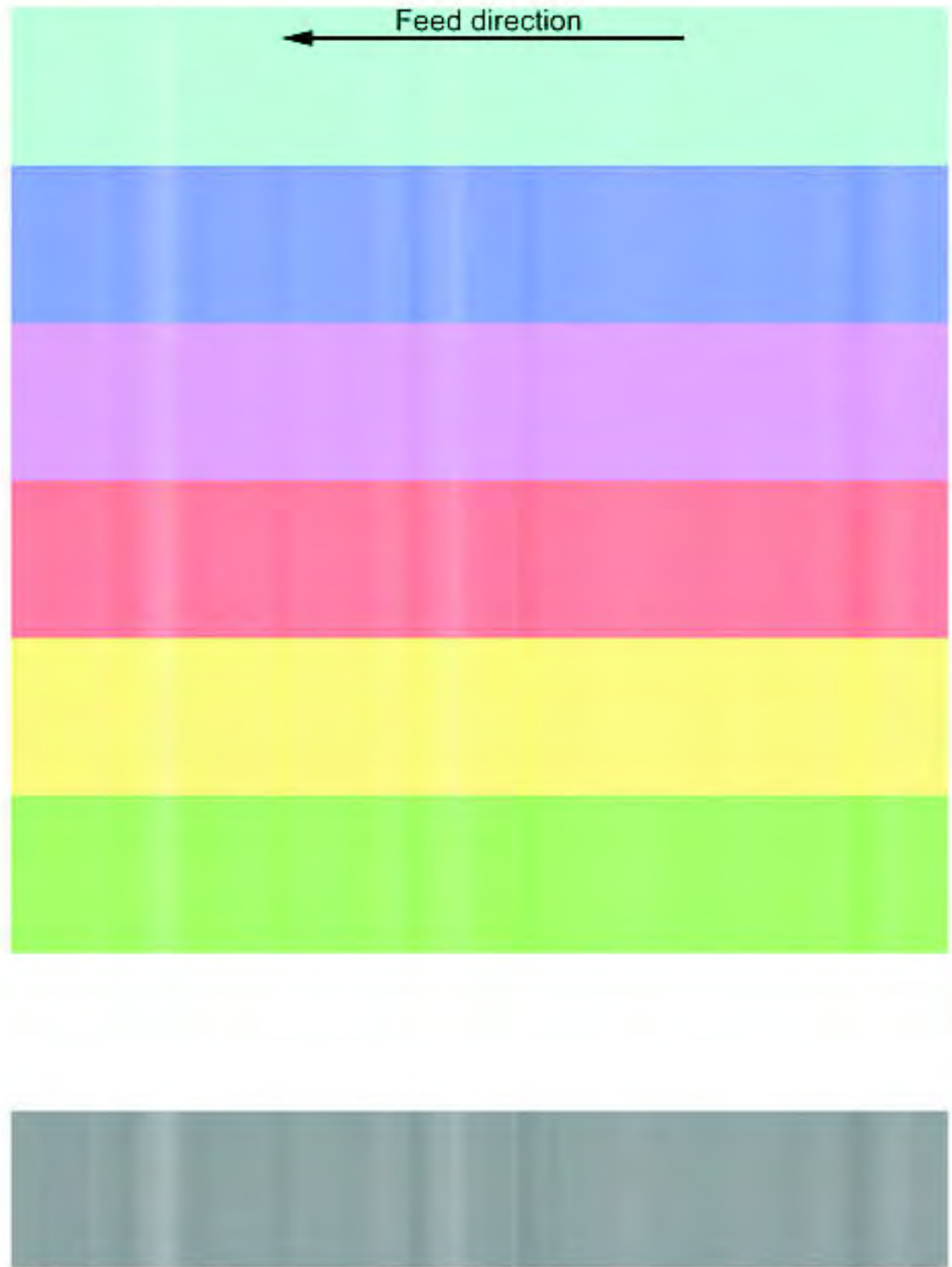
Figure 299. Poorly fused image (1 of 2)
