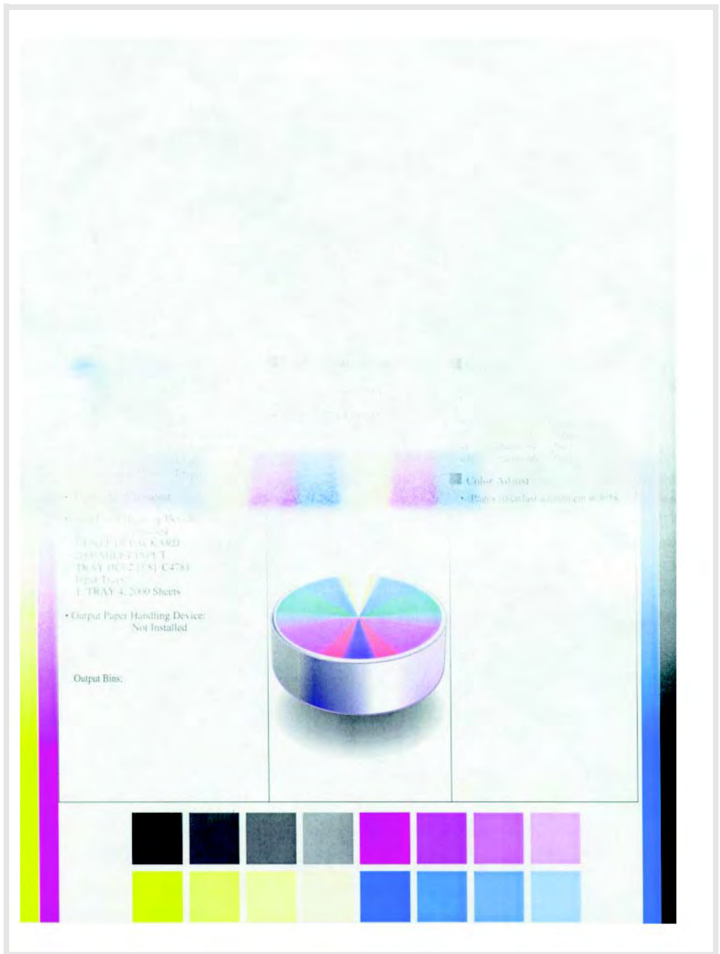
Figure 232. Fading resulting from broken transfer guide
