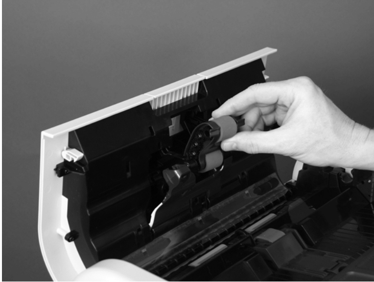
Figure 1-50 Remove the document feeder pickup and feed roller assemblies (3 of 3)
