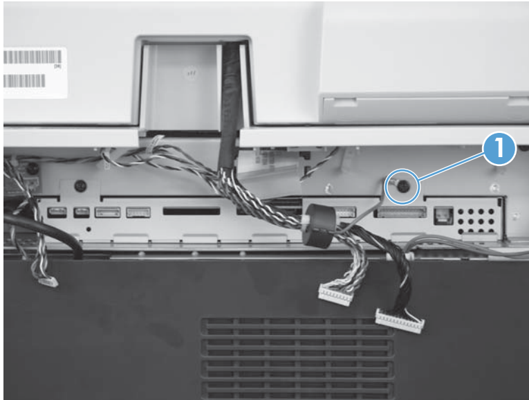
Figure 1-221 Reinstall the SCB
