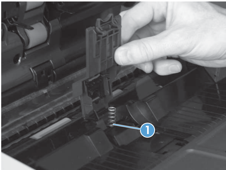
Figure 1-54 Reinstall the document feeder separation pad
