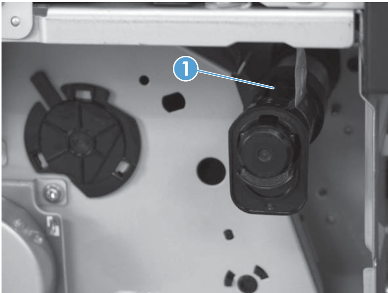
Figure 1-181 Remove the residual toner feed assembly (2 of 6)
