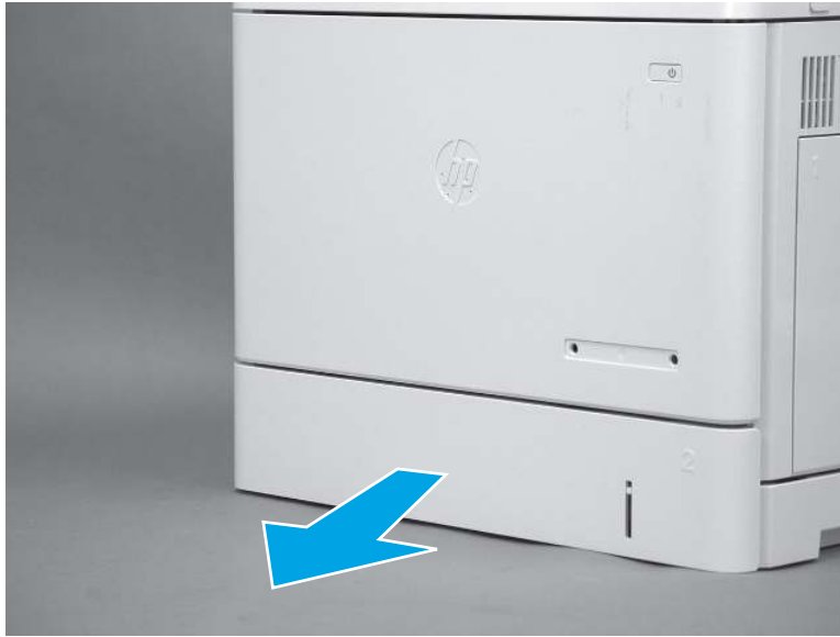
Figure 5-260 Pull the tray out
