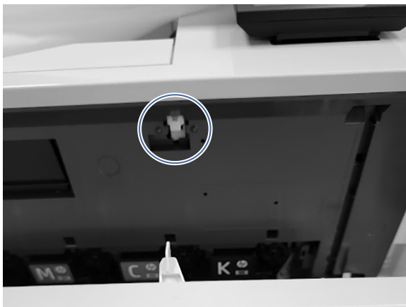
Figure 4-49 Defeat the front door interlock
