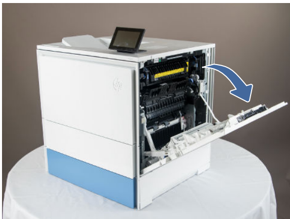
Figure 5-265 Open the right door
