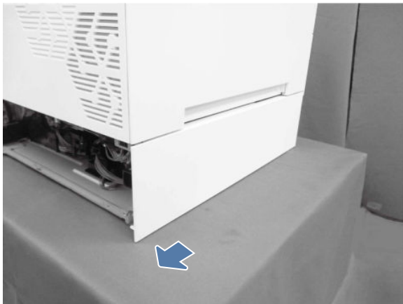
Figure 5-210 Remove the left lower cover
