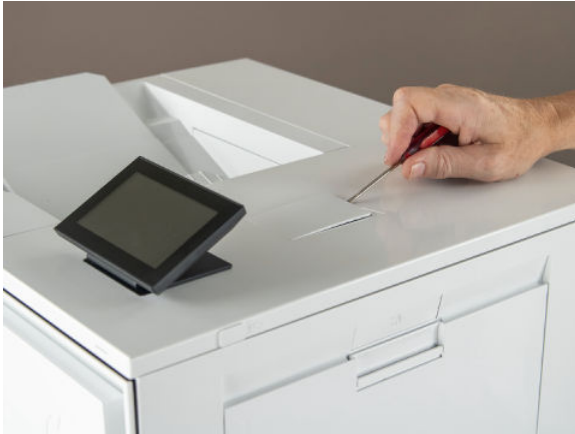
Figure 5-117 Release the cover
