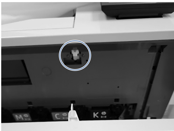
Figure 4-102 Defeat the front door interlock
