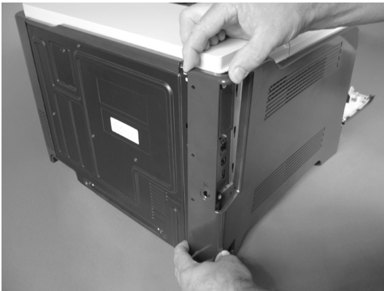
Figure 1-139 Remove the left cover (2 of 5)
