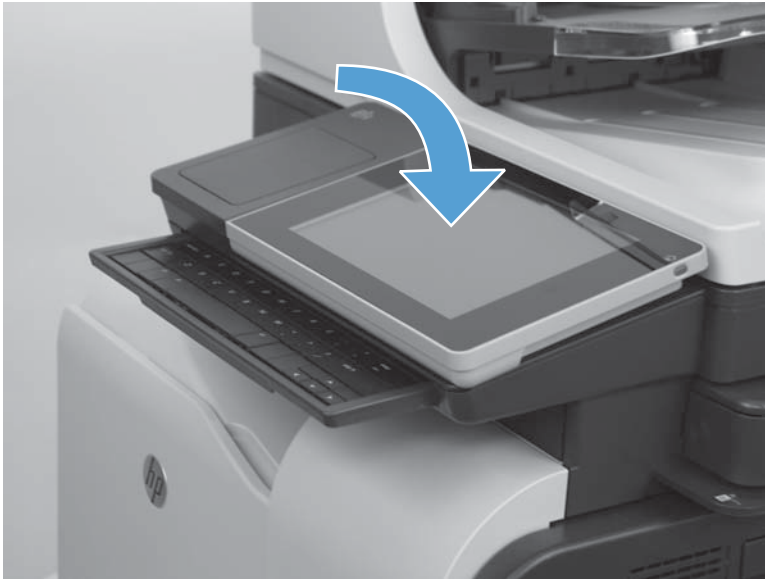
Figure 1-90 Reinstall the control-panel assembly (12 of 13)
