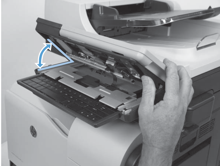
Figure 1-80 Reinstall the control-panel assembly (2 of 13)
