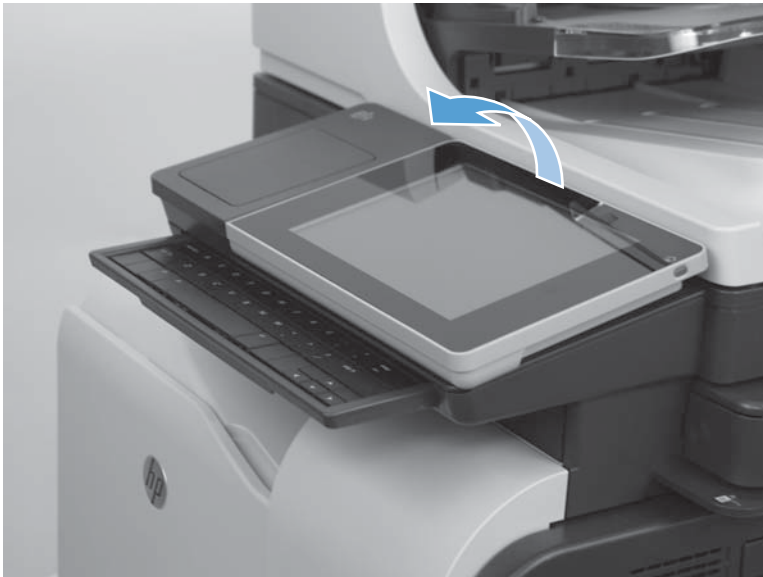
Figure 1-68 Remove the control-panel assembly (3 of 13)
