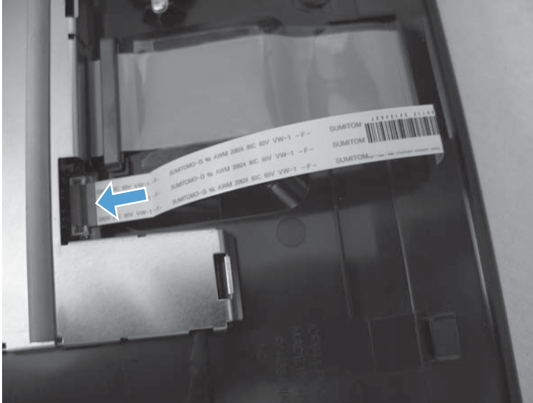
Figure 1-97 Reinstall the control-panel assembly to keyboard FFC (2 of 4)
