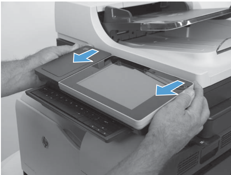
Figure 1-72 Remove the control-panel assembly (7 of 13)
