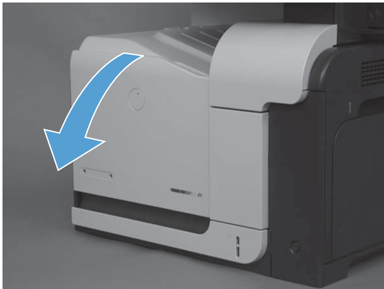
Figure 1-11 Remove the toner-collection unit (1 of 4)
