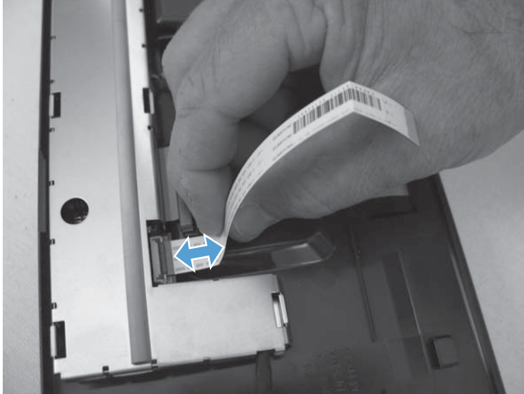
Figure 1-99 Reinstall the control-panel assembly to keyboard FFC (4 of 4)
