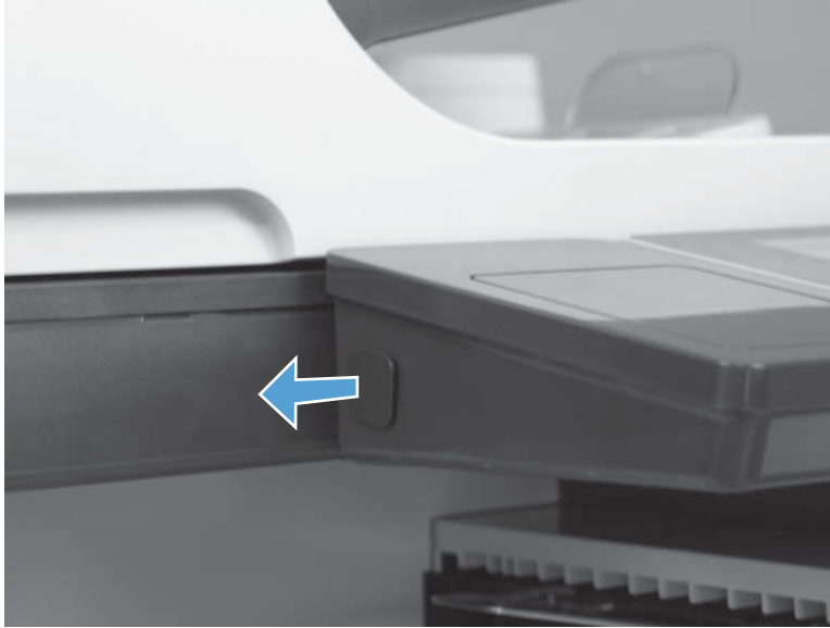
Figure 1-120 Remove USB cover
