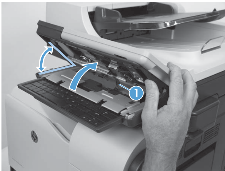
Figure 1-62 Raising the control panel to access the FFC connector (1 of 2)
