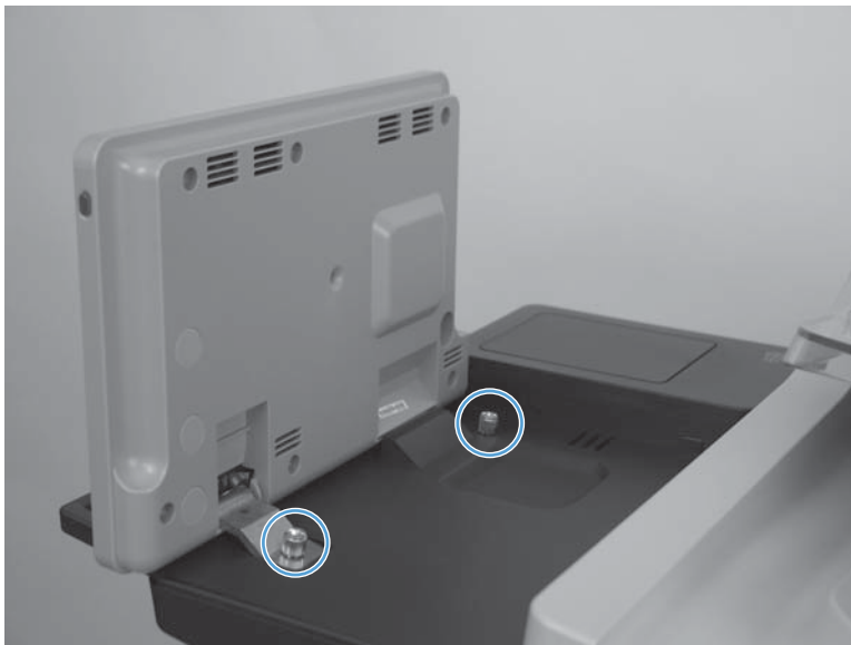
Figure 1-70 Remove the control-panel assembly (5 of 13)
