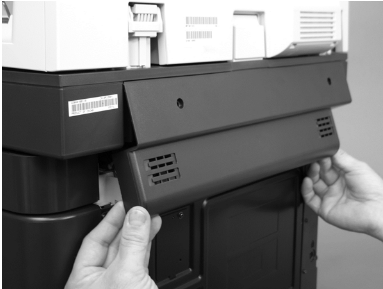
Figure 1-145 Remove the rear-upper cover (3 of 3)
