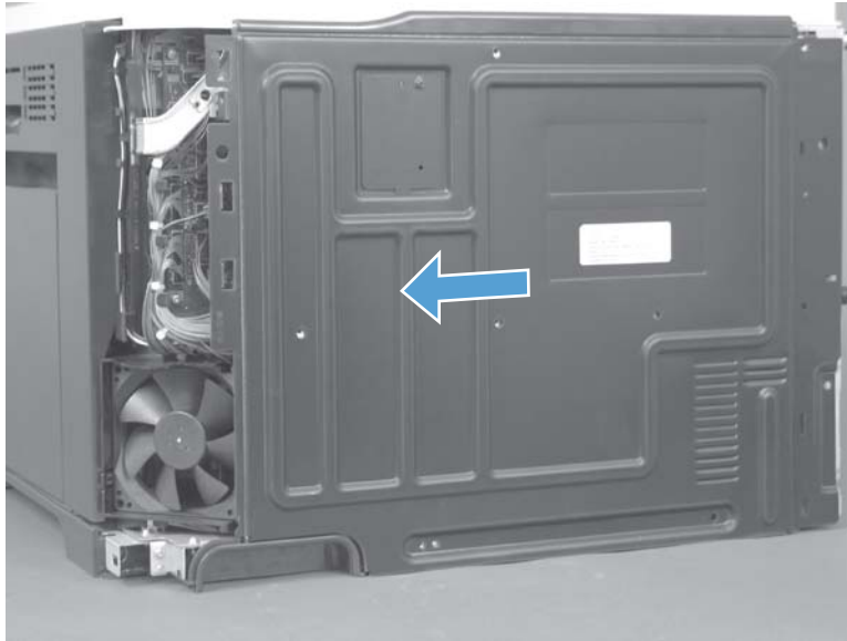
Figure 1-148 Remove the rear cover (2 of 2)
