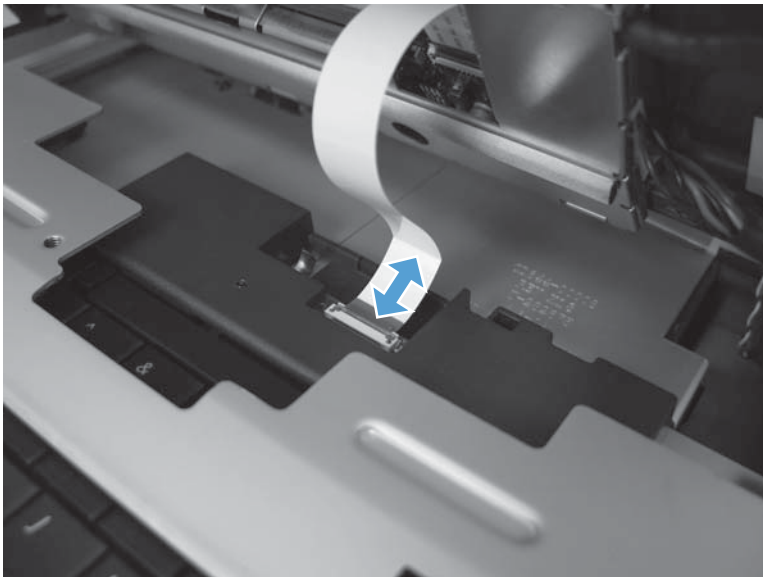
Figure 1-83 Reinstall the control-panel assembly (5 of 13)
