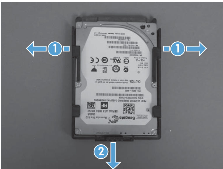
Figure 1-20 Remove the HDD (3 of 3)
