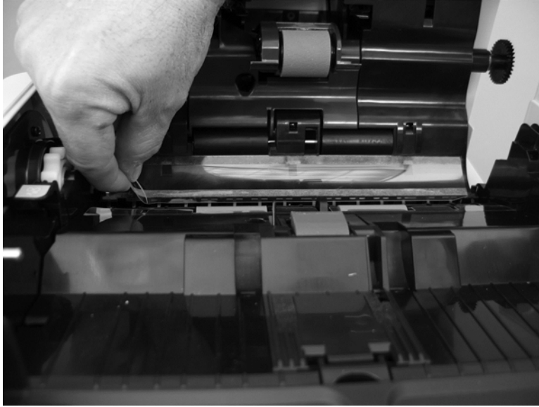
Figure 1-176 Remove the deskew mylar and separation mylar (3 of 3)
