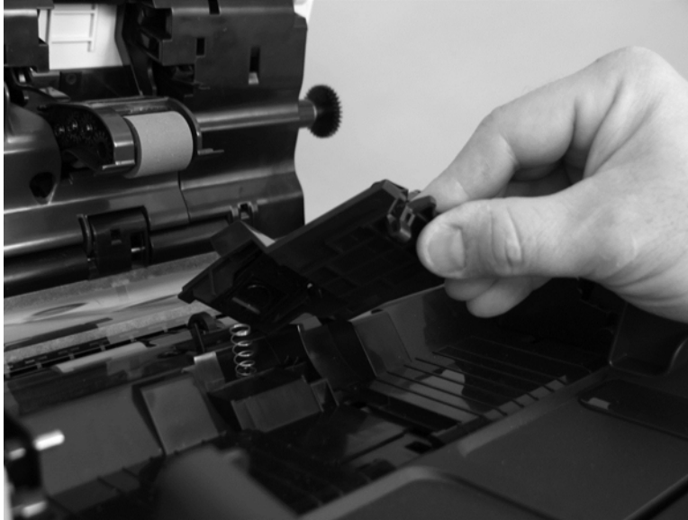
Figure 1-55 Remove the document feeder separation pad and separation pad spring (5 of 5)
