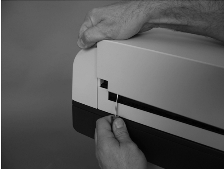
Figure 1-183 Remove the document feeder jam-access cover (5 of 5)
