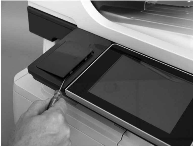
Figure 1-121 Remove the HIP cover
