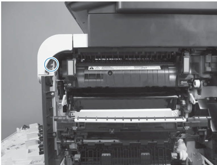
Figure 1-123 Remove the front-upper cover (2 of 4)
