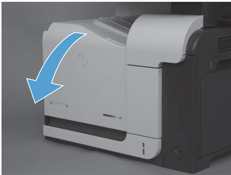
Figure 1-43 Remove the front-door assembly (1 of 2)
