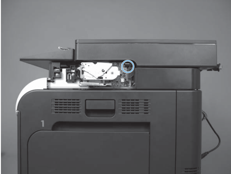
Figure 1-201 Remove the scanner assembly (2 of 5)
