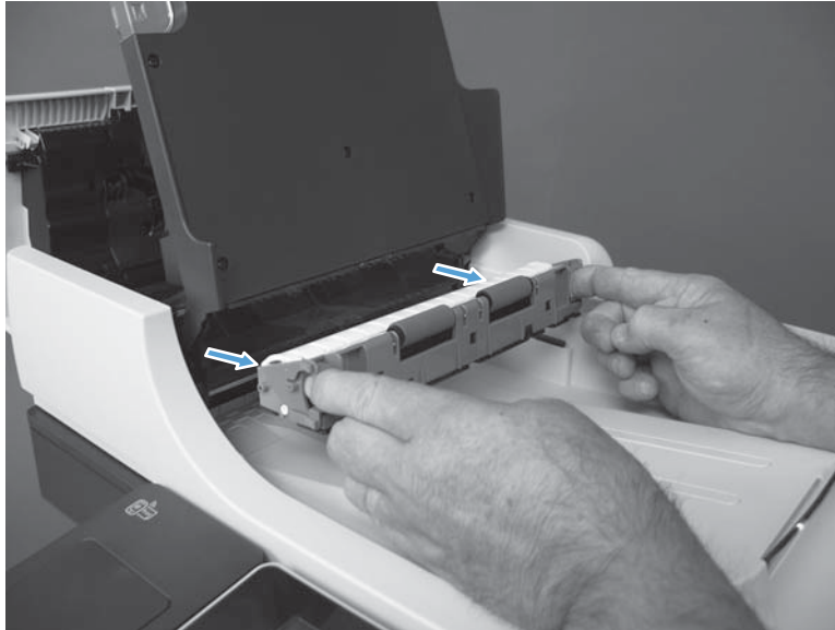
Figure 1-115 Remove the back-side background selector assembly (3 of 3)
