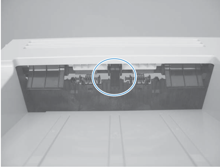
Figure 2-16 Test the output bin full sensor
