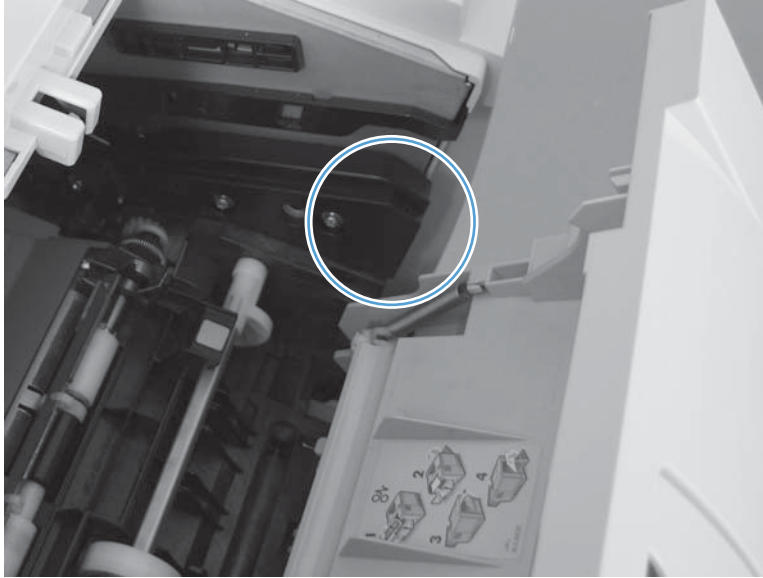
Figure 2-2 Test the cartridge door switch
