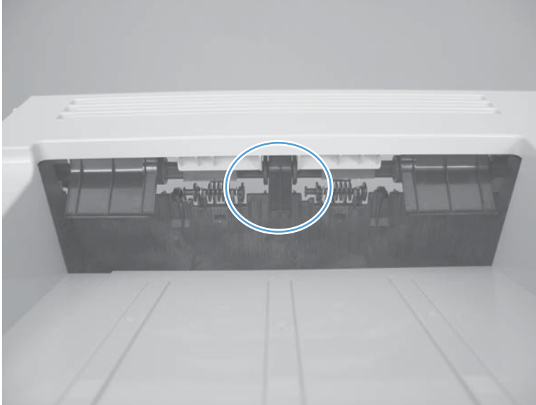
Figure 2-10 Test the output bin full sensor
