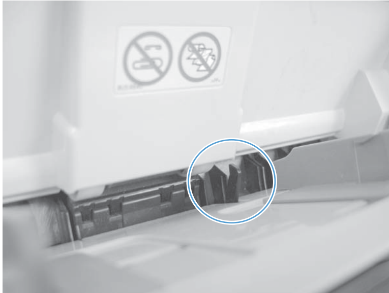
Figure 2-13 Test the Tray 1 paper sensor
