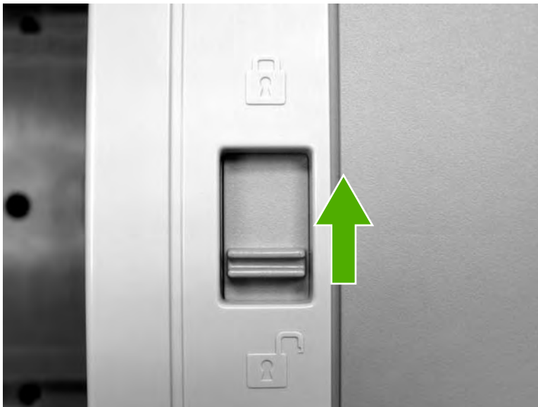
Figure 6-282 Remove the scanner right cover (1 of 2)
