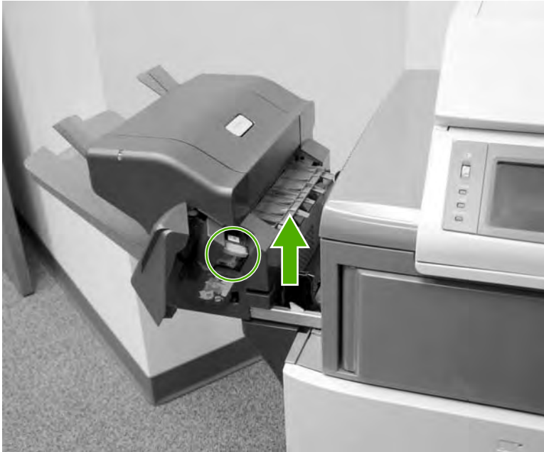
Figure 6-17 Replace the staple cartridge (2 of 3)
