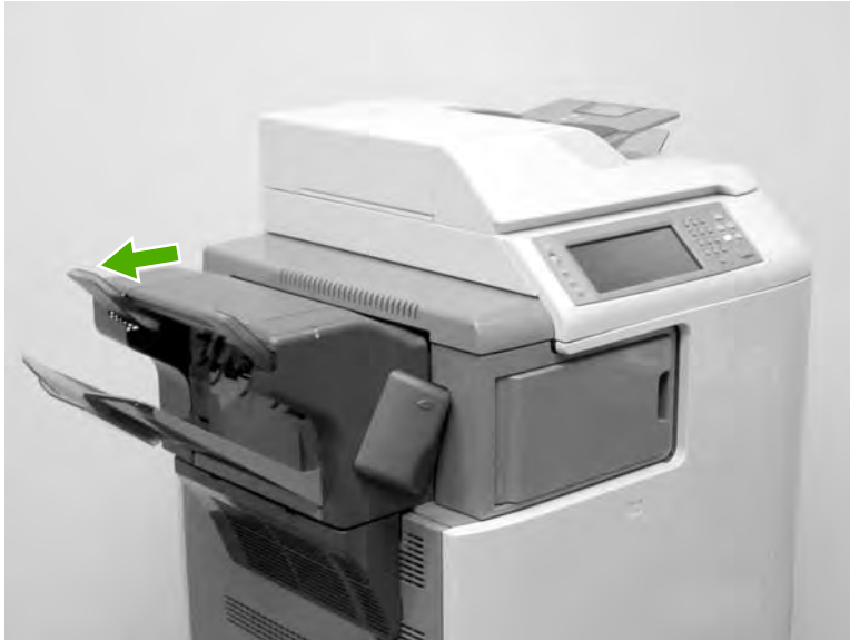
Figure 6-11 Remove the stapler/stacker (1 of 5)
