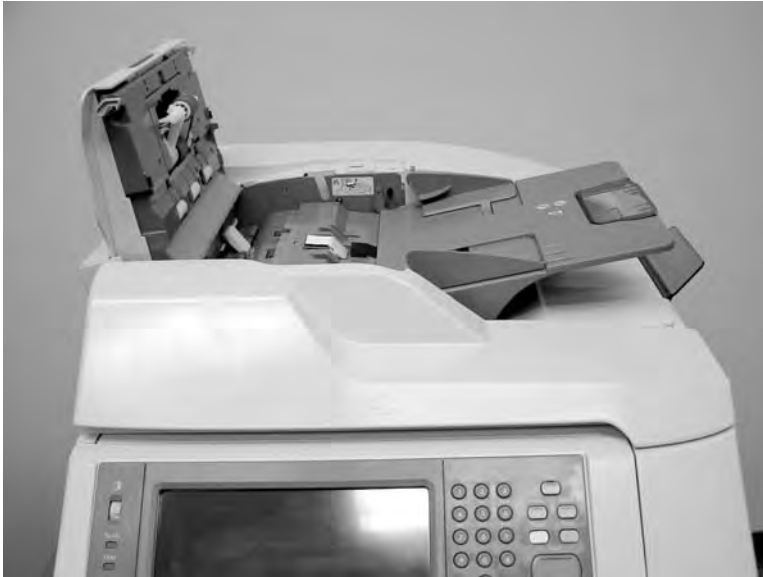
Figure 6-31 Remove the ADF pickup and feed rollers (1 of 3)
