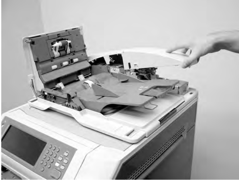
Figure 6-315 Remove the ADF rear cover (3 of 3)
