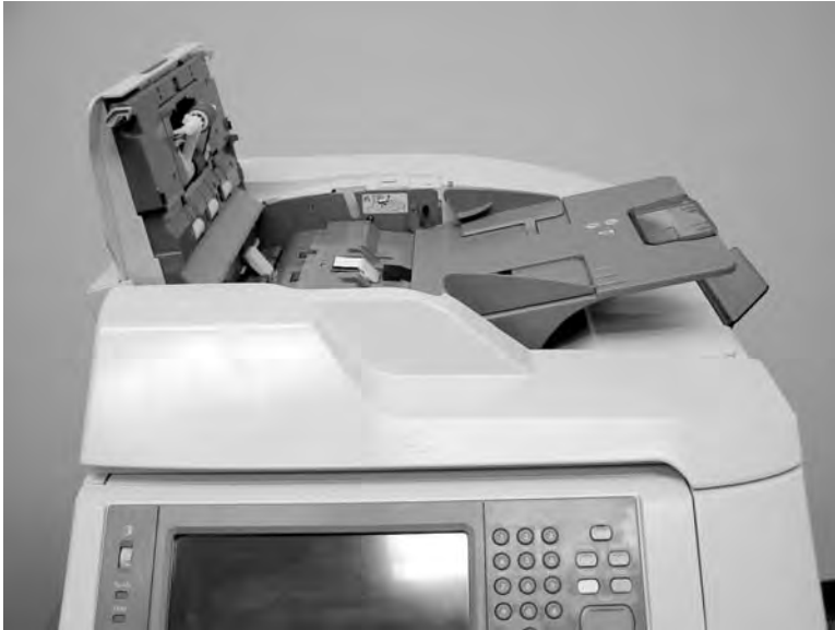
Figure 6-28 Remove the ADF input tray (1 of 3)
