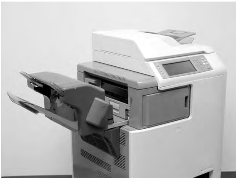
Figure 6-12 Remove the stapler/stacker (2 of 5)
