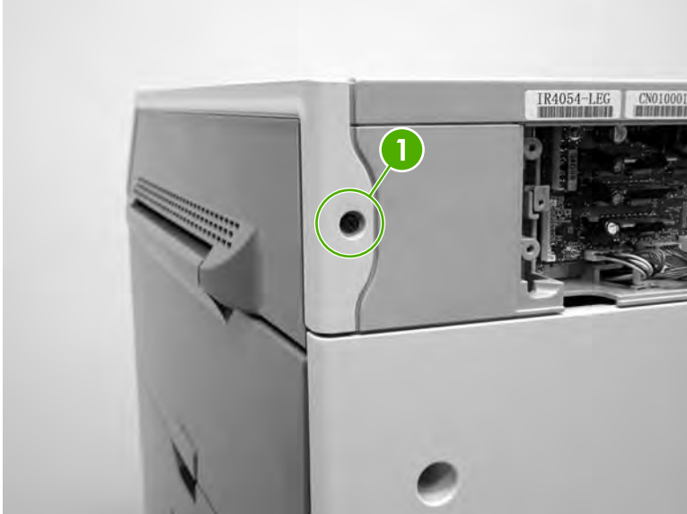
Figure 6-275 Remove the scanner assembly (1 of 5)
