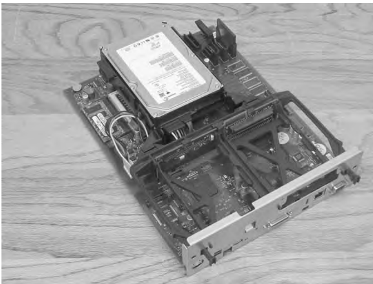
Figure 6-61 Remove the formatter (2 of 2)
