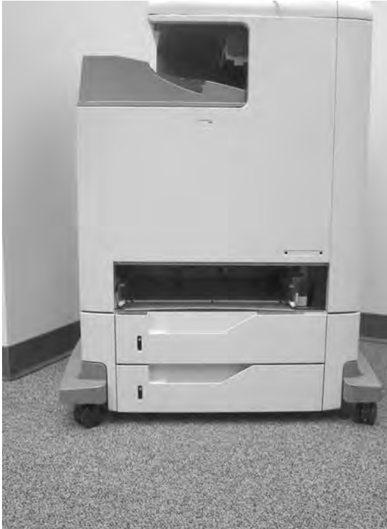
Figure 6-45 Remove the tray 2, 3, or 4 pickup and feed rollers (1 of 2)
