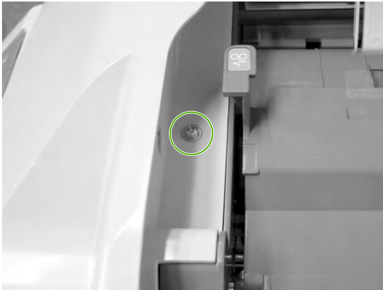
Figure 6-311 Remove the ADF front cover (1 of 2)
