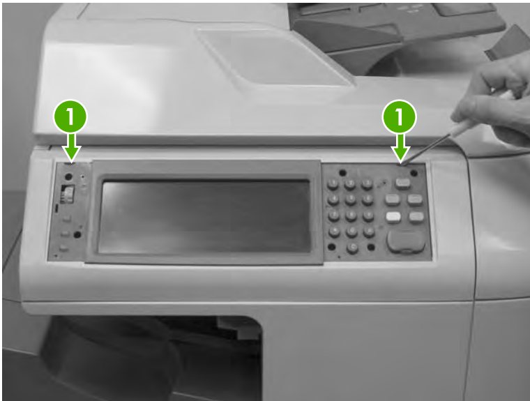
Figure 6-6 Remove the control panel (1 of 2)
