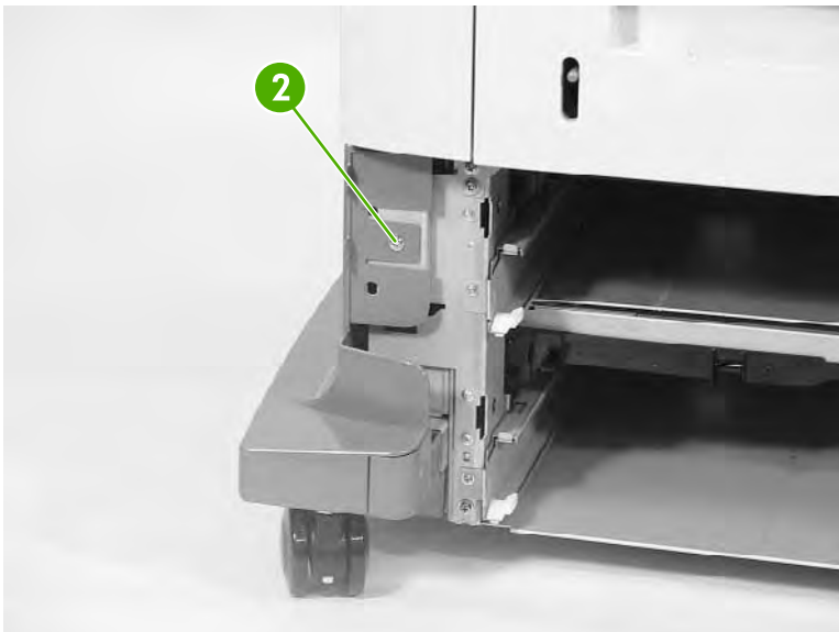
Figure 6-335 Remove the left cover (2 of 3)
