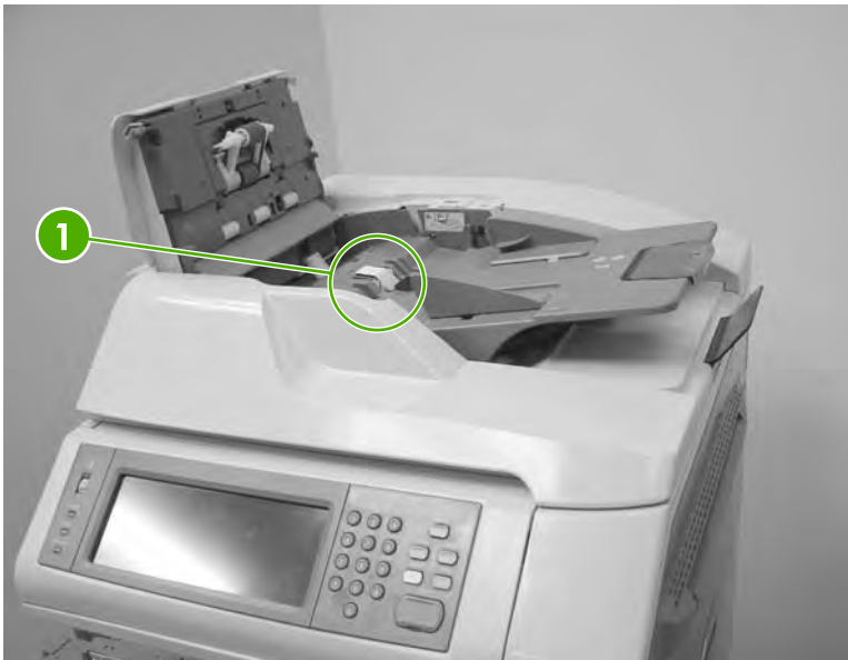
Figure 6-35 Remove the ADF separation pad (2 of 4)
