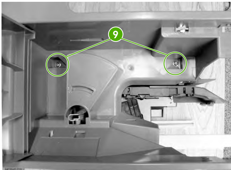
Figure 6-370 Remove the IPTU front cover and front door (5 of 6)
