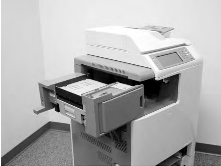
Figure 6-9 Remove the IPTU (2 of 3)
