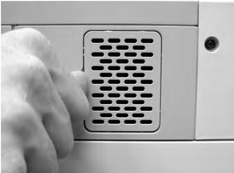
Figure 6-57 Remove the scanner filter (1 of 2)
