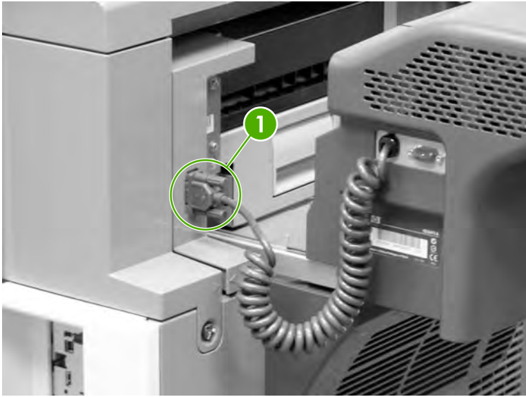
Figure 6-13 Remove the stapler/stacker (3 of 5)
