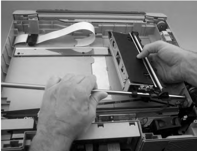
Figure 6-289 Remove the optical assembly (5 of 10)
