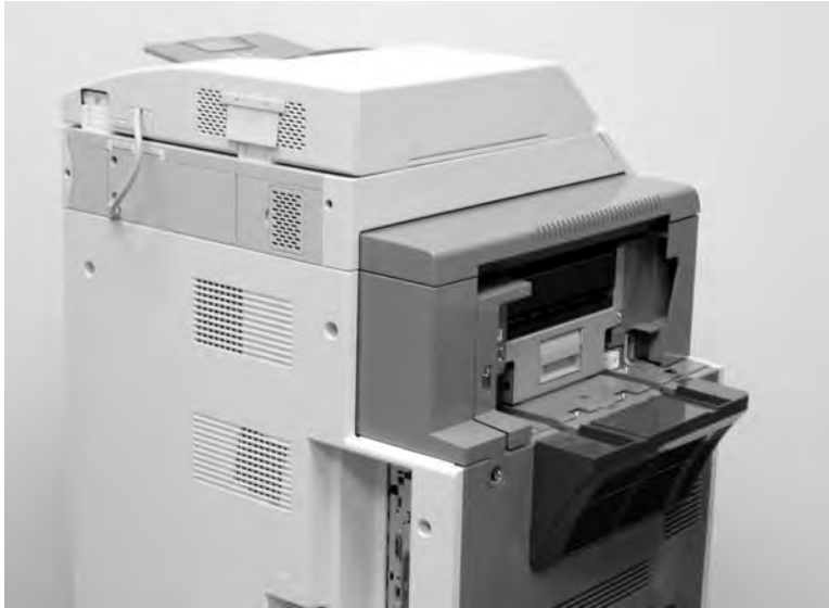
Figure 6-15 Remove the stapler/stacker (5 of 5)
