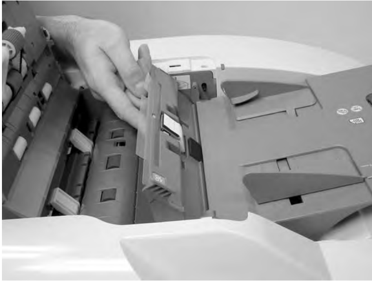
Figure 6-36 Remove the ADF separation pad (3 of 4)
