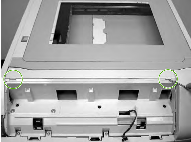
Figure 6-273 Remove the top covers (1 of 2)
