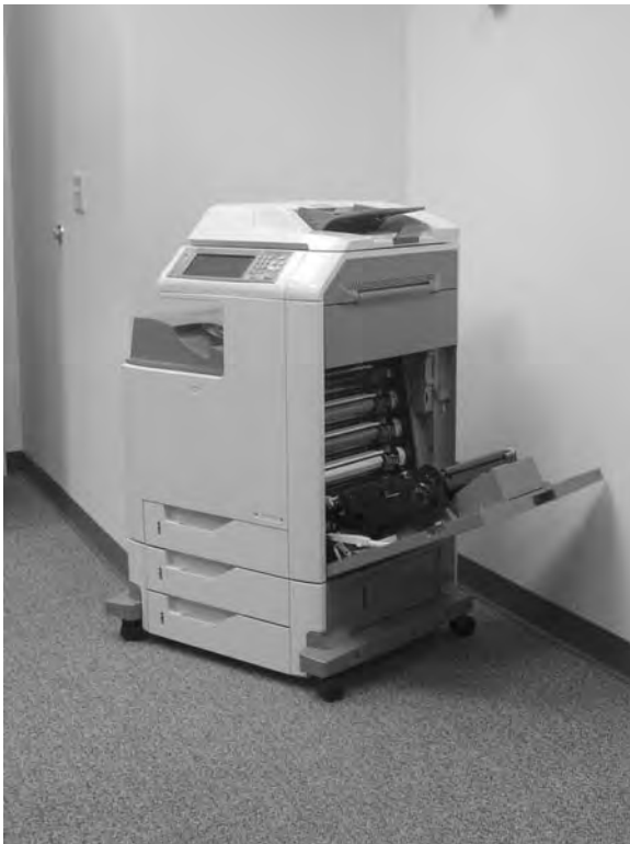
Figure 6-22 Remove the ETB assembly (1 of 4)
