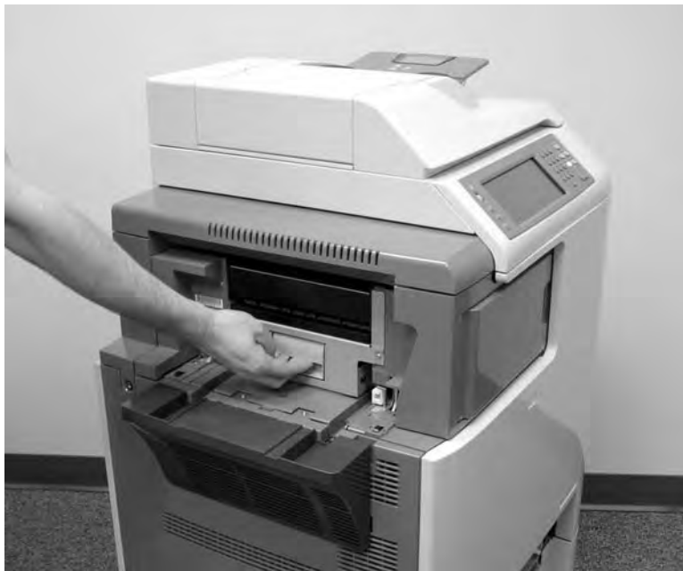
Figure 6-8 Remove the IPTU (1 of 3)
