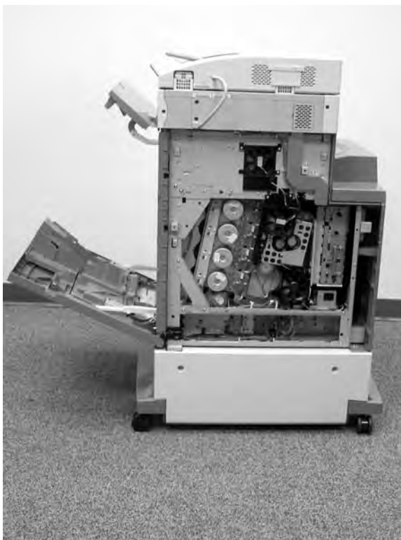
Figure 6-82 Remove the rear cover assembly (4 of 4)
