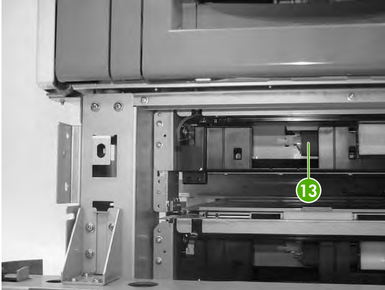
Figure 6-354 Remove the upper pickup assembly (8 of 9)
