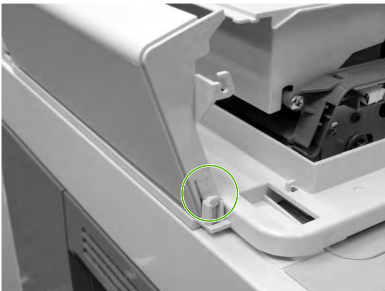
Figure 6-317 Remove the ADF left cover (2 of 2)
