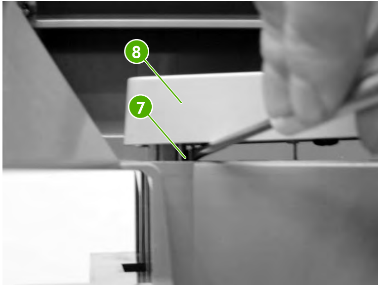
Figure 6-369 Remove the IPTU front cover and front door (4 of 6)
