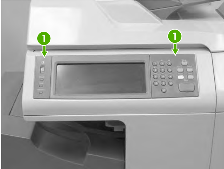
Figure 6-5 Remove the control panel overlays
