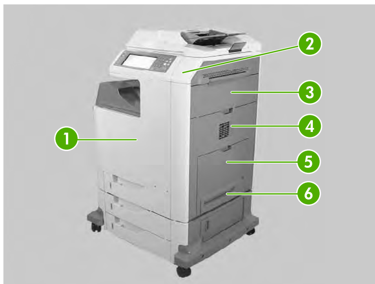
Figure 6-75 Cover, door, and panel locations (1 of 2)
