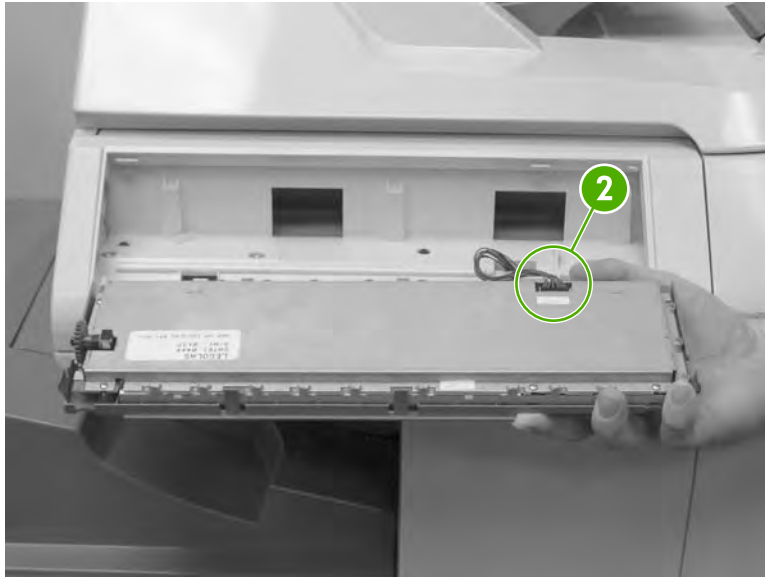
Figure 6-7 Remove the control panel (2 of 2)
