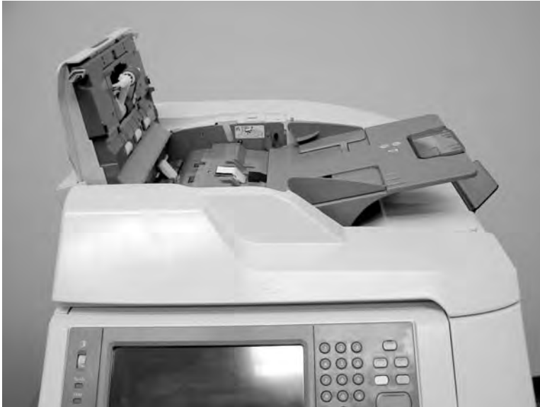
Figure 6-313 Remove the ADF rear cover (1 of 3)
