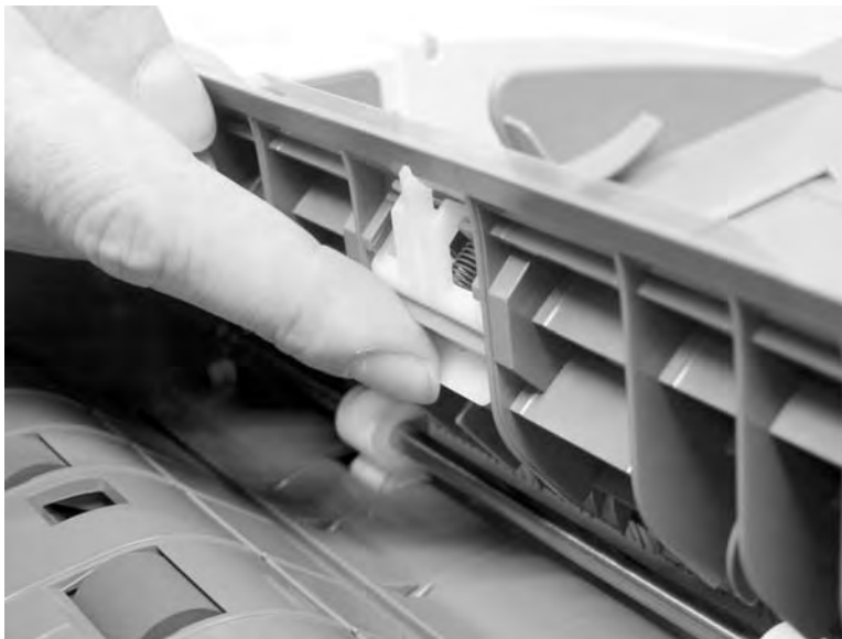
Figure 6-37 Remove the ADF separation pad (4 of 4)
