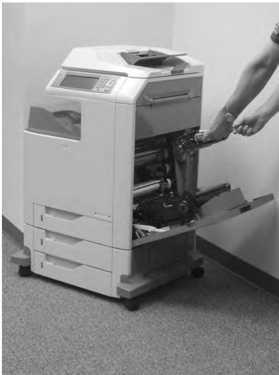
Figure 6-4 Remove the print cartridges (3 of 3)
