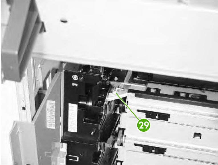
Figure 6-190 Remove the delivery assembly (13 of 15)
