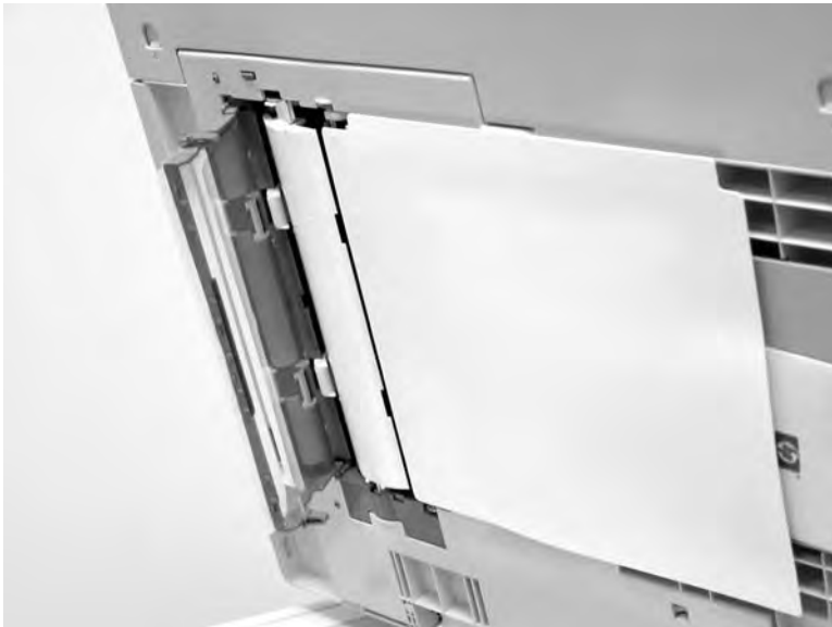
Figure 6-307 Remove the ADF white mylar backing (2 of 3)
