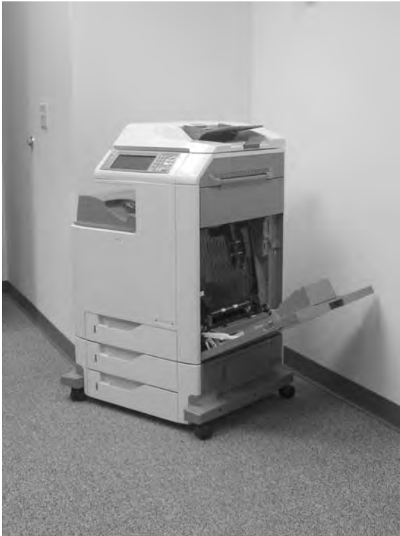
Figure 6-2 Remove the print cartridges (1 of 3)
