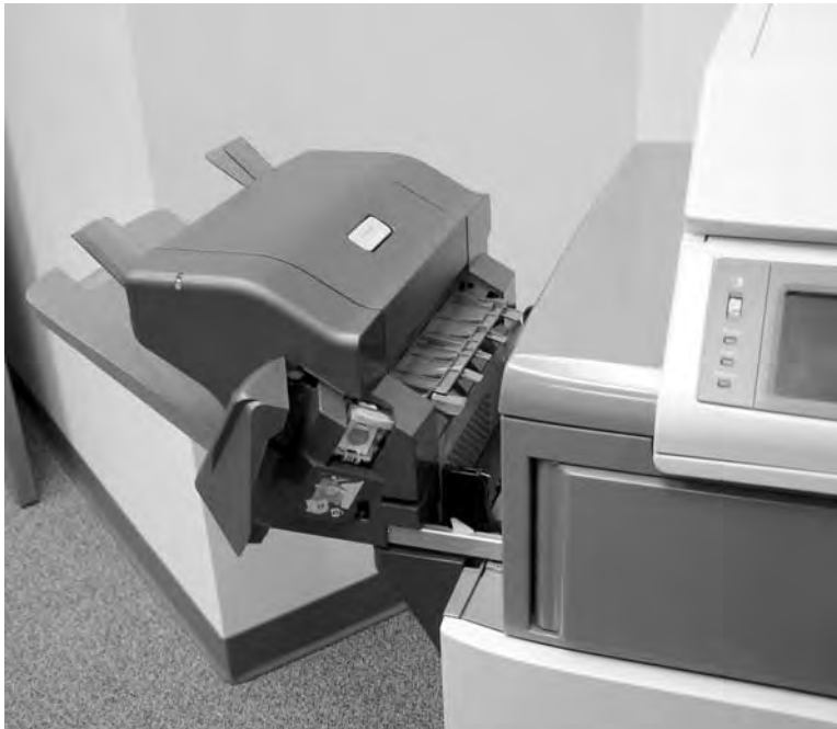
Figure 6-16 Replace the staple cartridge (1 of 3)
