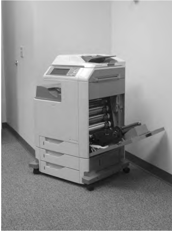
Figure 6-3 Remove the print cartridges (2 of 3)
