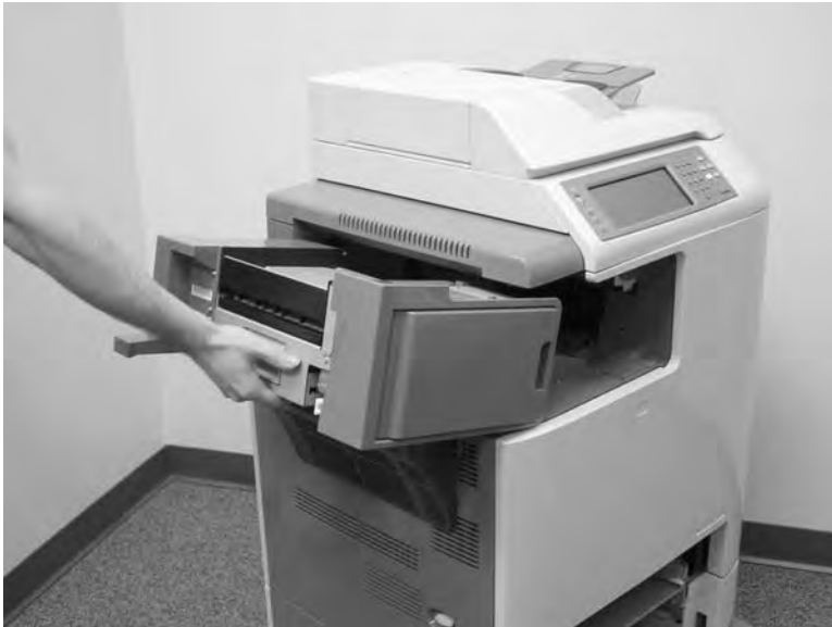
Figure 6-10 Remove the IPTU (3 of 3)
