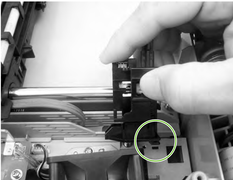
Figure 6-301 Reinstalling the scanner home position sensor
