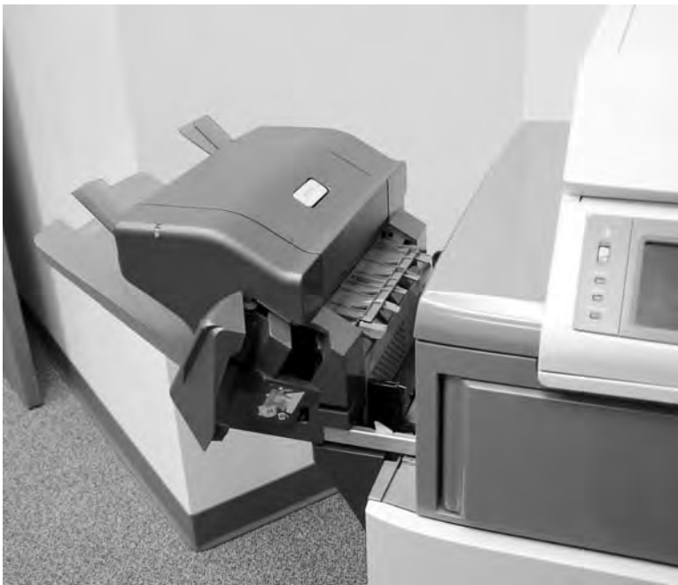
Figure 6-18 Replace the staple cartridge (3 of 3)
