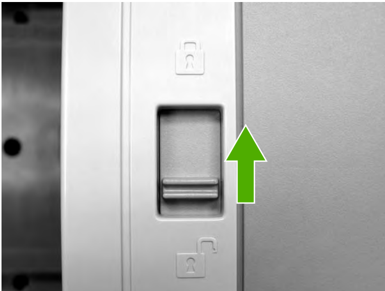
Figure 6-280 Remove the scanner left cover (1 of 2)
