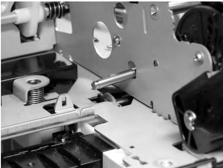
Figure 6-207 Remove the pickup motor assembly (2 of 3)
