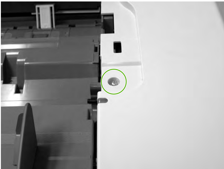
Figure 6-314 Remove the ADF rear cover (2 of 3)
