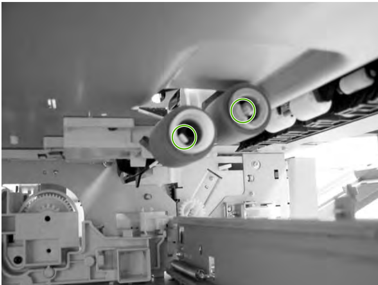
Figure 6-46 Remove the tray 2, 3, or 4 pickup and feed rollers (2 of 2)
