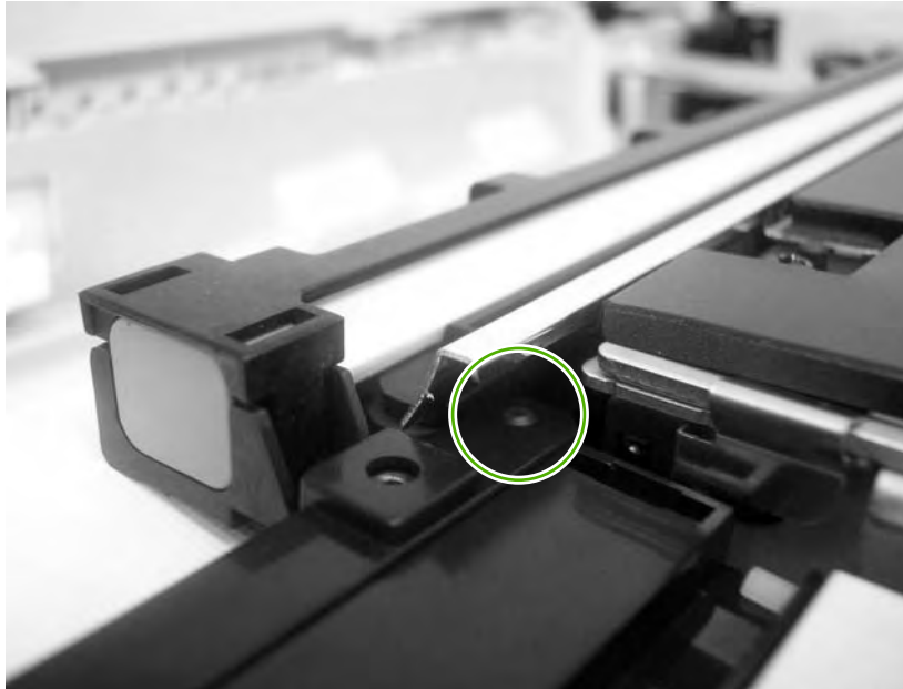
Figure 6-291 Remove the optical assembly (7 of 10)
