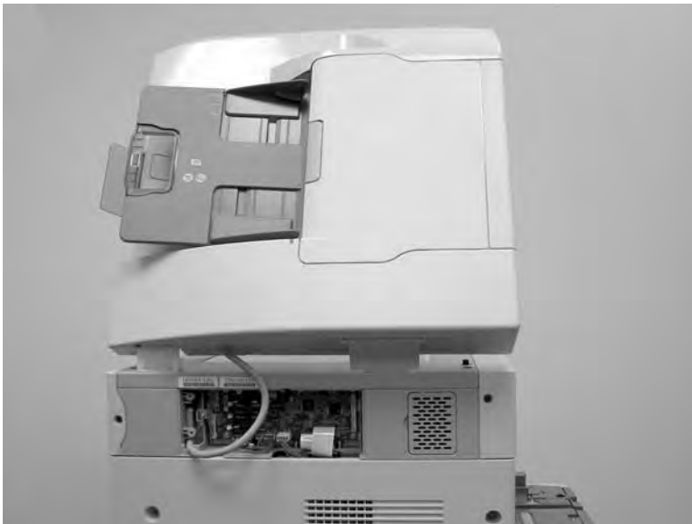
Figure 6-272 Remove the ADF assembly (3 of 3)
