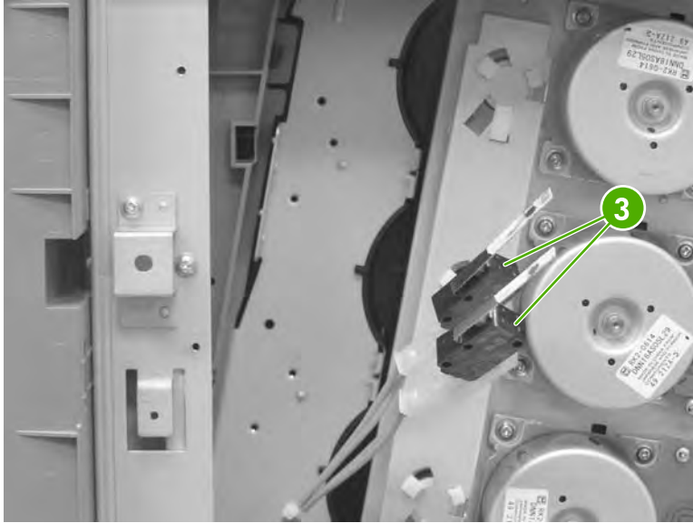
Figure 6-268 Remove the door-open switch assembly (3 of 3)
