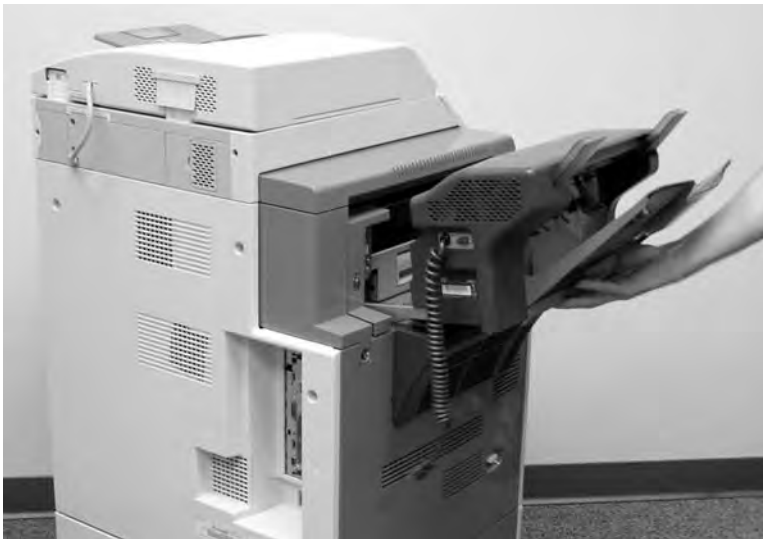
Figure 6-14 Remove the stapler/stacker (4 of 5)
