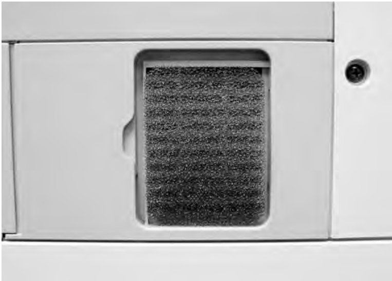
Figure 6-58 Remove the scanner filter (2 of 2)
