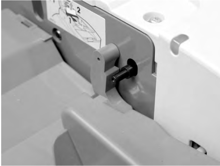
Figure 6-30 Remove the ADF input tray (3 of 3)
