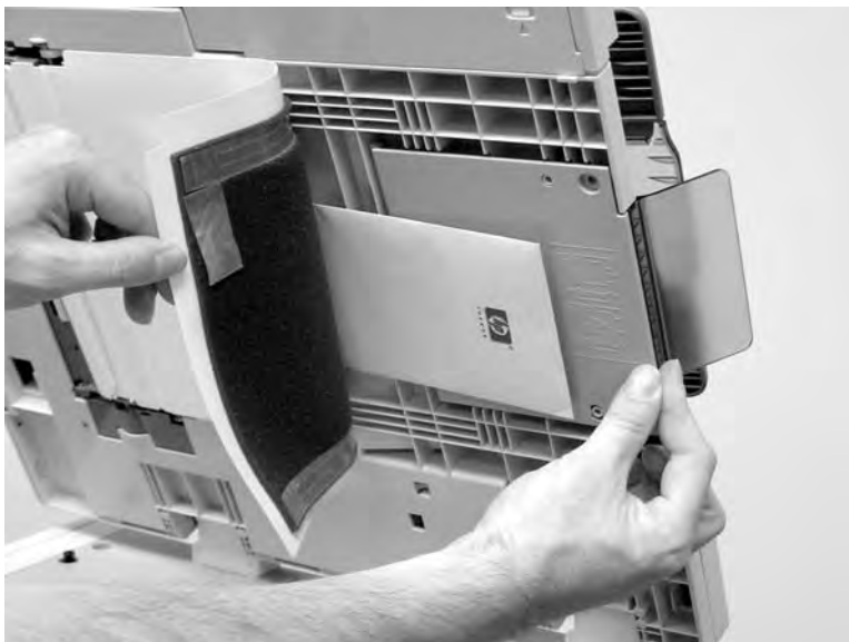
Figure 6-305 Remove the ADF output bin extension (2 of 2)
