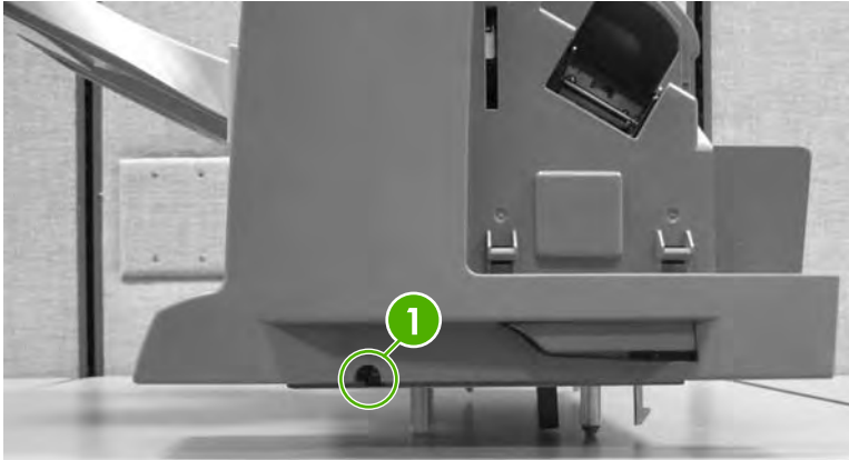
Figure 6-185 Remove the left cover (1 of 2)
