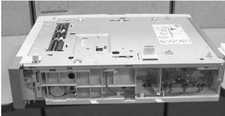
Figure 6-162 Remove the right cover (2 of 2)
