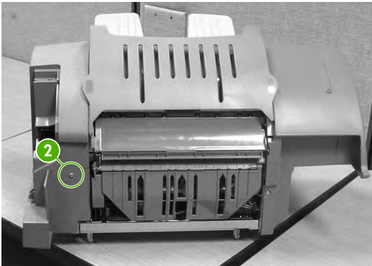
Figure 6-186 Remove the left cover (2 of 2)
