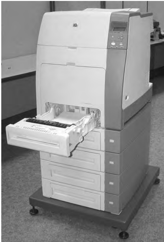
Figure 6-16 Remove the paper tray
