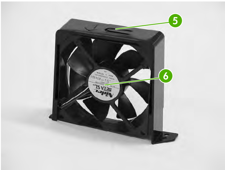
Figure 6-132 Remove the upper exhaust fan (2 of 3)
