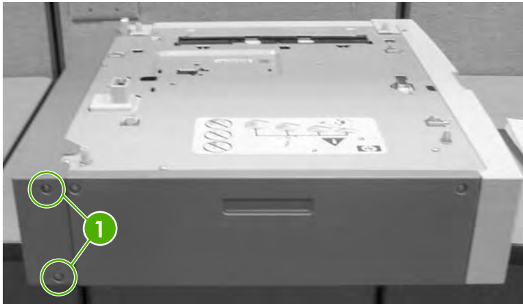
Figure 6-161 Remove the right cover (1 of 2)
