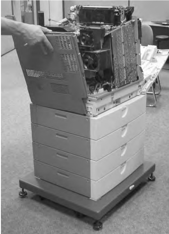
Figure 6-48 Remove the rear cover
