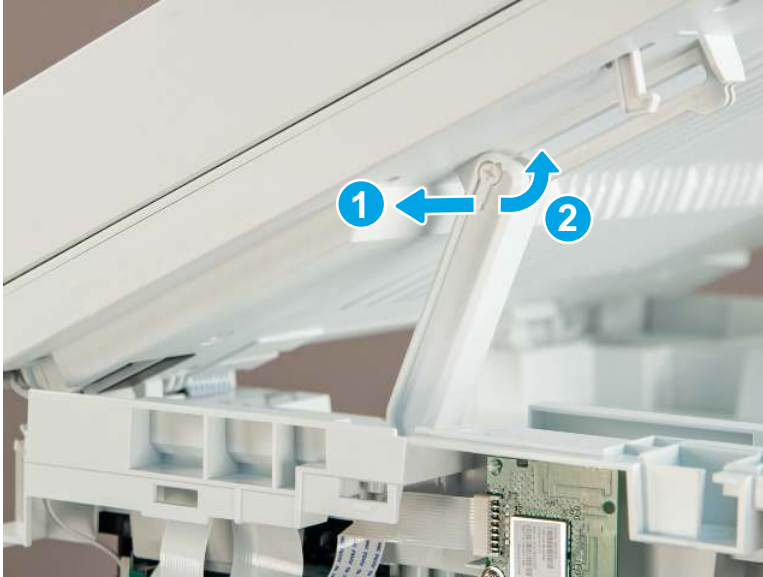
Figure 5-373 Remove the slider pin
