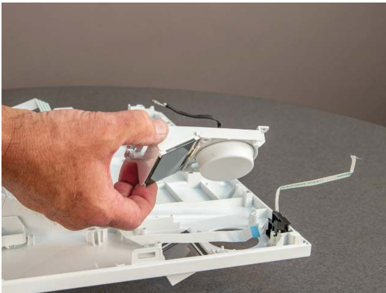
Figure 5-30 Remove the control panel
