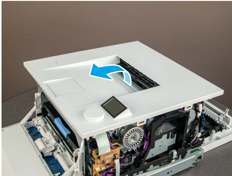
Figure 5-129 Remove the cover
