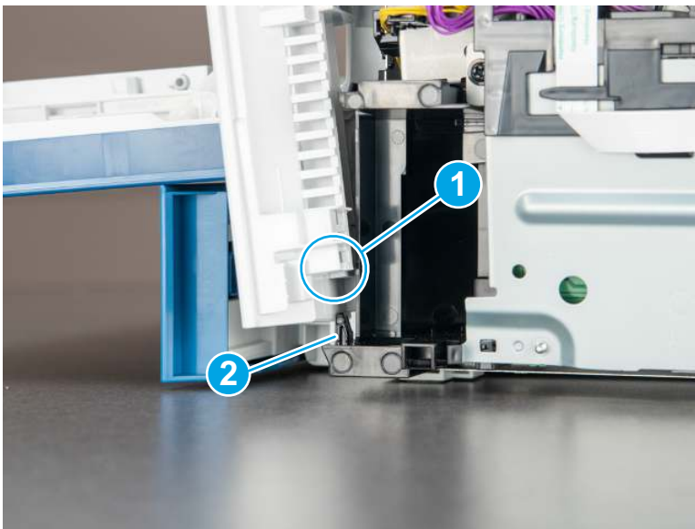
Figure 5-537 Cover alignment pins
