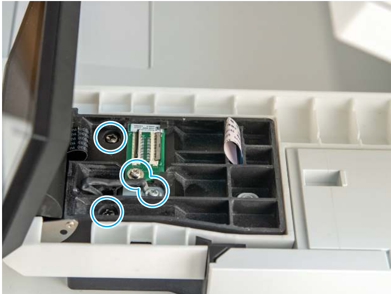
Figure 5-41 Remove four screws
