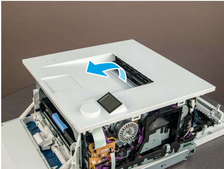
Figure 5-28 Remove the cover
