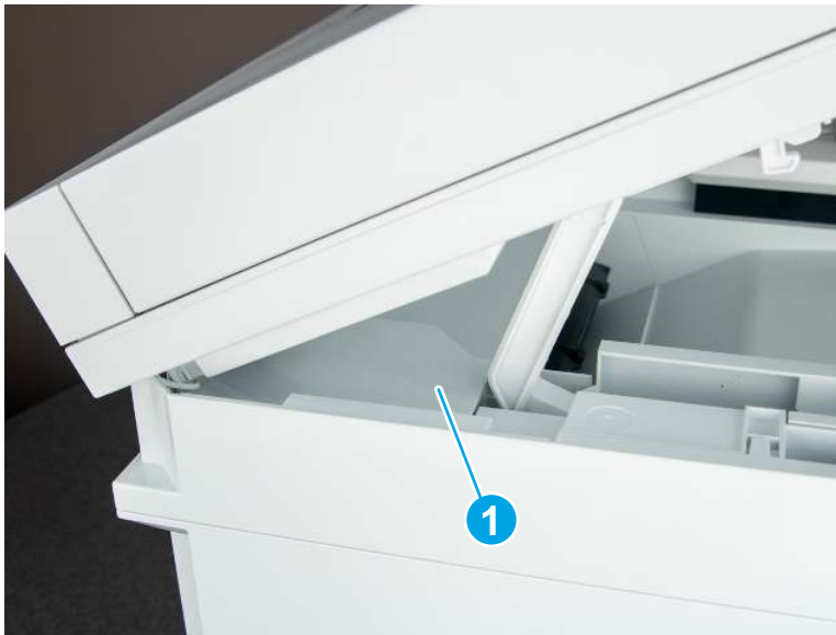
Figure 5-64 Remove the cover
