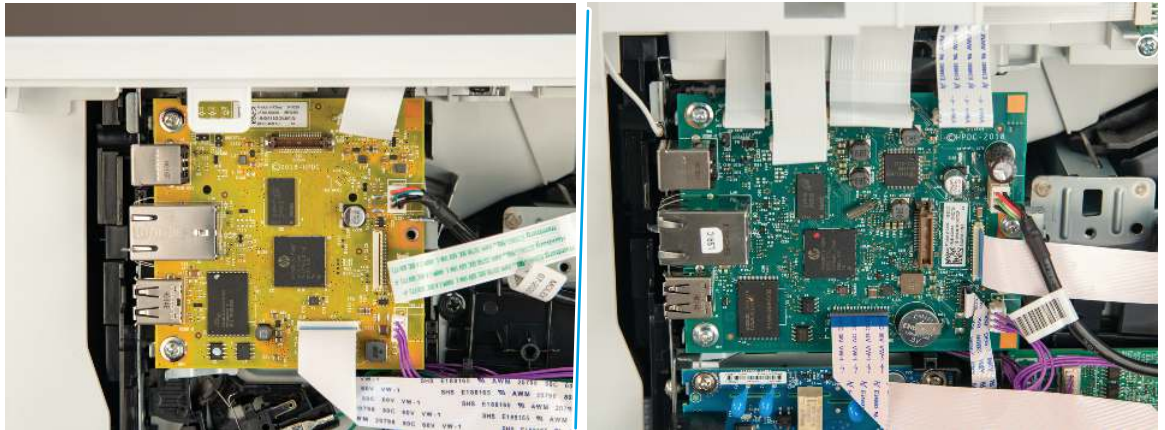
Figure 5-657 Disconnect all of the connectors (SFP/MFP)
