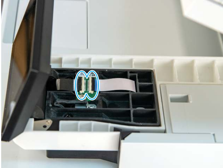
Figure 5-40 Disconnect two FFCs
