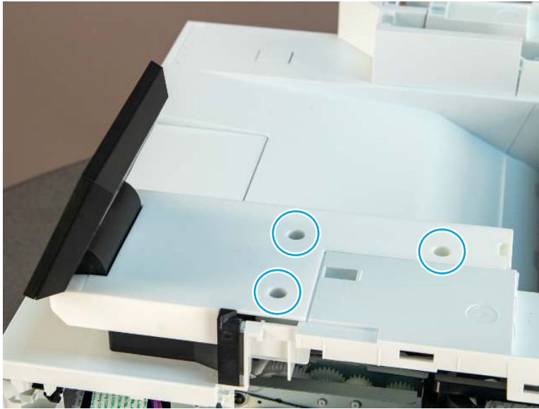
Figure 5-160 Remove three screws
