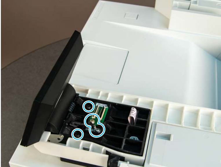
Figure 5-234 Remove four screws
