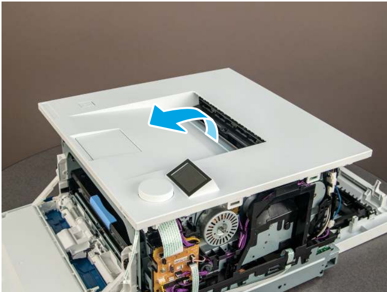
Figure 5-760 Remove the cover
