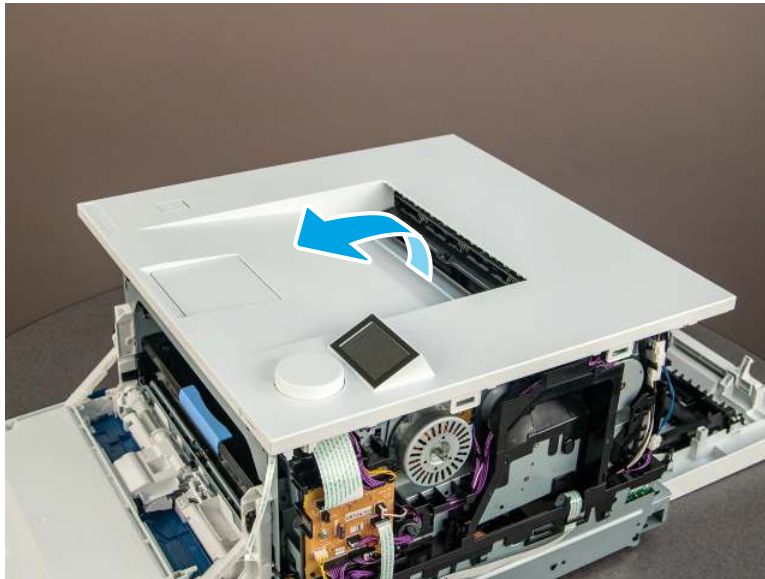
Figure 5-225 Remove the cover
