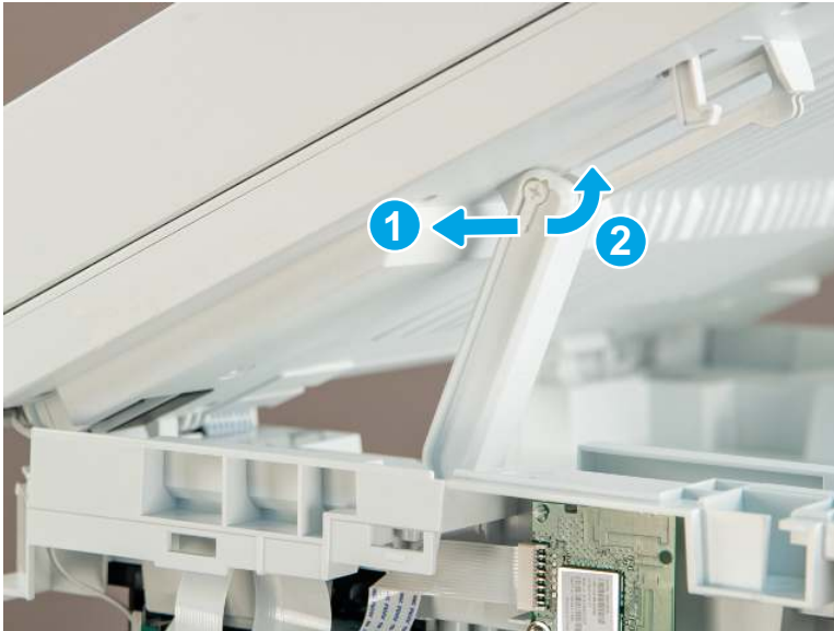
Figure 5-5 Release the slider pin
