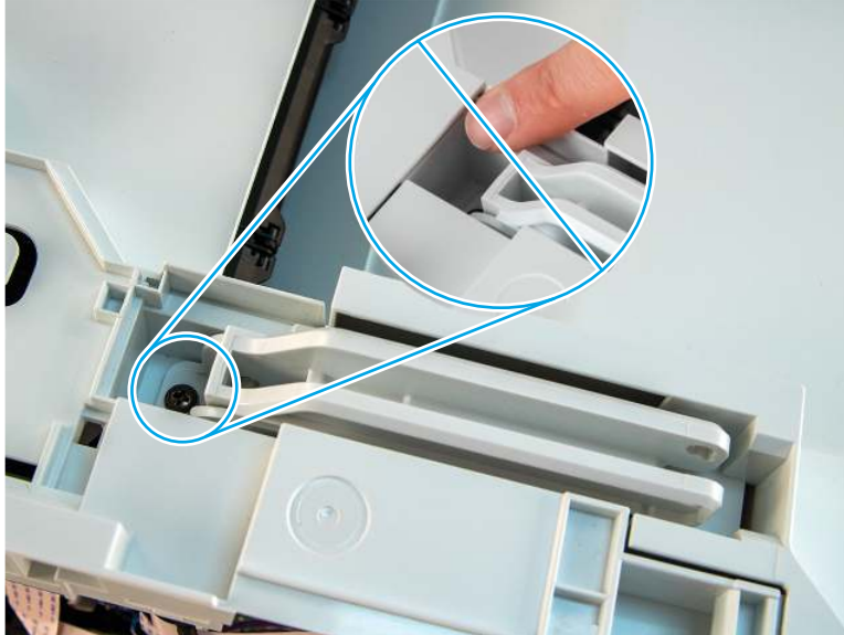
Figure 5-156 Remove one screw
