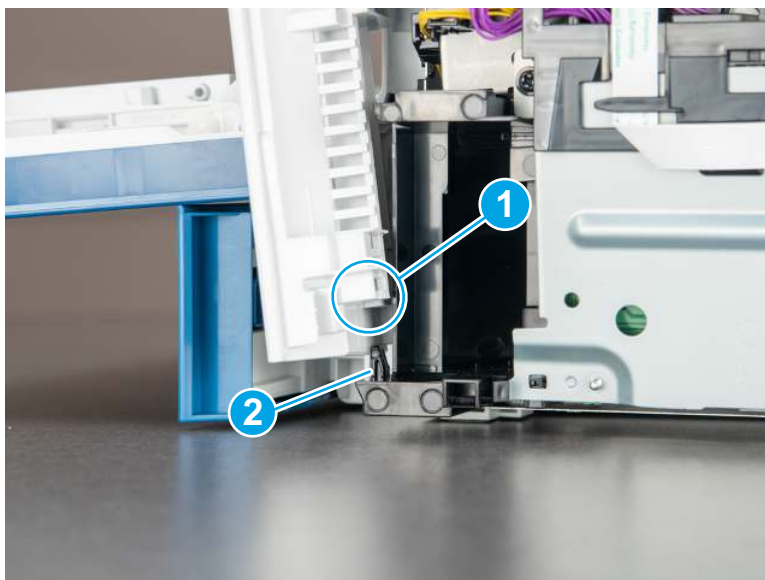
Figure 5-785 Cover alignment pins
