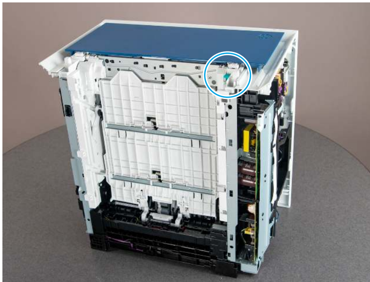
Figure 5-988 Release the assembly
