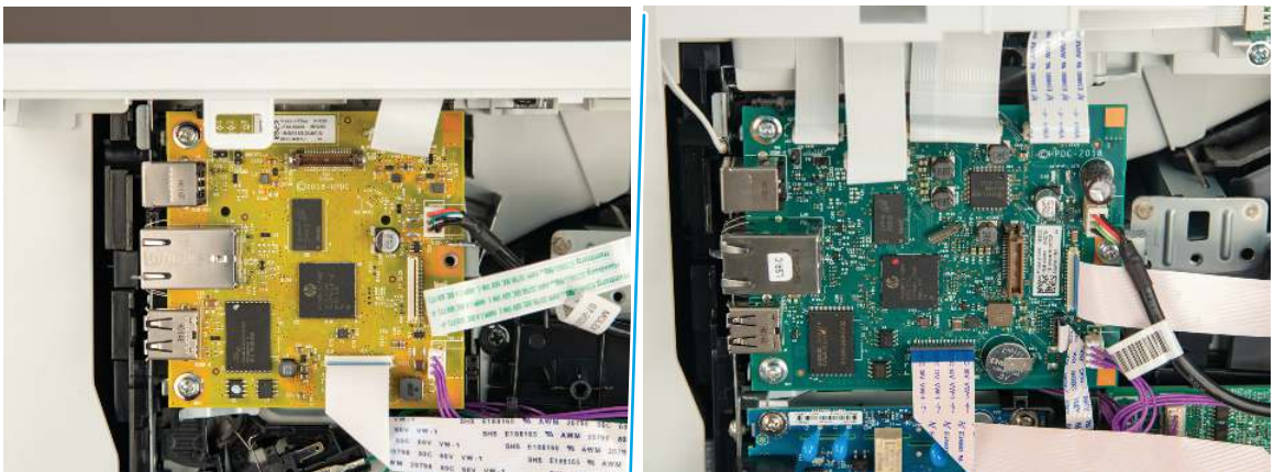
Figure 5-717 Disconnect all of the connectors (SFP/MFP)
