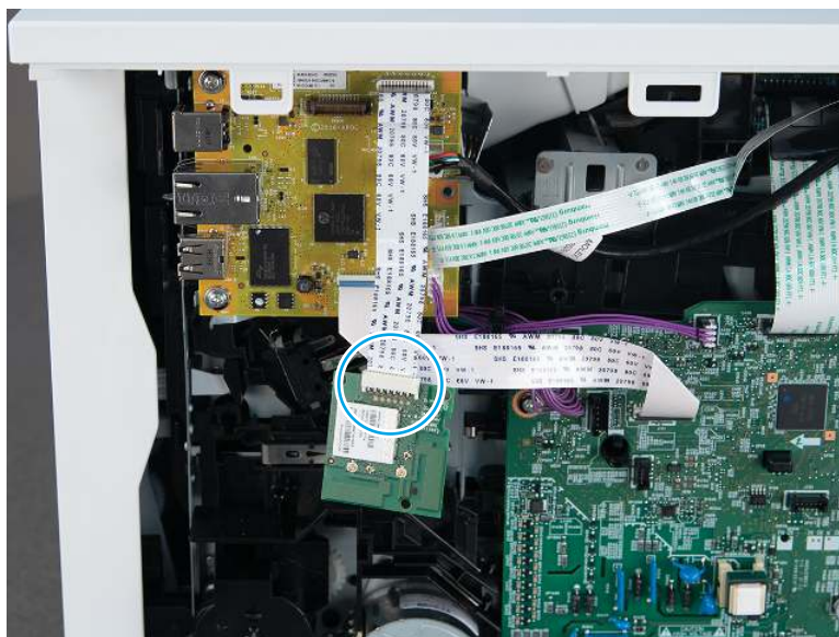
Figure 5-250 Remove the PCA
