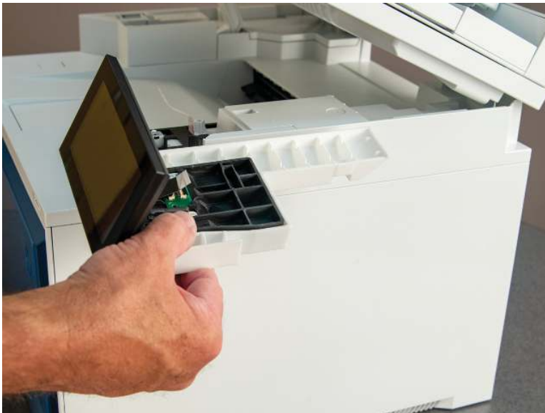
Figure 5-43 Remove control panel and mount base
