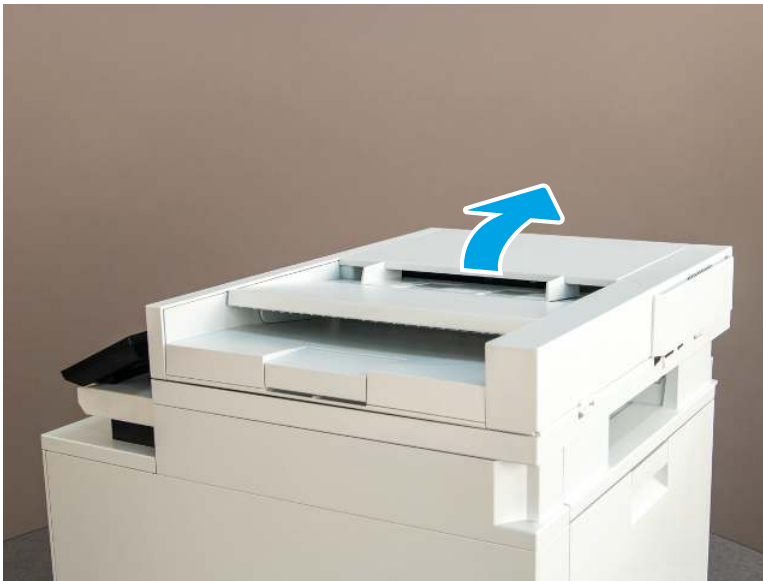
Figure 5-1 Open the cover
