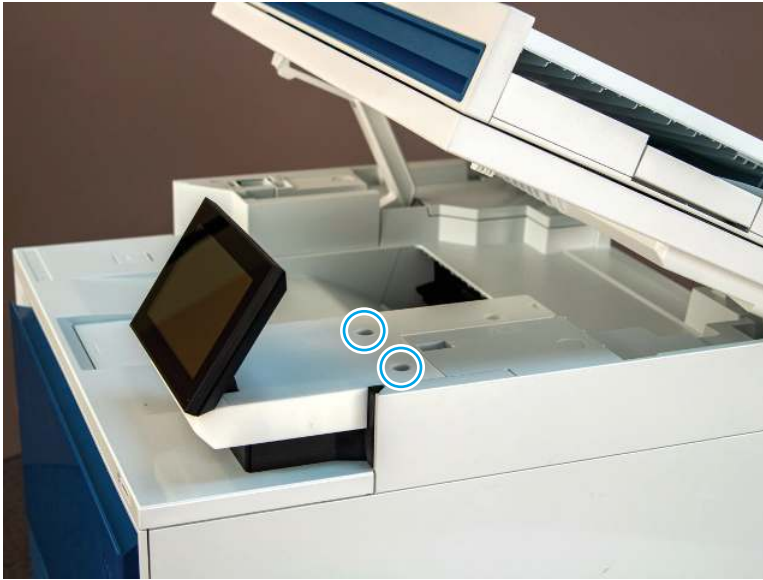
Figure 5-38 Remove two screws
