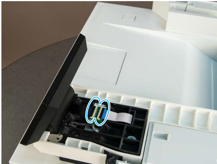
Figure 5-233 Disconnect two FFCs
