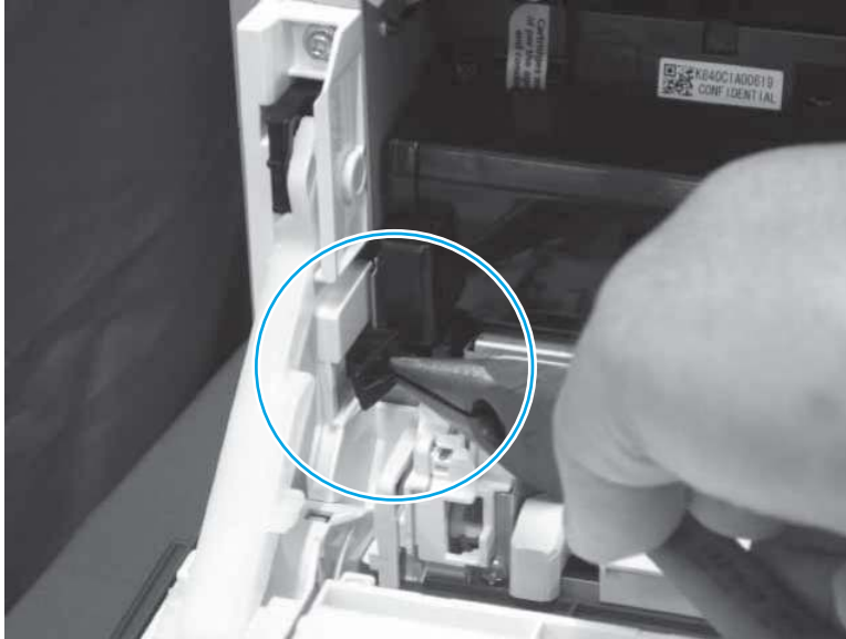
Figure 5-824 Remove the stopper (left side)
