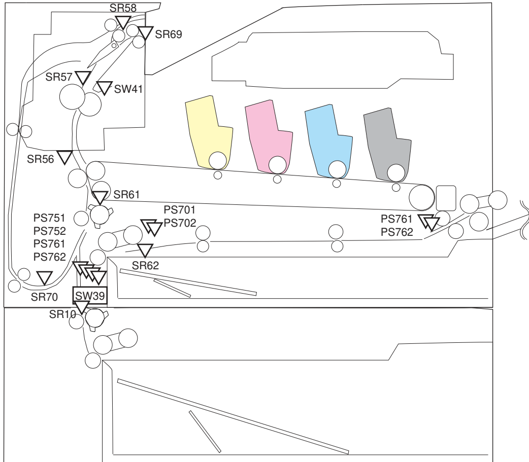
Figure 4-30 Sensors and switches (base printer)
