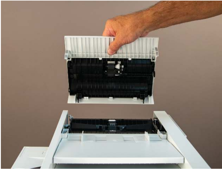
Figure 5-4 Remove the cover
