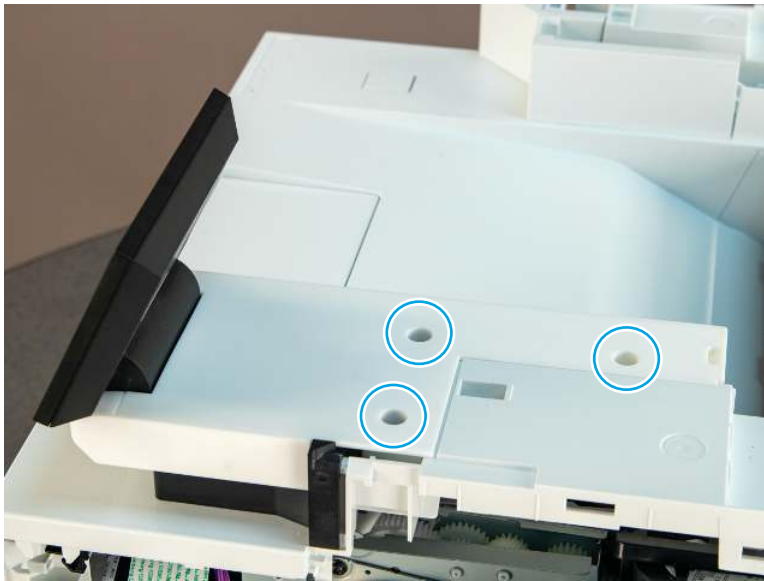
Figure 5-399 Remove three screws
