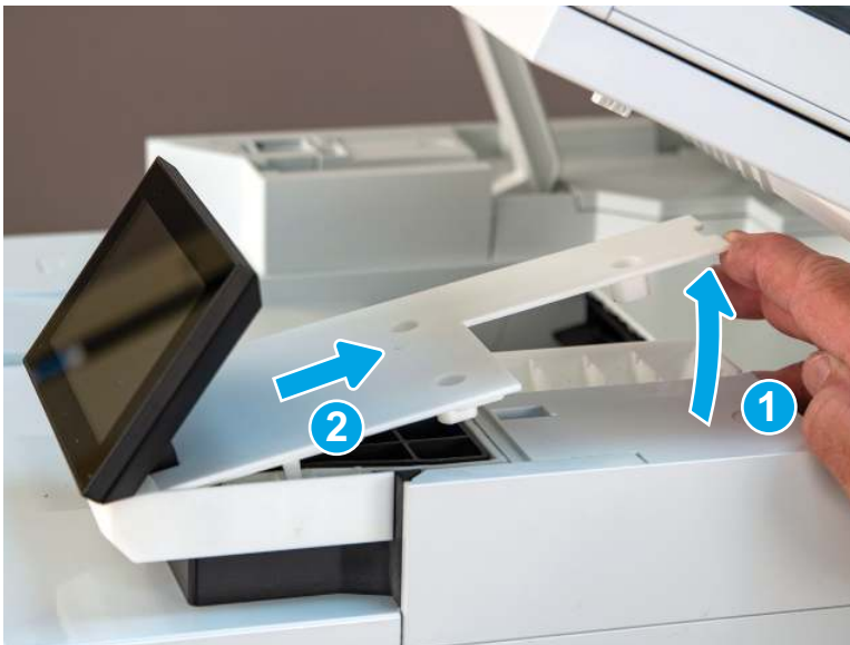
Figure 5-39 Remove the cover
