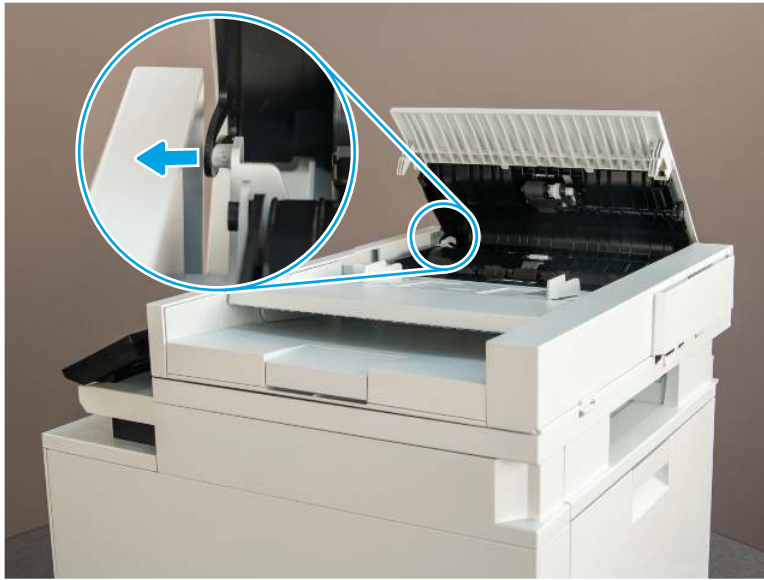
Figure 5-2 Release the clip
