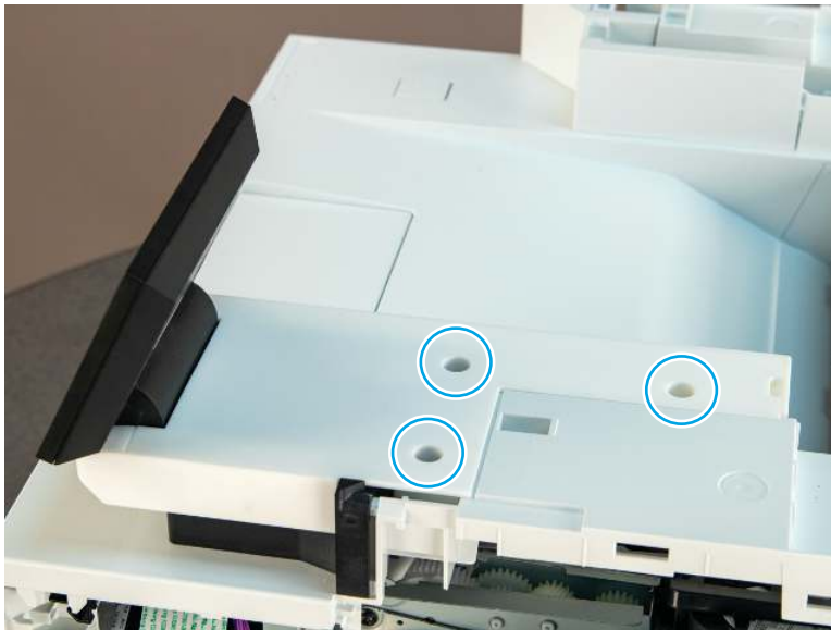
Figure 5-515 Remove three screws
