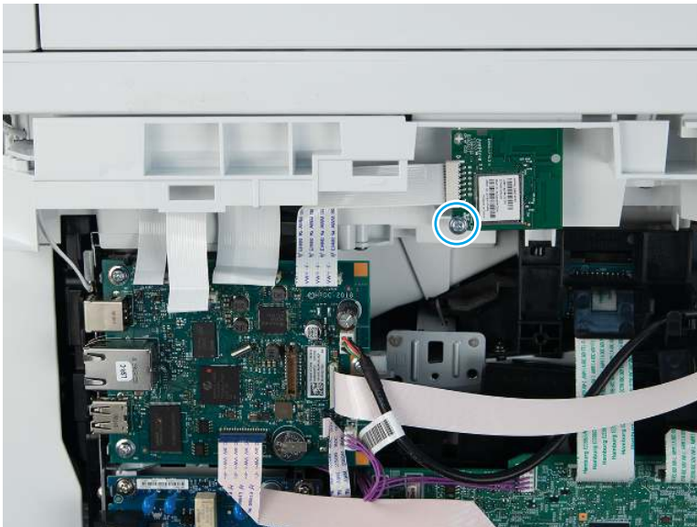
Figure 5-256 Remove one screw
