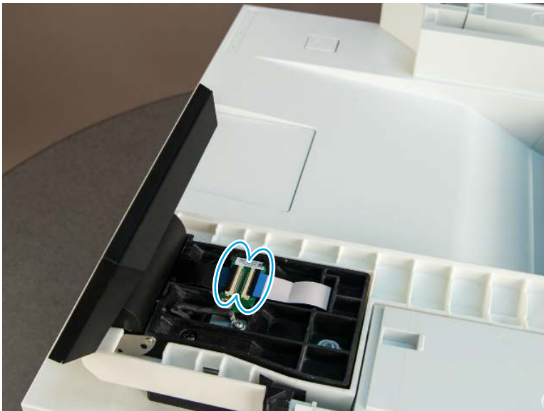
Figure 5-839 Disconnect two FFCs
