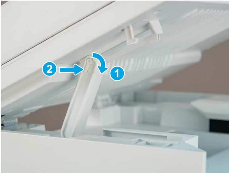
Figure 5-37 Reinstall the slider pin
