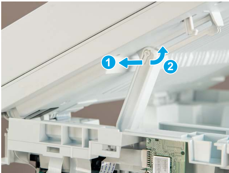
Figure 5-489 Remove the slider pin
