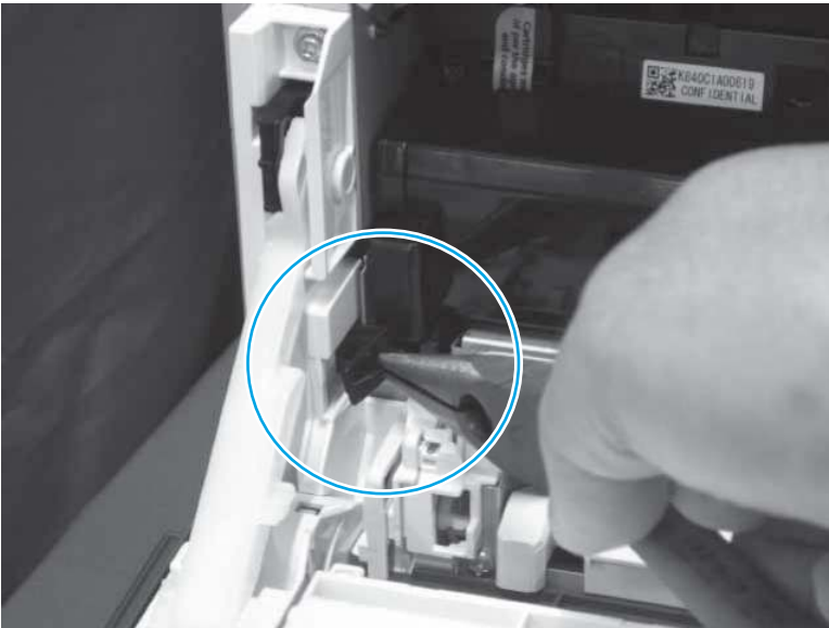
Figure 5-438 Remove the stopper (left side)
