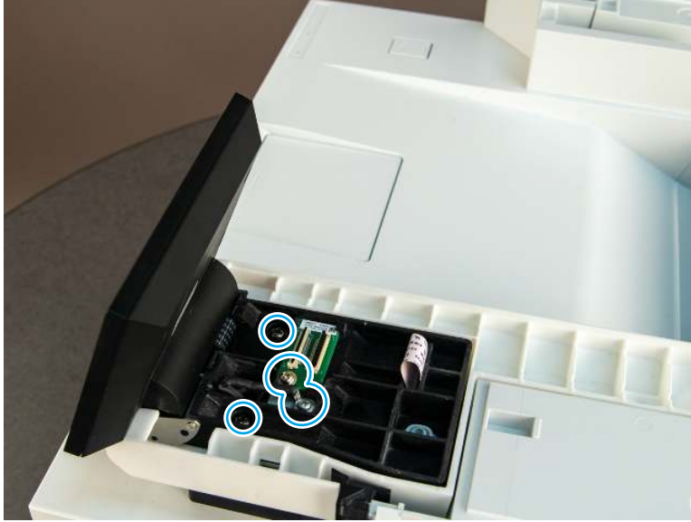
Figure 5-840 Remove four screws
