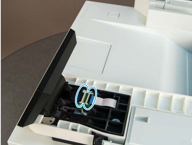
Figure 5-162 Disconnect two FFCs
