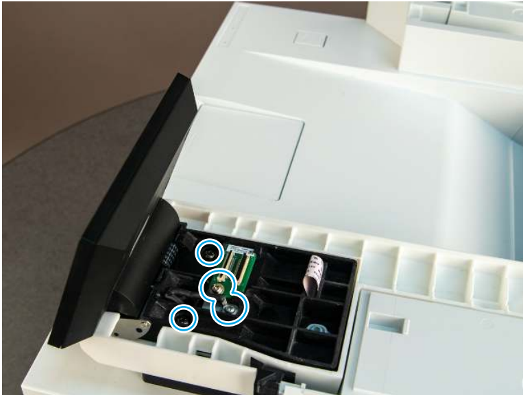
Figure 5-163 Remove four screws
