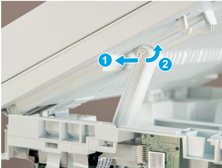
Figure 5-205 Remove the slider pin
