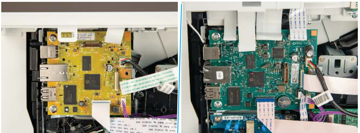
Figure 5-774 Disconnect all of the connectors (SFP/MFP)
