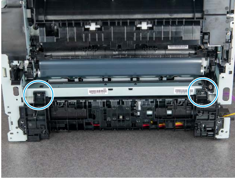
Figure 5-1060 Release two bosses
