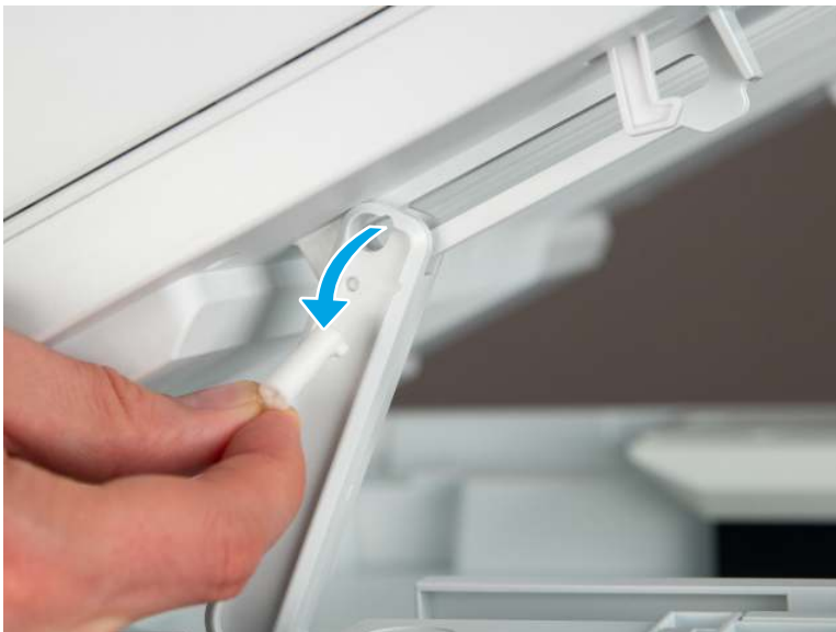
Figure 5-6 Remove the slider pin
