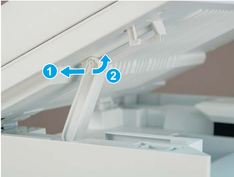
Figure 5-35 Remove the slider pin
