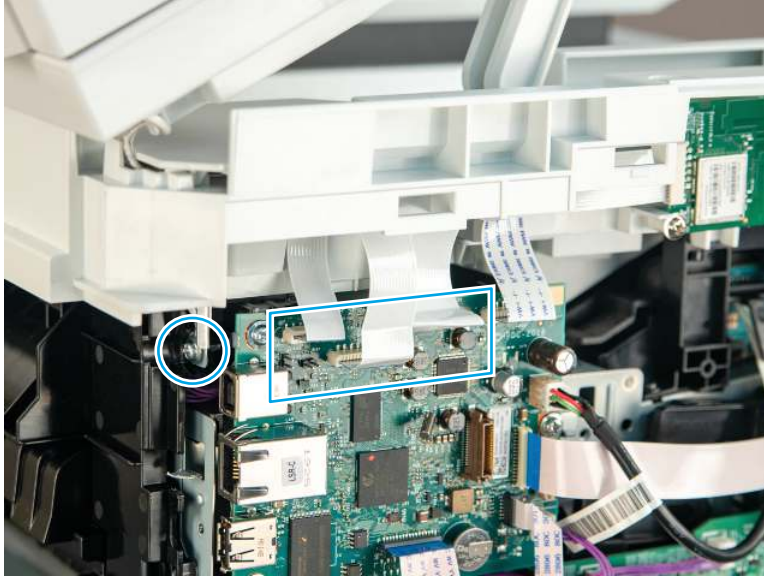
Figure 5-204 Disconnect FFCs and remove screw
