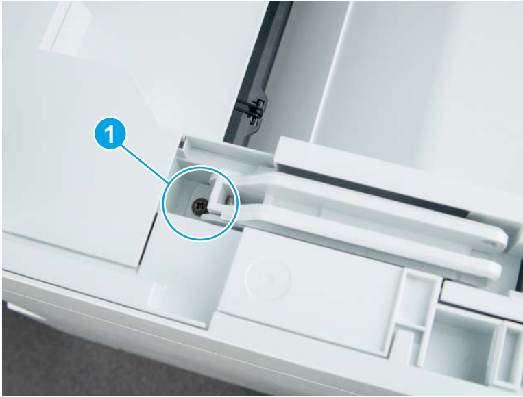
Figure 5-9 Remove one screw
