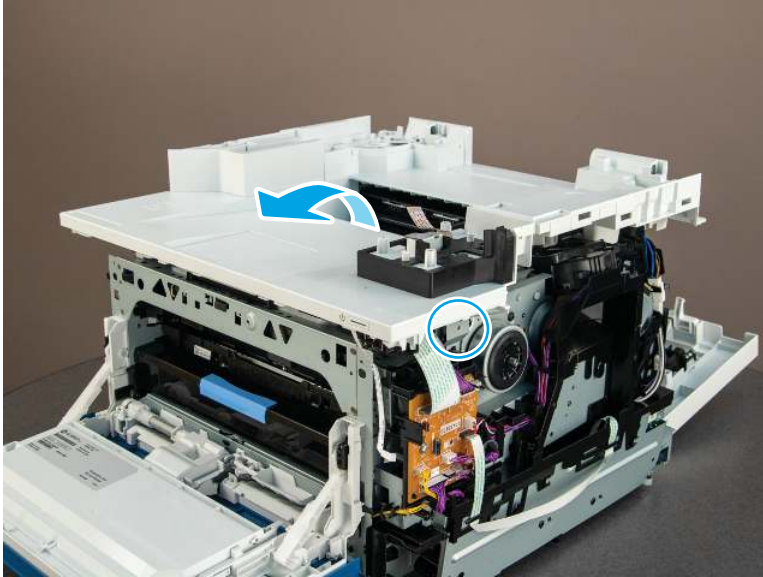
Figure 5-166 Remove the cover
