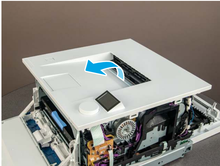
Figure 5-703 Remove the cover
