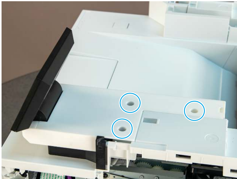
Figure 5-766 Remove three screws
