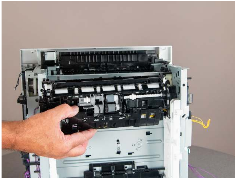
Figure 5-1137 Remove the feed upper guide assembly
