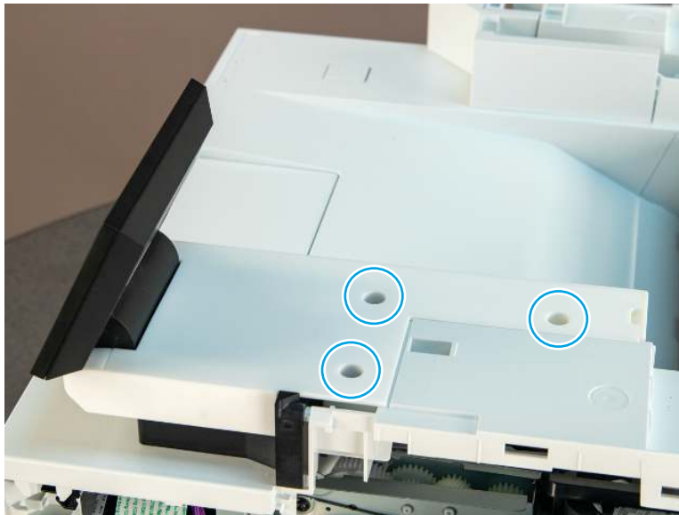
Figure 5-837 Remove three screws
