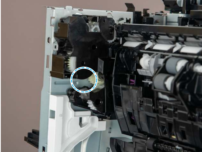
Figure 5-1130 Release one tab
