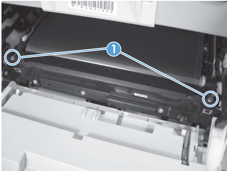
Figure 1-88 Remove the ITB (1 of 6)
