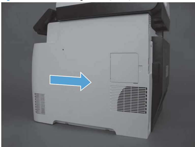
Figure 1-21 Remove the right cover (2 of 3)
