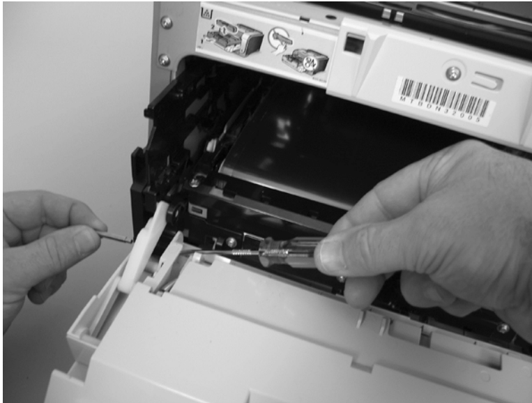
Figure 1-77 Remove the front-door assembly (2 of 10)
