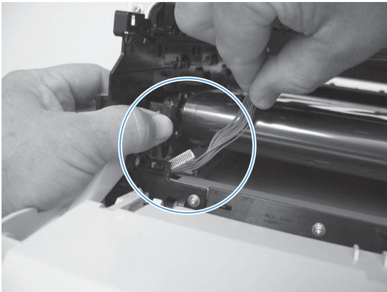
Figure 1-128 Reinstall the color-misregistration sensor assembly PCA (1 of 2)
