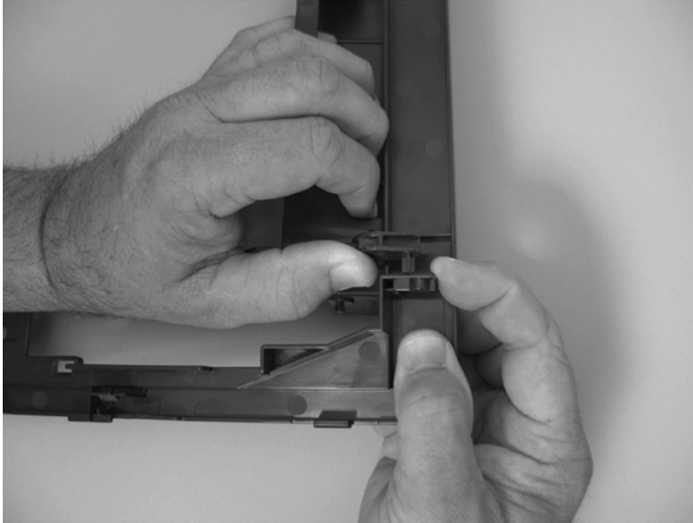
Figure 1-47 Remove the rear cover and feed guide (simplex product) (5 of 6)
