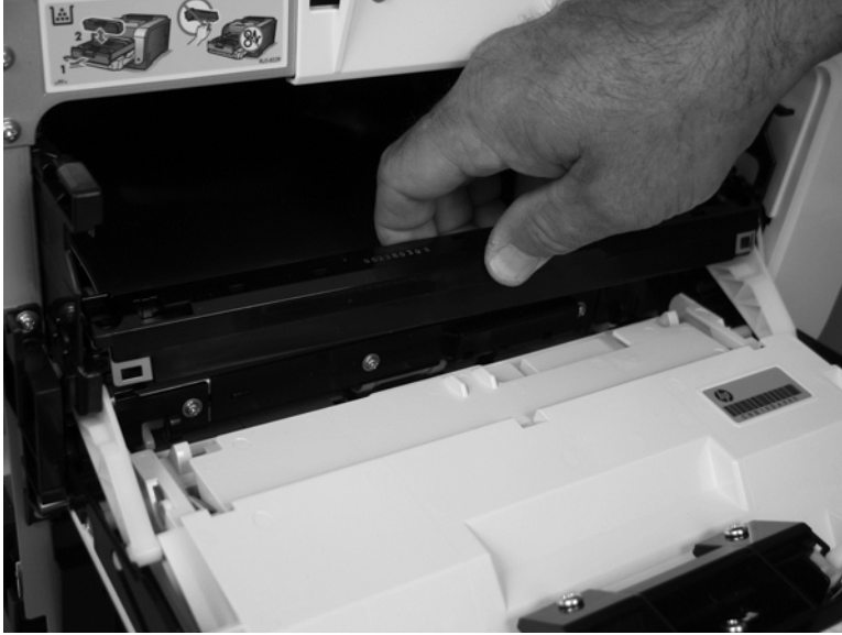
Figure 1-127 Remove the color-misregistration sensor assembly PCA (4 of 4)
