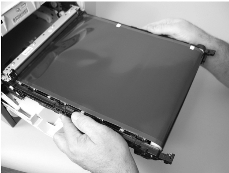
Figure 1-93 Remove the ITB (6 of 6)
