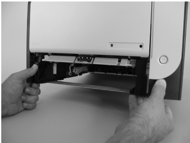
Figure 1-6 Remove the pickup roller (1 of 3)
