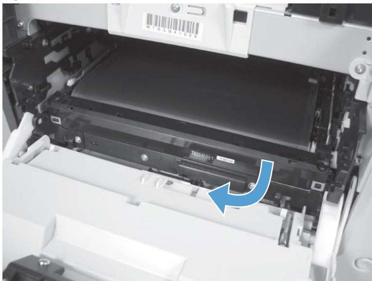
Figure 1-89 Remove the ITB (2 of 6)
