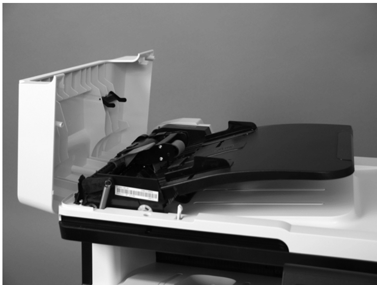
Figure 1-23 Remove the document feeder input tray (2 of 2)
