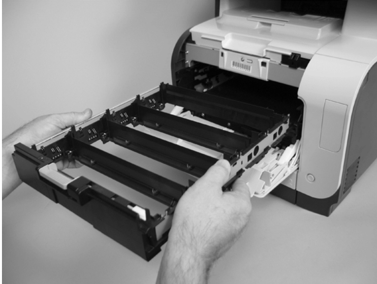
Figure 1-18 Remove the print-cartridge drawer (3 of 3)
