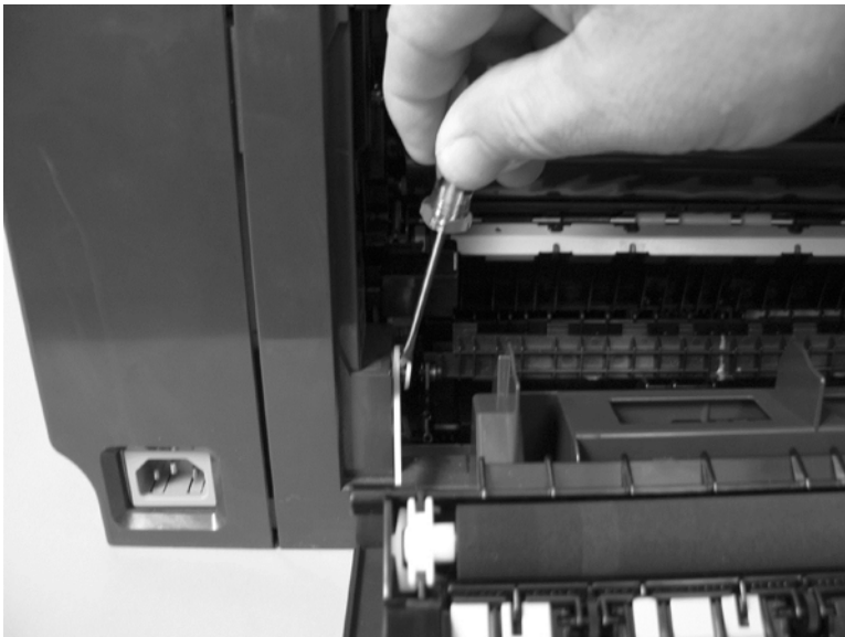
Figure 1-34 Remove the Rear-door stopper and link cap (simplex product) (2 of 2)
