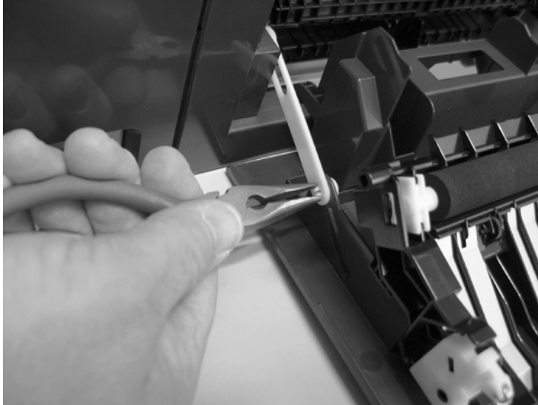
Figure 1-35 Remove the rear door (simplex product) (1 of 4)
