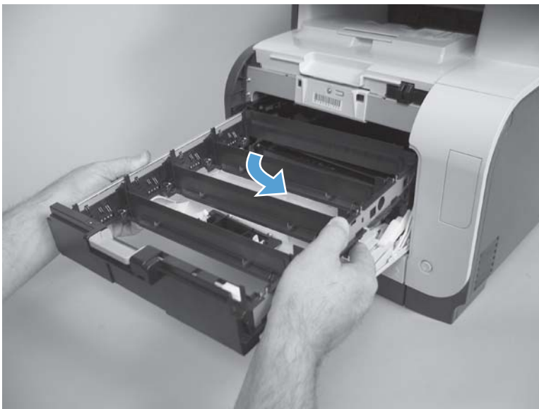
Figure 1-17 Remove the print-cartridge drawer (2 of 3)
