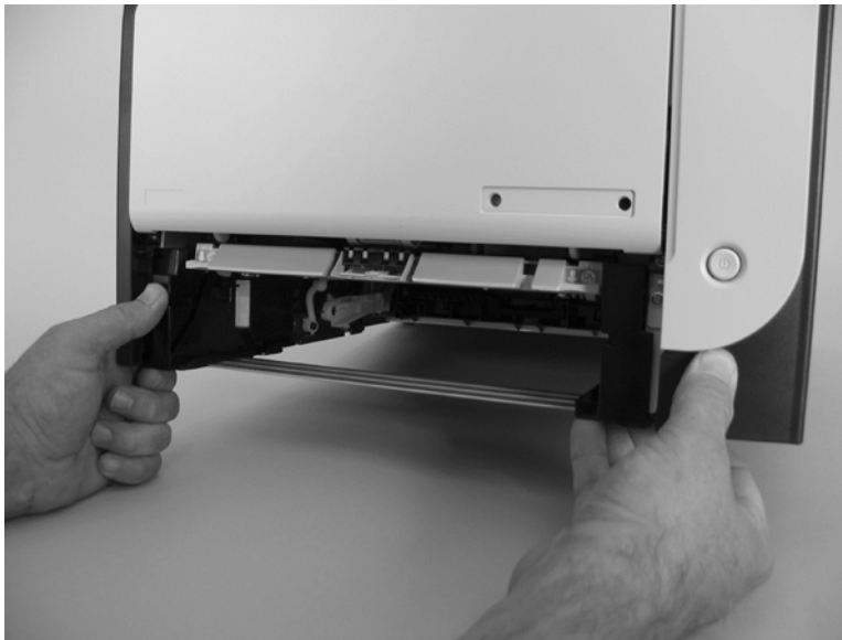
Figure 1-4 Remove the pickup roller (1 of 2)
