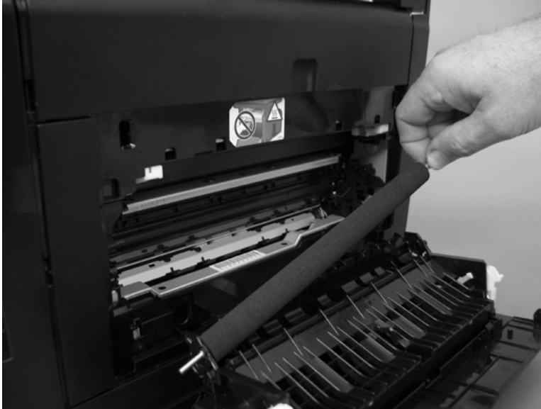
Figure 1-8 Remove the transfer roller (3 of 3)
