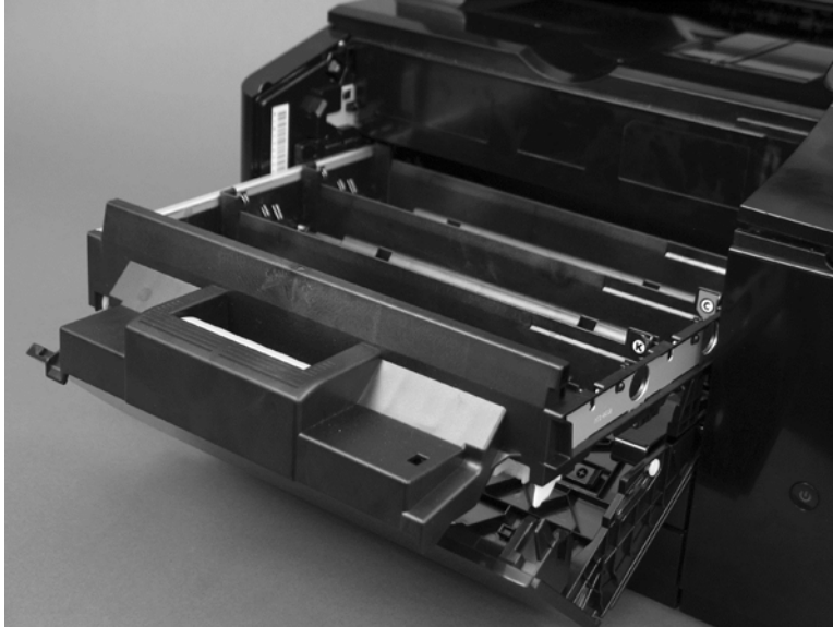
Figure 1-9 Remove the toner-cartridge drawer (1 of 4)
