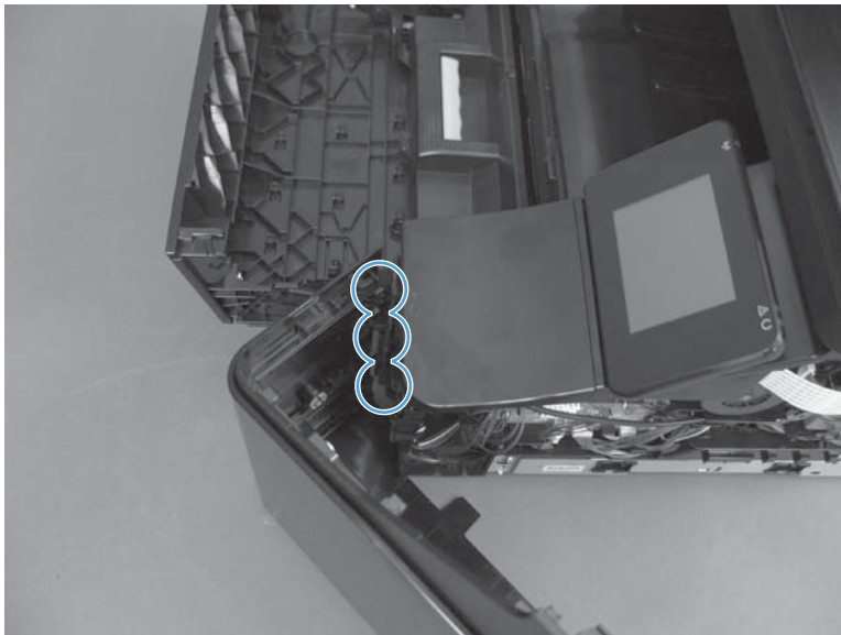
Figure 1-17 Remove the right cover (5 of 5)
