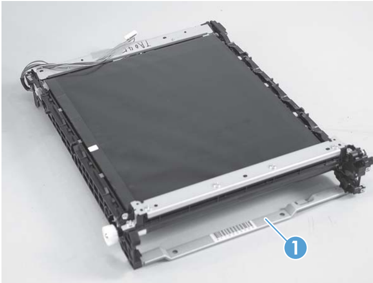
Figure 1-69 Reinstall the ITB (1 of 2)
