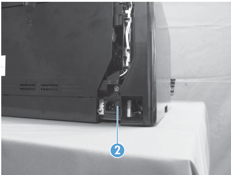
Figure 1-21 Remove the left cover (4 of 5)
