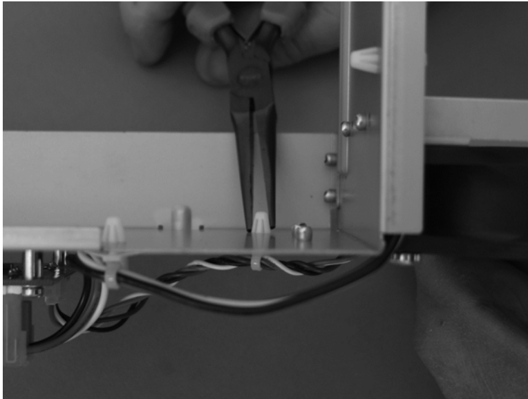
Figure 2-62 Remove the fan assembly (1 of 3)
