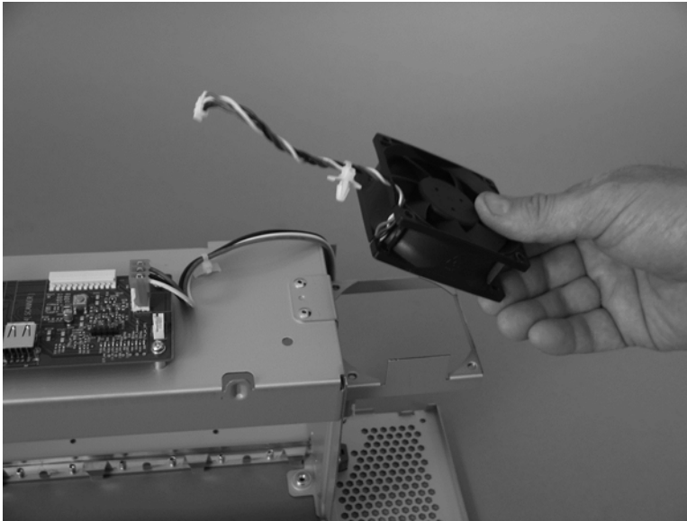
Figure 2-64 Remove the fan assembly (3 of 3)
