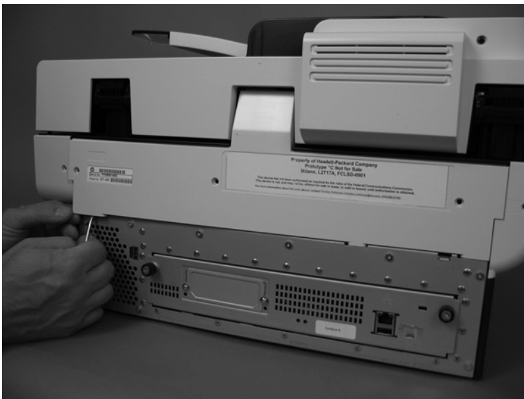
Figure 2-33 Remove the flatbed scanner and ADF assembly (3 of 7)
