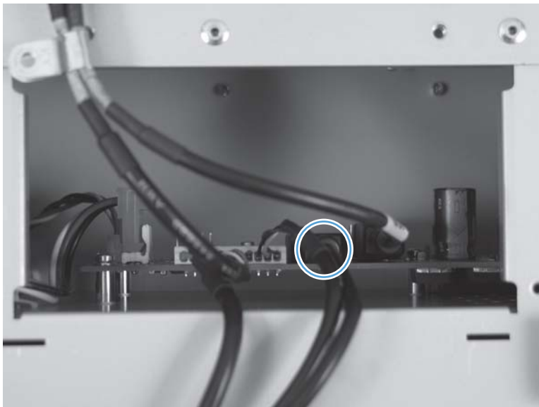
Figure 2-48 Remove the control-panel cable (1 of 3)
