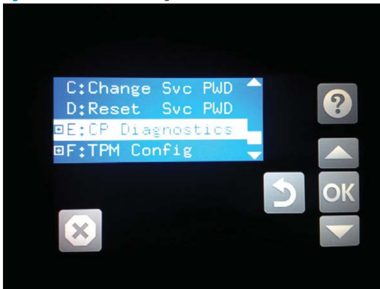
Figure 2-27 Access the CP Diagnostics menu
