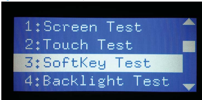
Figure 2-33 Open the softkey test
