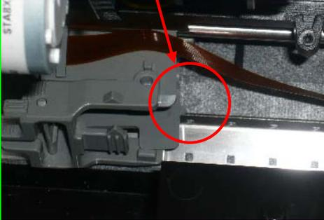
(13) Fix the IM Holder Shaft with the Shaft Stopper.
