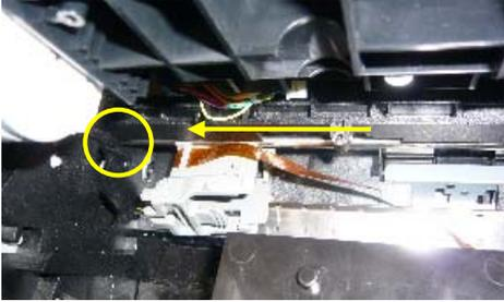
Ⓕ Check that the tab on the Holder Unit and the edge of the IM Holder Rail are aligned.
