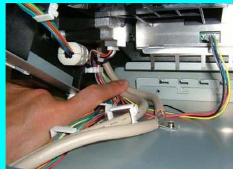
When closing the CT Base, check that the CCD-B Cable touches the rising edge of the plate and does not touch the Feed Motor Unit 2.
