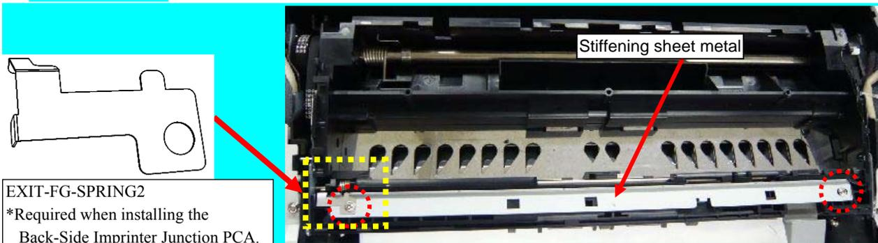
(8) Attach the Back-Side Imprinter Junction PCA and EXIT-FG-SPRING2 to where the stiffening sheet metal was fixed with three tapping screws.
