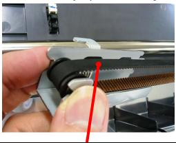
Remove the belt from the tension pulley
