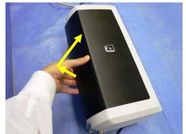
(2) Lifting up the Inverter from the groove, disconnect the three connectors connected on the Inverter, and remove the Inverter.
