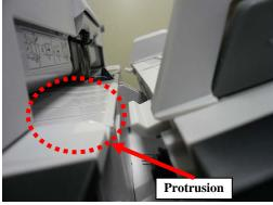
Note: Make sure that there is no gap between the Chute ASSY and the scanner after installation.
