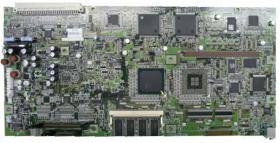
Control PCA for fi-6770/fi-6770A PA03576-D807 Control PCA for fi-6750S PA03576-D832
