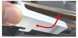
(7) Remove the tension pulley from the bracket groove, and then the belt from the tension pulley.
