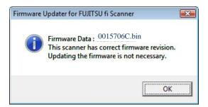
7) When firmware update is completed, the following appears. Click on "OK" to terminate the update procedure.
