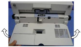
(4) Place the scanner so that the connector inlet faces up, and remove the seven screws A that secure the PCA unit.
