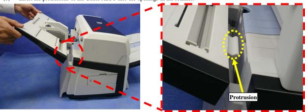
Note: Make sure that there is no gap between the Chute ASSY and the scanner after installation.
