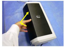
(2) Lifting up the Inverter from the groove, disconnect the three connectors connected on the Inverter, and remove the Inverter.
