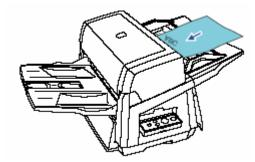
Note: If the documents to scan are long, slide the Paper Chute Extension out from the ADF Paper Chute up to the position where the documents can be fully supported.
