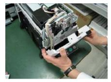
Note 4: When installing the Panel unit A, rotate the clear plastic part to fix.
