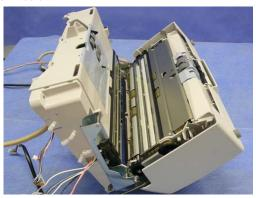
(4) With a flat-blade screwdriver, unlatch the claws at both sides of the Background unit F, and then remove the Background unit F.
