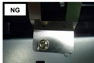
Gap between aligning position: 1mm or less
