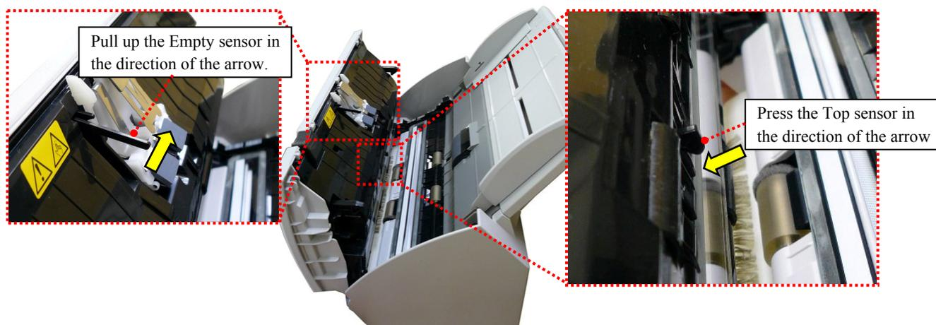
2. Let go of levers of the Top sensor and the Empty sensor.
