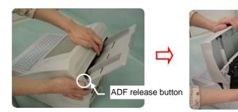
3) Pull the ADF paper chute obliquely upward (toward rear of the scanner) to remove.
