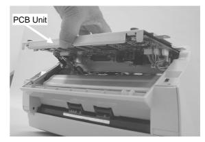
Disconnect seven connectors, which are connected to the PCB UNIT, and remove the PCB UNIT. To replace the CONTROL PCA, go to Section 5-12.
