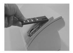
3) Take out the PANEL PCA and disconnect one connector from the PANEL PCA.
