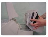
After removing two Guide Blocks, pull out the scanner section to the back.
