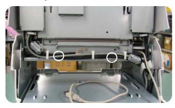
6) Bump the KB UNIT against the front of the scanner, and raise the KB UNIT to remove it.
