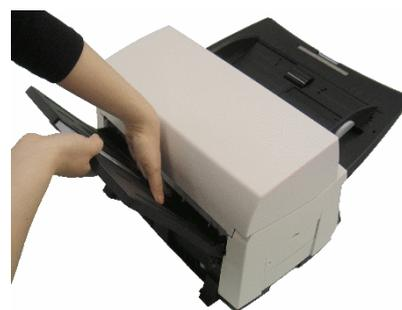
3. Remove the cover (black) located under the stacker.
