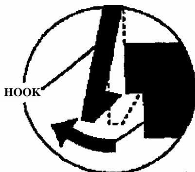
Do not use excessive force when removing parts held in place with hooks.
