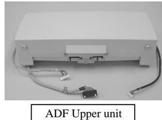
Note: Be careful not to damage the glass on the ADF Upper unit.
