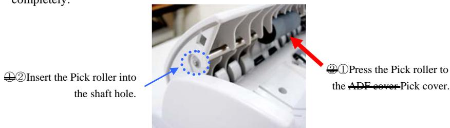
2. Pinch the Roller lock inwardly with two fingers and place it to the original position to fix the Pick roller
