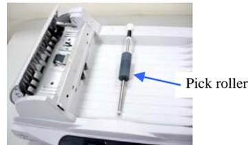
5. When the left end of the Pick roller is removed from the shaft hole, remove the Pick roller.
