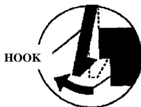
Do not use excessive force when removing parts held in place with these hooks.
