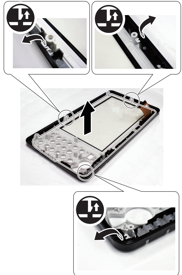
9. Remove the Touch Panel PCB. • 3 Claws
