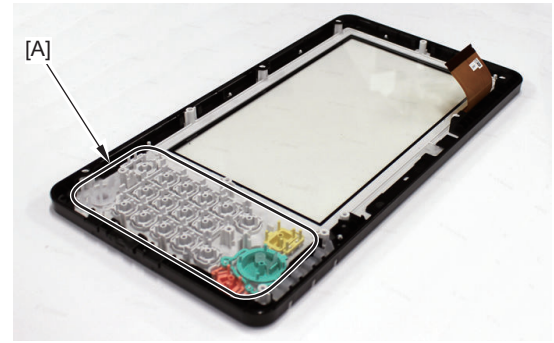
9. Remove the Touch Panel PCB. • 3 Claws
