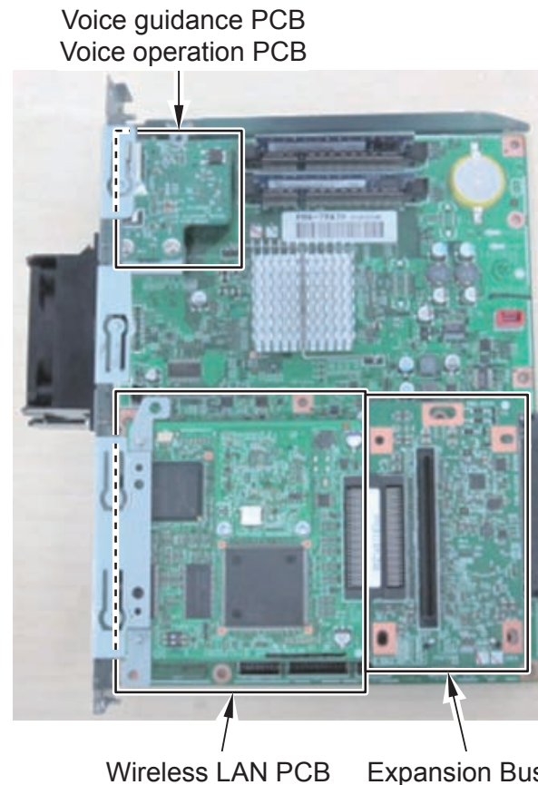
Main controller PCB1
