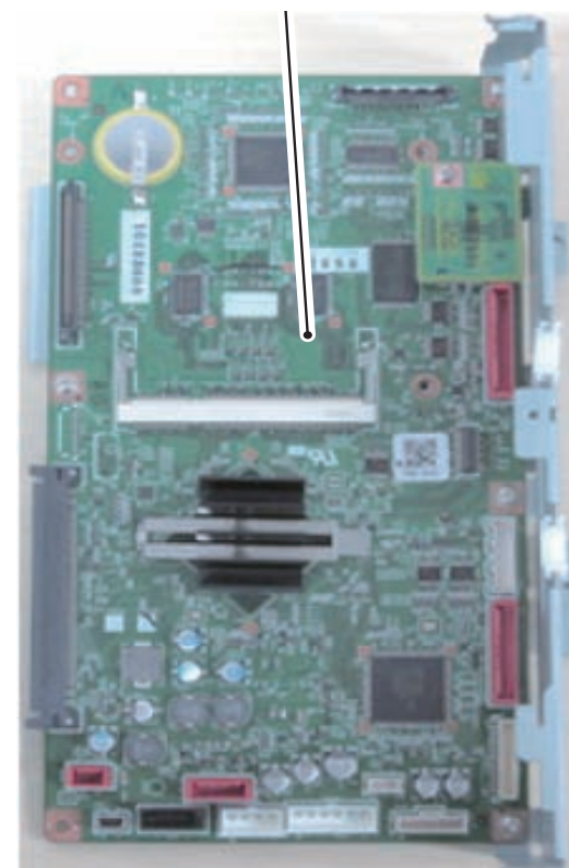
Main Controller PCB 2
