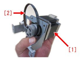
[Note] When replacing to the paper delivery drive assembly (L), be sure to also replace the timing belt [B] at the same time that is included in the set. 110F jam occurs when using the old type timing belt [A] as the number of teeth of the new type is different from the old type originally attached to the engine.
