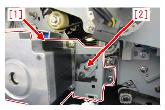
6) Tighten the screw which was loosened in the step 5) and attach the rear cover. [ Service parts]
