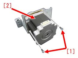
4) After attaching the timing belt [2] that is included in the set to the paper delivery drive assembly (L) [1] with the motor attached, attach the whole thing to the machine using the 2 screws removed in the step 2).
