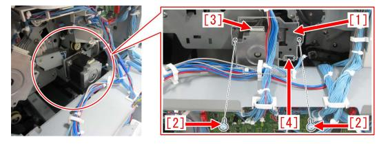
3) Remove the 2 screws [1] and then remove the motor [2]. Then, attach the motor to the paper delivery drive assembly (L) which is included in the set. To attach the motor, use the 2 screws that were previously removed [1].
