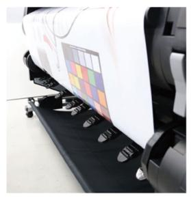
Tension is optimized by the Active Roll Brake Unit.
