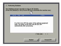
When the shutdown process completes, the main power switch of the machine switches to the " $\bigcirc$ " side automatically.
