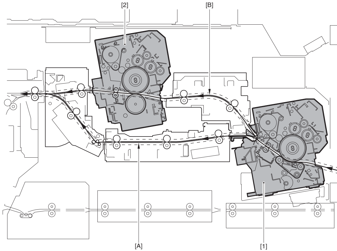
[1] Primary fixing assembly (belt fixing) [A] Single feed path [2] Secondary fixing assembly (roller fixing) [B] Tandem feed path
