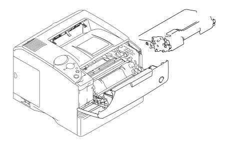
5) Remove the separation plate ASSY.
