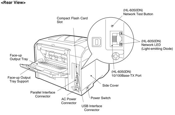
\*The printer illustration is based on HL-6050DN.
