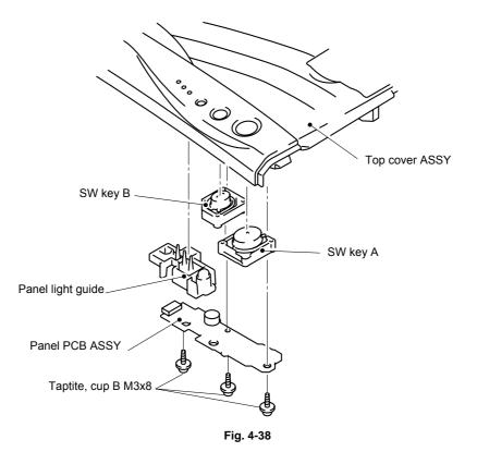
(6) Remove the panel light guide 2 and the diffusion film from the panel guide.
