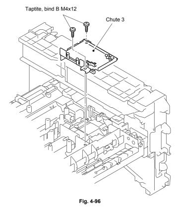
(22) Remove the two bind B M4x12 Taptite screws, and then remove the chute 3.
