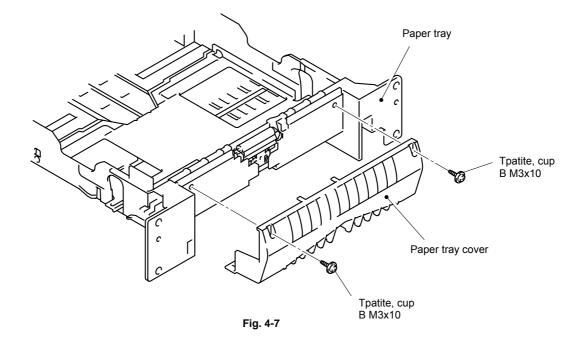
(5) Remove the two Taptite, cup B M3x10, and then remove the paper tray cover.
