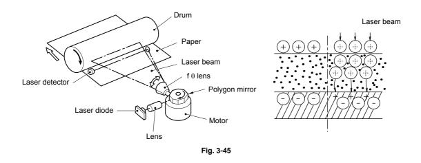
The area exposed to the laser beam is the image to be printed. The surface potential of the exposed area is reduced, forming the electrostatic image to be printed.
