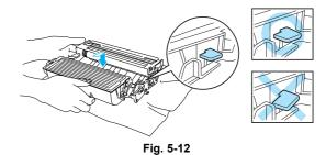
(7) Clean the primary corona wire inside the drum unit by gently sliding the blue tab from right to left several times. Return the tab to the home position before you put the drum unit back in the printer. If you do not, printed pages may have a vertical stripe.
