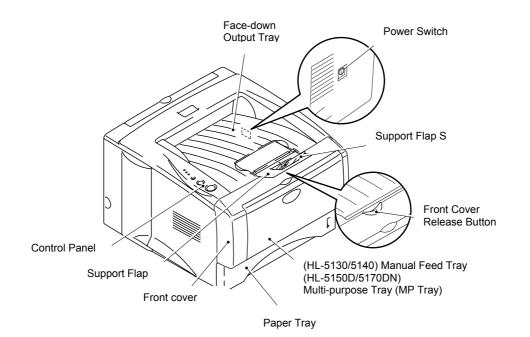
\*The printer illustration is based on HL-5150D and HL-5170DN. Fig. 1-1
