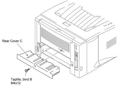
3) Remove the bind B M4x12 Taptite screw, and then remove the rear cover C.
