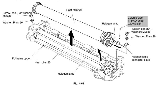
When re-assembling the halogen heater lamp, ensure that the direction of the halogen heater lamp is correct referring to the figure above.
