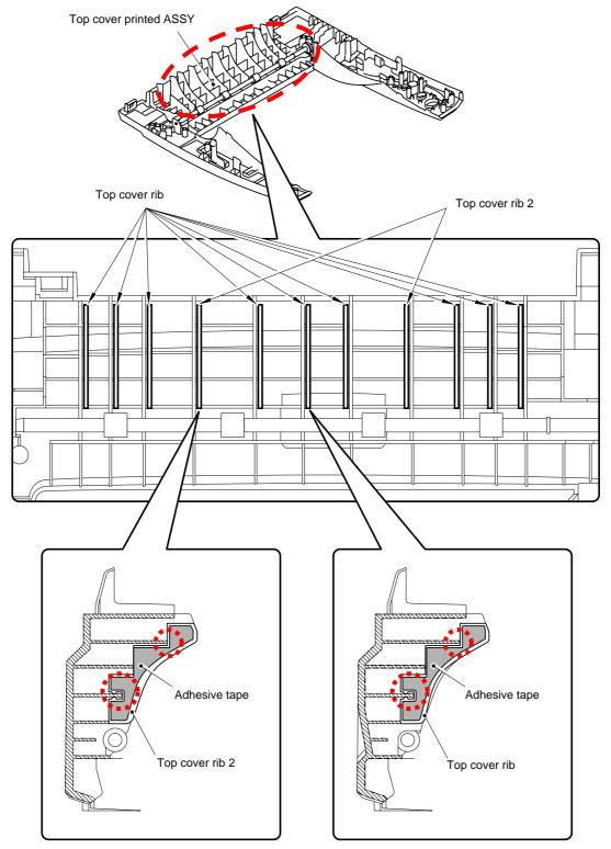
NOTE: Pay attention to the location circled by red color dotted line to attach the additional ribs against the ribs of the Top cover printed ASSY.
