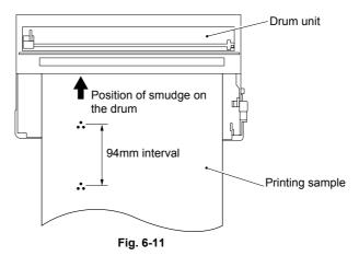
(2) Turn the drum gear by hand while looking at the surface of the photosensitive drum.
