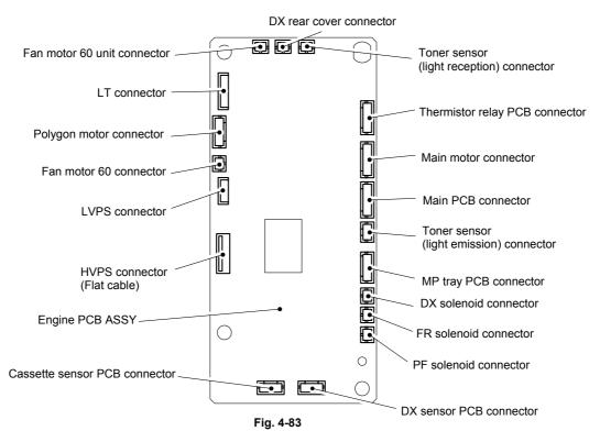
(2) Remove the two bind B M4x12 Taptite screws, and then remove the engine PCB ASSY.
