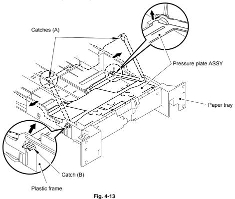
(16) Unhook the pressure plate spring from the plastic hook to remove the two pressure plate springs.
