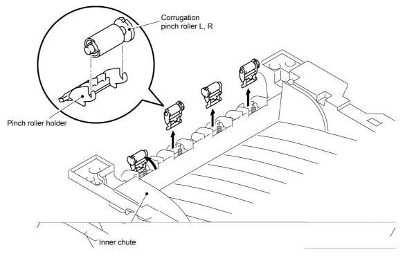
(9) Remove the corrugation pinch roller L, R and pinch roller holder.
