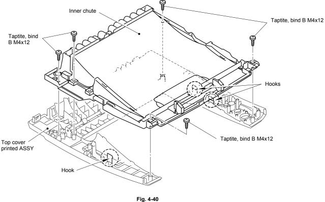
(7) Remove the five bind B M4x12 Taptite screws, and then remove the inner chute.
