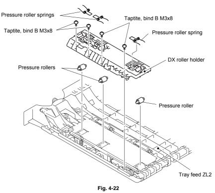
Set pressure roller, and assemble pressure roller spring after assembling DX roller holder.
