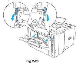
(5) Put the envelopes in the MP tray so that they touch the back of the tray and remain under the maximum paper height guides on both sides of the tray. Do not put more than 3 envelopes in the MP tray at any one time, or it may cause a jam.
