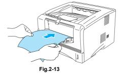
NOTE: Make sure the paper is neatly stacked and in the proper position on the manual feed tray. If it is not, the paper may not be fed correctly, resulting in a skewed printout or a paper jam.
