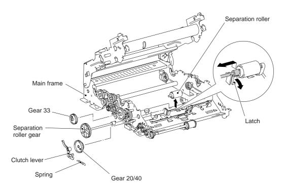
(4) As shown below, release the latch with the tip of a flat screwdriver and slide the separation roller support to the right and lift it up.
