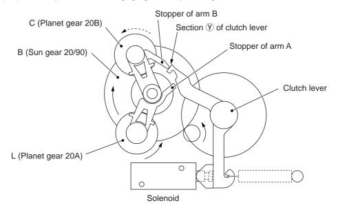
Arm B Blocked by Section ③ of Clutch Lever
