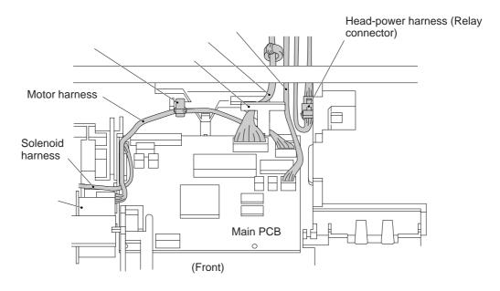
(6) Remove four screws "b" and lift up the main frame. "b" Main coverMain frame
