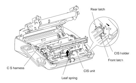
(4) Remove the CIS holders R and L as shown below.
