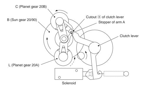
Arm A Locked by Cutout ® of Clutch Lever
