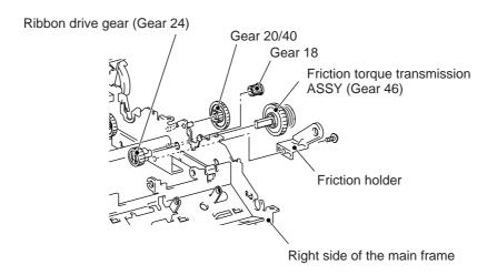
(4) At the inside of the right rear side of the main frame, remove the retaining ring E3 and then take out the slip gear 40, friction pad, and back tension spring.
