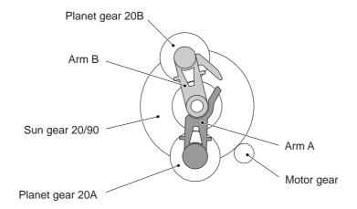
**Planetary Gear System**
