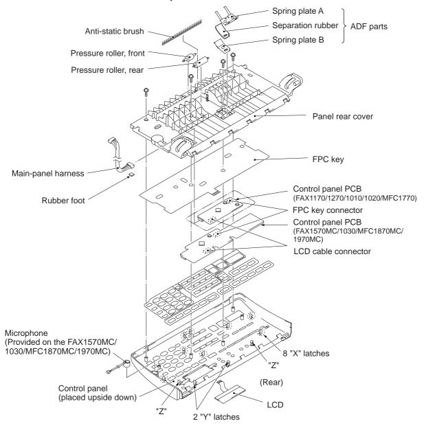
(8) To take out the LCD, remove the control panel PCB and the FPC key in step (6). As shown below, insert the tip of a flat screwdriver under clamp "D" in the direction of arrow F and push up clamp "D" slightly to release the LCD from clamp "C." In the same way, insert the screwdriver under clamp "A" to release the LCD from clamp "B."
