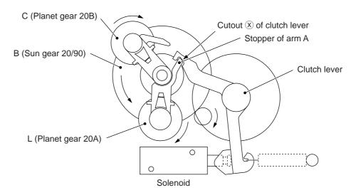
Arm A Locked by Cutout (X) of Clutch Lever
