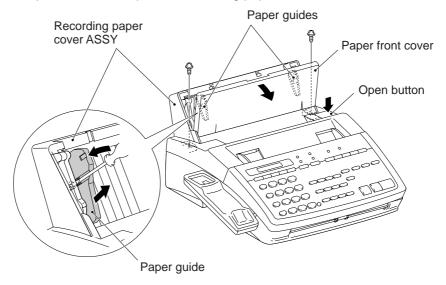
(5) Lift up the rear of the recording paper cover ASSY and take it out to the front.
