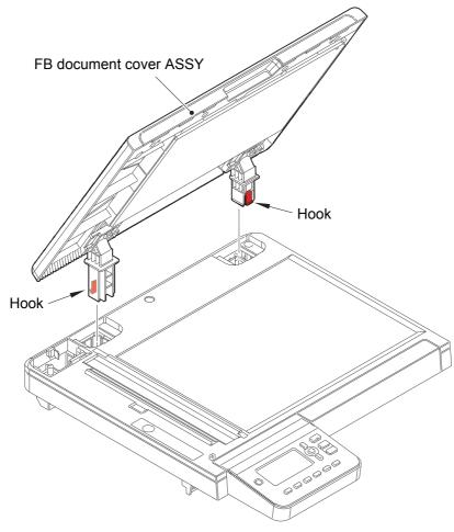
(2) <u>**Remove**</u> > DCP hinge base L, DCP hinge arm L
