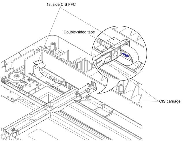
Harness routing: Refer to "1. 1st side CIS FFC".
