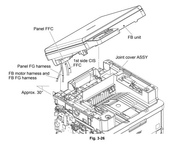
Harness routing: Refer to "1. 1st side CIS FFC, 26. Panel FFC, Panel FG harness (For models with 2-line LCD), 12. FB motor harness, FB FG harness".
