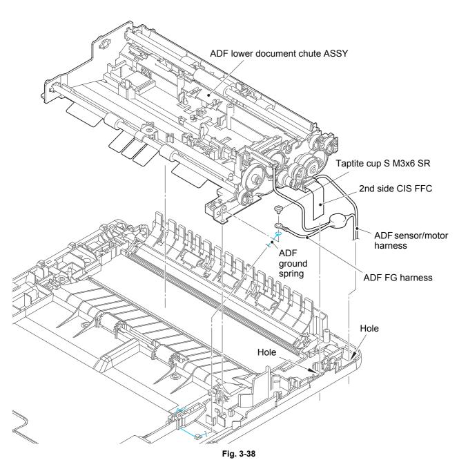
Harness routing: Refer to "3. ADF sensor/motor harness (For models with ADF), ADF FG harness".
