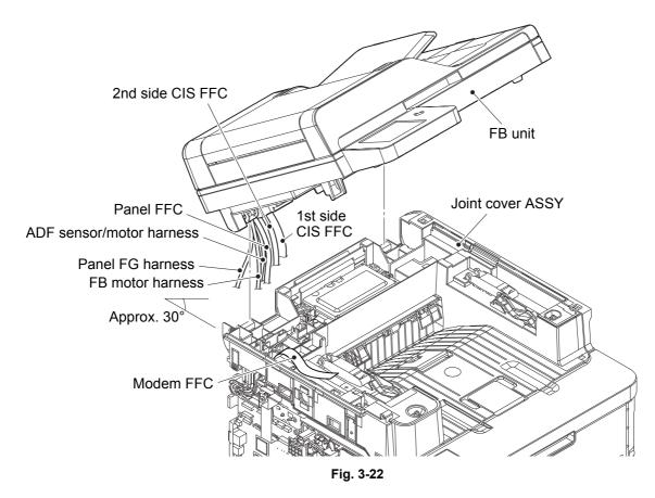
Harness routing: Refer to "2. 2nd side CIS FFC (For models with ADF), 1. 1st side CIS FFC, 22. Modem FFC, Modem FG harness L, Modem FG harness R, 25. Panel FFC, Panel FG harness (For models with touch panel), 12. FB motor harness, FB FG harness, 3. ADF sensor/ motor harness (For models with ADF), ADF FG harness".
