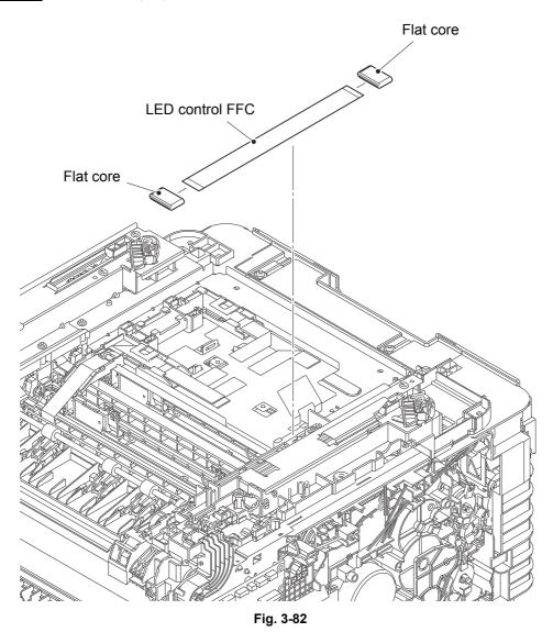
Harness routing: Refer to "16. LED control FFC, LED FG harness".
