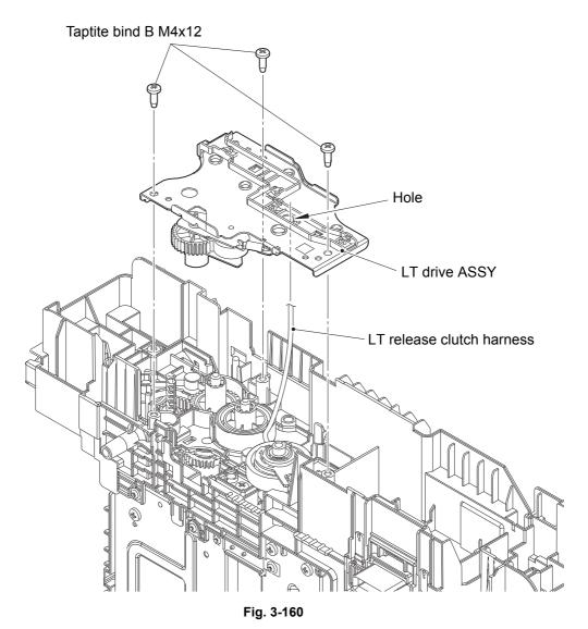
Harness routing: Refer to "20. LT release clutch harness".
