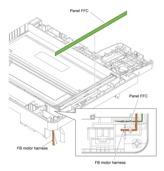
Harness routing: Refer to "25. Panel FFC, Panel FG harness (For models with touch panel), 26. Panel FFC, Panel FG harness (For models with 2-line LCD)".
