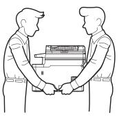
If you use a Lower Tray, DO NOT carry the product with the Lower Tray, as you may be injured or cause damage to the product because it is not attached to the Lower Tray.
