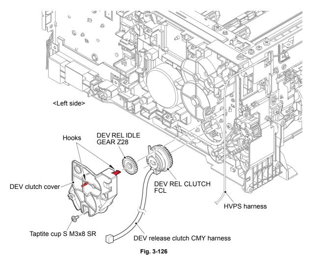
Harness routing: Refer to "6. DEV release clutch CMY harness, 14. HVPS harness".
