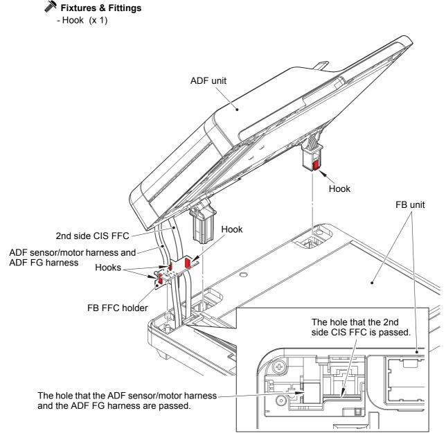
• Pull out the 2nd side CIS FFC, the ADF sensor/motor harness and the ADF FG harness
