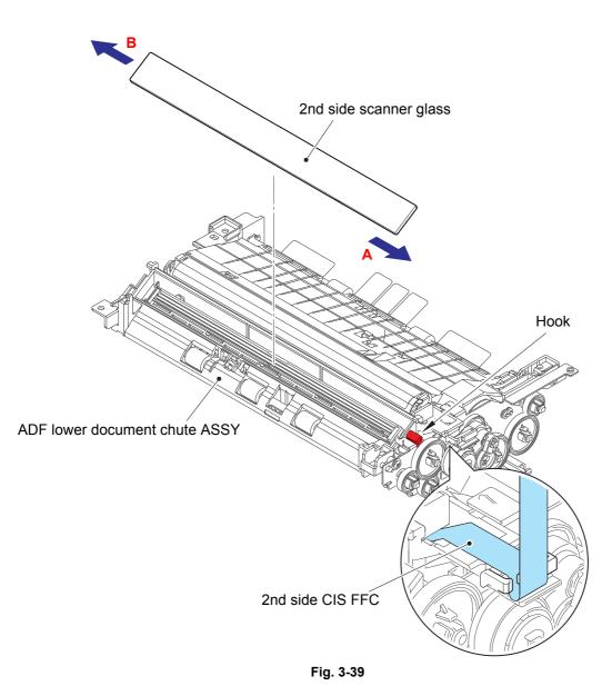
Harness routing: Refer to "2. 2nd side CIS FFC (For models with ADF)".
