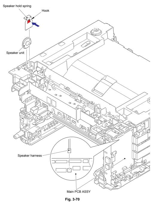
Harness routing: Refer to "6. Speaker unit, Modem (Main PCB side)", "7. Speaker unit, Modem (LVPS side)".
