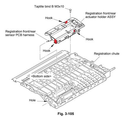
Harness routing: Refer to "2. Top side of the registration chute".
