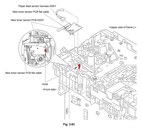
Harness routing: Refer to "3. Left side of the machine", "5. New toner sensor PCB ASSY".
